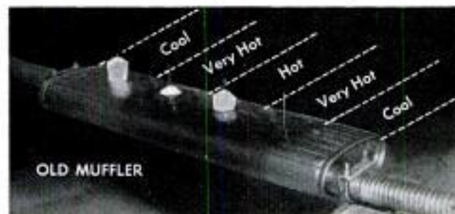
Above, old design melts candles unevenly. Below, the new muffler has even heat distribution, melts evenly
