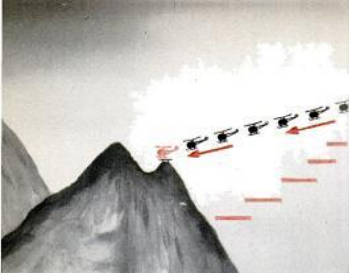
Steadily decreasing speed and altitude in approach, the Agar method permits zero ground-speed landing
