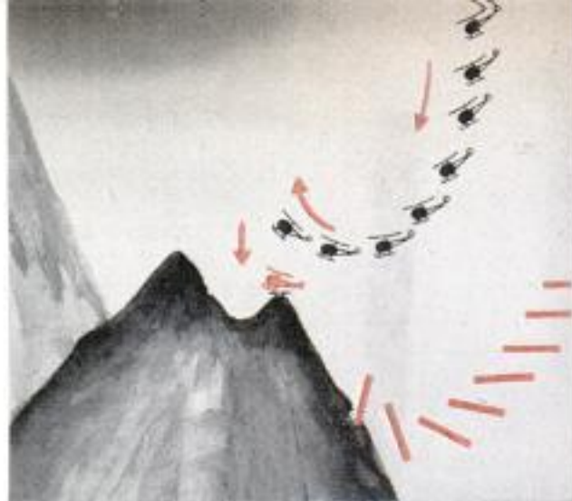
"Flare out" landing requires a vertical sloop, putting strain on the engine and making crash possible
