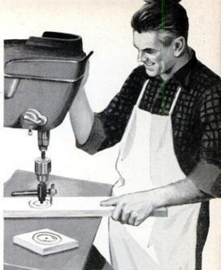
4. Above, long pieces of stock can be hand-held when using circle cutter, small pieces are clamped to table for safety. 5. Below, wooden rings are cut by using disk as jig to center holes, cut to inside diameter of rings, under circle cutter. Cutter is readjusted for outside diameter of rings and second cut is made
