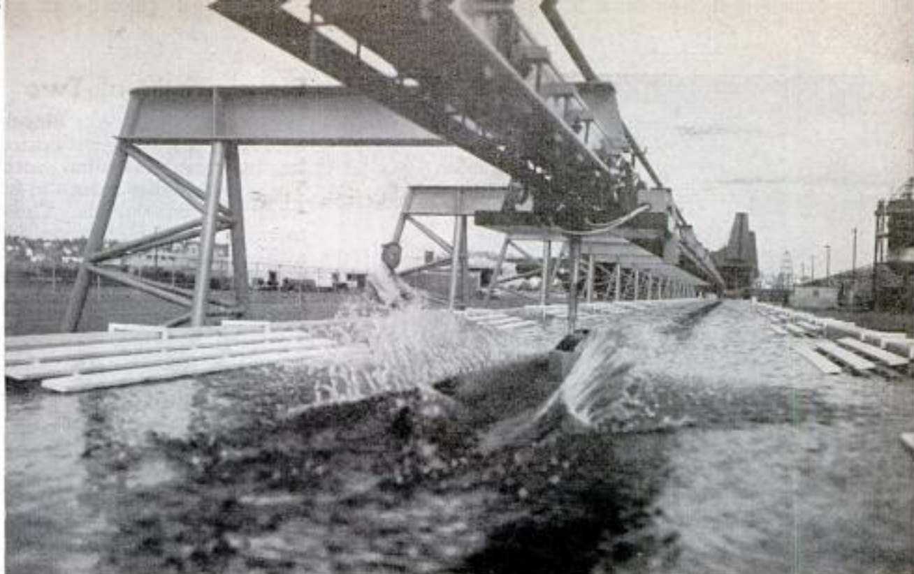
Seaplane hulls can be tested at speeds up to 68 miles per hour in Convair's new hydrodynamics laboratory
