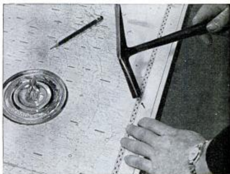
Below, frame is attached to mounted map with finishing nails. Heads of the nails are set below the surface and holes filled
