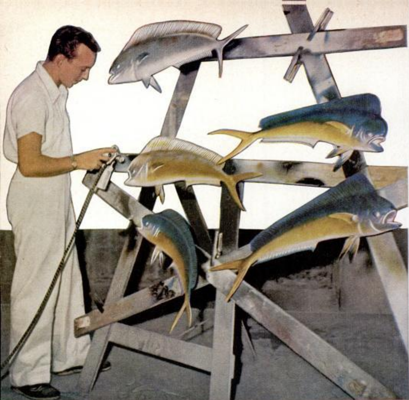
Painting is done with an airbrush, followed by touch-up by hand. Right, varying shades make red snapper difficult to paint
