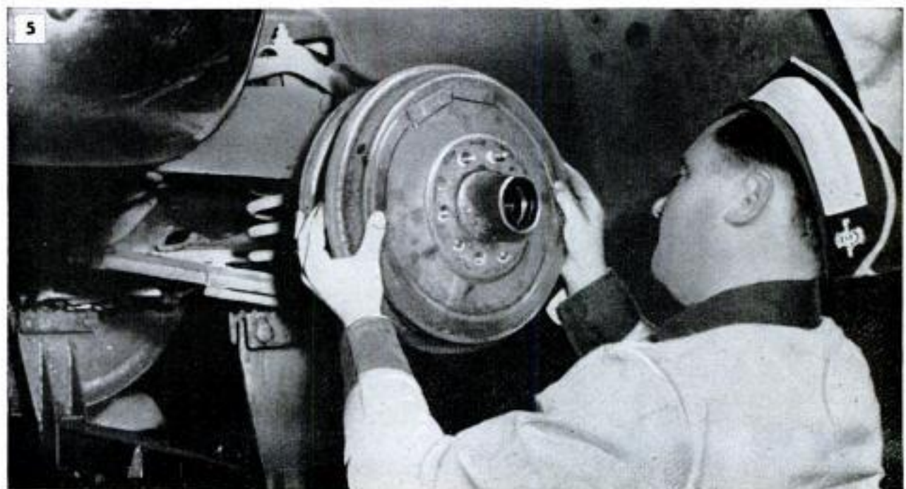
With drums reinstalled, brakes are bled and adjusted so there is no drag, good pedal. Below, front-wheel bearings are repacked before drums are reinstalled. In latter operation, care is taken not to use an excess of grease which may run onto brake drums
