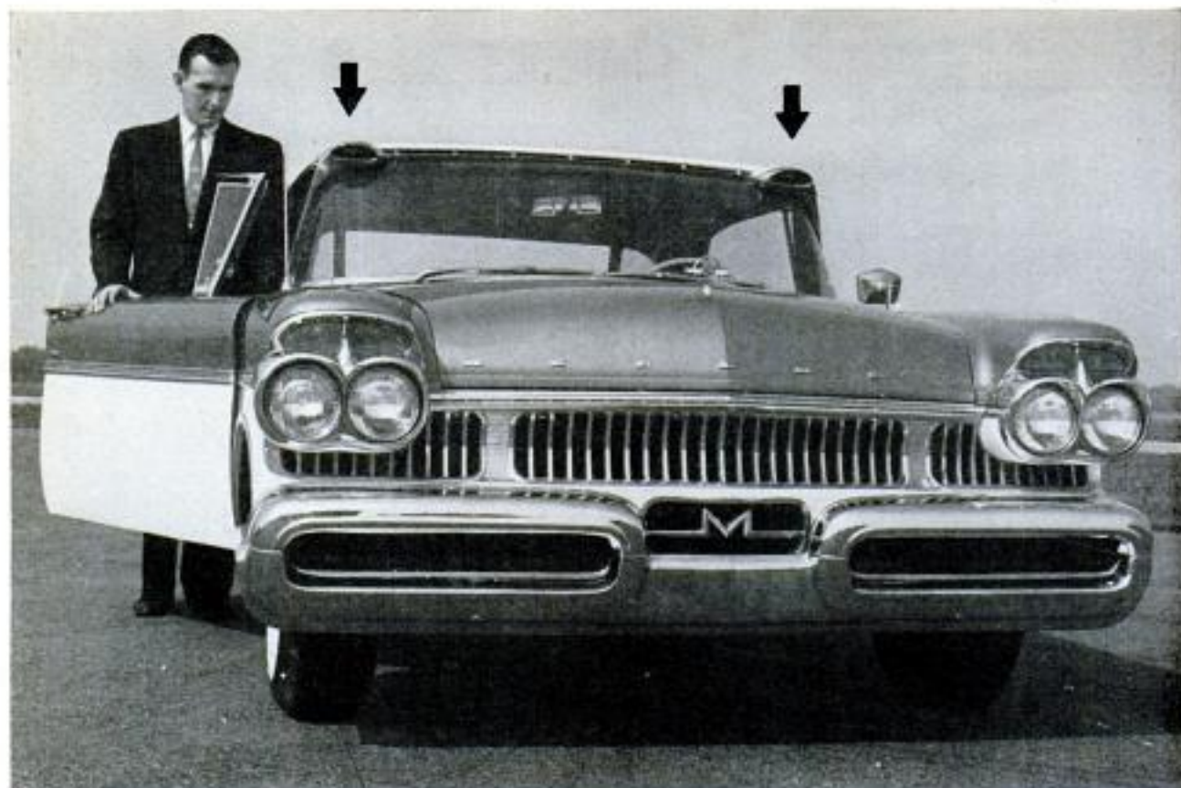
Arrows point to the air-intake pods atop compound-wrap windshield. Dual headlights are optional on Cruiser
