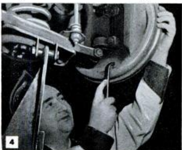
With drums reinstalled, brakes are bled and adjusted so there is no drag, good pedal. Below, front-wheel bearings are repacked before drums are reinstalled. In latter operation, care is taken not to use an excess of grease which may run onto brake drums
