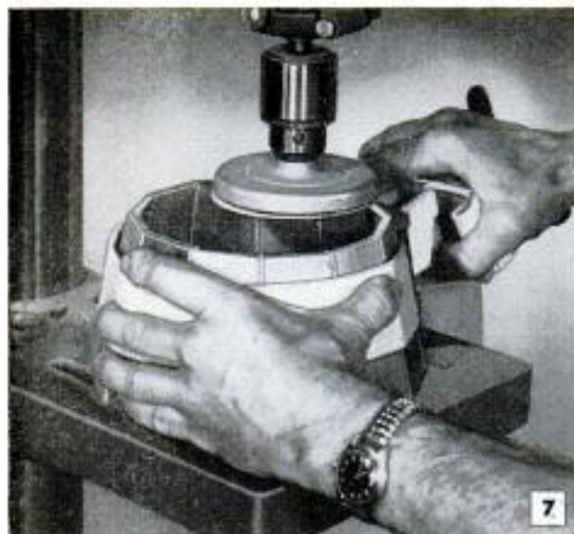
7 Sanding disk chucked in drill press is used to sand uneven ends of staves. Lock quill for final sanding
