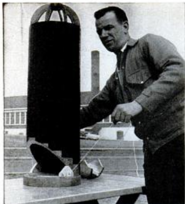
Model showed engineer that small triangular segments at opposite balance points held up structure
