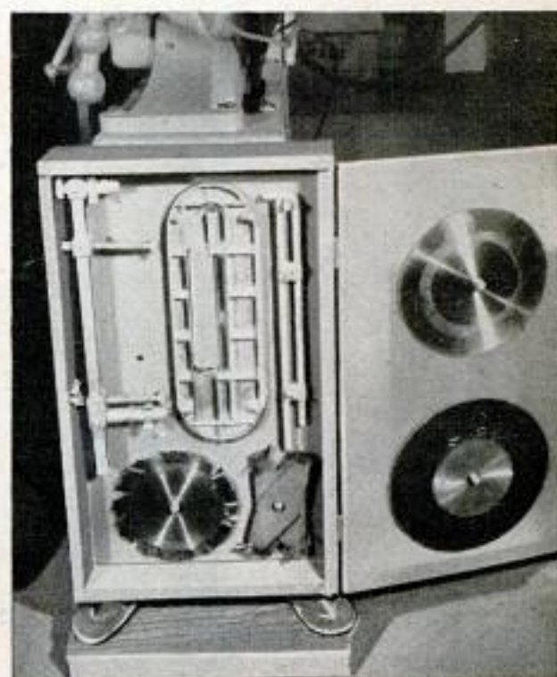
Stands containing no motor or machinery are suitable for built-in type of cabinet as shown above
