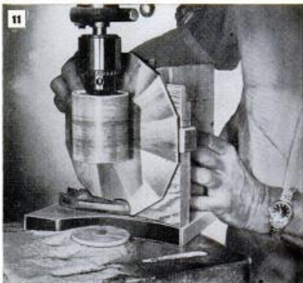
10 When dishing sections of pyramidal lid, each stave must be held on a level axis to assure uniformity
