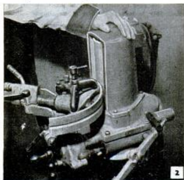
After wheels are removed, boots on wheel cylinders are pulled back and cylinders checked for leakage. Below, new brake lining is buffed to a true radius
