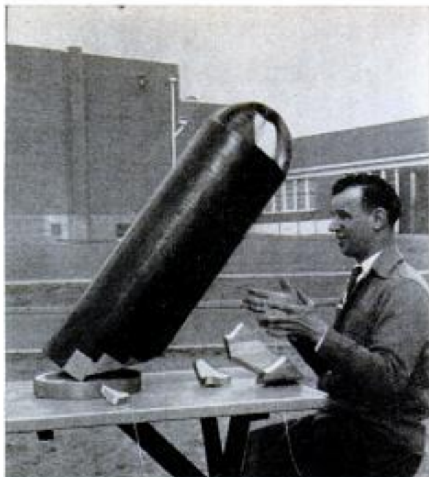
When triangular segments were removed simultaneously with jerk on a string, model fell straight and true
