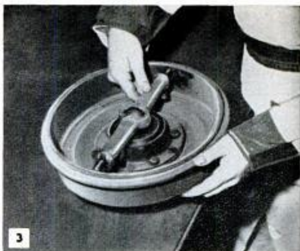
Above, drums are checked for true radius and to see if they have been turned oversize beyond limits
