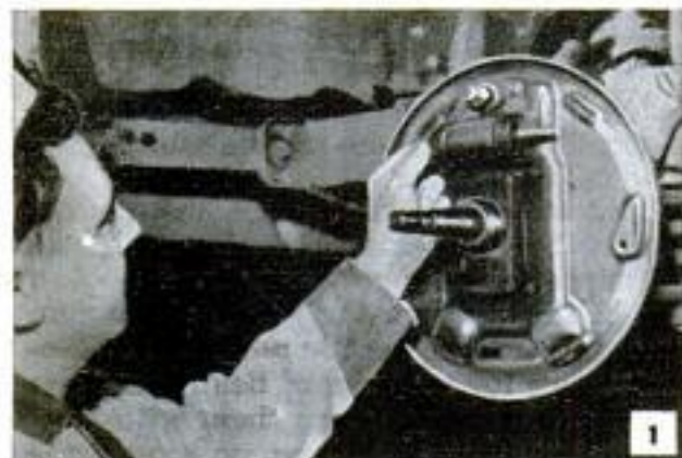
After wheels are removed, boots on wheel cylinders are pulled back and cylinders checked for leakage. Below, new brake lining is buffed to a true radius
