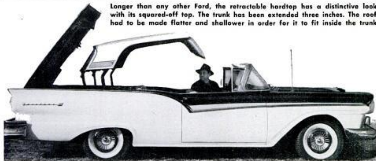
Above, as the top lowers, its forward edge folds under to shorten its overall length. The whole operation is automatic once the button is pushed. It takes 40 seconds for the cycle and it can't be started until the engine is stopped and transmission in neutral. If you just want to load the trunk, you stop the cycle when the trunk lid has opened, but before the top has moved
