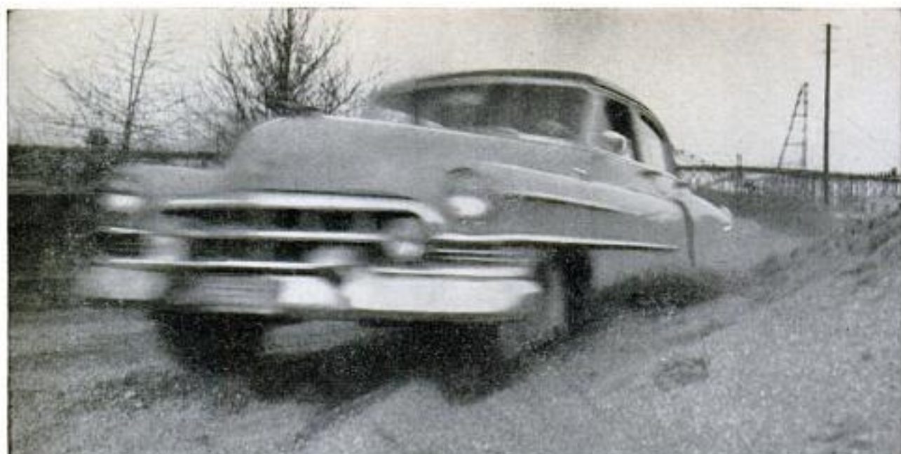
Driven off the road into a pile of sand at 40 miles per hour, the test car shows no signs of loss of control
