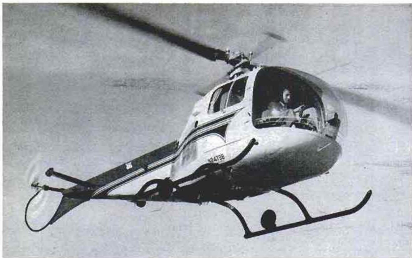
Bell 47J Ranger, capable of carrying more than 1000 pounds of payload, will be delivered early in 1957
