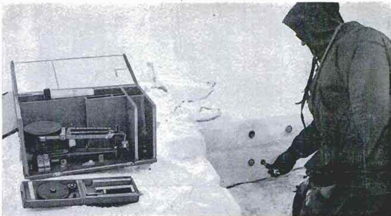
Thermometers and scales are used to check the temperature and density of snow prior to building airstrip
