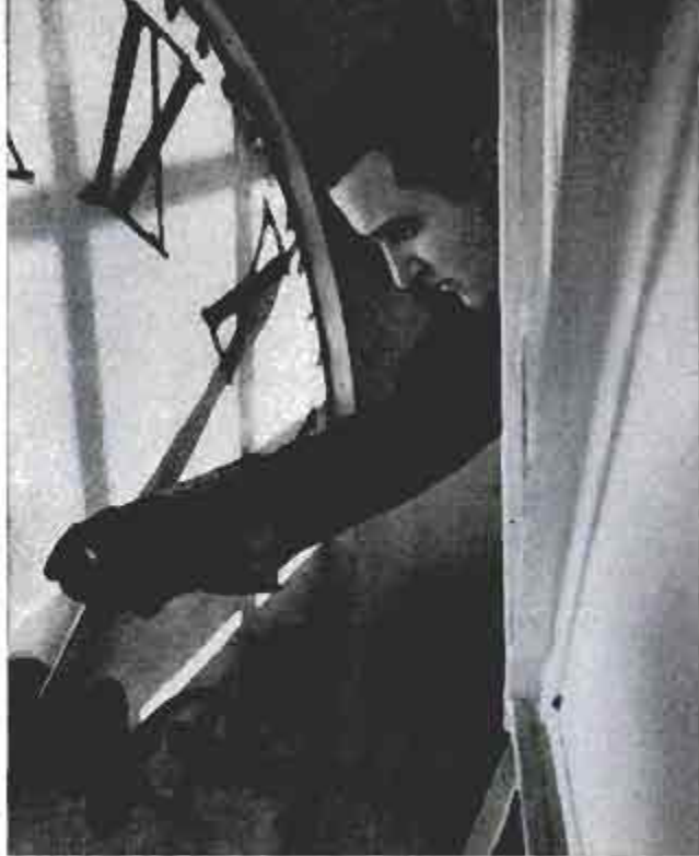
Behind a glass clock dial a repairman oils gears of rod that makes clock's hands turn at different rates
