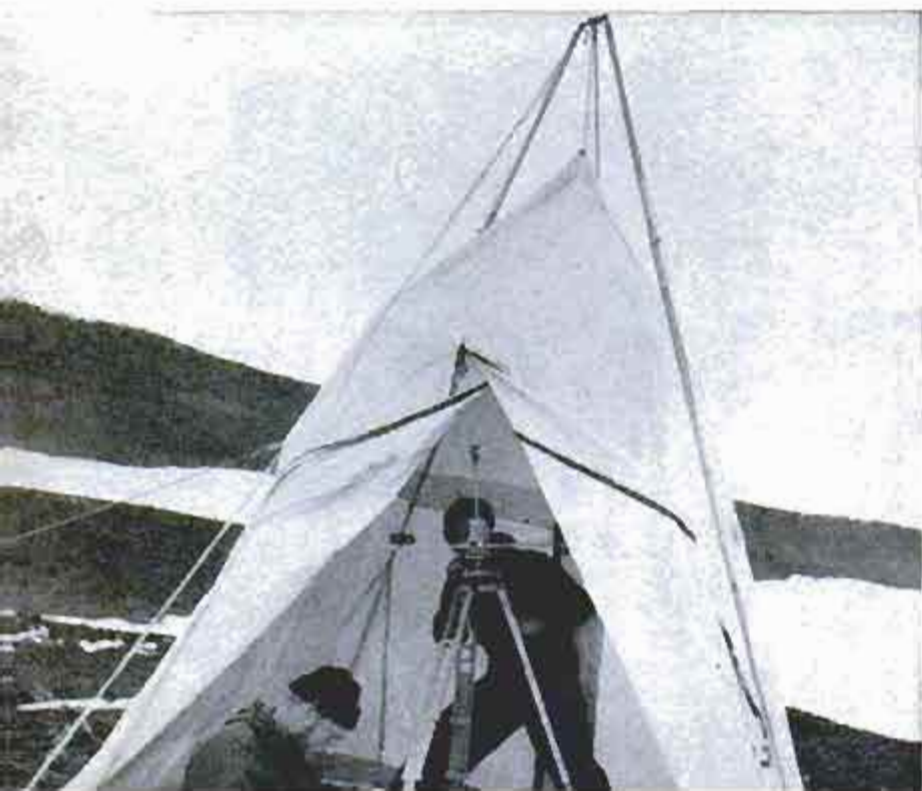
Navy technician, below, protected by tent that can be erected in five minutes, sets up instrument to check earth's magnetic field
