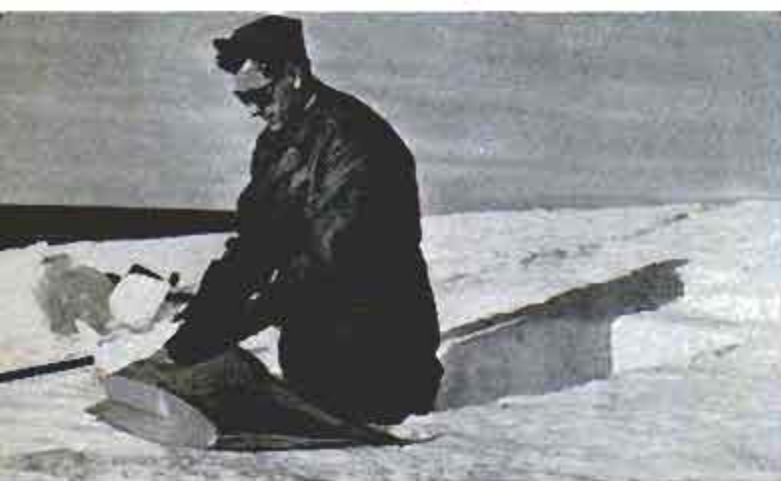
Scientist collects sample of snow in paper bag. Snow is melted, and radioactive tritium then tells how long ago the snow fell. Below, movie camera records cosmic-ray penetration of atmosphere near the pole
