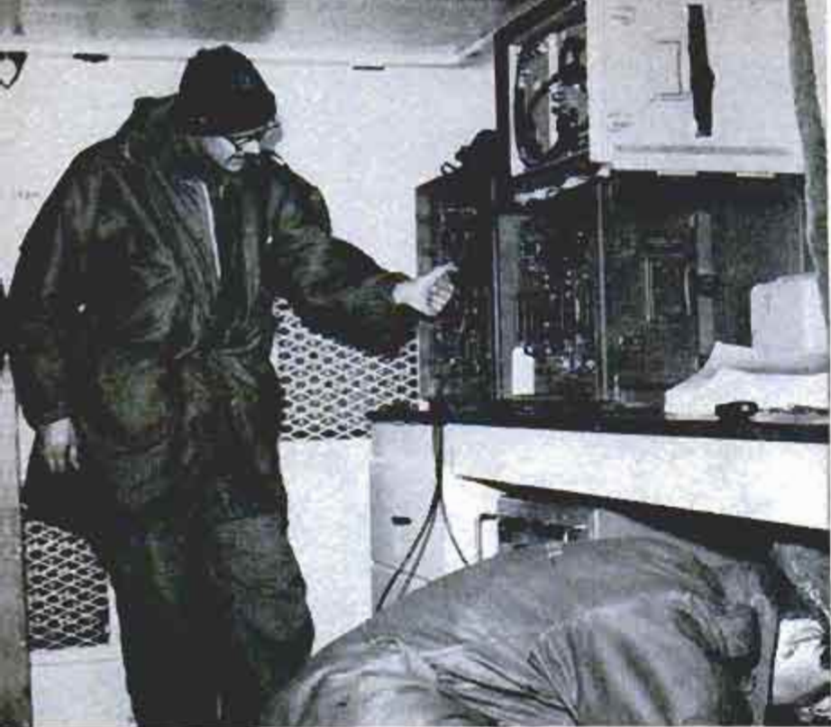
Inside an insulated hut, a Signal Corps team sets up equipment to test radio transmission through the deep blanket of ice. Lightweight hut can be towed into place by a Weasel, below, or parachuted already assembled from a flying boxcar. The huts have precut openings for heater stacks and ventilation
