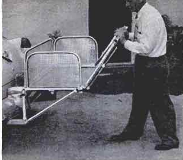
Stoiadin folds up four rear panels against the front half when he wishes to carry only half a load snugly
