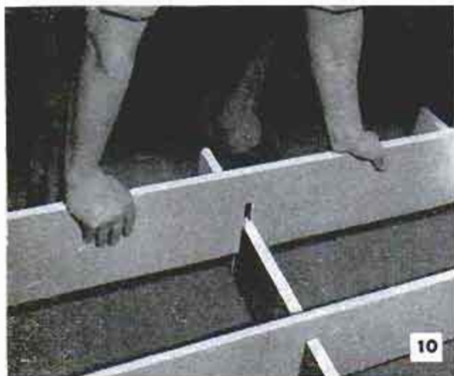
Accurate cutting of shelves allows a snug fit and assembly to integrated unit without nails or glue
