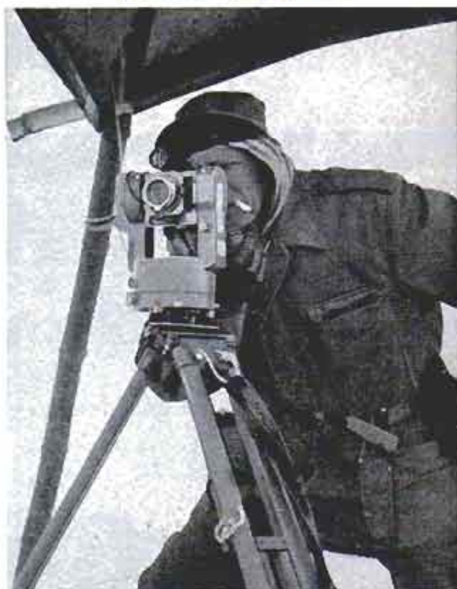
Photo theodolite permits surveyor to photograph his sightings, make his calculations later from photos
