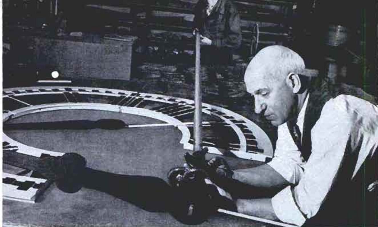
New clock assembly is laid out. The pine hour and minute hands are balanced by the short, white, iron rods
