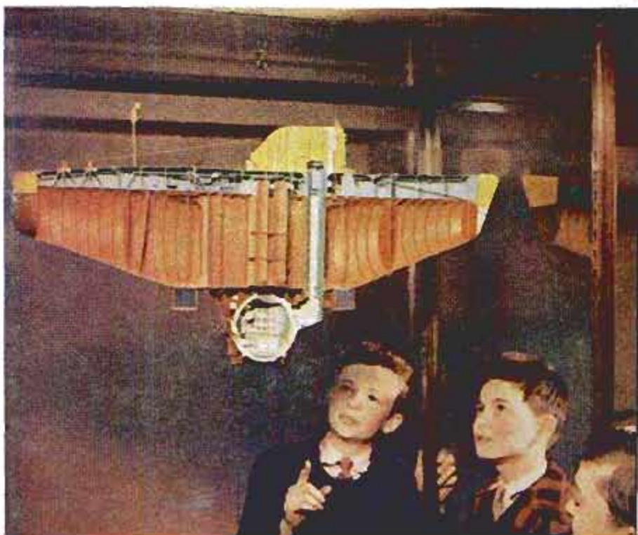
Here's a cross section of the bathysphere in which a pair of French naval experts made a record descent of 13,500 feet
