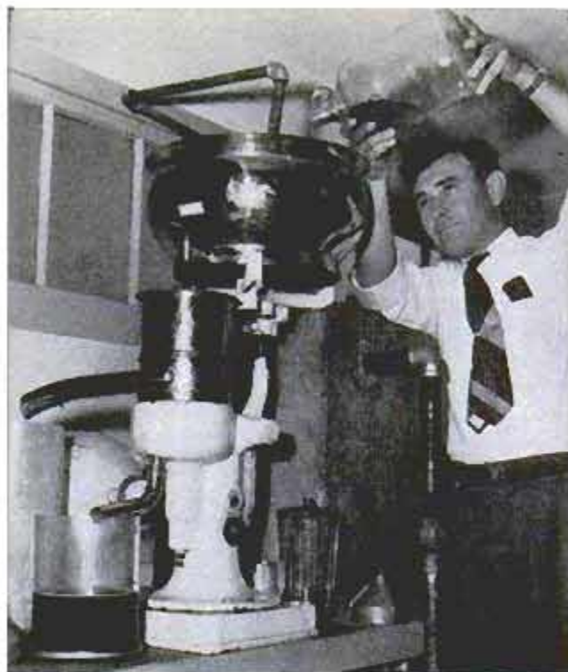
Extracting algae from water with separator, above, is not as economical as chemical precipitation method
