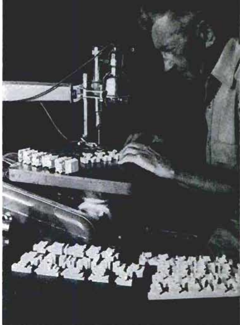
Each of the nine strips formed by cutting the block lengthwise may then be crosscut into smaller pieces making this unusual puzzle even more complicated to put together
