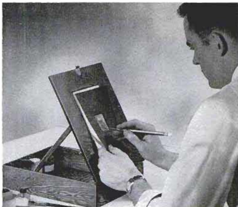
Retouching is done with cover of case open so that light can shine through the ground glass and illuminate the negative
