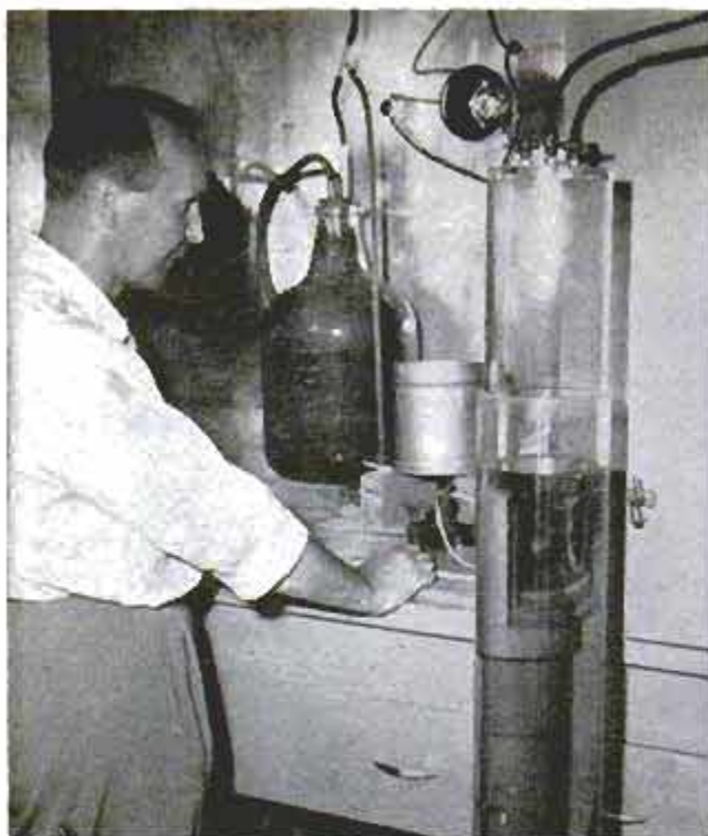
Research apparatus measures the gases given off by the dried algae after treatment for use as a fuel
