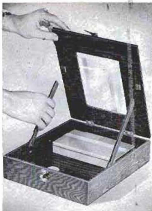
The cover is held open by two arms resting against cleats on underside
