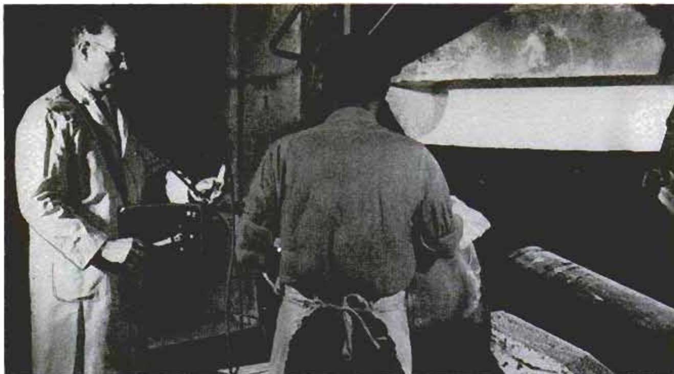
Industrial hygienist for rubber company takes sample of dust near workman who applies pigment to tires
