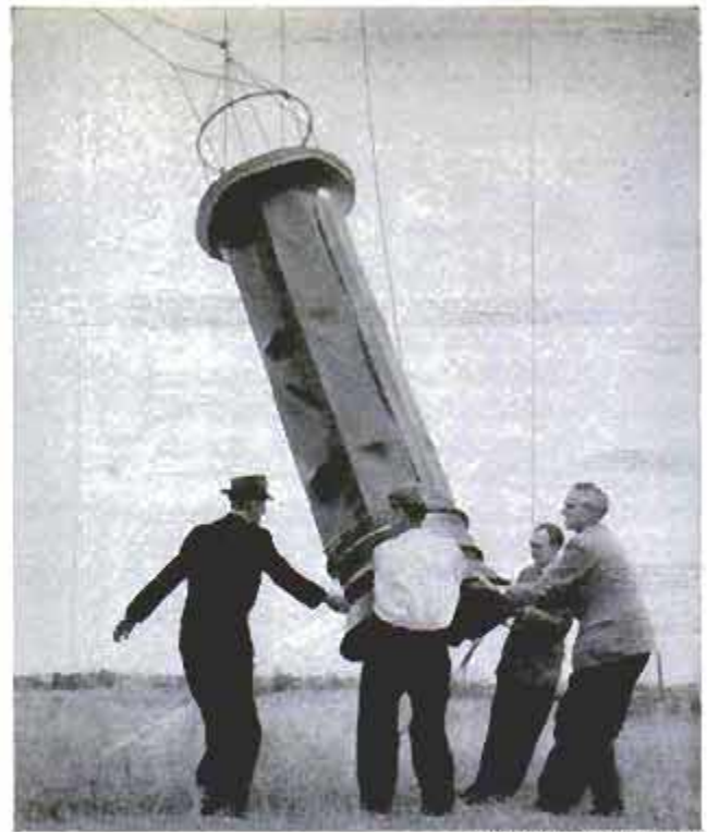
Trap 10 feet long harvests about 7500 flies per day, which are sucked into bag by powerful electric fans
