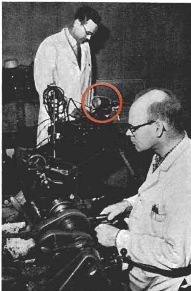
Microphone (red circle) in noisy factory picks up sound for recording on tape for laboratory study
