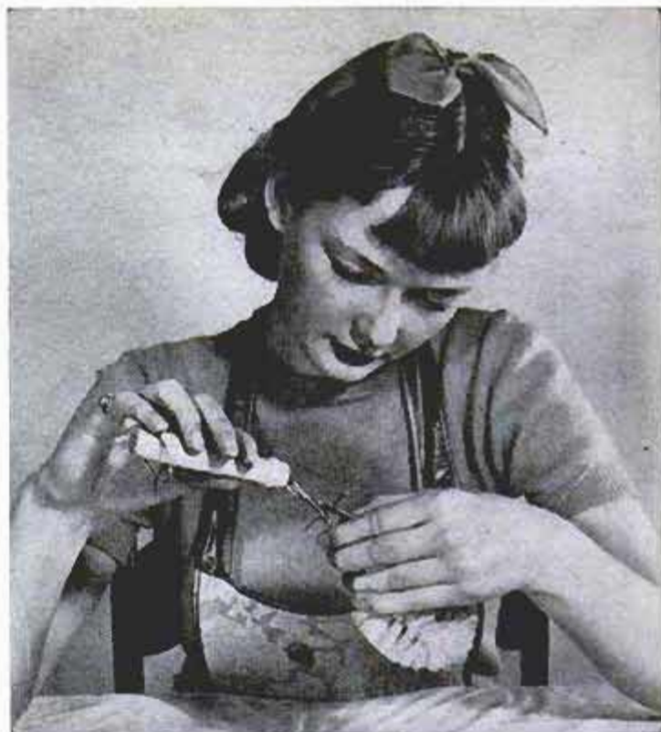
Tighten loose handle on household brush by spreading twisted wire and gluing tang back in handle
