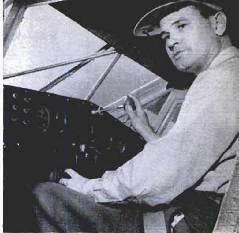
Professional look is carried into the cabin and instrument panel. Windshield is made of curved plastic
