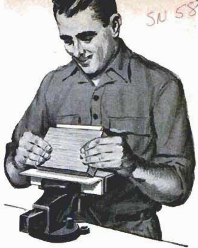
Above, 110-v. current passing through 220-v. hot-water heating element produces right amount of heat to soften plastic for bending without scorching
