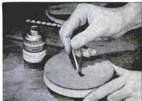
Periodically, depending on rate of use and type of operation, adhesive on FLEXBAC® Pad should be renewed with adhesive reactivator.
