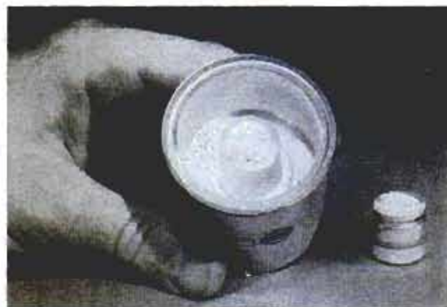
A scintillation crystal of sodium iodide is sealed in an aluminum housing to protect it from moisture
