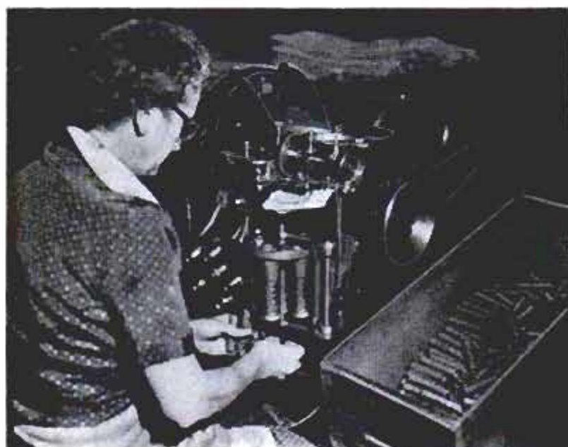
High-speed sorter separates and counts coins from pennies to half dollars, rejects slugs and foreign coins Semiautomatic machine wraps and counts rolls. Armed guard places bags on conveyor for delivery to surface
