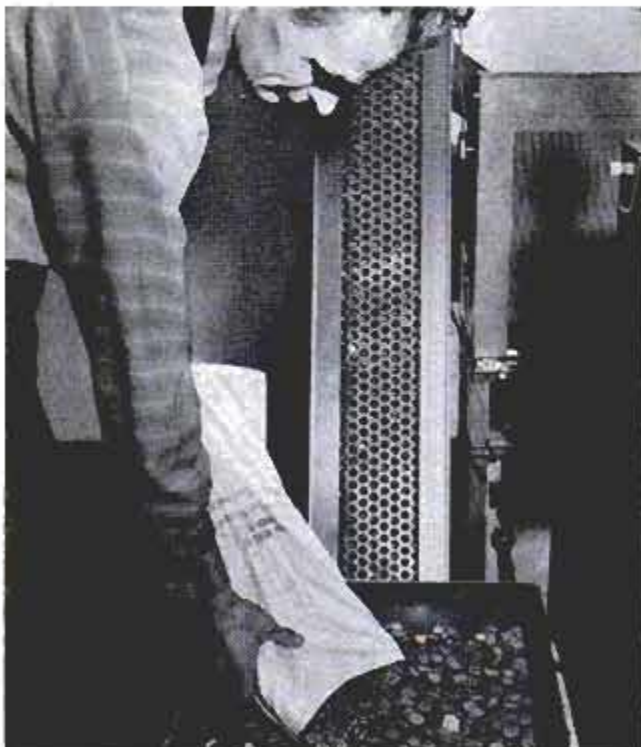
Pennies are dumped into a hopper. Covered belt in the background will carry them to counting head
