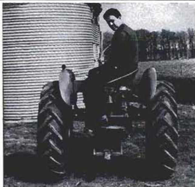
Tractor operator does not have to twist around when using seat, which turns to the side when required
