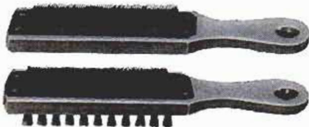
File card, top, is for more general use. File brush, bottom, combining brush and card, is used especially on finer cut files. Overall length: 10 inches.
