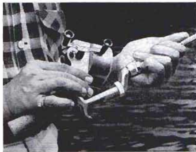
Cutter head removes for sharpening blades without disturbing their setting.
