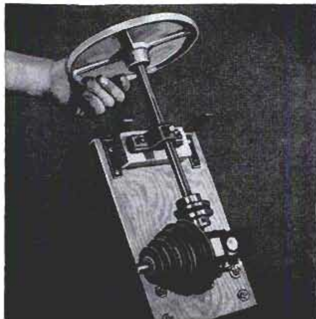
Speed-reducing drive assembled ready for installation in stool. Turntable is on 8-in. aluminum sanding disk
