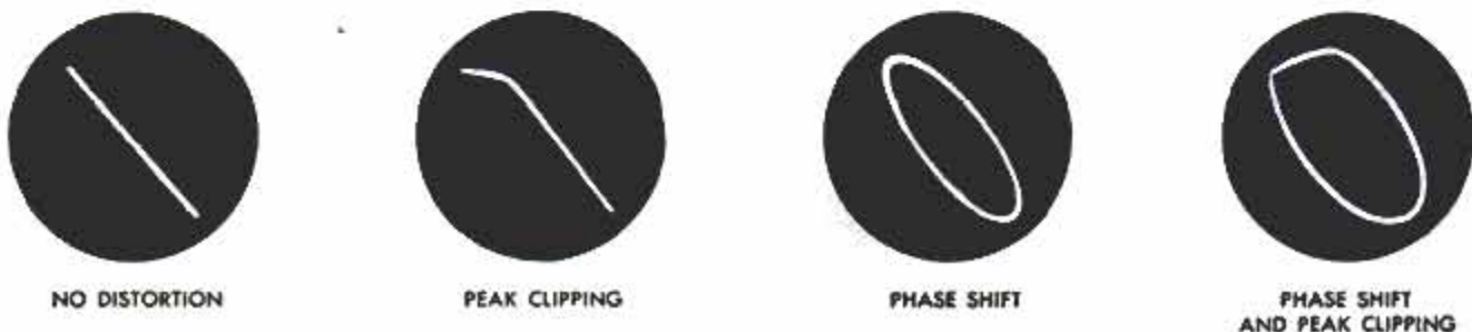
Fig. 4. Oscilloscope shows amplifier distortion. Top, with "saw tooth" sweep. Bottom, with sine-wave sweep
