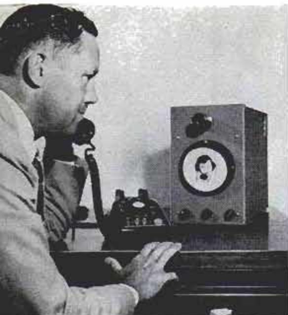
Experimental model at left has camera and screen in same unit. "Desk model" at right has a separate camera
