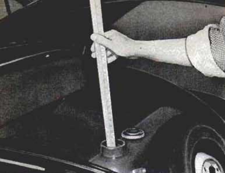
Above, the VW has no gas gauge. If you must know how much gas you have, use a yardstick! Below, some owners dislike the roller accelerator pedal (arrow)
