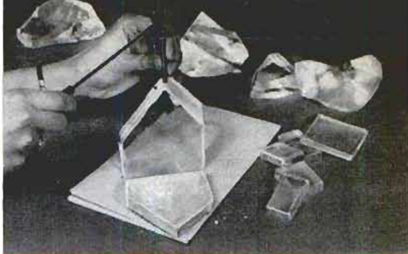
Laboratory worker splits a rock-salt crystal along natural cleavage planes, using hammer and chisel
