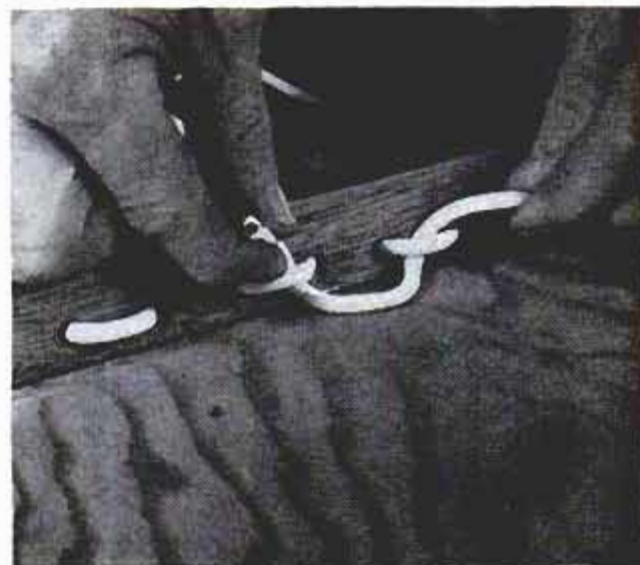
The end of the cord is fastened by weaving through return loops on the outside of one of the stringers
