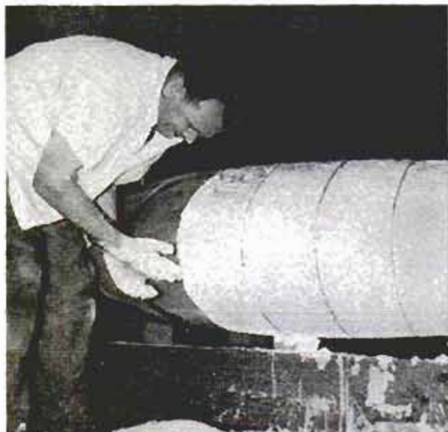
Plaster is then applied by hand to form the master over which the glass-fiber female mold is created
