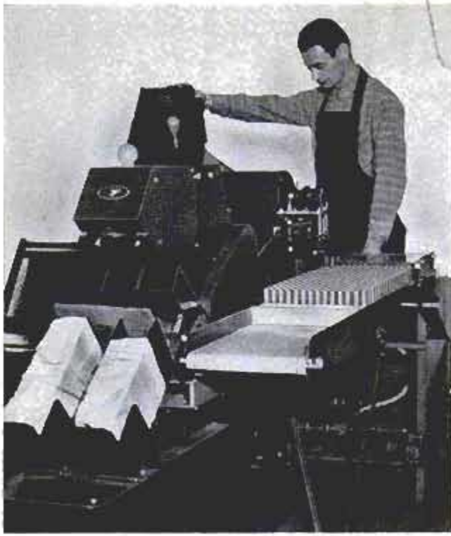
Handling pennies through quarters, this machine counts and wraps coins, delivers 1000 rolls per hour
