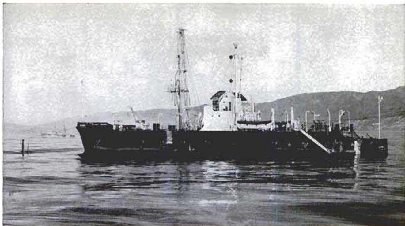
Surplus LSM has been converted for use in deep-sea drilling operations to explore for tidelands oil
