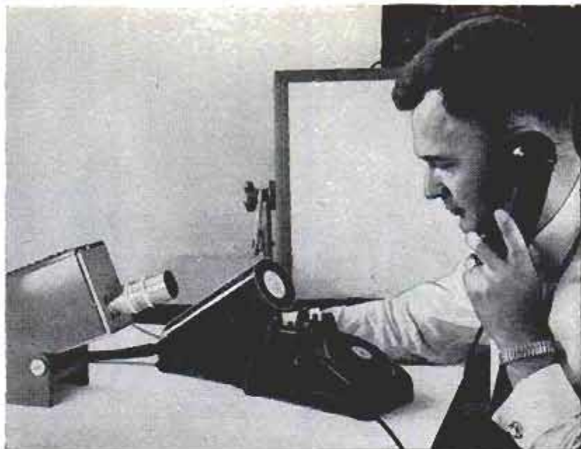
Experimental model at left has camera and screen in same unit. "Desk model" at right has a separate camera
