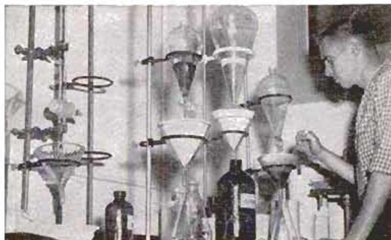
Chemical apparatus in the laboratory of the California Institute of Technology is used to separate some metals from granite
