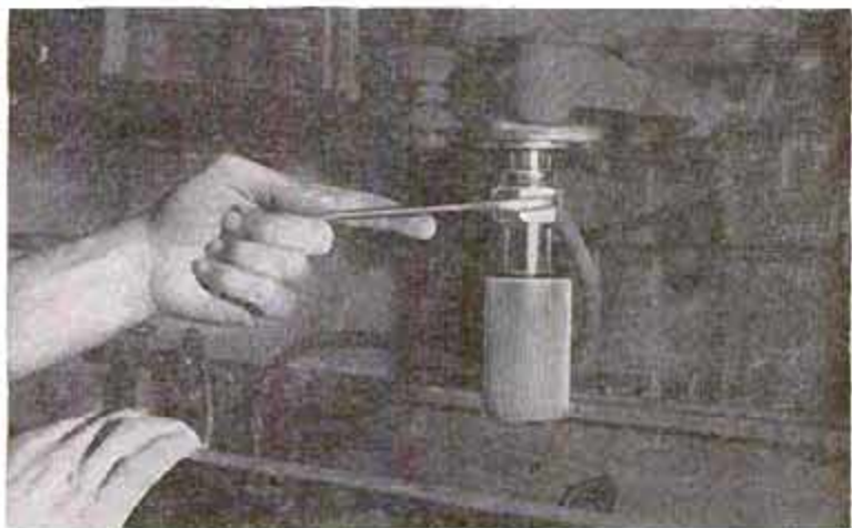
Above, in appearance the spark-machining unit is very similar to a small vertical milling machine. In the inset a fairly large electrode (cutting tool) is being attached to the spindle
