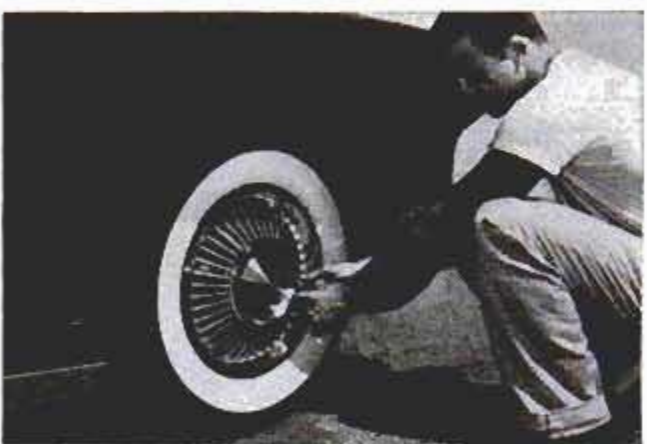
Hub caps cost $26 apiece, are assembled of 40 vanes. Below, seat backs are biscuited. Note the grab strap
