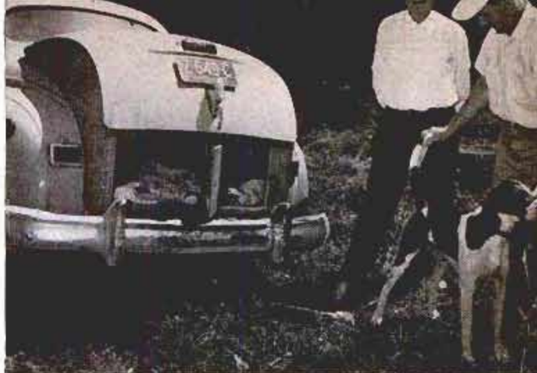
Plywood box converts the trunk of this car into a hauling crate. The wire is one by two-inch turkey wire. Crate accommodates two or three large dogs
