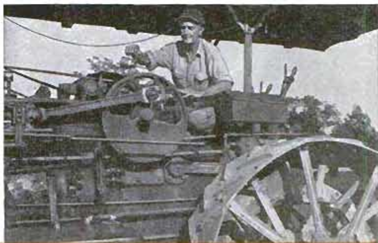
Below, the Jumbo, Alexander's first traction engine, as it appeared after he finished the refurbishing. The Jumbo gave 45 horsepower at the belt and 16 at the drawbar
