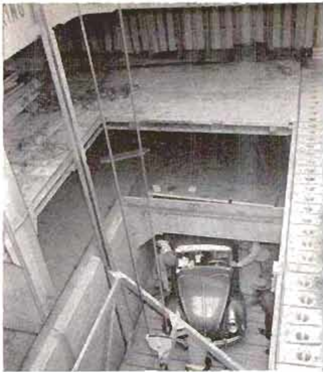
All cars are carried under cover on three decks. A VW is pushed onto the elevator from bottom deck here
