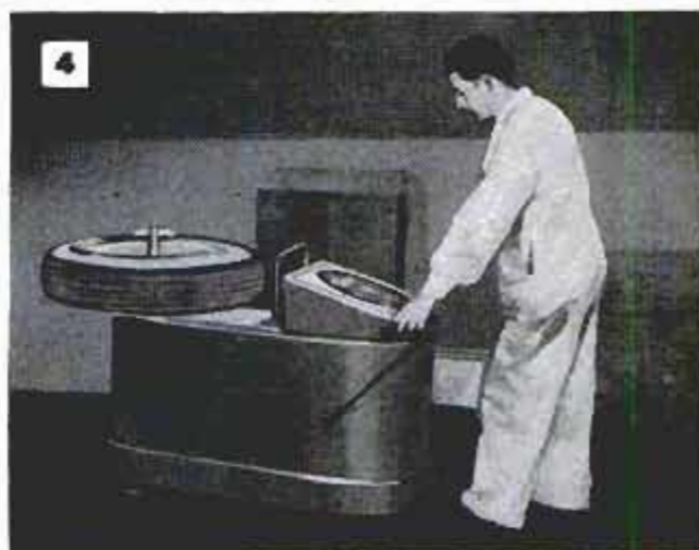
Above, familiar wheel-balancing machine balances wheel-and-tire assembly when removed from car. Below, lateral runout is checked by using dial indicator contacting sidewall lubricated with soap and water
