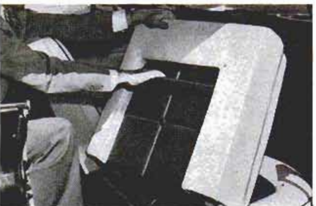
Hub caps cost $26 apiece, are assembled of 40 vanes. Below, seat backs are biscuited. Note the grab strap
