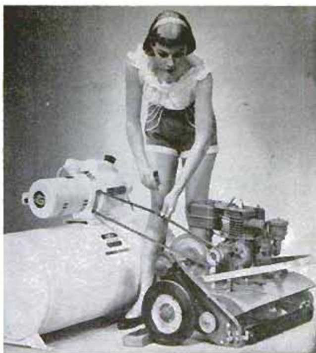
Pulley mounted on electric water pump permits it to be operated by gasoline engine during emergencies
