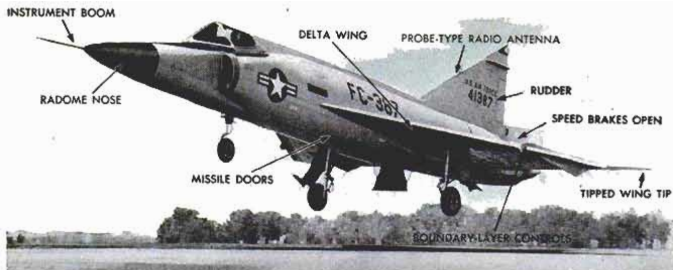
An F-102A shown in an approach to a landing, with its various parts and outstanding features identified
