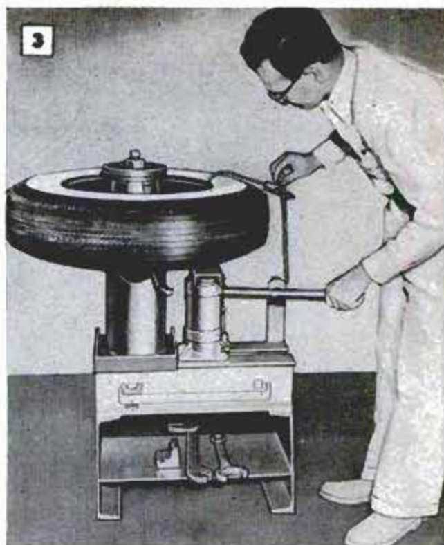
Wheels can be straightened without removing tire by using this machine employing hydraulic pressure
