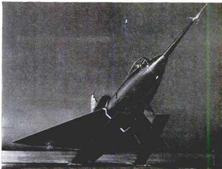
Convair Sea Dart, billed as world's fastest seaplane, uses a delta wing. An early model is pictured. Later ones have a single hydro-ski instead of two
