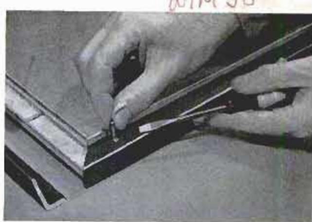
Above, steel angles that protect edges of ceramic tile are screwed to rabbet on underside of table top
