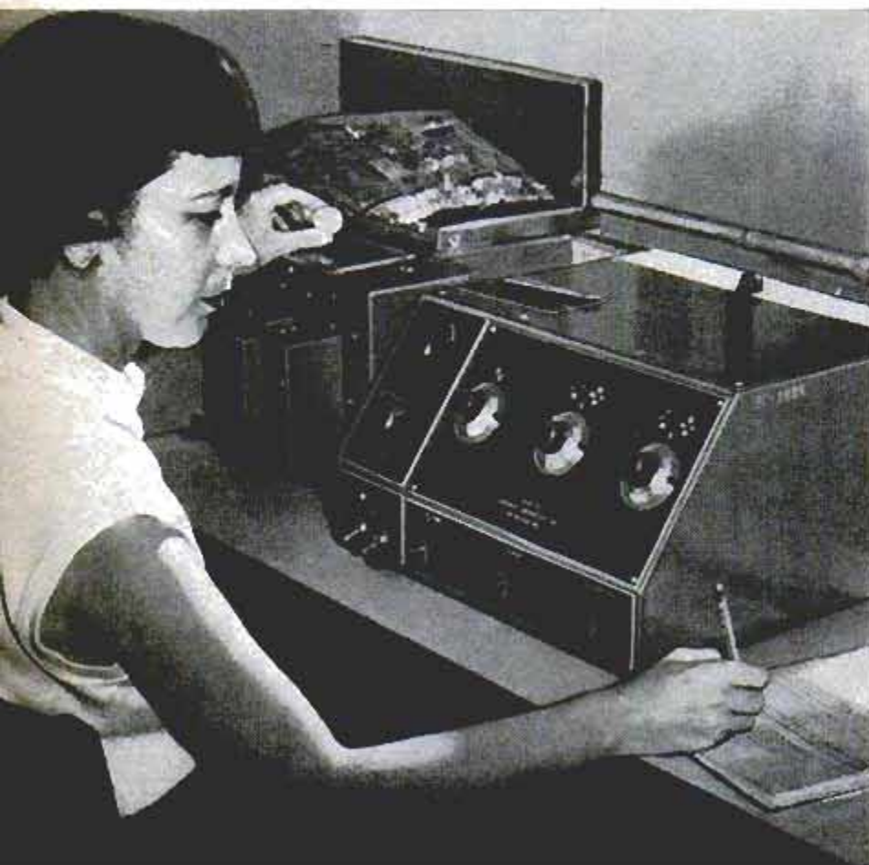
Above, manager Tito Capogrossi of the Cornell Electronics Stores, a warehouse crammed with equipment, pushes remote-control switch to operate samples on display panel. Below, in the home Economics Department, shade of potato chip is tested on electronic color meter
