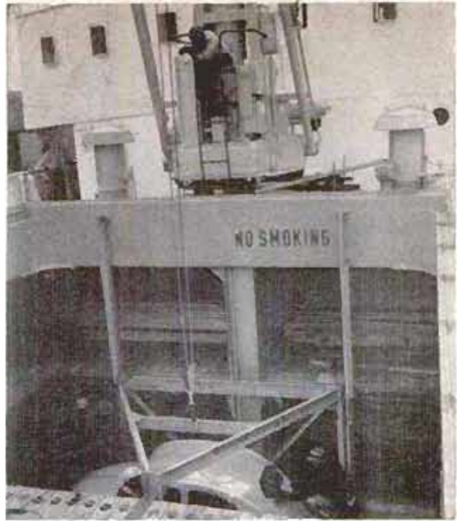
Operator raises elevator until it's level with door in side of ship (below) through which the VW is then rolled onto dock. No gas is in cars during voyage
