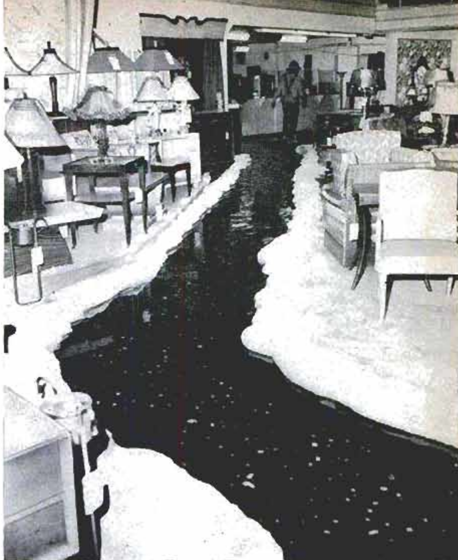
Los Angeles Fire Dept. photo Water channeled down stairway from fire above is directed to street by sawdust dikes that leave the surrounding carpets dry
