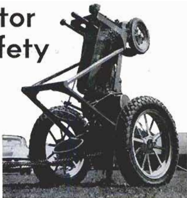
Rear-axle hitch causes tractor to rear backward
