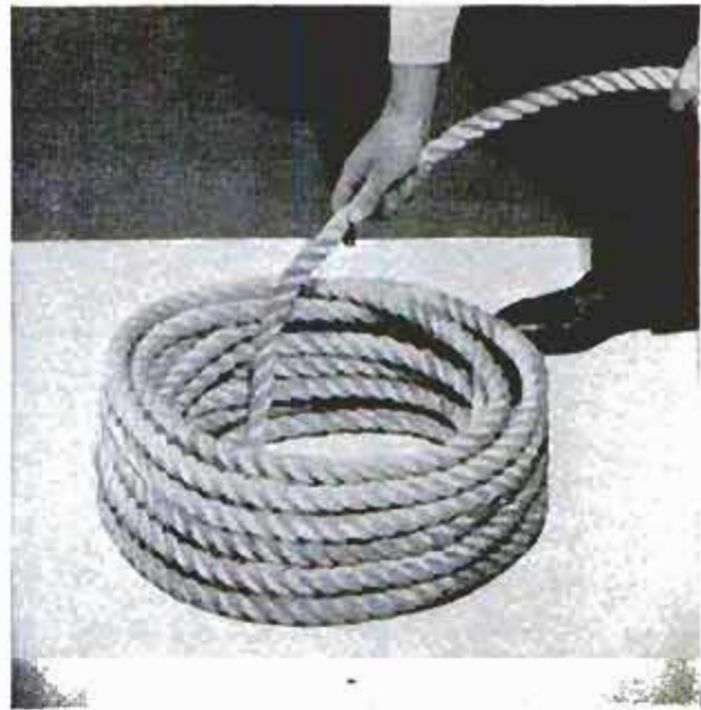
2. Unwind new right-laid rope counterclockwise from inside of coil, unwind left-laid rope, clockwise
