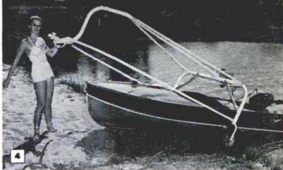
Above, lightweight boat trailer carries small boat suspended at bow and stern by sling and snap for easy launching at beach
