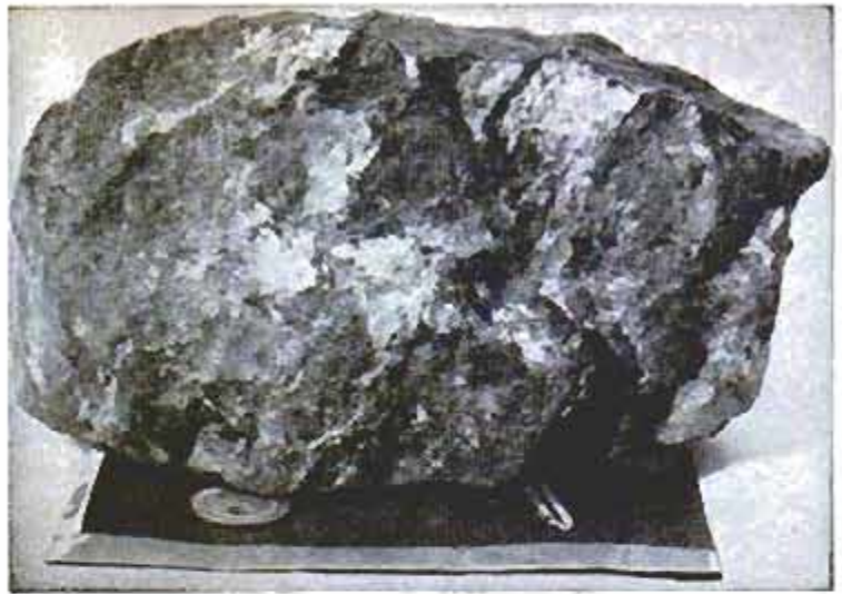
Above, uranium in specimen acts like X ray, penetrates opaque envelope and film emulsion except where blocked by metal
