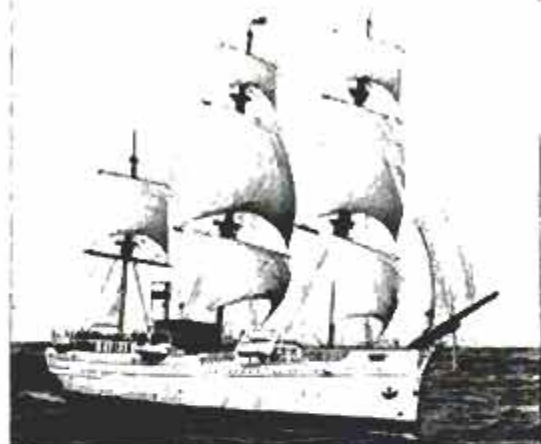
Ship appears to be full size in film. It is towed past the camera by an underwater cable
