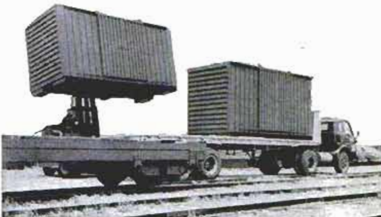
Adapto flatcar, in addition to being convertible, also can be used in railroad-truck piggyback service, as shown above
