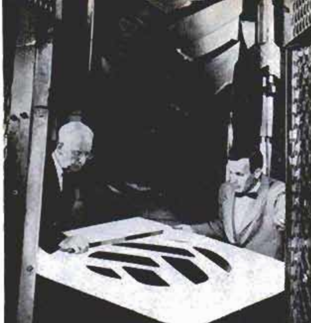
Engineers at General Tire Co. "fingerprint" huge tire to check area of ground contact under 18-ton load
