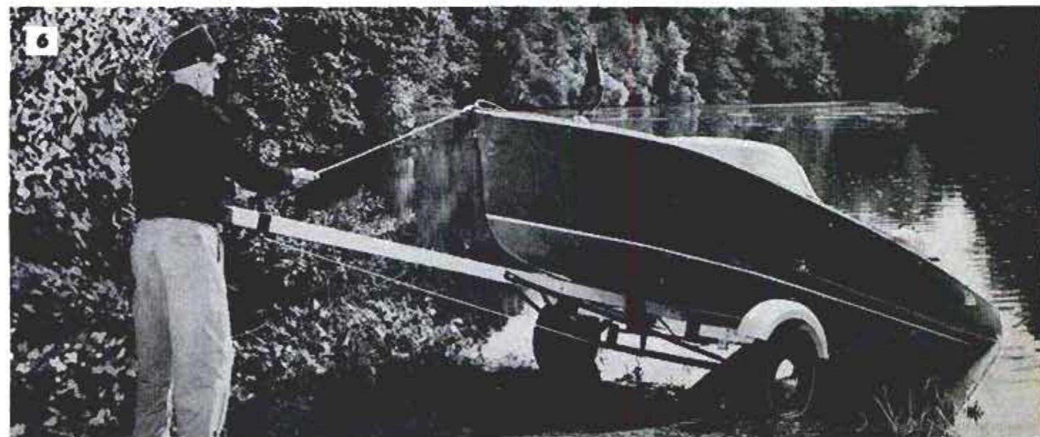
Wooden roller used for launching light boat or canoe can be turned to cylindrical shape or shaped to fit bottom of hull
