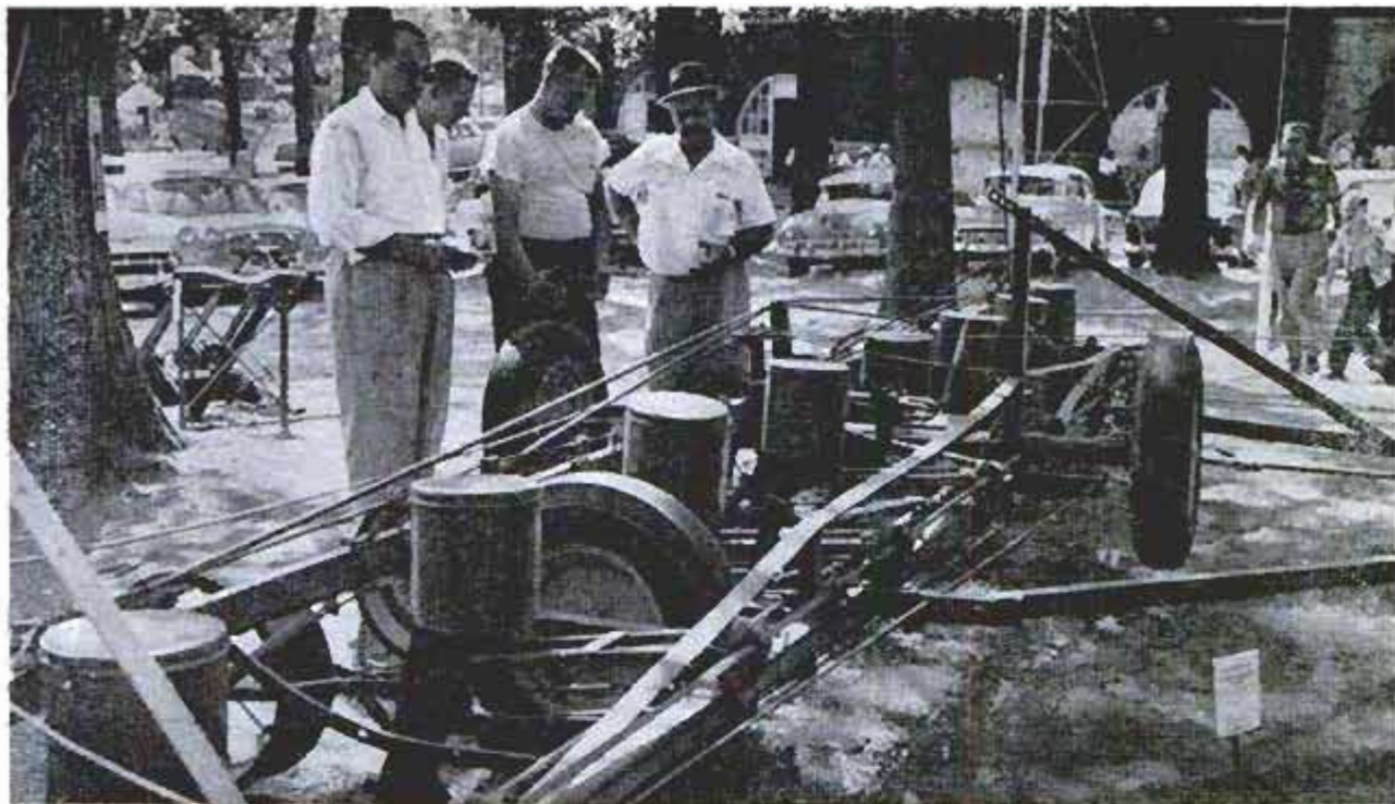
Eight-row corn planter speeds planting. Stand-by wheels are lowered hydraulically for endwise transport
