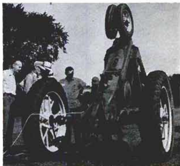
Upended tractor rests on V-frame. Below, tractor jumps the steering rail of ramp and starts sidewise tip. This tractor was used because it adapts to remote control
