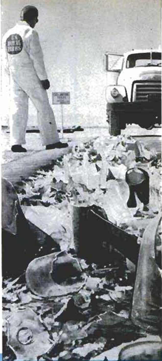
U. S. Rubber Company runs new "wire" tires through a bed of broken glass to demonstrate their toughness
