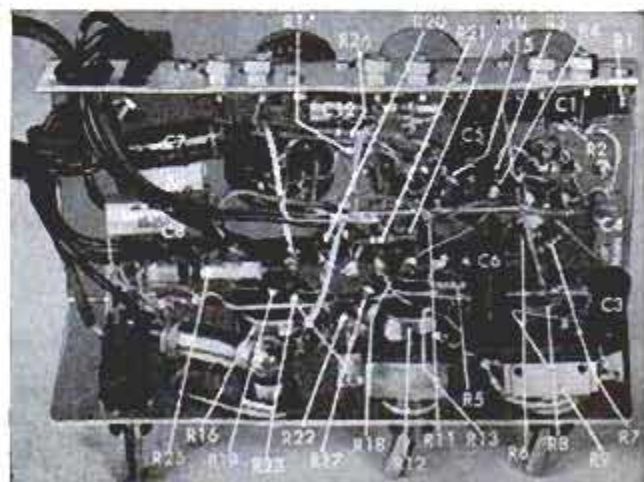
Fig. 5. Left, rear view of completed mixer. Right, under-chassis view shows exact location of small parts
