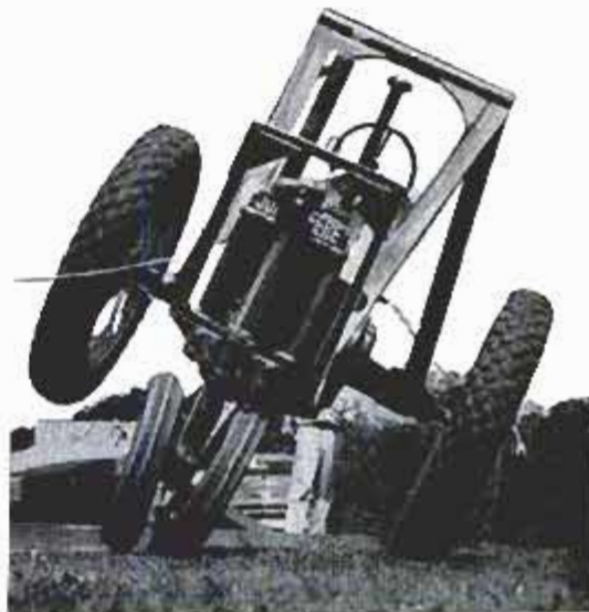
Upended tractor rests on V-frame. Below, tractor jumps the steering rail of ramp and starts sidewise tip. This tractor was used because it adapts to remote control
