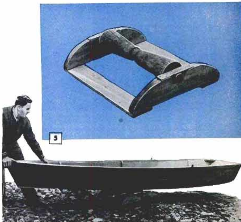
Wooden roller used for launching light boat or canoe can be turned to cylindrical shape or shaped to fit bottom of hull
