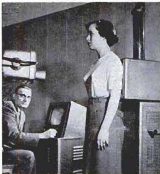
Remote-control fluoroscopic examination using Lumicon gives operator brighter picture to study
