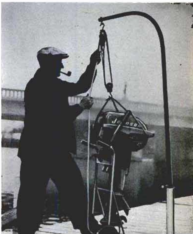
Above, motor is steadied with one hand until clear of boat to prevent damage to transom and propeller. Below, before lifting motor off dock make certain motor sling is well secured to lower-tackle block
