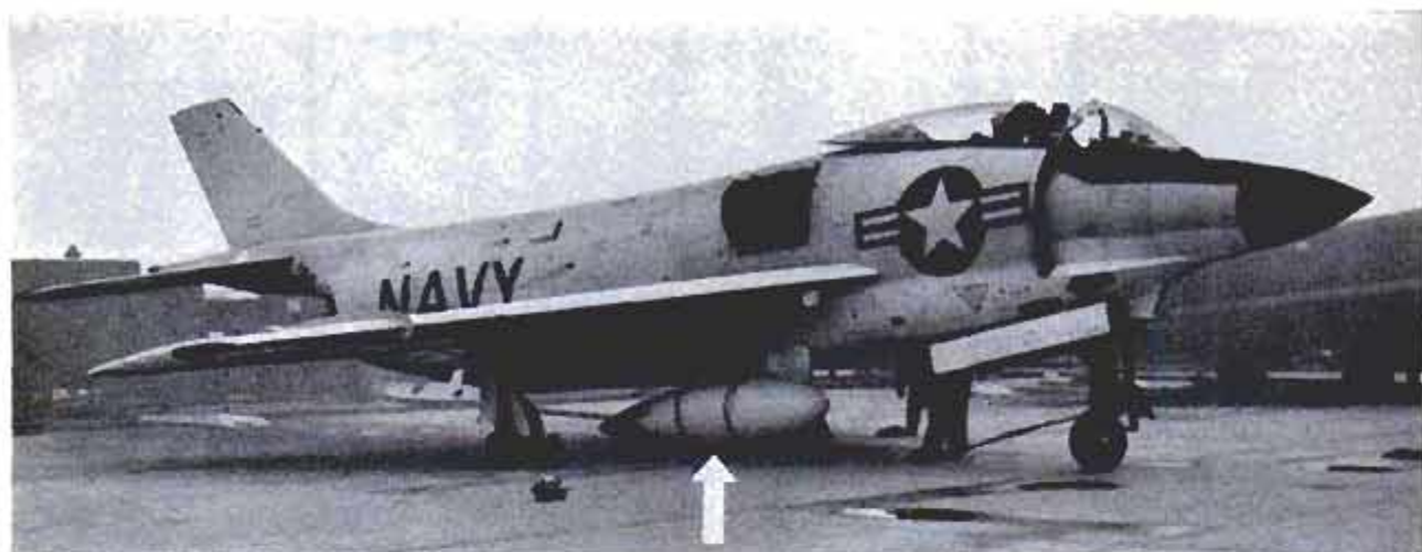
White arrow points to the gas-turbine starting pod. The pod can be carried on plane or mounted on wheels
