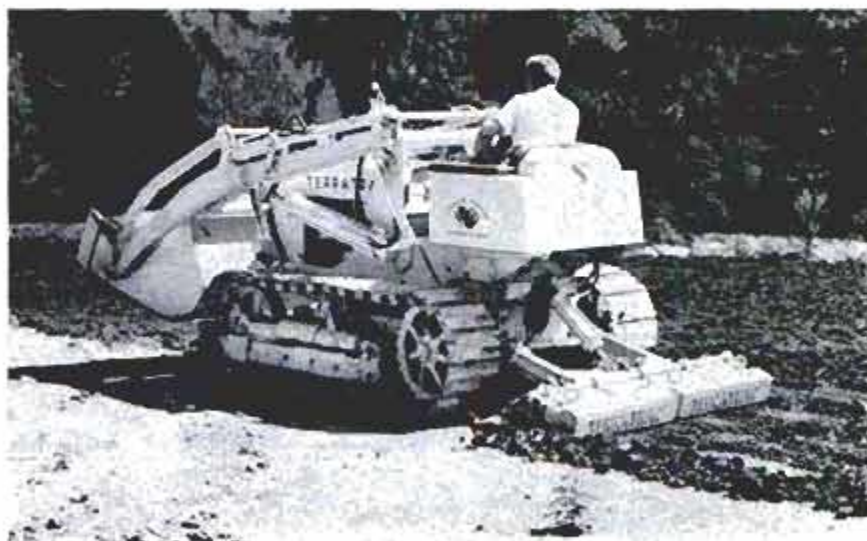
Power shovel and leveler are among many tools that mount on the tractor
