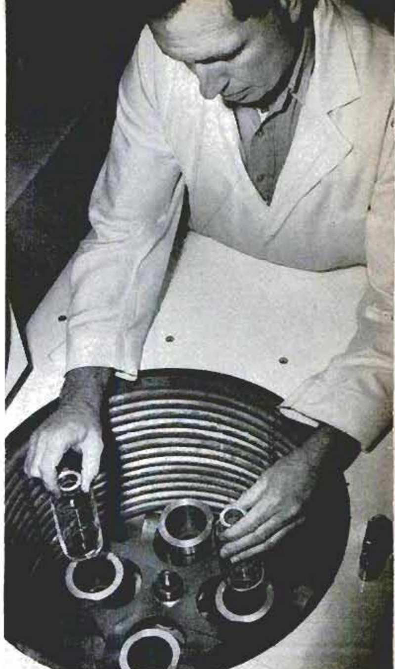
Refrigeration coils in centrifuge keep viruses alive while molecular weight of the substance is determined
