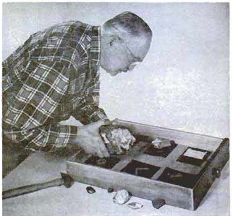
Above, heavy white area on print made from this test indicates a very rich ore sample. Below, ore samples are placed on envelopes containing squares of unexposed film in drawer
