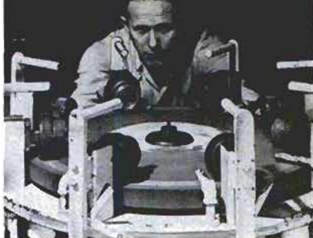
Laboratory technician tests samples of new rubber compounds on abrasive wheel for wearing qualities
