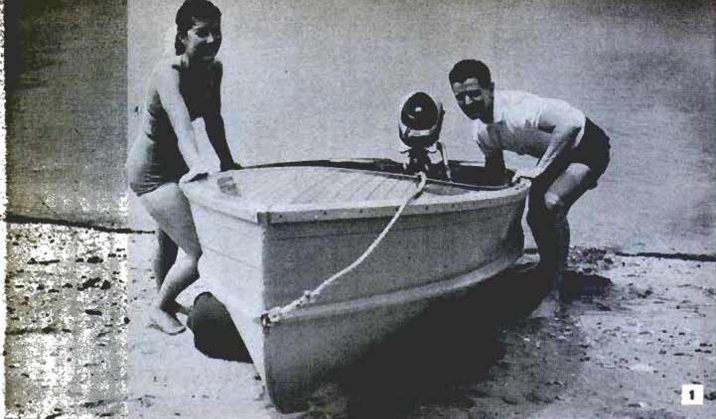
Boat is easy to launch on beach, hull is protected from sharp stones when inflatable rollers are used
