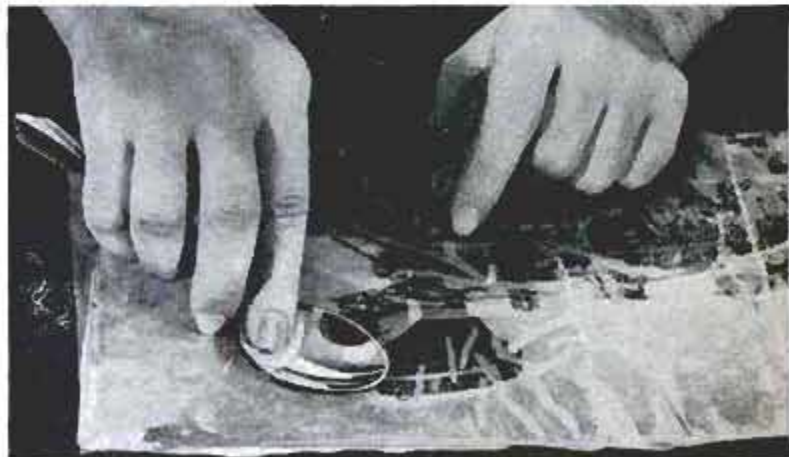
Above, smooth out all air bubbles with back of spoon. Below, ironing completes transfer of ink to frisket
