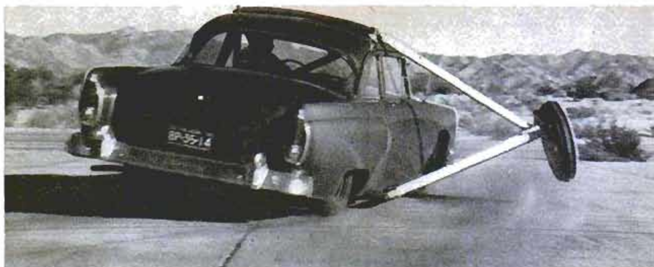
Equipped with outriggers to prevent rolling, test cars make screeching turns as they "wring out" new tires
