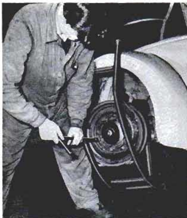
Mechanic tightens nuts on old auto wheel which is welded to cradle, fastening it to the brake drum
