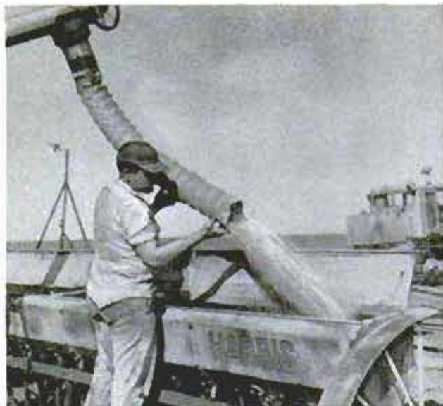
Seed for the huge machine is hauled in trucks. Automatic augers send seed spouting into the drill bins
