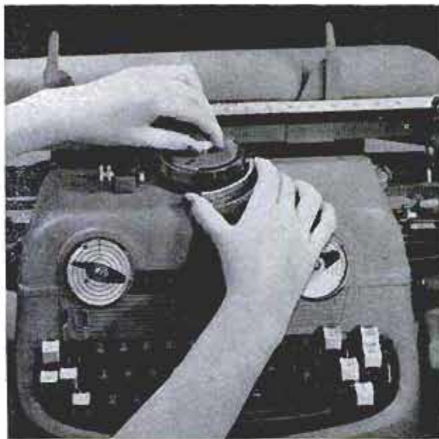
Type font of one language is quickly exchanged for that of another. Operator follows some code for all
