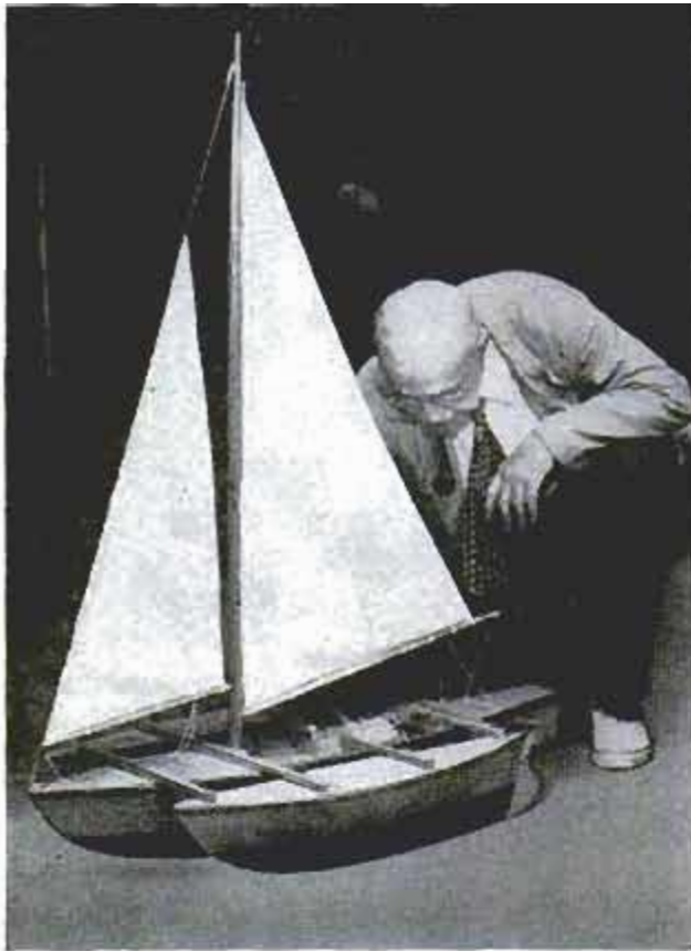
Before starting the full-size tripont, Dr. Herman built a scale model to test seaworthiness of design
