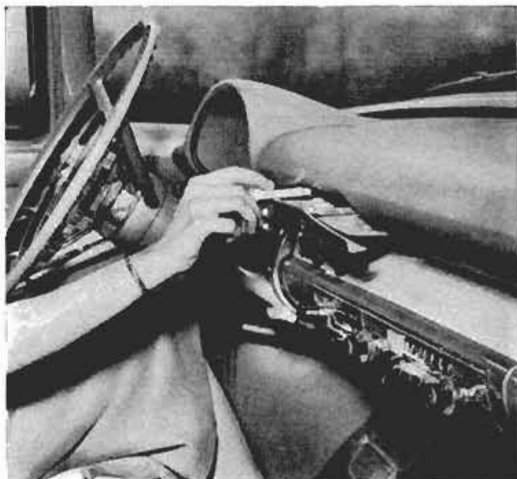
Above, owners like instrument panel and safety steering wheel. Below, they complain that padded dash makes ash-tray opening so narrow cigarettes often burn plastic covering. Some say protruding radio and heater knobs were not designed for safety
