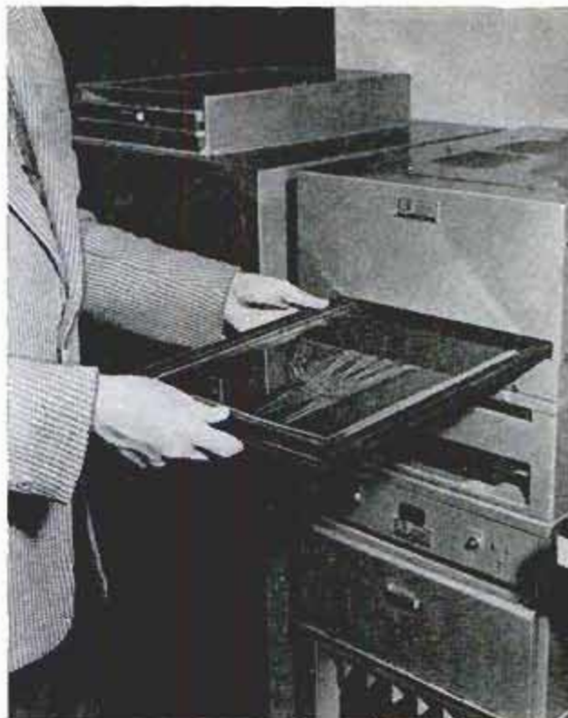
Electrostatic image becomes visible when sprayed with powder in developer. Below, picture has 3D quality
