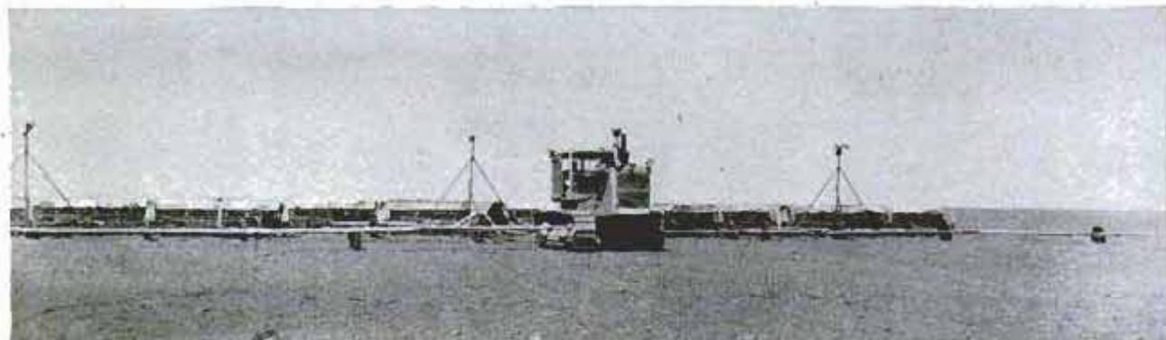
Machine stretches across Texas farmland. Made by assembling 11 standard drills, it plants swath 154 feet wide
