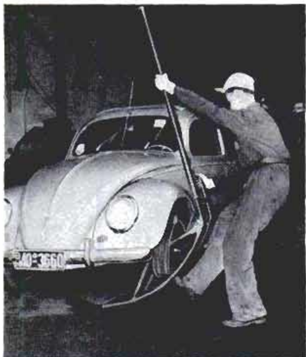
Long iron bar is slipped over pipe on cradle and mechanic grasps it high up to rock the cradle over
