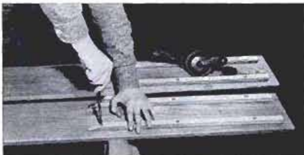
Keel strips, above, are mounted on the bottom of the skis at the rear, each one approximately 1 in. in from the side and rear edges. Place the tapered ends of the keel strips toward the front end of the skis
