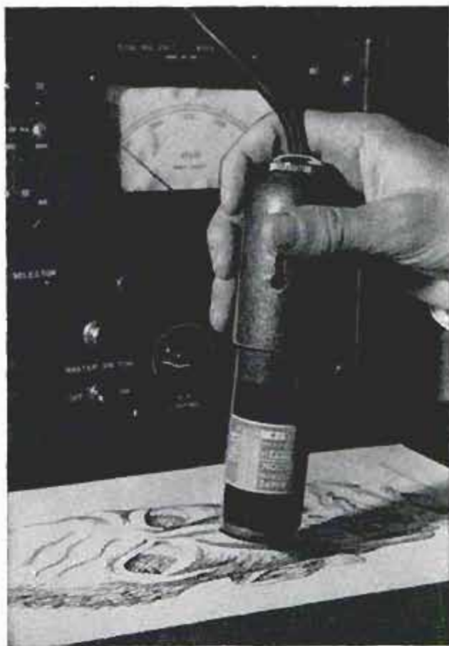
Geiger counter measures radioactivity to determine required exposure time—from half a day to six months
