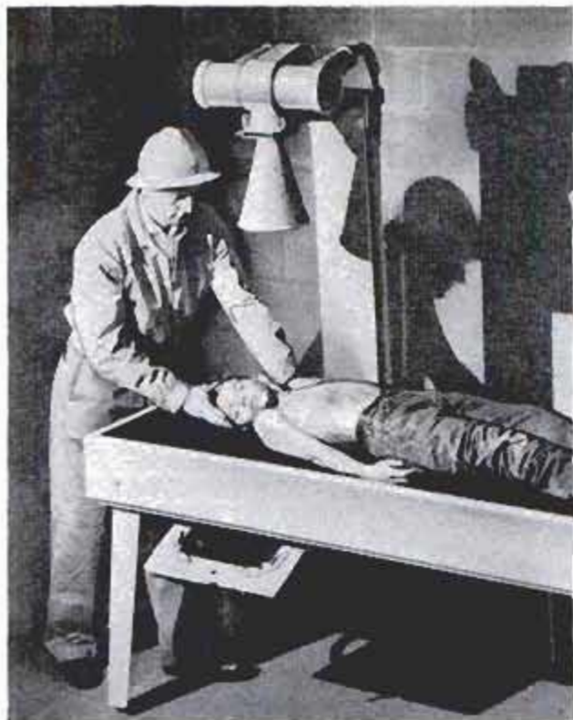
Conventional X-ray tube above patient directs beam through him to register electrostatic image on plate
