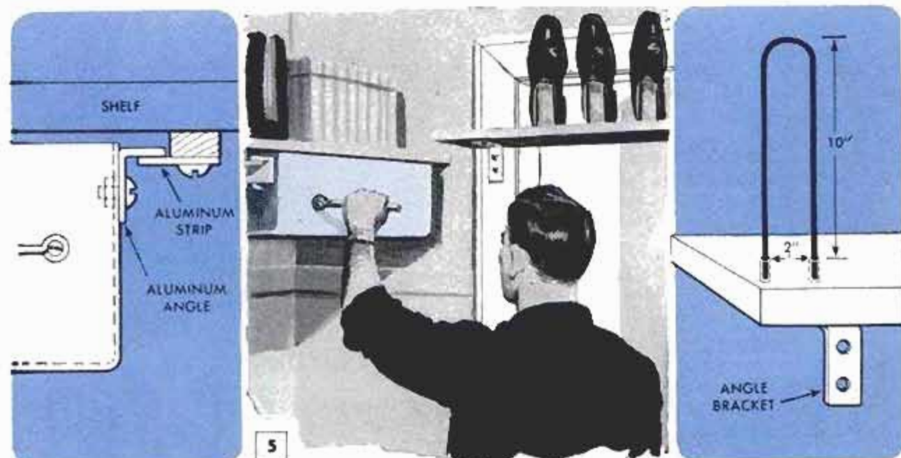
Closet space is fully utilized by installing drawer for hat and glove storage and overhead rack for shoes
