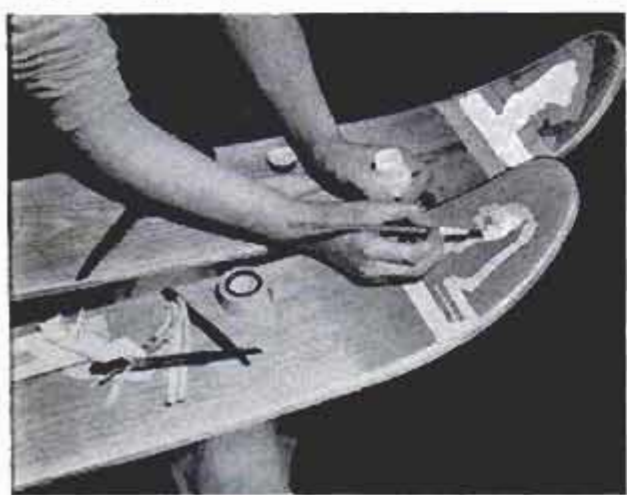
A touch of originality is illustrated above in the "brand" designs being painted on the toe of each ski. Masking tape is used to outline the design
