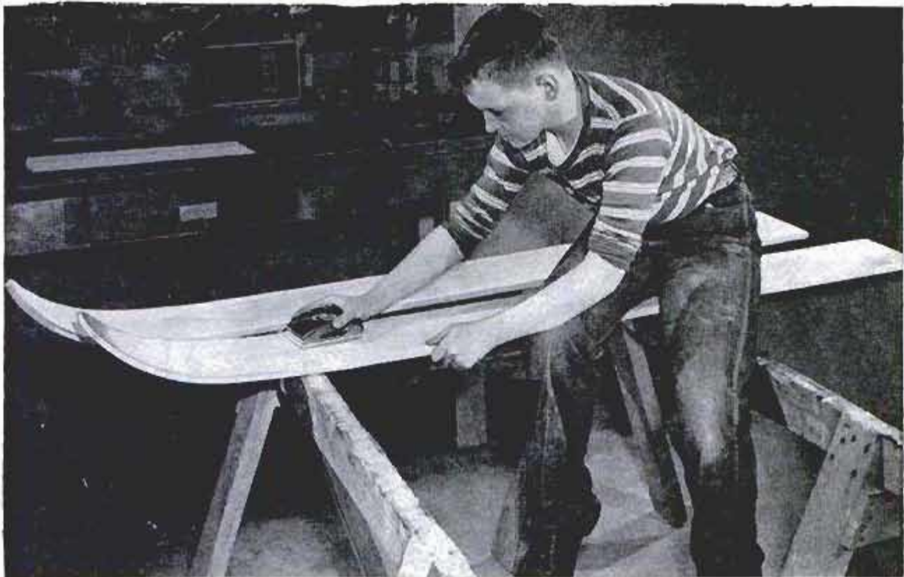
Top edges are beveled, and the entire surface sanded with waterproof sandpaper dipped in water
