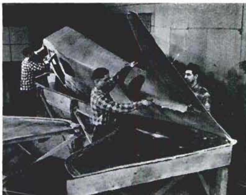
Large, low-cost dies are used to shape each half-fuselage in one piece. The plastic is light in weight and helps to insulate cabin
