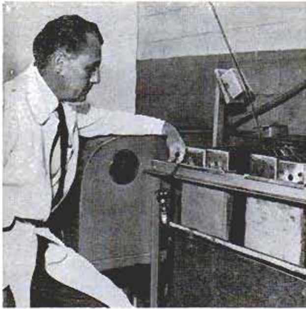
Motor that turns drive shaft is encased in housing beside Bailey. It is gauged by automobile speedometer
