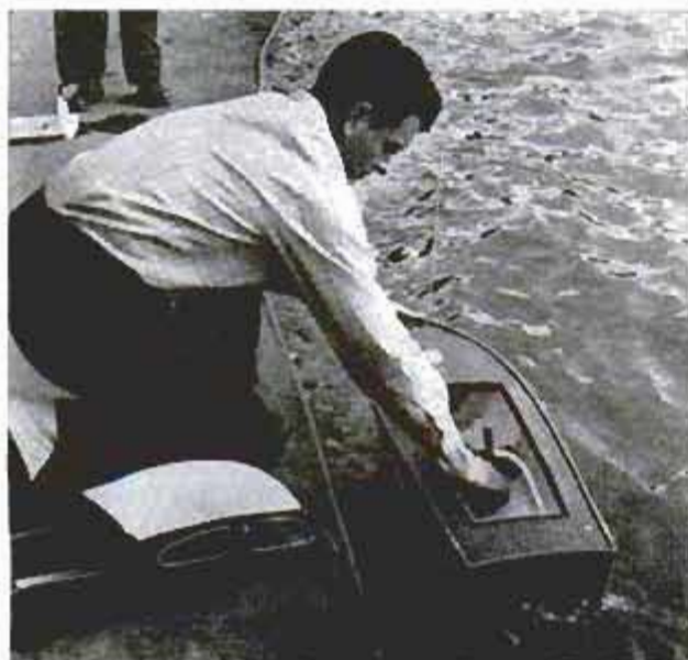
Engine is started and final adjustments made with boat in water. Top is put in place and cruise begins
