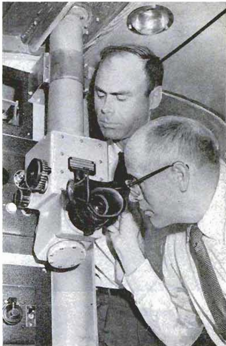
Periscope being evaluated in flight tests by Civil Aeronautics Administration representatives for use in transport planes
