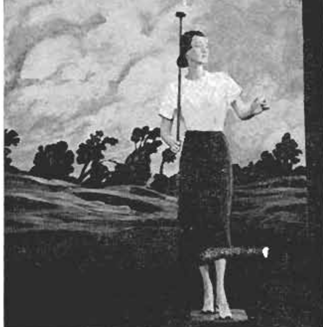
Bolt in lightning lab shows that a golf club with a steel shaft can actually become a lightning rod
