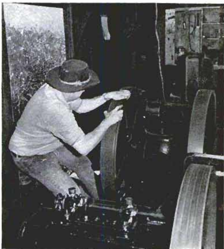
Huge metal roofs have been built on the islands to collect rainwater, which then is drained off into redwood storage tanks and saved for future use. Below, engines of the new water system are started by hand. They pump water up the mountainside
