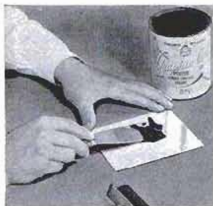
Screen-process ink is daubed on a sheet of glass, rolled down even
