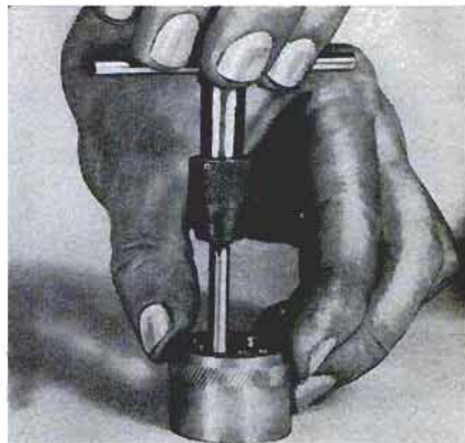
GUIDE FOR HAND TAP takes standard taps up to ½ in., assures straight, true thread and reduces tap breakage to minimum. Suitable for use with any tap, taper, plug or bottom type. Comes with wood holder Griffith Tool Co., 237 E. Crescent, Elmhurst, Ill.
