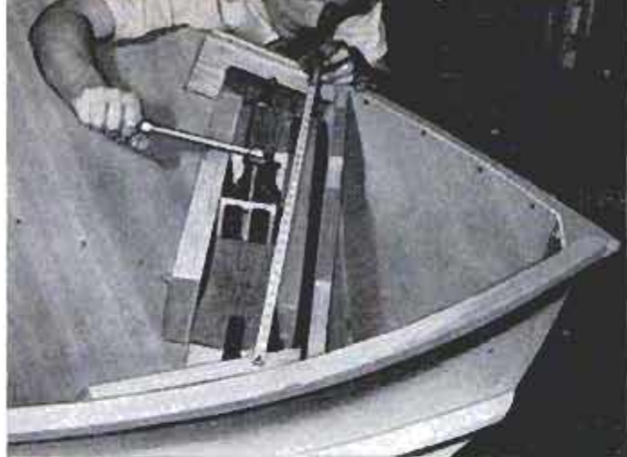
7. Hull-spreader jack can be made from scraps of wood or auto bumper jack can be used as shown here
