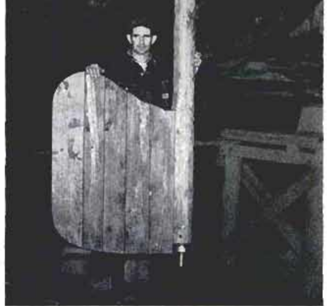
White-oak rudder has bronze bearing at foot of its six-inch post. Horizontal pins tie blade to post
