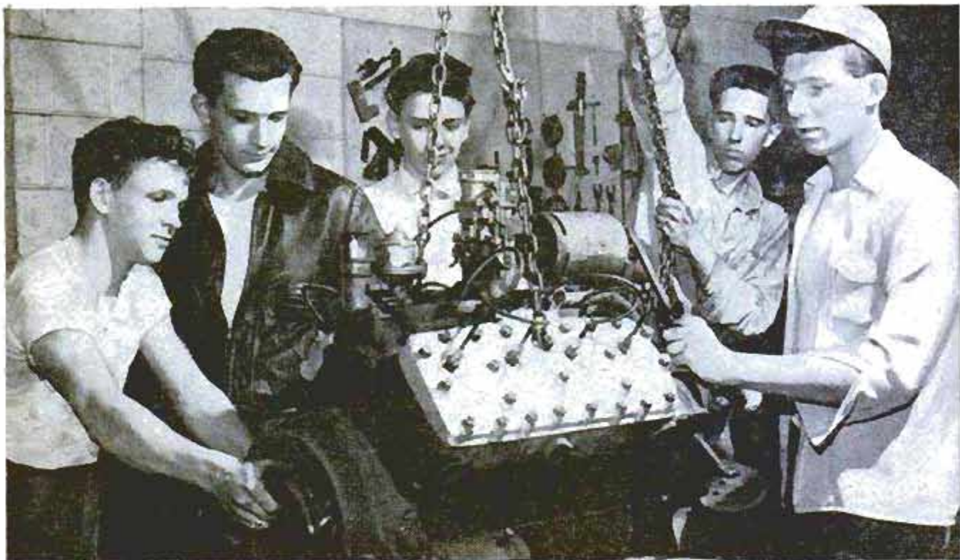
Complete overhauls are part of the program. These members are pulling a flathead V8 before tearing it down
