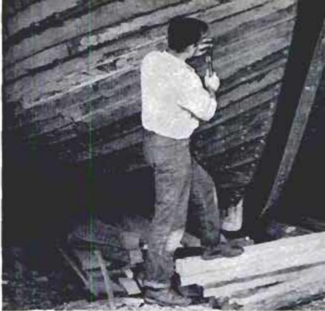
Each bolt and nail on exterior planking of hull was painted, countersunk and plugged with a wooden plug
