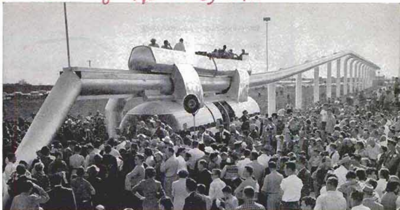
Monorail exhibit drew thousands. Height of rail at loading point is 10 feet. Standard operating height is 30
