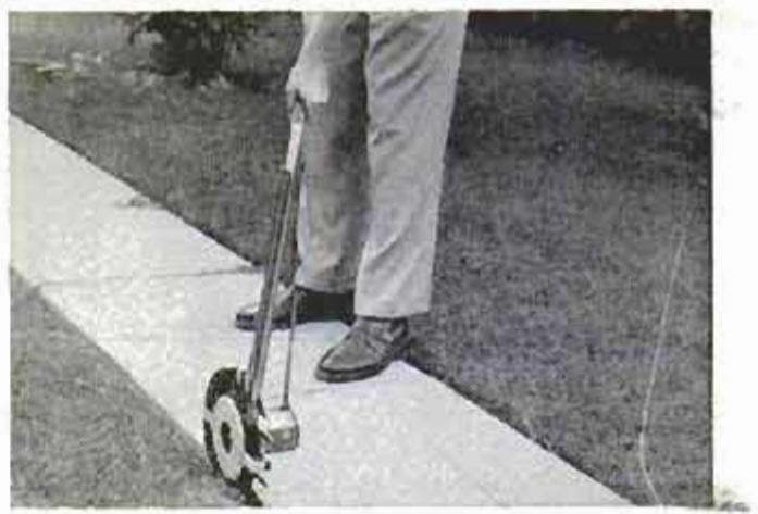
Equipped with long handle, blade is used in vertical position to edge lawn. Depth of cut is adjustable
