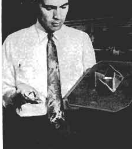
Metal diaphragm placed between tank and end of tube is ruptured on scored lines as gases explode into tube
