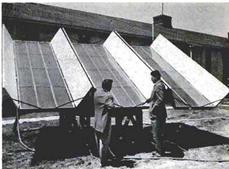
Heating surface of solar pump has 120 square feet, plus side reflectors to concentrate heat. The one-cylinder engine below the panels is run by steam from sulphur dioxide raised to the boiling point by the solar panels. It develops one horsepower
