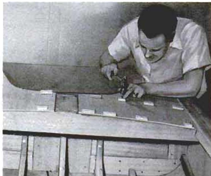
6. Plywood is "clamped" to deck beams while glue dries by using finishing nails in wooden blocks
