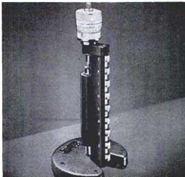
HEIGHT GAUGE has a micrometer head which raises and lowers a series of blocks, or steps, spaced 1 in. apart. Settings within .0001 are possible throughout the range of the instrument. Comes in two heights Brown & Sharpe Mfg. Co., Providence 1, R. I.
