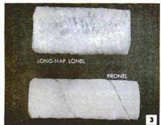
Mohair, above, is ideal for applying enamels. Its short nap holds less paint, flows enamels better. Long-nap lonel, below, is excellent for use on masonry. Pronel is used on fairly smooth surfaces
