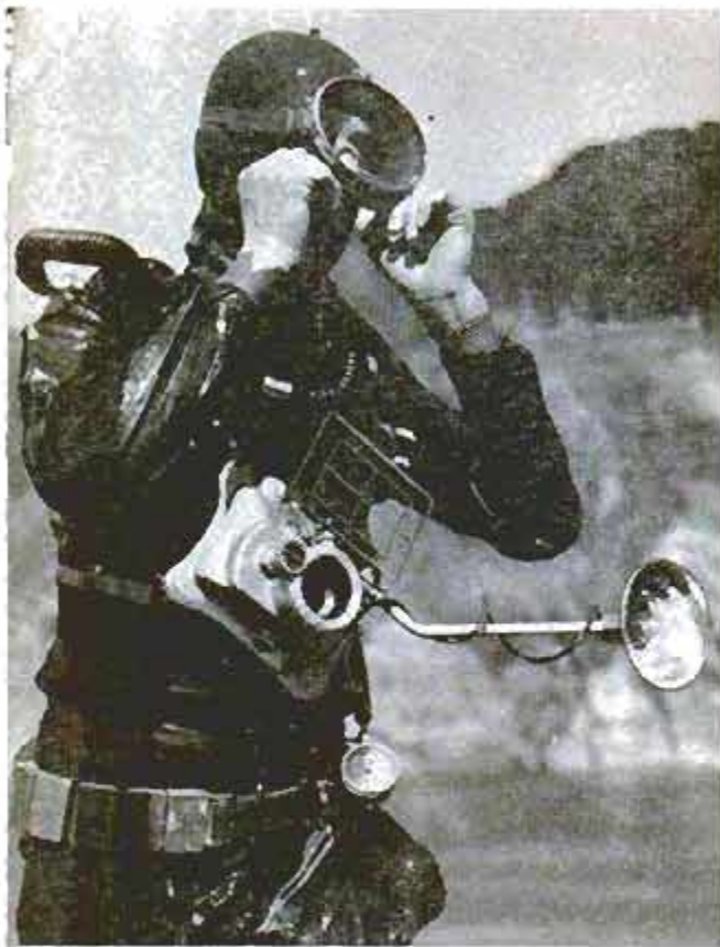
Watertight flash unit on underwater camera case permits taking color pictures far below the sea
