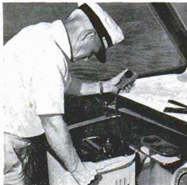
Queen Mary officer operates shipboard loran set. Time difference in arrival of two signals is shown on scope and indicated numerically on dial at lower left. Below, skipper uses set's remote-control dial
