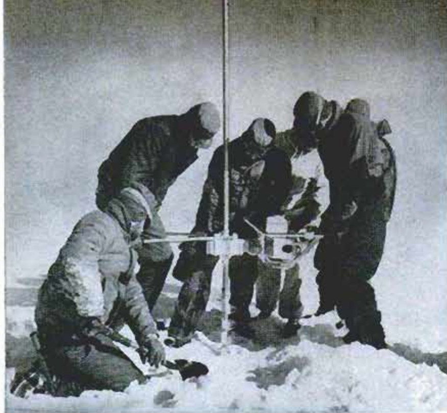
Seabees test thickness of bay ice with a 20-foot motor-driven auger to make sure ice will hold heavy vehicles. Below, icebreaking USS Glacier cuts 30-mile channel through 15-foot bay ice so ships can get closer to camp for unloading. Bow of ship is driven up onto ice to break it
