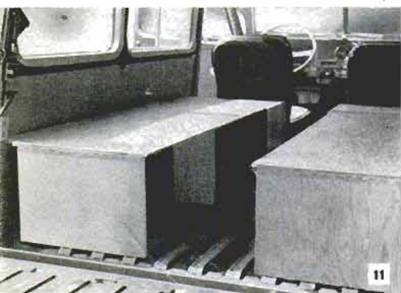
11 Above, bunk deck is attached by metal brackets to storage box forward and is supported by a member at rear fender well and a hinged end support. A sash lock secures end support to wooden runner on car floor. Right, lounge pads from outdoor furniture make comfortable, lightweight mattresses
