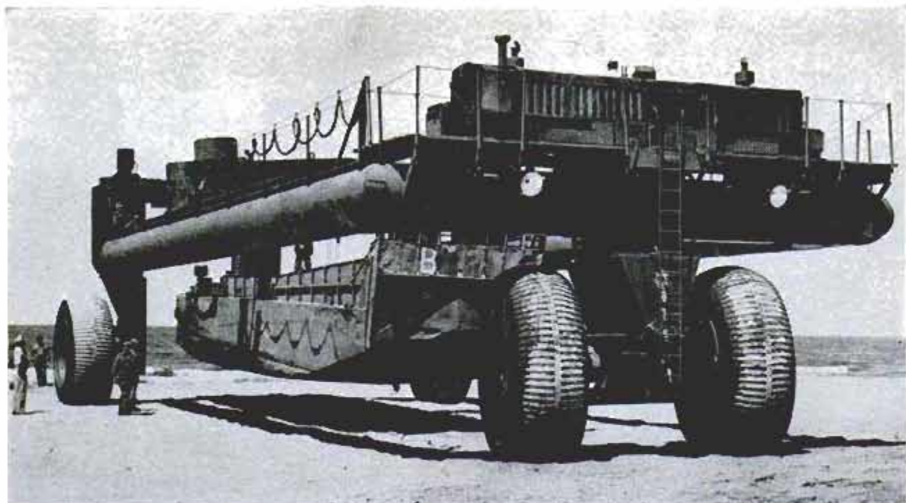
Heavy landing craft is dropped on the beach by the LeTourneau retriever at completion of salvage operation
