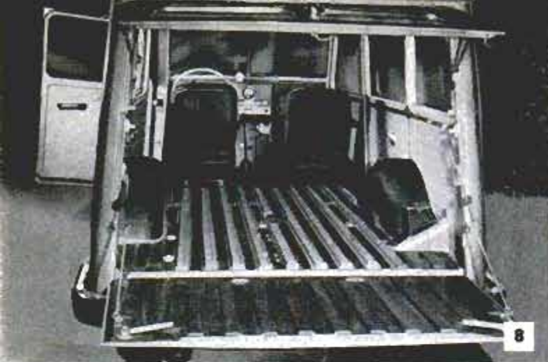
8 One of narrow back seats is converted to driver's seat to permit unobstructed movement inside car for convenience when en route or when wet outside
