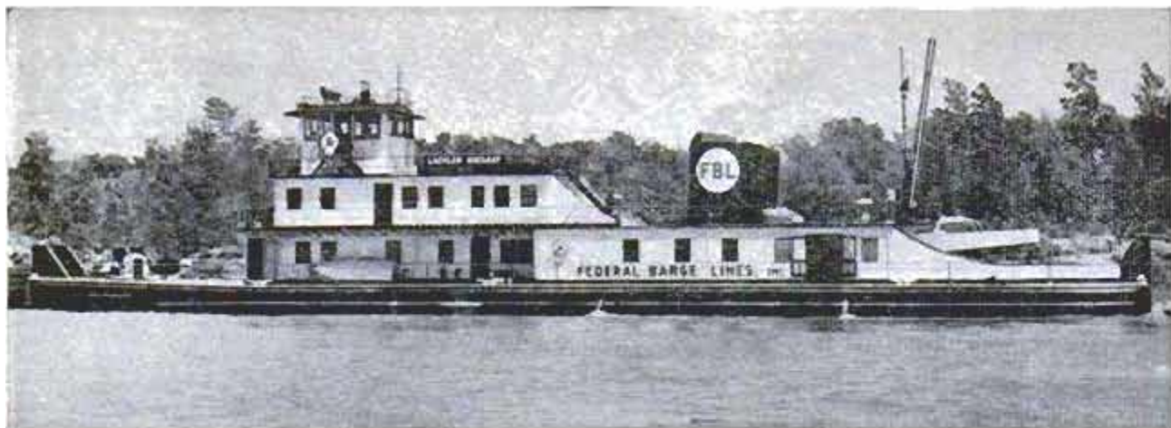
Lachlan MacLeay , 162 feet long and 45 feet wide, has a draft of 5½ feet, plies between St. Louis and Omaha
