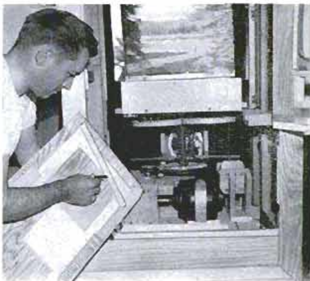
Electric motor drives shaft that turns worm gear to revolve pulleys. Set, with speaker hanging from it, turns on pipe standard. Below, picture takes place of TV screen when it is turned to the other side
