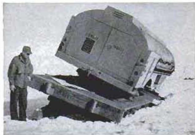
Narrow runners on this bobsled trailer could not support a 3000-gallon fuel tank on sugarlike snow
