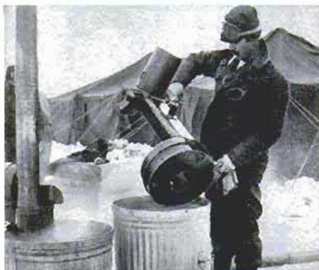
Hot water was obtained by placing immersion heater in can and shoveling in snow—25-gallon capacity
