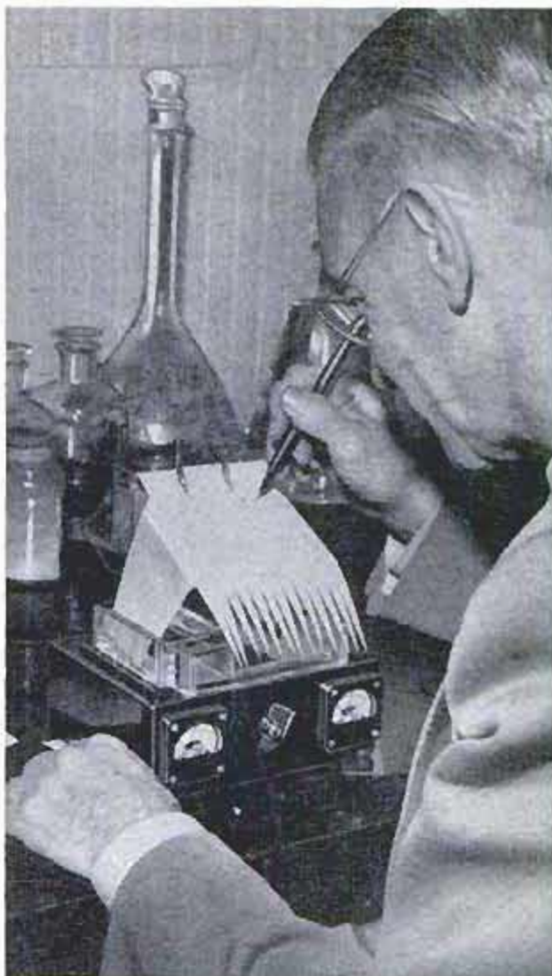
Electric current flows across filter paper in the electrophoresis method, separating the ingredients
