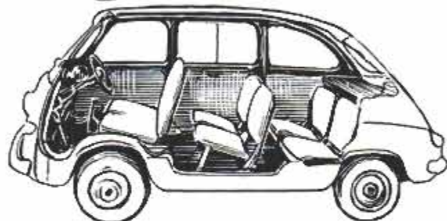
Above, Italy's tiny station wagon is rear-engined. Right, top two sketches show two seat variations. Rear seats in both versions fold as in lower sketch
