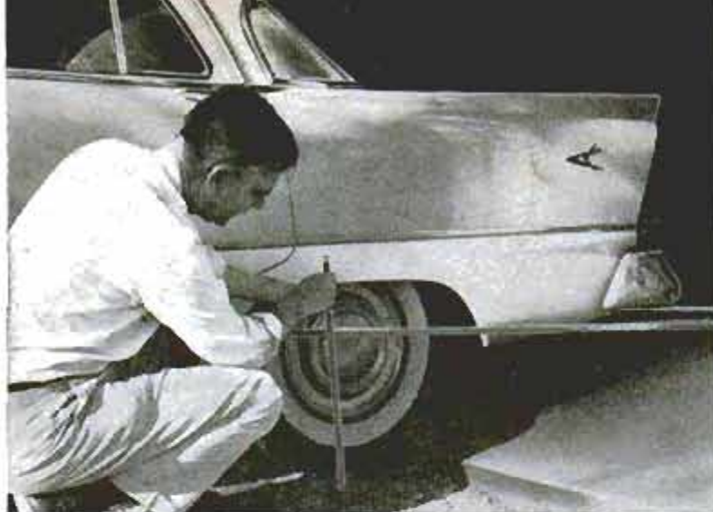
Like many cars, Plymouth has a long overhang that may damage tail pipe on steep incline like garage ramp, above. Photo below shows how little clearance there is as car descends the ramp
