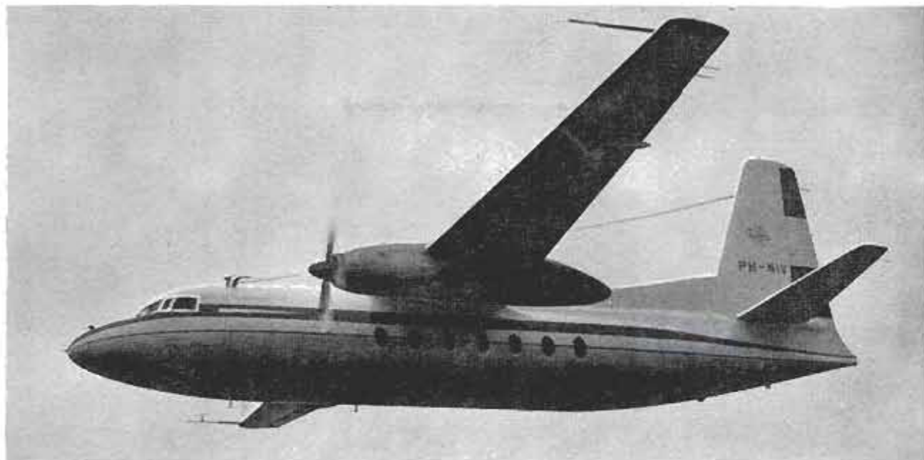
Fokker F-27 flies at 280 miles per hour, but lands at 75. It can carry up to 28 passengers comfortably
