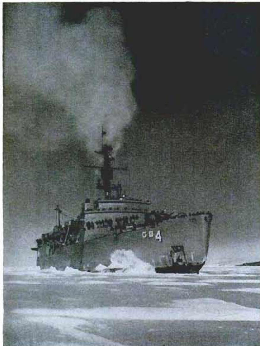
Seabees test thickness of bay ice with a 20-foot motor-driven auger to make sure ice will hold heavy vehicles. Below, icebreaking USS Glacier cuts 30-mile channel through 15-foot bay ice so ships can get closer to camp for unloading. Bow of ship is driven up onto ice to break it
