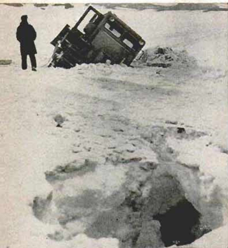
Snow-roofed crevasse near McMurdo base trapped 35-ton tractor that had to be winched out carefully
