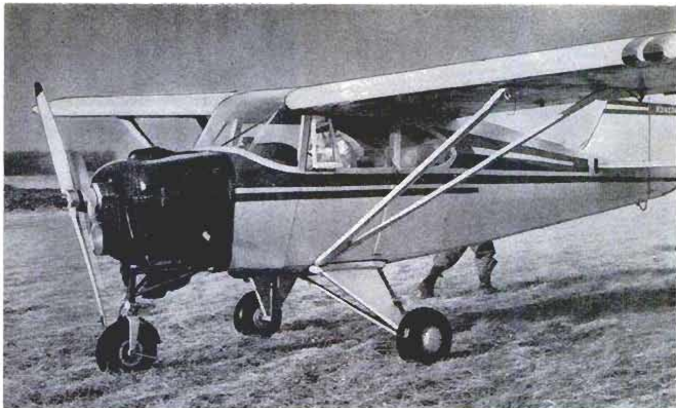
Back propeller linked through pulley to lower engine is spinning. Front propeller operates from top engine
