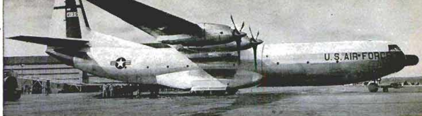
Newest transport by Douglas for the Air Force, the C-133A, carries a radar scanner in its big, black nose
