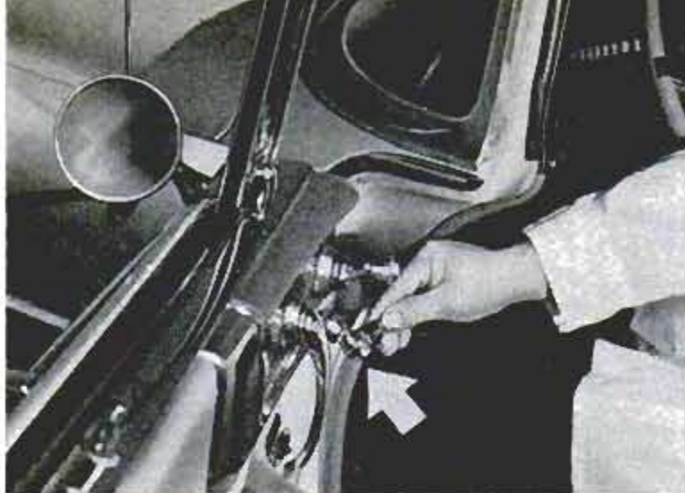
Owners report they like the rear-view-mirror control. Handle inside door (arrow) lets driver move mirror with window closed
