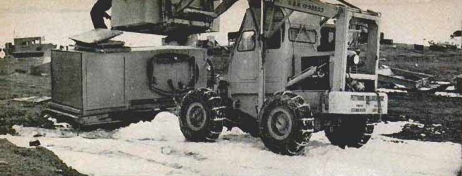
Snow melter, above left, produces 1000 gallons of drinking water per hour from four scoops of clean snow
