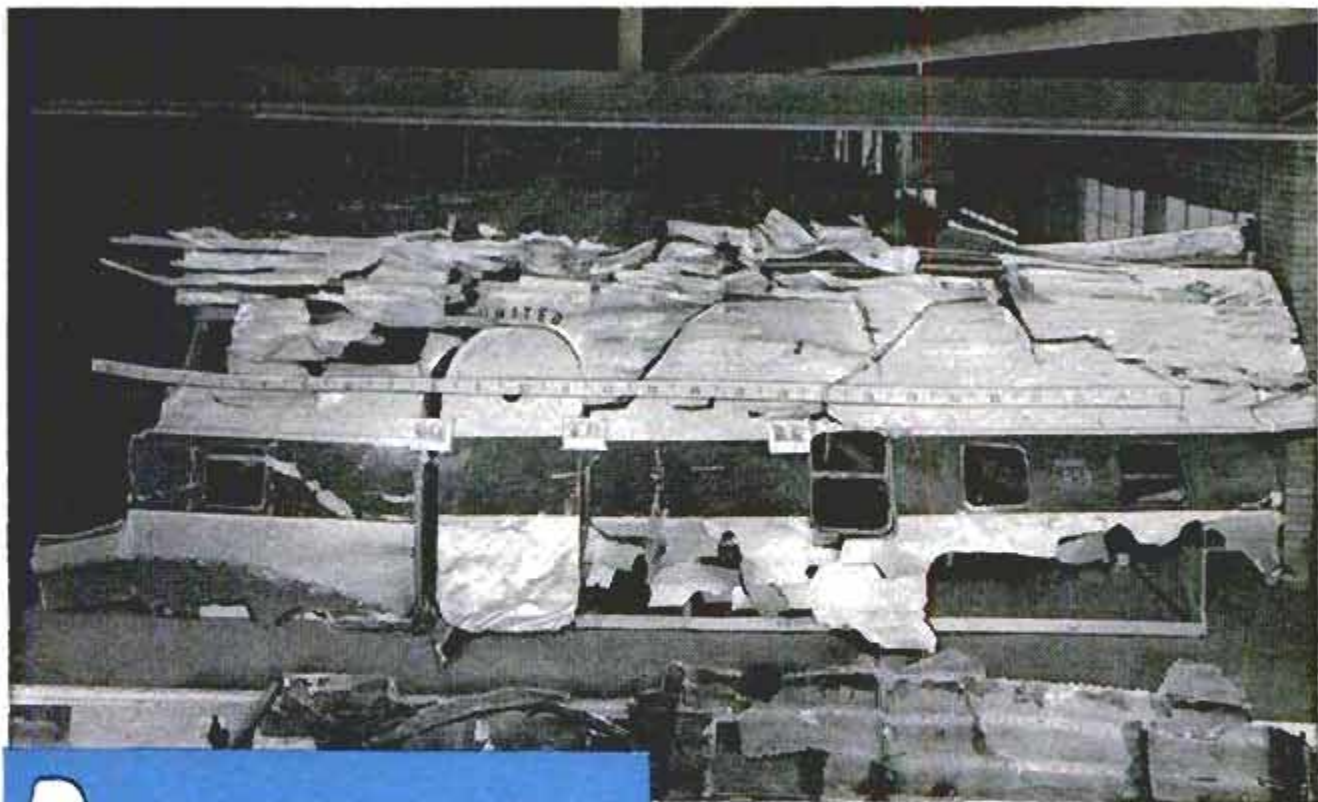
Like a giant puzzle, pieces of liner are put back together to confirm investigators' theories. This is section of fuselage containing No. 4 baggage hold
