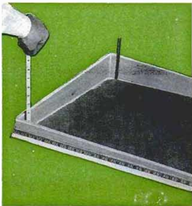
Above, the height of the box at its corners corresponds to the elevations at the corners of the lot. Below, surface of the sand should be shaped to approximate the contours and grades found on the lot
