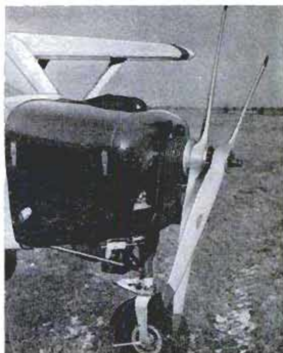
Top engine is installed upside down. Eight V-belts in separate grooves link back prop to lower engine
