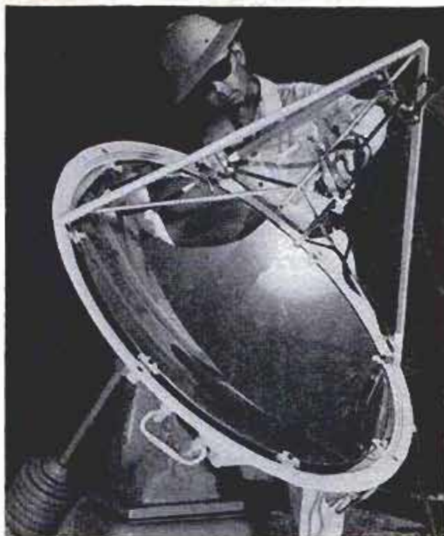
Solar engine called the Novoid produces pulsations through cycle of boiling water and condensing steam
