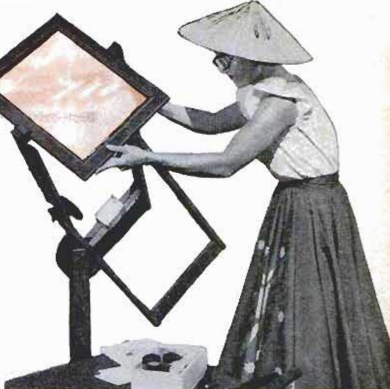
Pottery glazing with solar heat of over 1000 degrees is new twist to ancient art. Flat lens focuses rays
