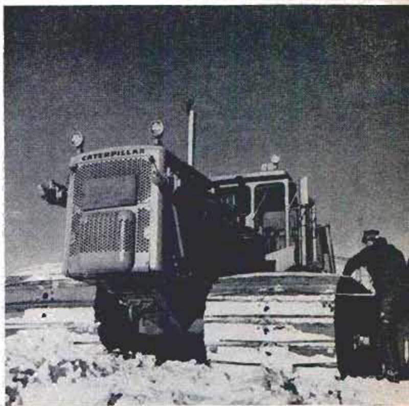
Even tractors wear snowshoes in Antarctica. This 35-ton prime mover has five-foot-wide steel tracks
