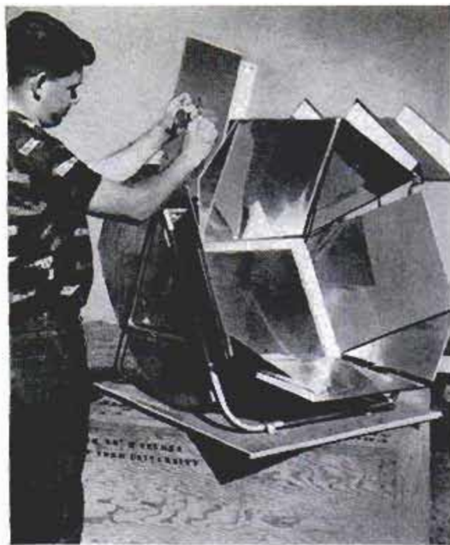
Solar stove with one glass wall which can be pointed toward sun. Aluminum side panels concentrate heat
