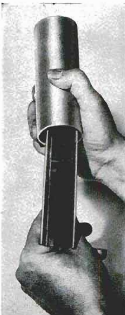
Kaleidoscope is made by taping two long mirrors at V-angle into tube. Weegee demonstrates device's image-dividing effect
