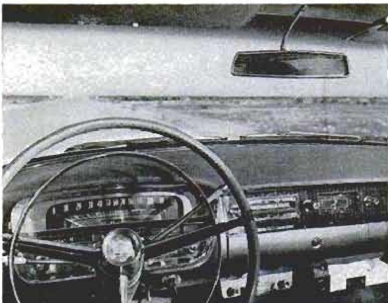
Above, new this year is the center-mounted brake pedal. It straddles the steering column and is easily operated by either foot. Below, some owners complain about the extra-big horn ring. It is too close to the steering-wheel rim for comfort
