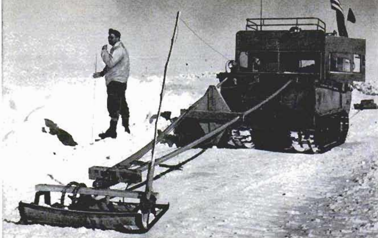
Probing electronic boom on crevasse-detector Weasel locates hidden cracks that booby trap snow vehicles
