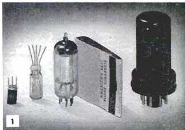
Tiny transistor, left, is dwarfed by conventional subminiature, miniature and standard vacuum tubes
