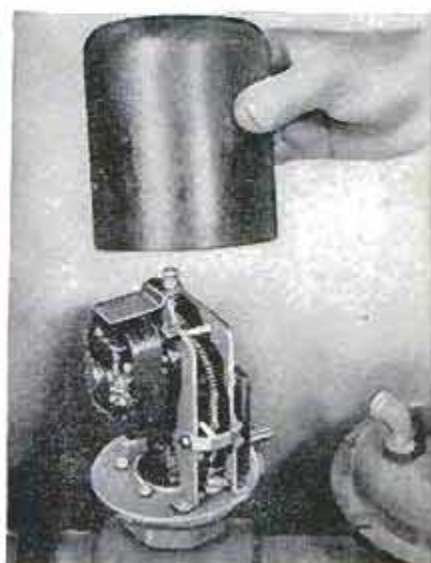
Tiny motors that operate clocks, gas valves and similar units require application of special oils
