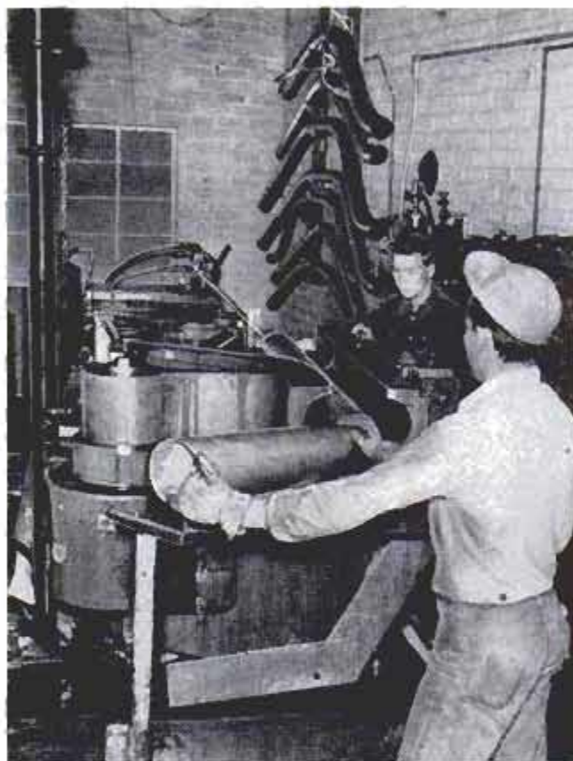
Array of different shapes for irrigation tubes can be seen behind the press, above, which produces them
