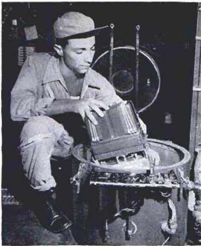
Airman inspects dropsonde that is dropped through storm by parachute and sends information by radio
