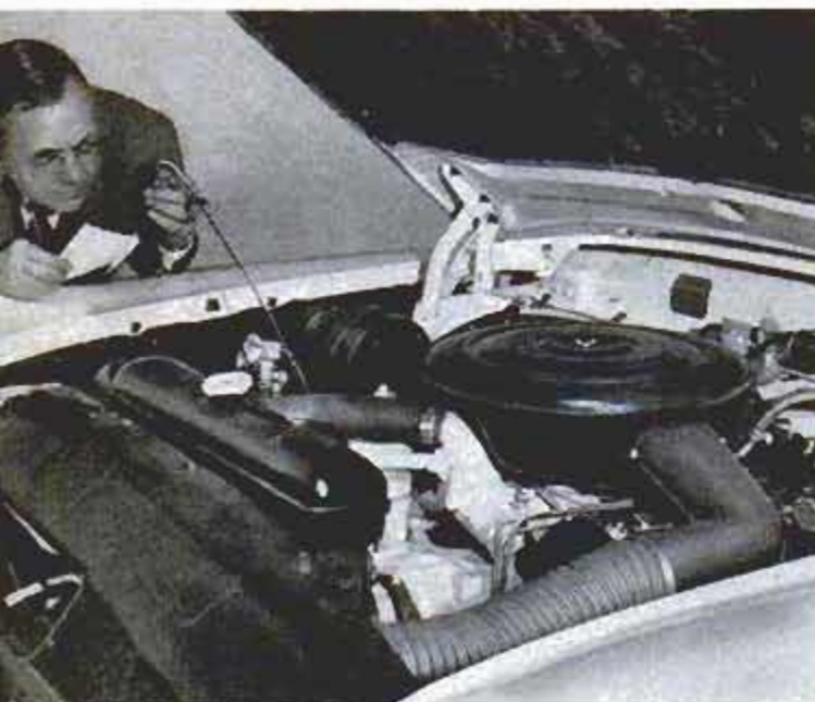
Carburetor air is drawn through grille via duct in foreground. Despite crowded compartment, long dipstick is easy to use. Below, accelerator linkage is "suspended" to eliminate need for hole in floor mat
