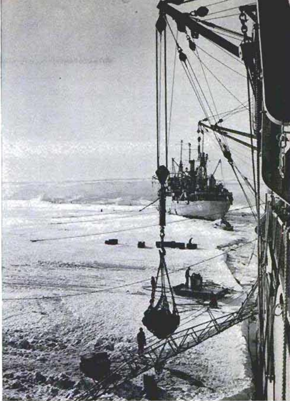
Supply ships of a previous expedition tie up to "dead men" sunk into the ice shelf. Then cargo nets start dipping out tons of supplies
