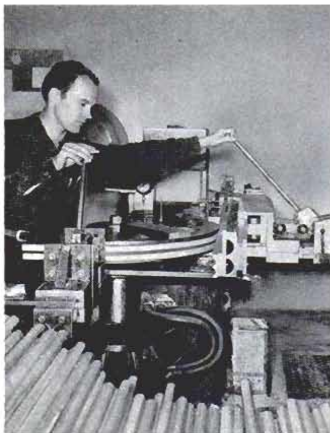
Tubes of small diameter, used to irrigate a single furrow, are bent two at a time in hydraulic presses
