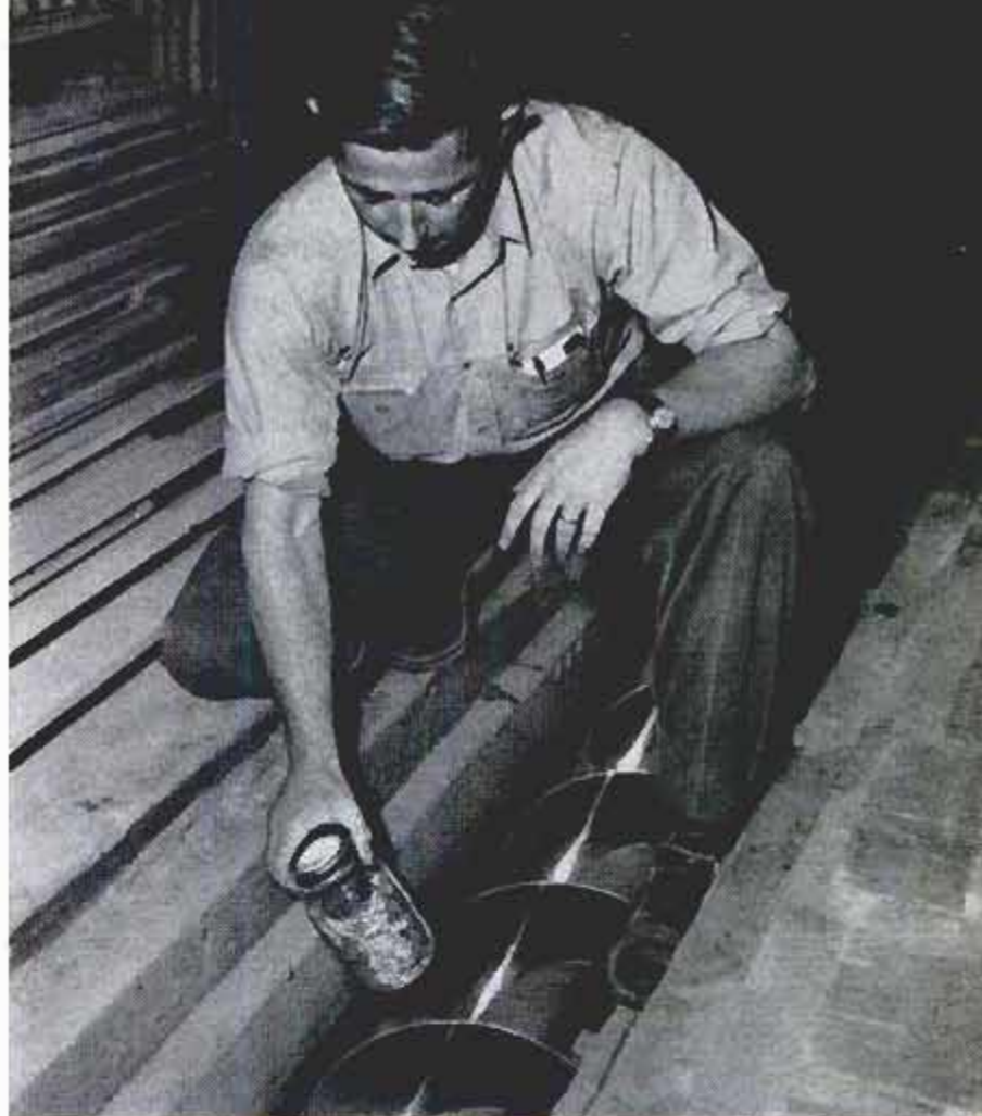
Live khapra beetles in screened Mason jar are placed in screw conveyor. Channel was then covered for test of gas penetration
