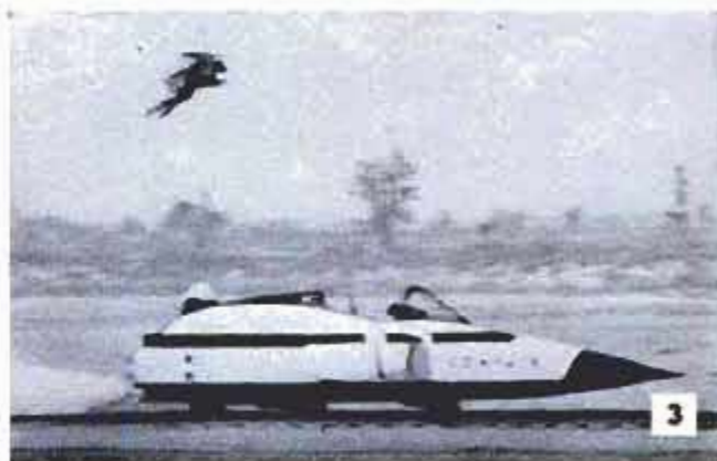
4. Pilot coming down safely under parachute. Below, sled is built for 16 rockets, but so far no more than eight have been used. Two of 10 rockets shown are used to sustain top speed. Water brake stops sled
