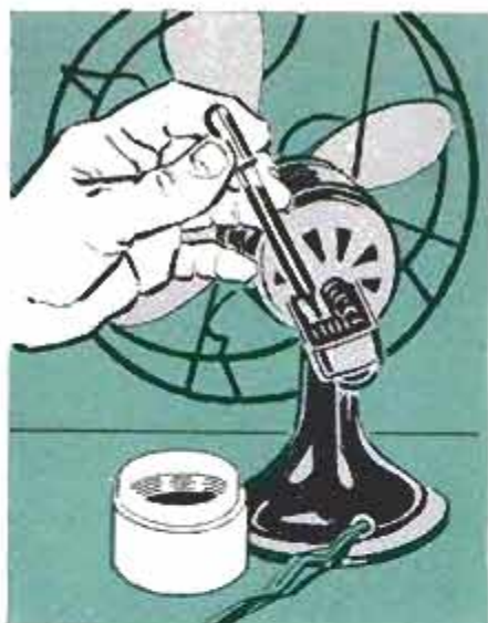
The oscillating mechanism of an electric fan usually requires a special gear oil applied sparingly
