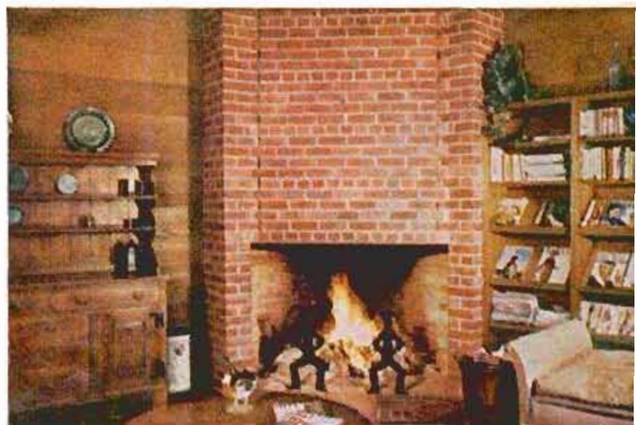
Above, serving as a room divider, this variation of the Swedish fireplace gives firelight to both living and dining rooms. Flue must be extra large so cross drafts won't force smoke sidewise. Below, corner type takes little floor space
