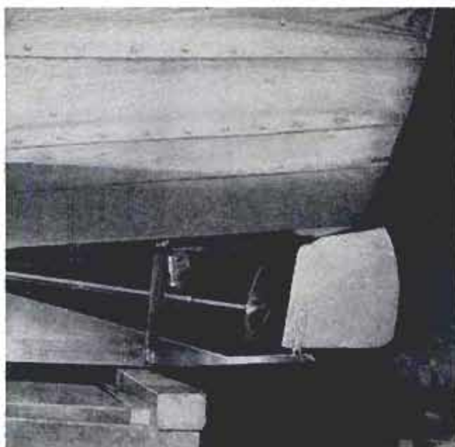
Deadwood area of the keel is cut away, making the boat respond more quickly to the oversize rudder
