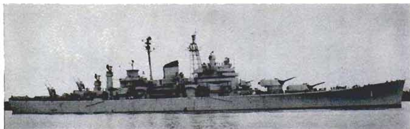
Tests of the supersonic Terrier missile were conducted from the USS Mississippi (above) before the USS Boston (below) was reconditioned as first guided-missile cruiser. The Boston is 673 feet long
