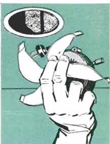
Some kitchen fans have motors operating in a vertical position. Clean motor thoroughly after servicing
