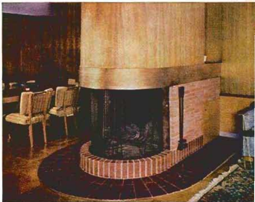
Above, serving as a room divider, this variation of the Swedish fireplace gives firelight to both living and dining rooms. Flue must be extra large so cross drafts won't force smoke sidewise. Below, corner type takes little floor space
