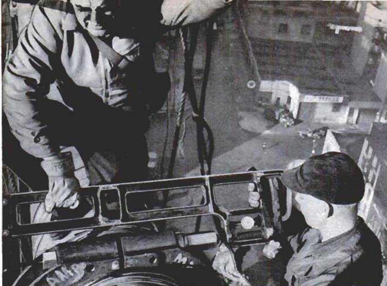
Investigators measure elongation of band bolts under stress, to determine maximum allowable stress in bolts
