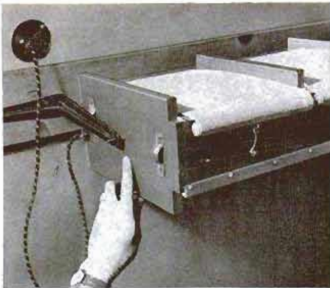
Drier rotates on "axles" consisting of \frac{1}{4} -in. bolts. Axles fit in slotted holes in metal shelf brackets
