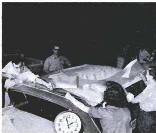
1:58 p.m. Masking for second color (light green). This is a big operation now because of two-tone fad
