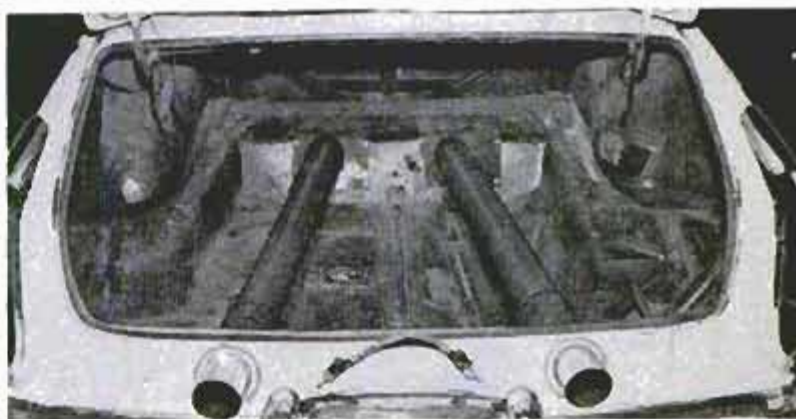
Top, Ford tailpipe crossover lets the driver hear the exhaust of troublesome right bank of cylinders. The Chrysler tailpipes run straight back through trunk
