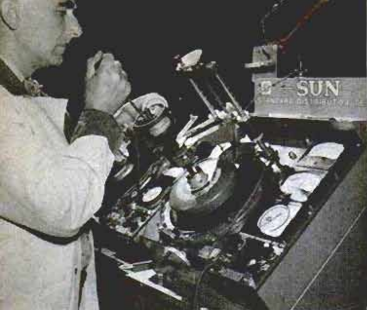
3. Calibrating distributor on tester synchronizes spark so it reaches each cylinder at right time
