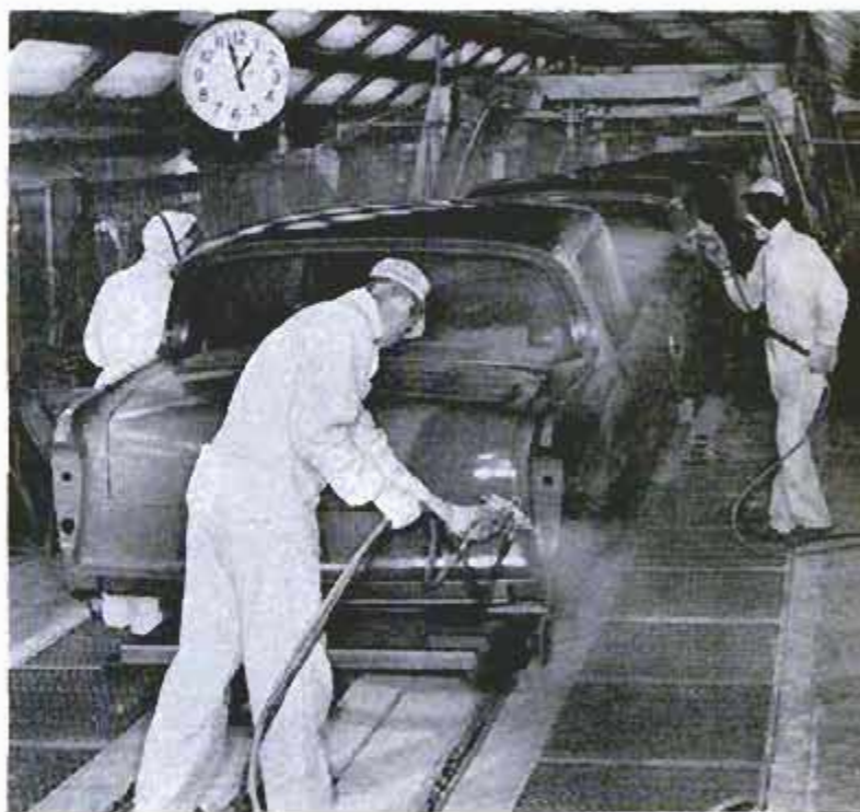
12:58 p.m. First color (dark green) goes on. Arch in background is an automatic paint-spraying machine
