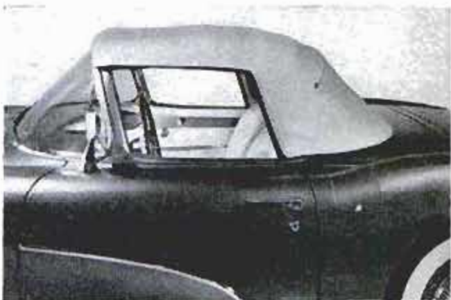
Top operation is automatic: First, the lid lifts up; next, up comes the top; finally, the lid closes itself
