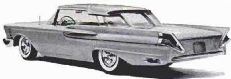
MERCURY Turnpike Cruiser is only 53 inches high. It seats four. Roof sections lift when doors open. Stoplights are recessed into edge of roof above the full-wrap side windows
