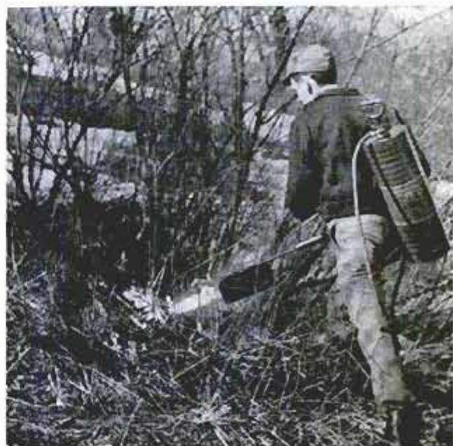
Above, winter uses for a weed burner are clearing snow and ice from driveways and walks and thawing the frozen water pipe you forgot to drain the night before. Below, flame-girdling kills unwanted shrubs
