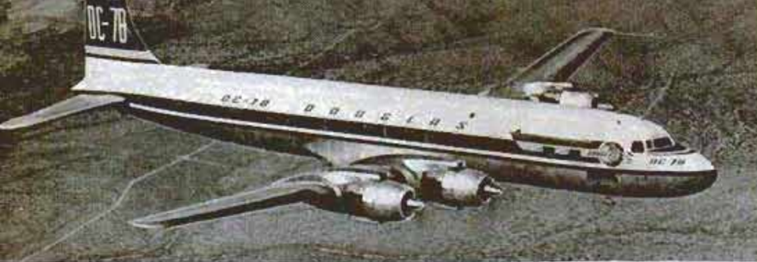
Turbocompound engines are now in use on many airliners, such as the Douglas DC-7B at the left and the Lockheed Super Constellation below
