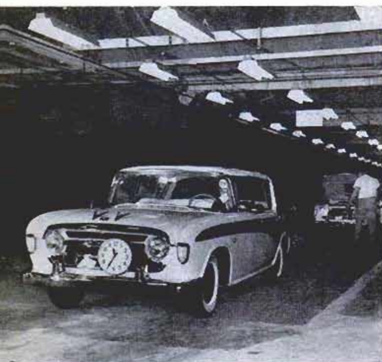
11:35 p.m. First time it moves under own power. It is now run through gears with rear wheels on rollers
