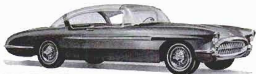
PACKARD Projector has stylized version of famed Packard radiator as vertical bar in front to act as grille guard, eliminating line-breaking bulges on bumper. Lights retract to enhance clean look. No chrome is used, not even around glass. Roof rolls back as door opens
