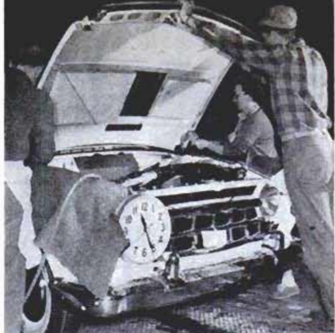
11:26 p.m. Hood is bolted on. It must have proper color, must wear the right emblem, Hudson or Nash
