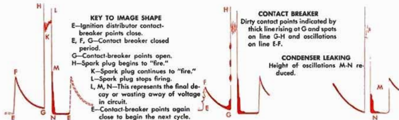
2. Upper photo, oscilloscope used with dynamometer gives picture of condition of ignition system. Below, key to image shape and two images which result when condenser leaks and contact points are dirty
