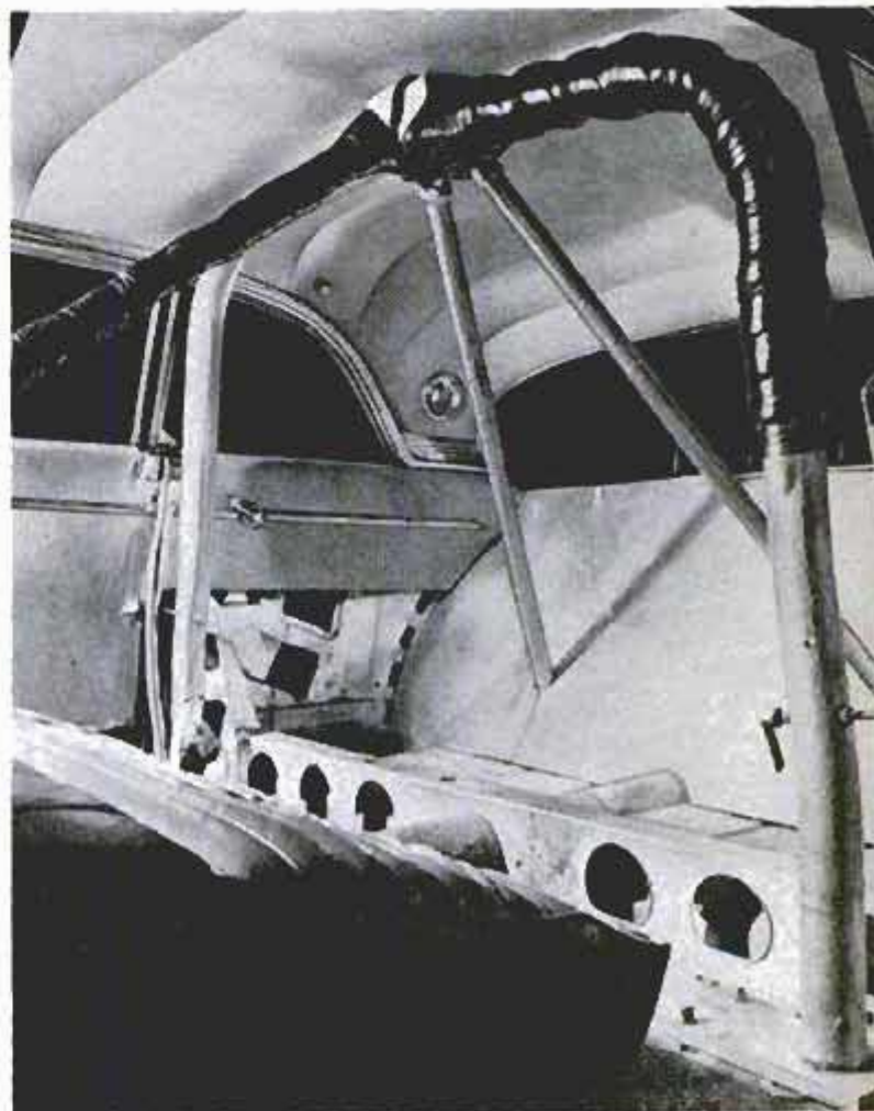
Rules require safety rollbar. Kiekhaefer adds three braces to stiffen frame and make car corner better
