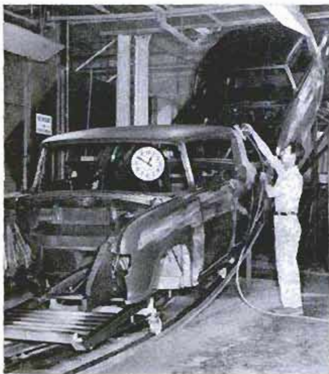
12:50 p.m. As body leaves drying oven after prime coat, it is sanded down to ready it for first color
