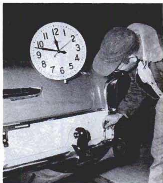
11:48 p.m. Final inspection. Any tiny blemishes in paint are touched up as car moves toward end of line
