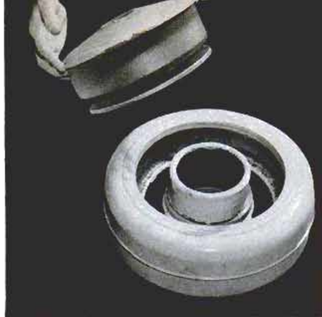
7. Tune-up includes cleaning and reoiling air cleaner. Cleaner has direct effect on carburetor efficiency
