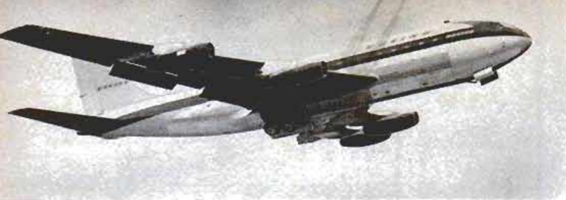
Two new jetliners due for service in 1958 are the Boeing 707 and Douglas DC-8. Both have engines suspended under wings
