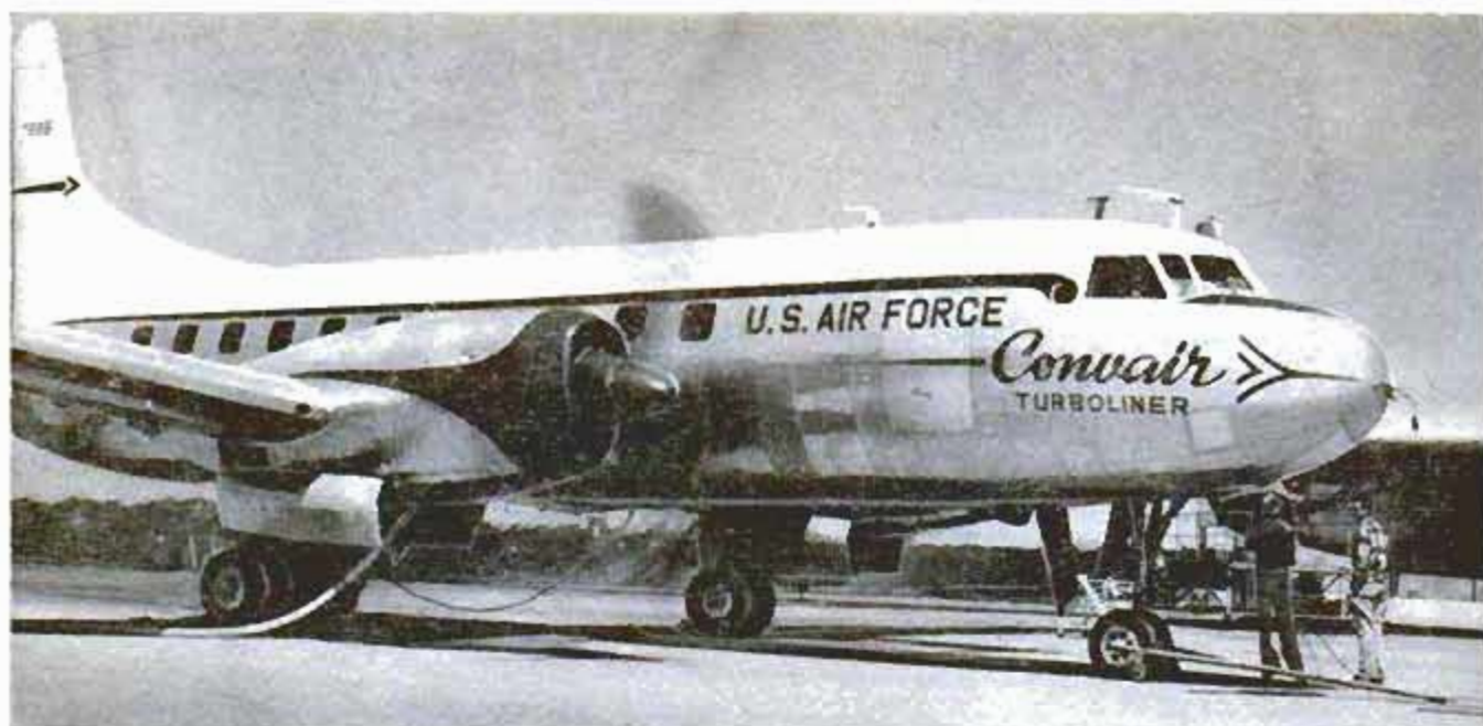
Present-day airliners, like the Convair above, are being tested for operation with turboprop engines
