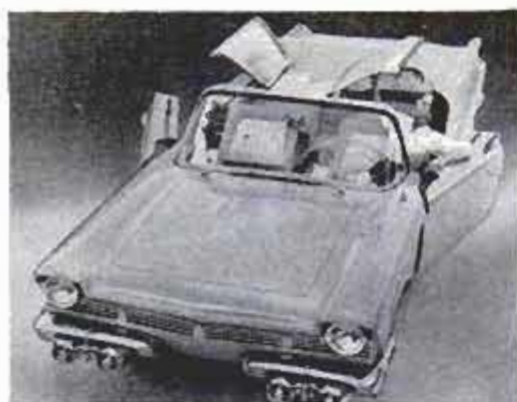
MERCURY Turnpike Cruiser is only 53 inches high. It seats four. Roof sections lift when doors open. Stoplights are recessed into edge of roof above the full-wrap side windows
