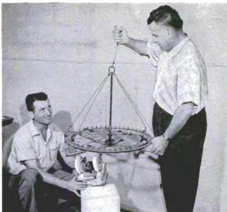
Yost and Macgowan examine their creation. Alarm clocks are encased in box below wheel. Pamphlets hang from rim of wheel
