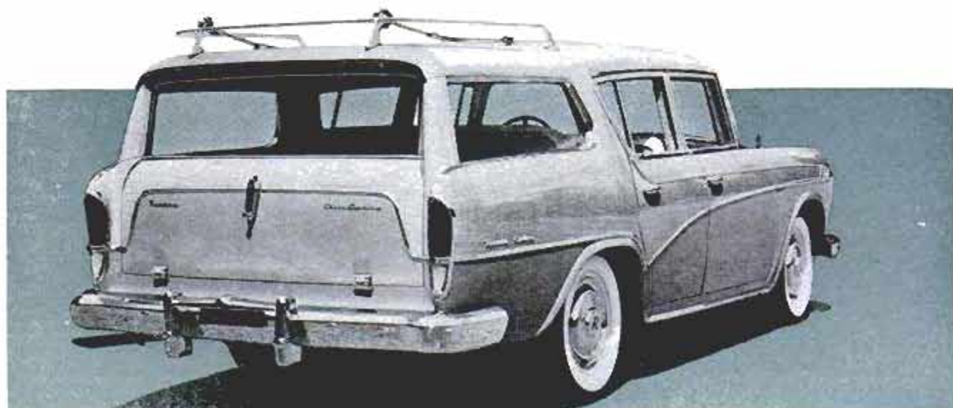
Above is the newest idea in body styling for 1956: a station wagon with four-door hardtop styling. It has no center posts between the doors. Below, the regular four-door wagon, known as the Cross Country
