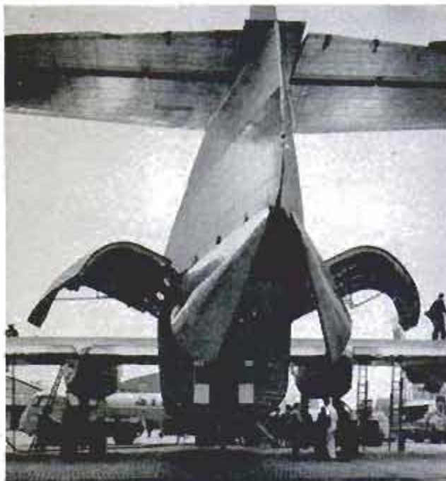
Unique construction of fuselage permits entire lower rear section to open for access to cargo hold
