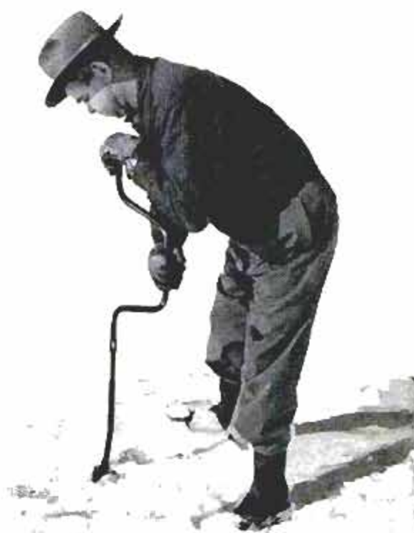
Drill designed for ice fishermen works like carpenter's brace. Below, heavy chisel is favorite tool
