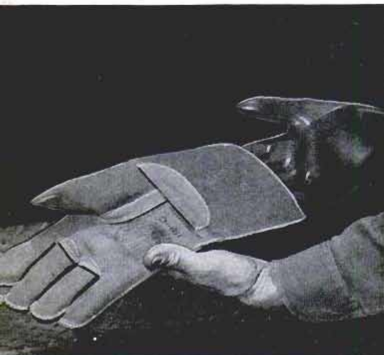
For work on a line carrying up to 7500 volts the lineman wears rubber gloves inside leather gloves. "Hot stick" is used to place fuse in top clip of holder. Other end of stick shoves it into bottom clip
