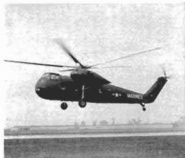
Developed as an assault transport for the Marines and comparable in size to a DC-3, the Sikorsky XHR25-1 carries 26 troops at 150 miles per hour
