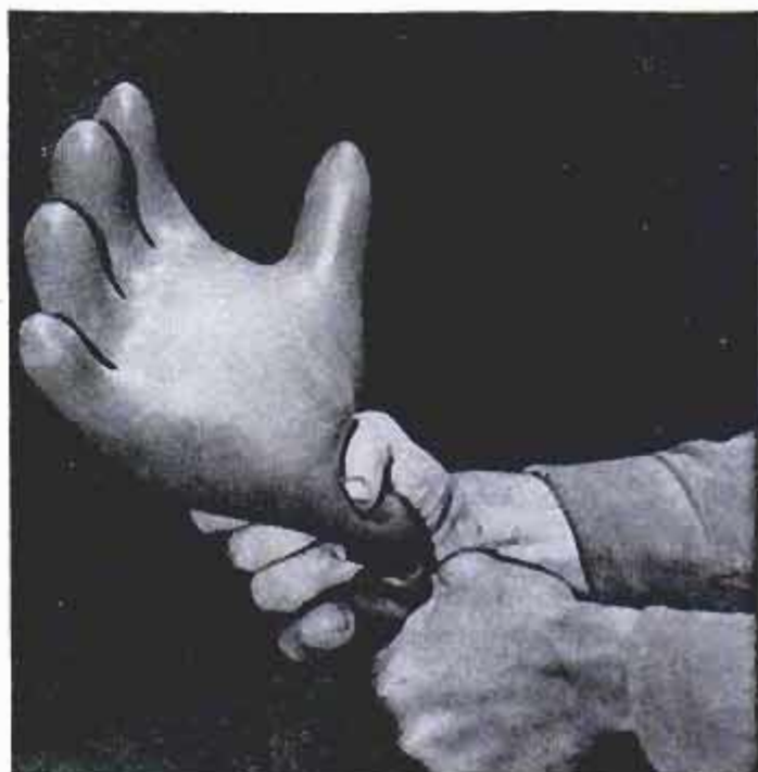
Rubber glove gets its daily roll test. A pinhole could be deadly. Below, this hot stick is lineman's socket wrench, used for clamping together two cables. Sticks are rotated to grip clamp, join nut and bolt
