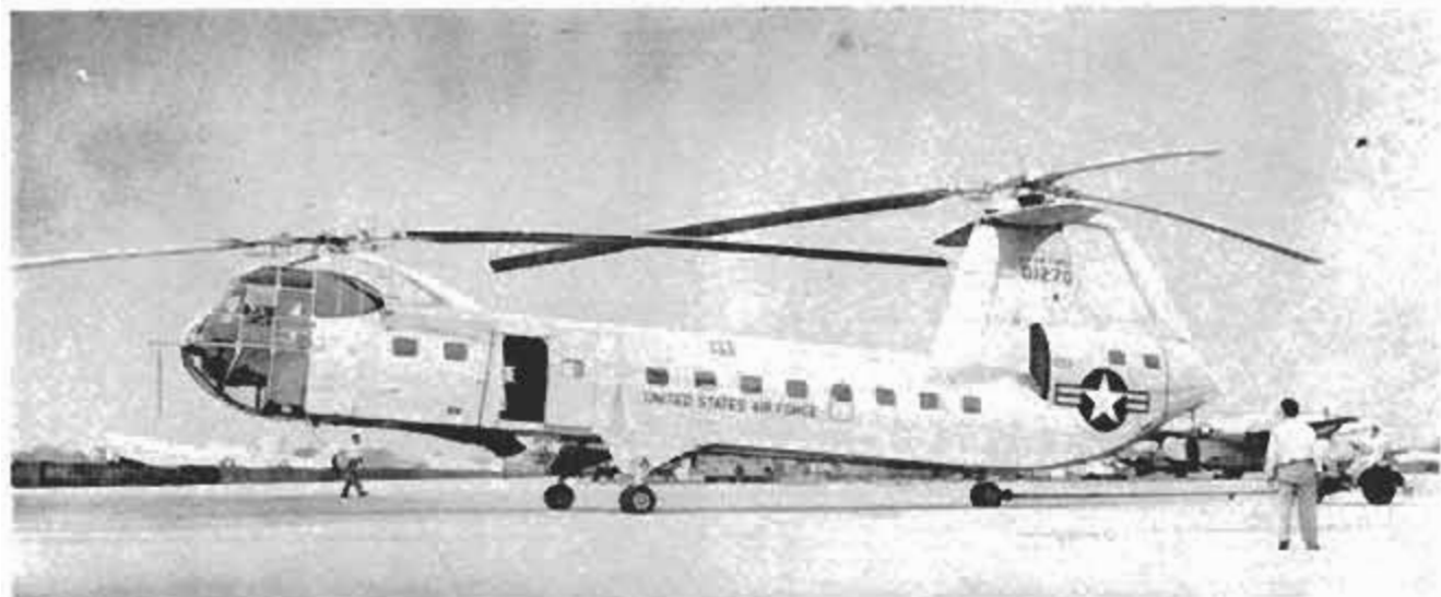
World's largest tandem-rotor helicopter is the Piasecki YH-16A. Each rotor is 82 feet in diameter and each is driven by an Allison shaft-turbine engine of 1800 horsepower. It can carry 40 fully equipped troops
