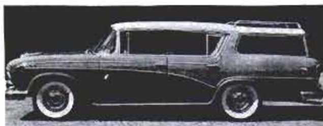
Above is the newest idea in body styling for 1956: a station wagon with four-door hardtop styling. It has no center posts between the doors. Below, the regular four-door wagon, known as the Cross Country
