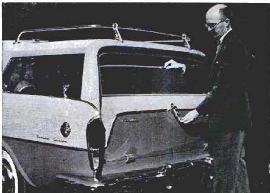
Featured on the Rambler station wagons is a crank-down rear window. It provides excellent ventilation and eliminates the transom-type top half of the door. The crank handle is outside and has a lock in it. You get an idea of the lowness of the new body here. Over-all, it is 58 inches high
