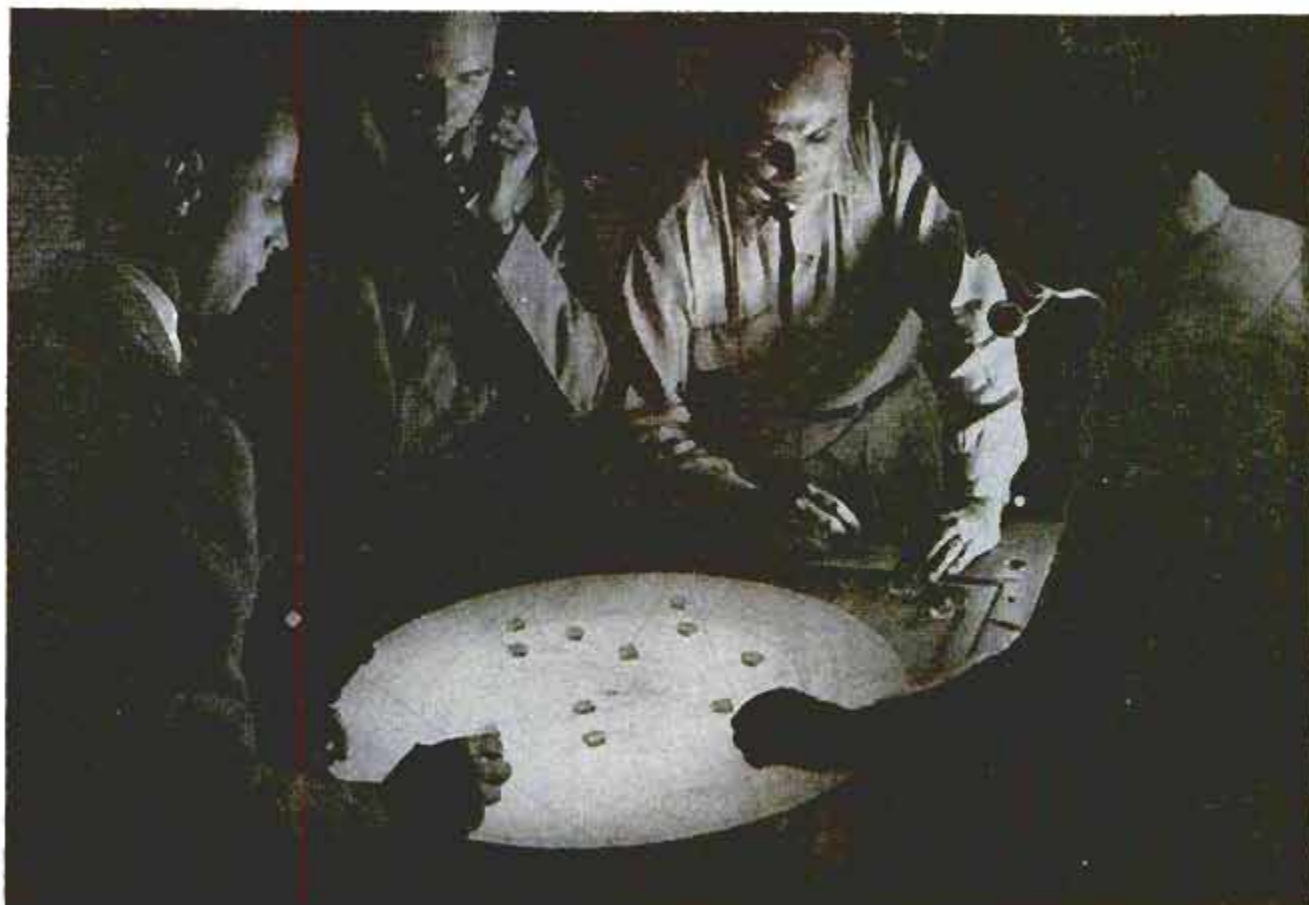
In experimental setup, radarscope is projected on glass table. Controllers move markers as the blips move
