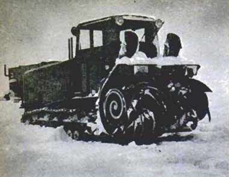
Snow digger is type used to clear mountain passes. Painted swirls on hubs warn when rotor is in motion
