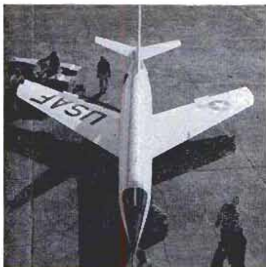
New Bell X-2 will be carried to flight altitude in bay of B-50 bomber which has been redesigned for the job
