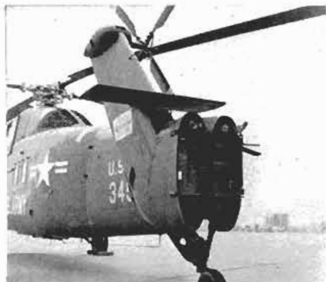
Sikorsky H-34A is the Army version of the Navy's HSS-1. The tail folds for stowing on a carrier, and the Army retained this feature for economy reasons
