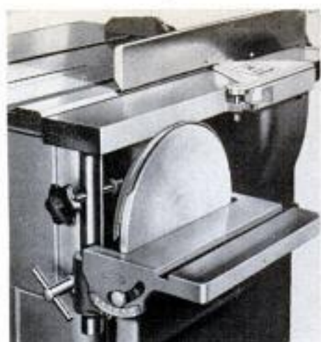
Sander is easily removed to expose power take-off for quick attachment of accessories. Powered by friction drive
