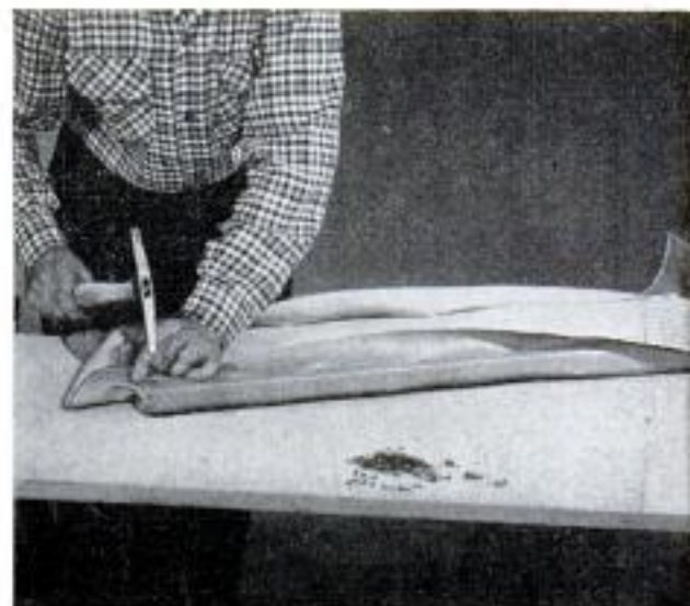
Foam rubber 1 in. thick is ideal for padding under the covering material, which may be any type desired
