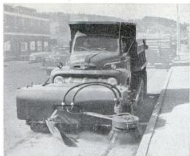
Sprinkler holds down dust as street-sweeper attachment picks up dirt in bin. Broom is 72 inches long
