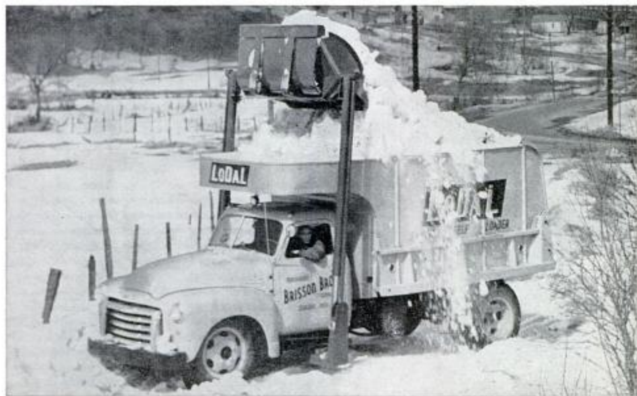
Combination of sideboard assembly and special refuse lip on bucket solves refuse-collection problems
