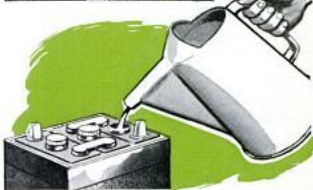
You can use any type of container to add water, but don't. Use a syringe and keep battery clean
