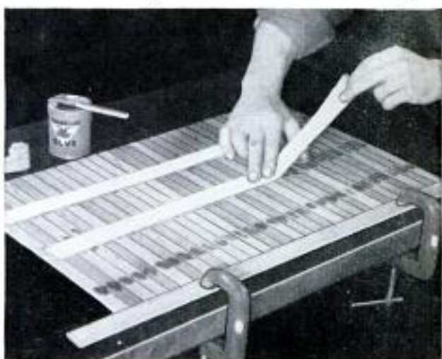
Butt the door slats against a straightedge and square them before joining with strips of cloth tape
