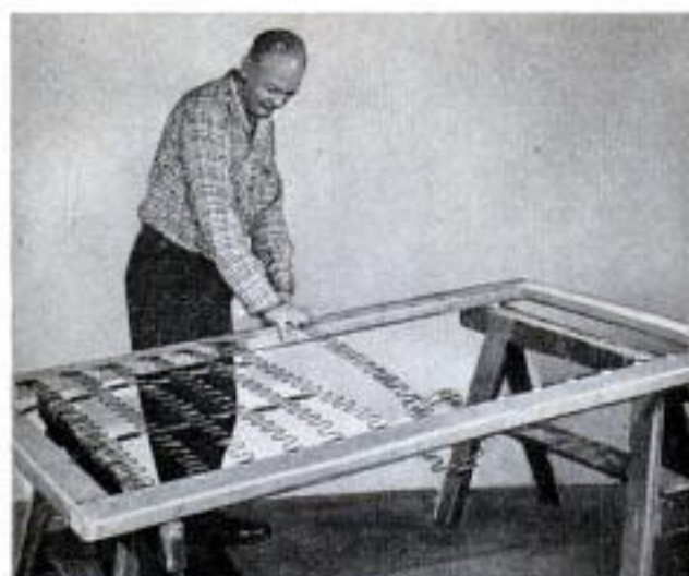
Sagless-type springs are fastened to frame of yellow pine 2 x 4s butt-joined and doweled together
