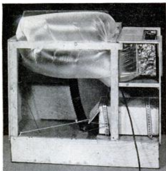
Rear view of accordion organ with back panel removed shows air bag and hose connection to blower
