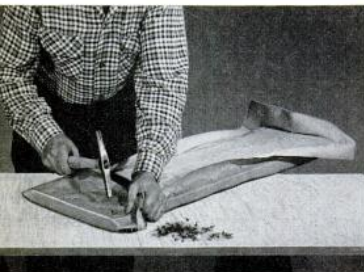
Storage units are faced with upholstered panel of ½-in. plywood which is screwed in place on the unit
