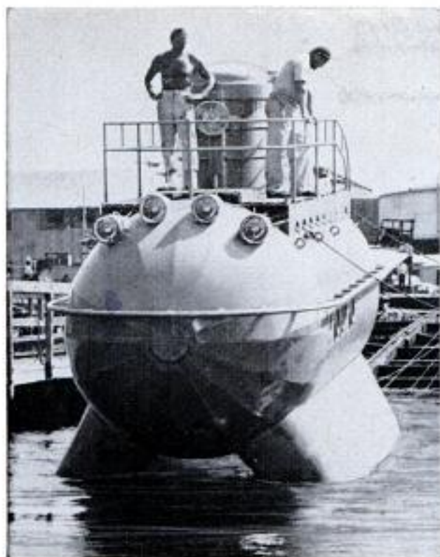
Craft enters water for trim trials. Fat "legs" support it on ocean floor and carry storage batteries
