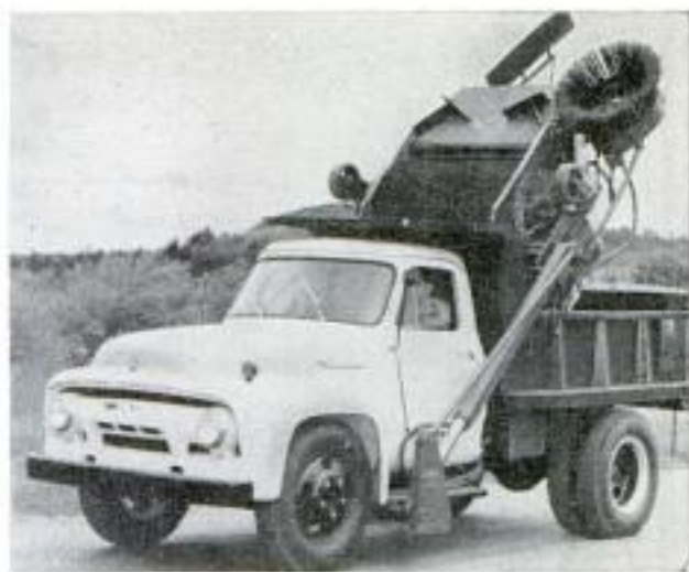
When the street-sweeper bin, with 1/2-yard capacity, is full, it is emptied into the dump box of truck
