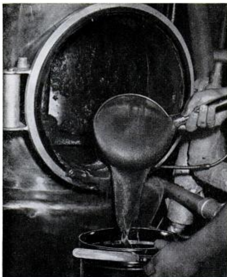
Tomato juice is concentrated into a semisolid inside a vacuum evaporator. Concentrate is spread on trays for further drying
