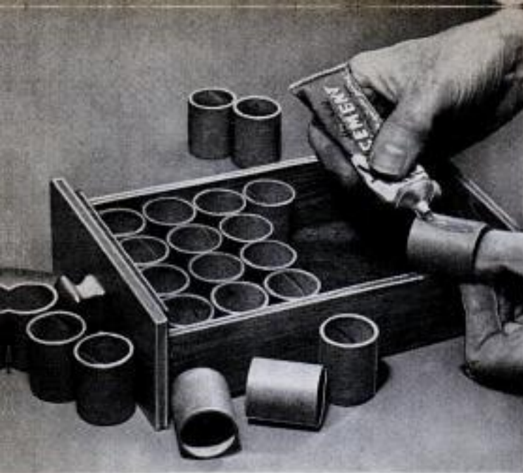
Storage drawer utilizes tube sections which are dipped in shellac or glue size and then glued together
