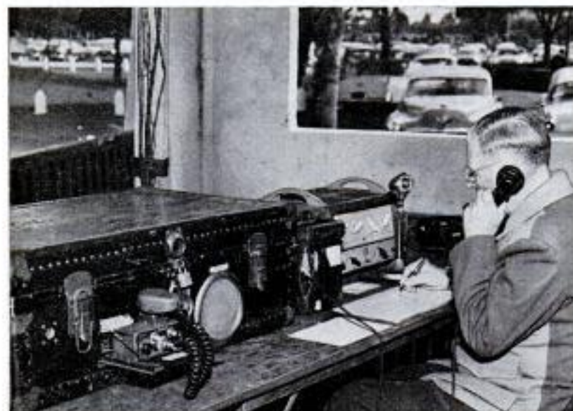
Portable radio transmitter built by Communications technicians is used at Miami-sponsored golf tournaments, parades and other special events. Speedphoto unit in Communications Center sends and receives photos, information, fingerprints of dangerous wanted criminals
