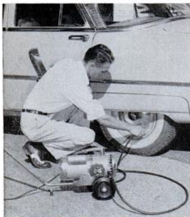
Because of its oilless construction, the compressor delivers clean, dry air without need of separator
