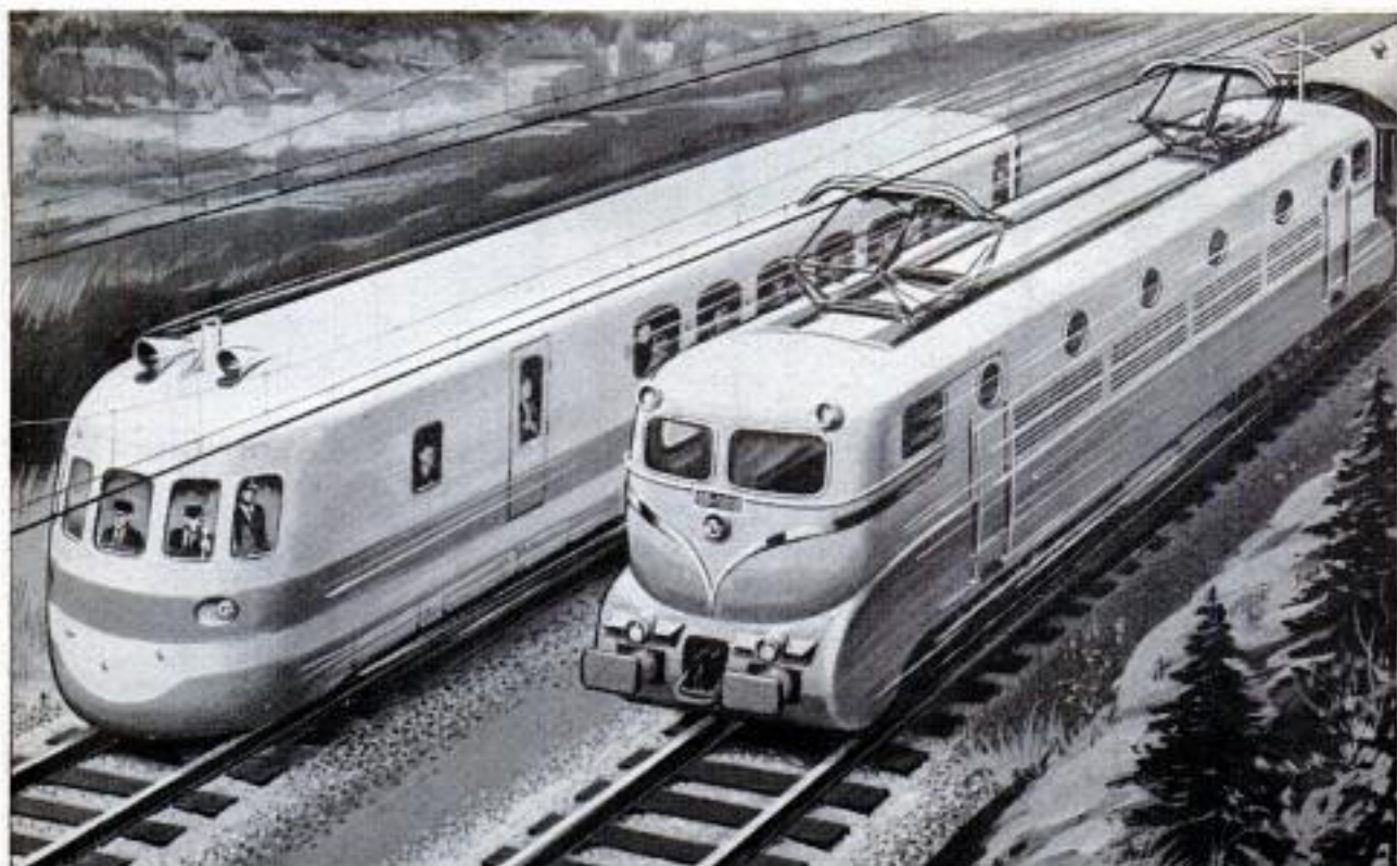
Officials in diesel railcar at left send verbal orders which are relayed to controls in robot train at right
