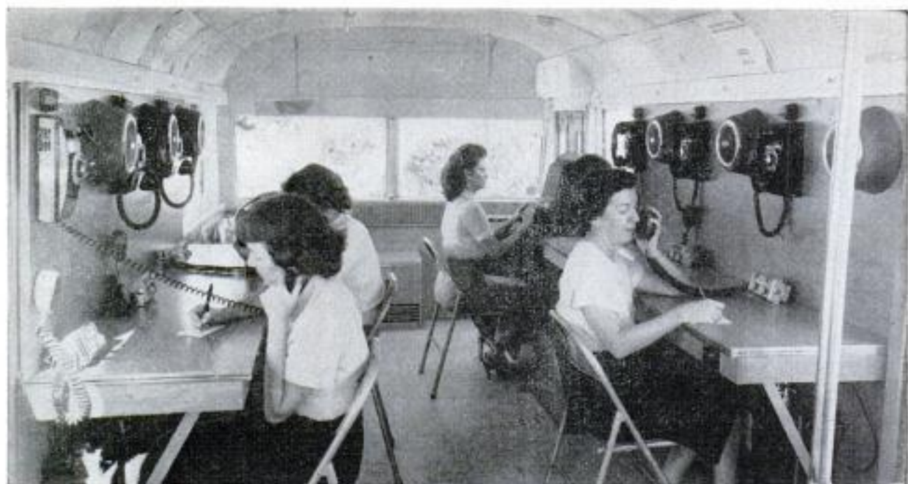
Converted city bus, which carries own generator, could be Miami communications headquarters in emergency
