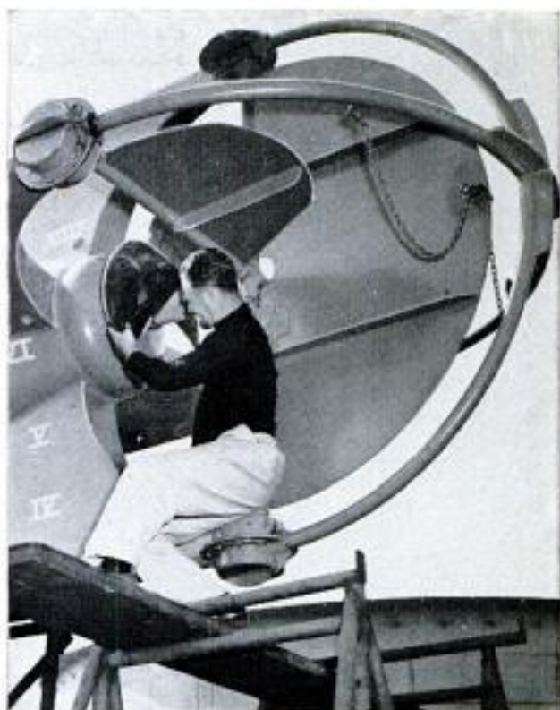
Inventor Martine checks propeller. Behind and above him are diving vanes and rudder that maneuver sub
