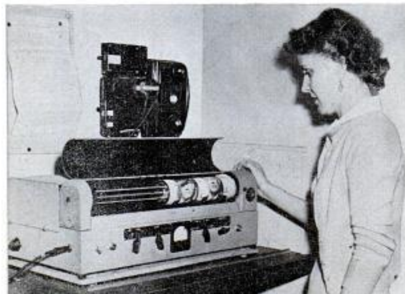
Portable radio transmitter built by Communications technicians is used at Miami-sponsored golf tournaments, parades and other special events. Speedphoto unit in Communications Center sends and receives photos, information, fingerprints of dangerous wanted criminals
