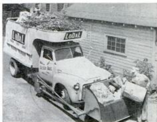
Combination of sideboard assembly and special refuse lip on bucket solves refuse-collection problems
