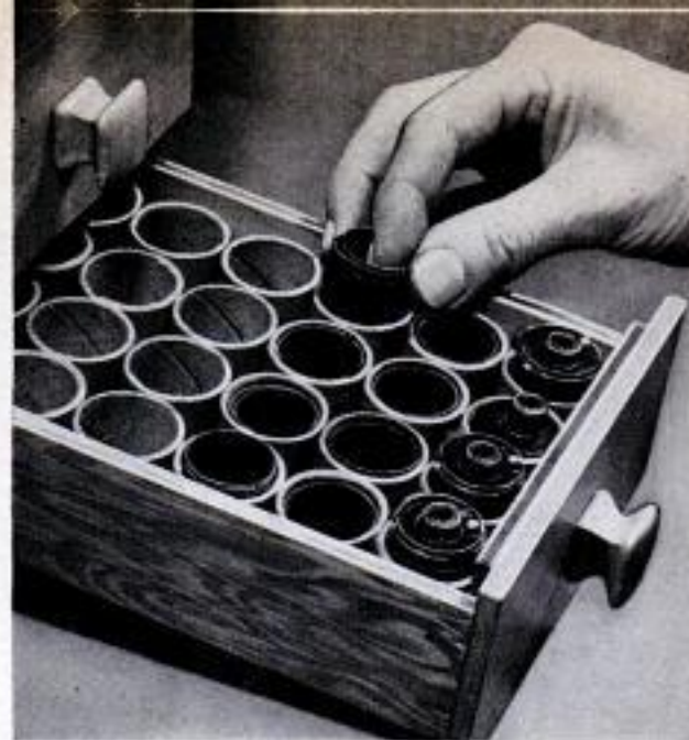
Honeycomb compartments made of tubing are ideal for storing rolls of 35-mm. film, buttons or small parts
