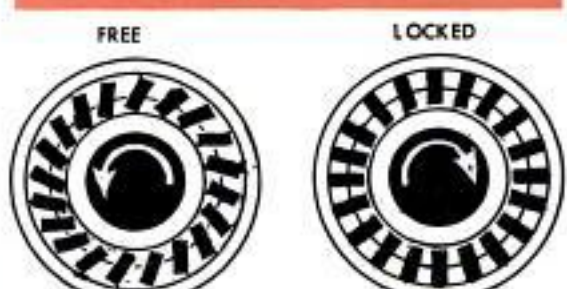
Sprag clutch turns freely one way (left) but as planetary reaction tries to go the other way, the tiny pawls jam so it cannot rotate
