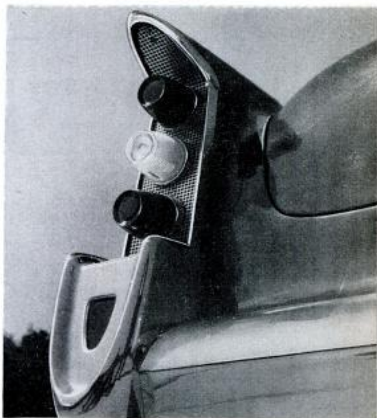
De Soto taillight assembly is three separate lights. Below, profile of two-door hardtop
