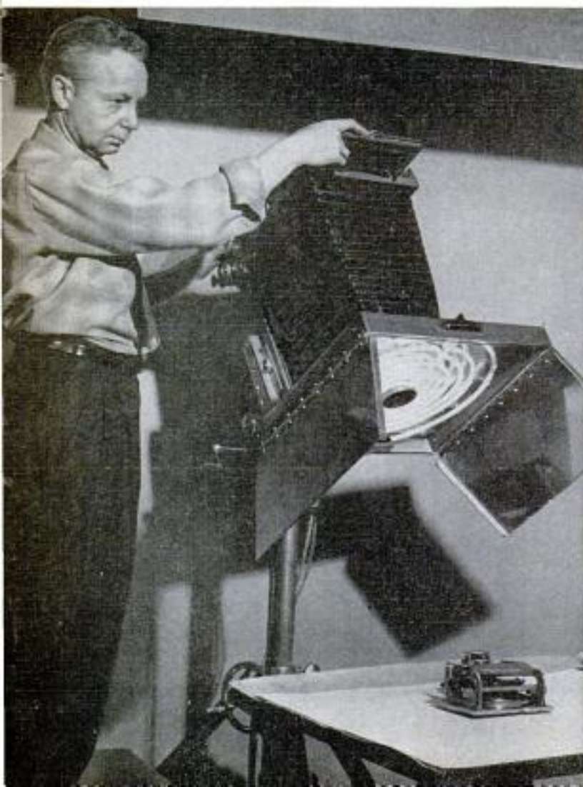
Hine puts one of his shadowless lights to work photographing a piece of machinery. Reflectors cover lamp when not in use
