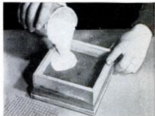
Plywood dam is set up around impression and plaster of paris is poured into mold, above. Hardware cloth, photo below, reinforces plaque
