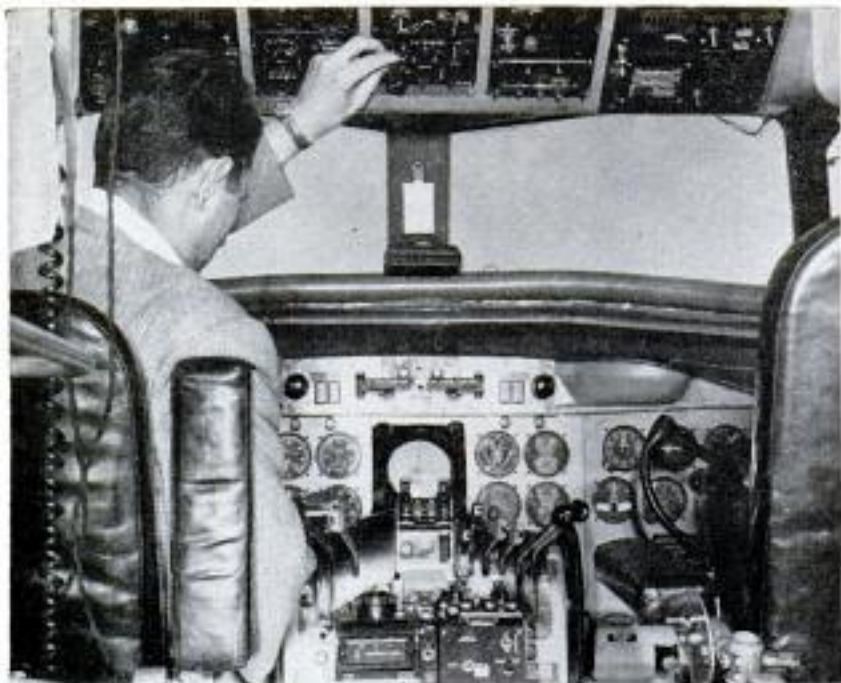
Tiny screen of weather-mapping radar is installed in center of instrument panel, while radar controls are mounted above the windshield
