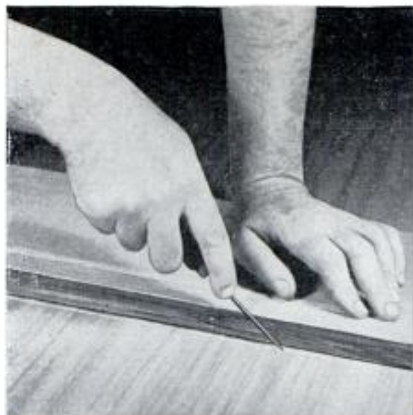
To cut laminate, score face through to core with ice pick or awl, using a straightedge as a guide
