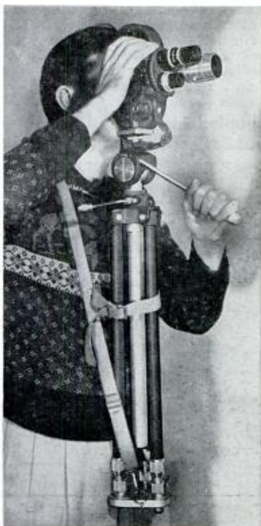
Suspended from the neck, the carrier provides stable support for the tripod when used as a unipod. The use of the tripod head for both upward and downward angles is retained by merely reversing the direction of tripod head
