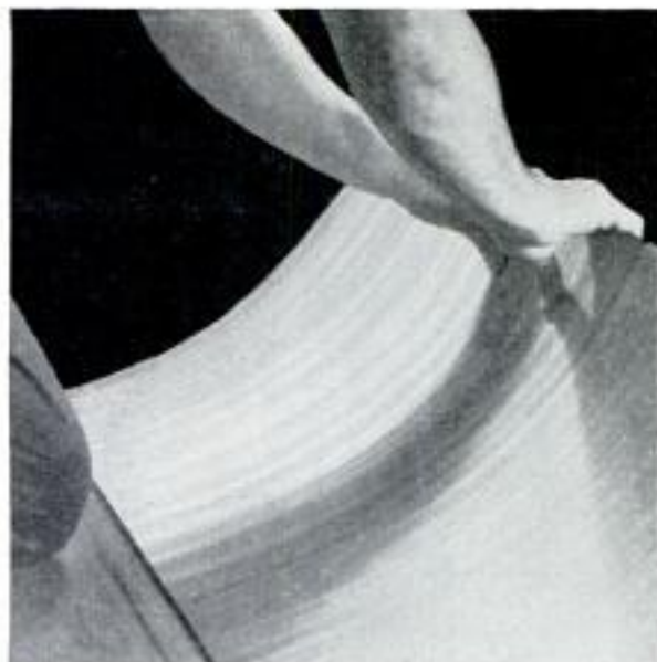
After scoring, hold the straightedge firmly against the scored line and bend the panel upward to break
