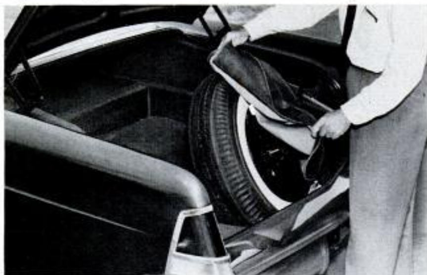
Spare-tire bulge in trunk lid is in keeping with the former Continental tradition. However, the tire location makes loading trunk very awkward
