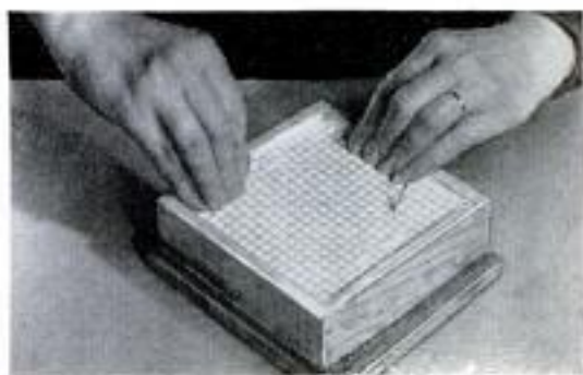
Plywood dam is set up around impression and plaster of paris is poured into mold, above. Hardware cloth, photo below, reinforces plaque
