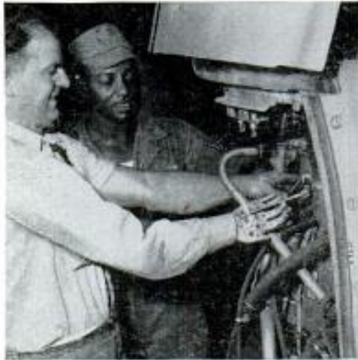
Inventor Roberts, right, looks on as Travis operates mechanical hand to tighten bolts
