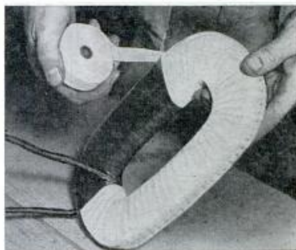
9. Finished coils are saturated with shellac or insulation varnish, then wrapped with plastic tape
