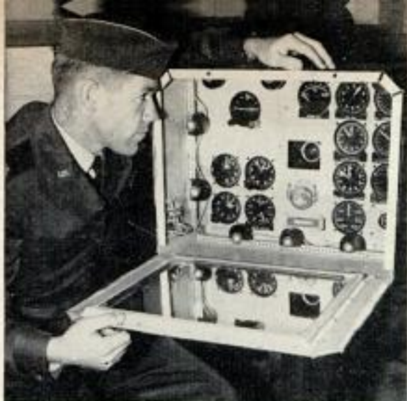
Special instrument panel is installed in plane being flight tested. Camera records instrument readings
