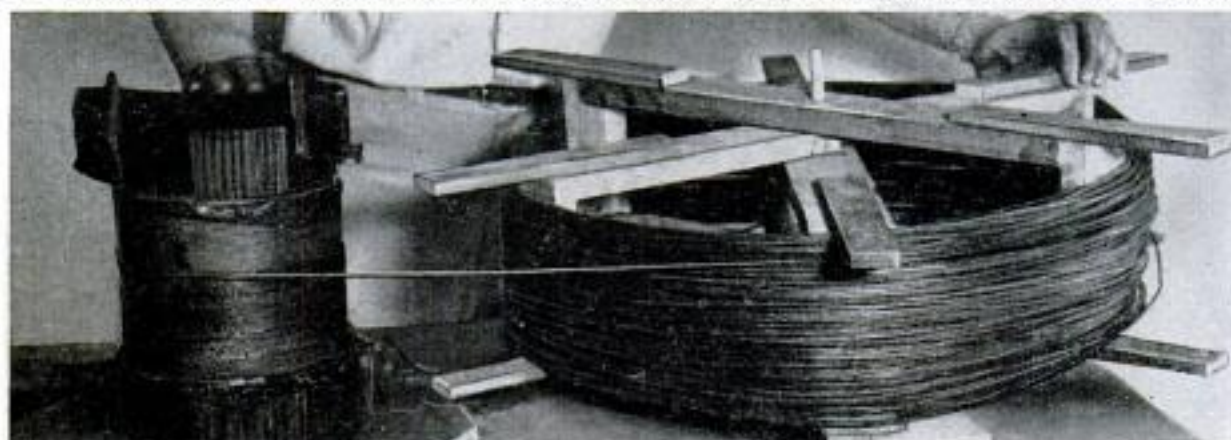
5. Unwind wire from transformer coil onto reel made from scrap wood. Turntables simplify this operation
