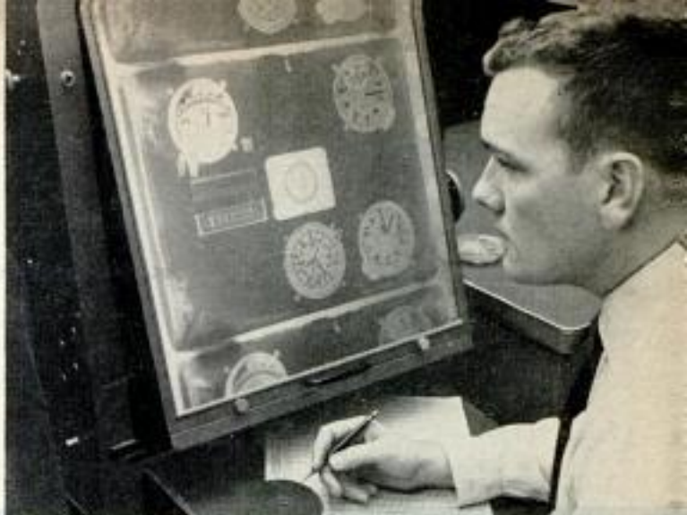
Film is projected after flight. Student pilot prepares his flight report after reading instruments
