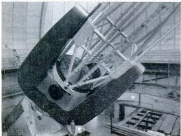
Seventy-ton fork of the instrument dwarfs man standing beside it
