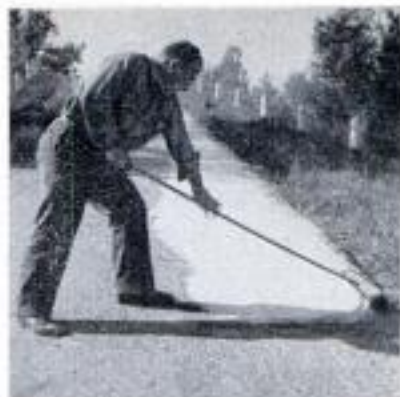
1 With temperatures in the 90s, workman "ices" a 35-percent hill by spreading liquid soap over it
