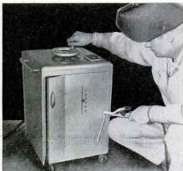
23. Decal numbers equally spaced along indicator slot permit judging relative heat at any setting
