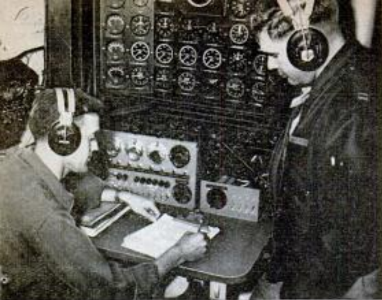
Project engineer records instrument readings during testing of C-124C Globemaster as test pilot watches
