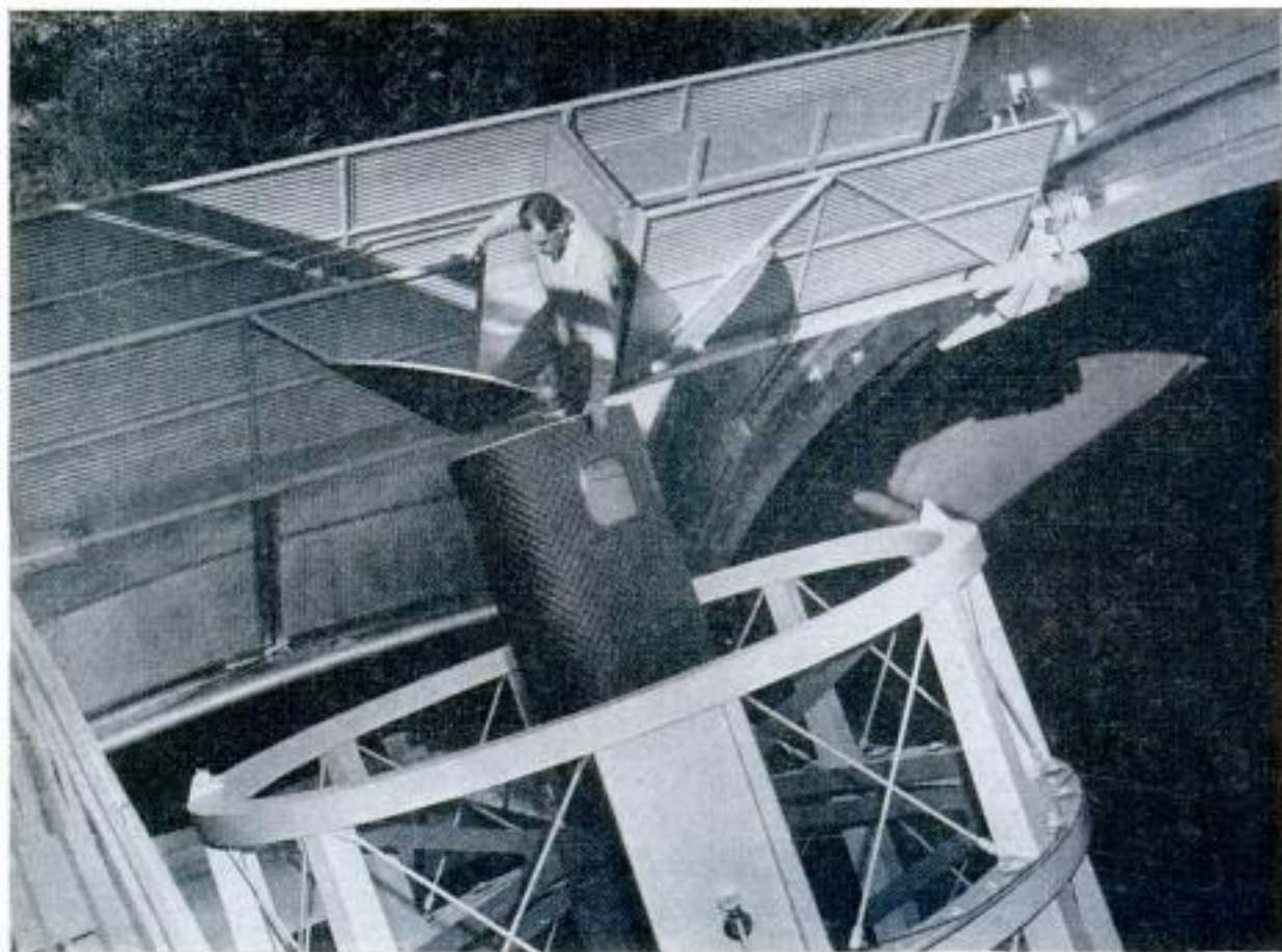
Astronomer steps from elevator into booth at upper end of telescope. Below, outside view of observatory
