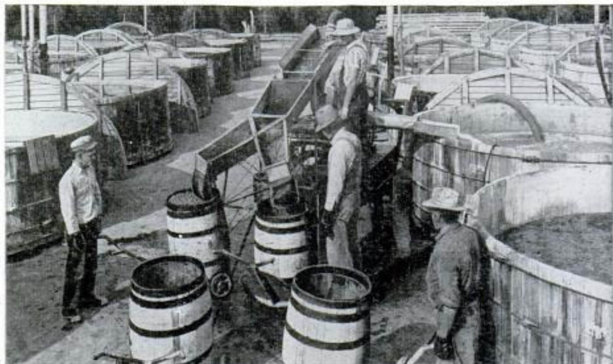
Green olives are pumped from washing vats into 50-gallon barrels and covered with a weak brine solution
