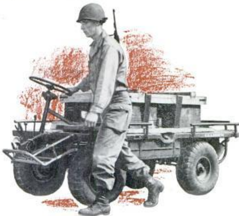
Flat-bed Jeep under test on Munson course has folding steering wheel that permits driver to walk alongside
