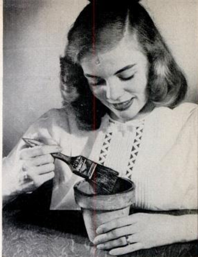
Coat of paint inside flowerpot will seal porous clay and prevent moisture from evaporating rapidly. Use rubber-base, or other paint that won't harm plants
