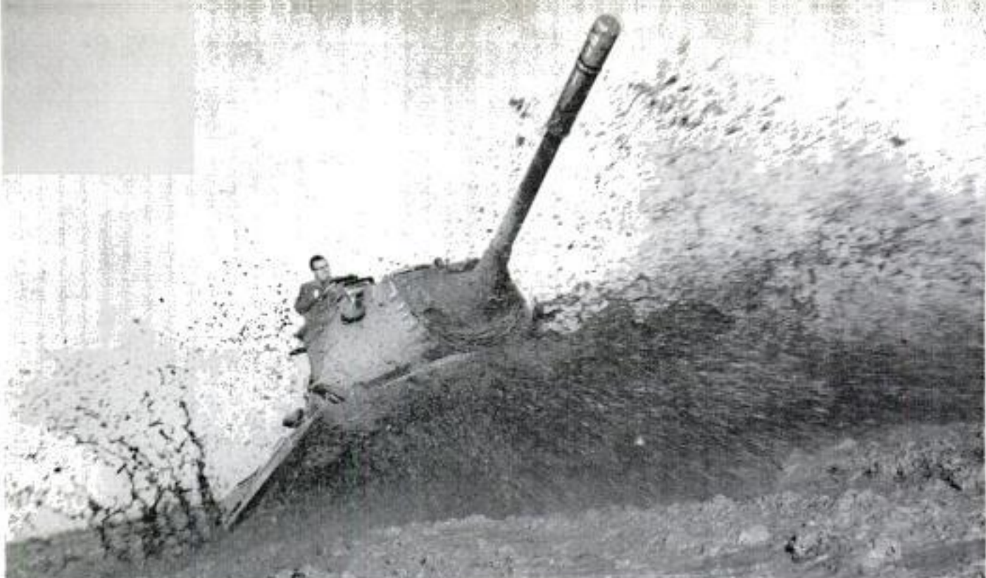
Big tanks, like this M47 hitting the mud at Perryman, become covered with as much as two tons of caked mud
