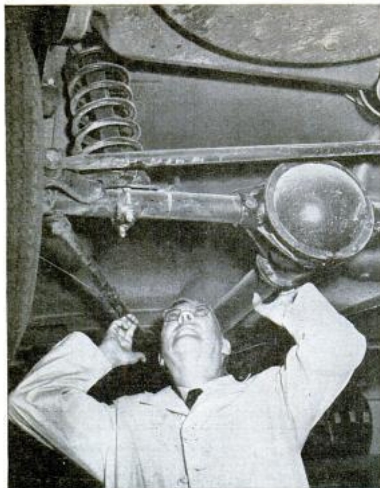
Hudson now has coil springs in the rear and a torque-tube drive. Clymer does not like this system with its greater unsprung weight
