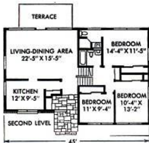
This split-level home was built in Wayne, Pa., by Madway Engineers and Constructors. It was designed by Theodore Bradow. Exterior materials are brick, Philippine mahogany, plywood and asbestos panels. Home provides large storage area
