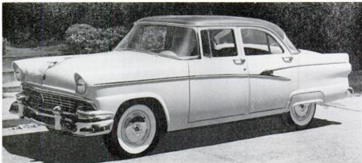
Ford Customline models feature a new chrome trim that runs the full length of the car. Grille is restyled
