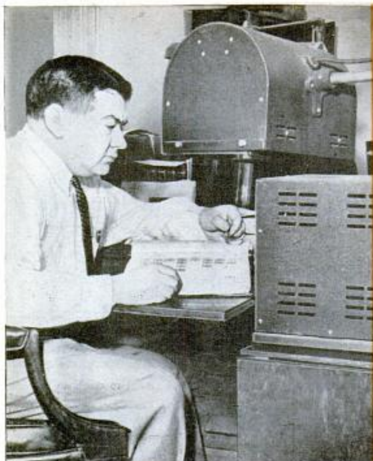
Expert uses quartz lamp to compare fluorescence of ink on a questionable stamp with ink on a genuine one. Stamp at top right was overprinted for airmail service. Below it is a fake. Note differences in type
