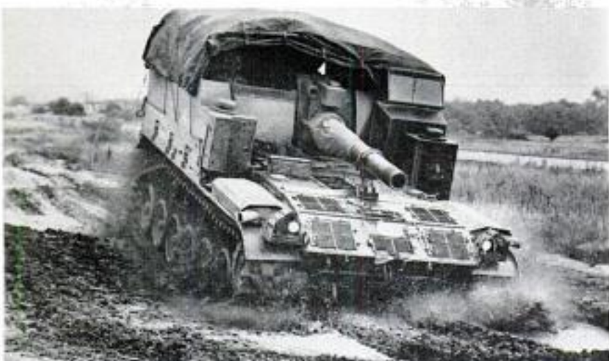
Newest mobile weapon to take the bumps and churn through the mud at Perryman is M44 155-millimeter self-propelled howitzer
