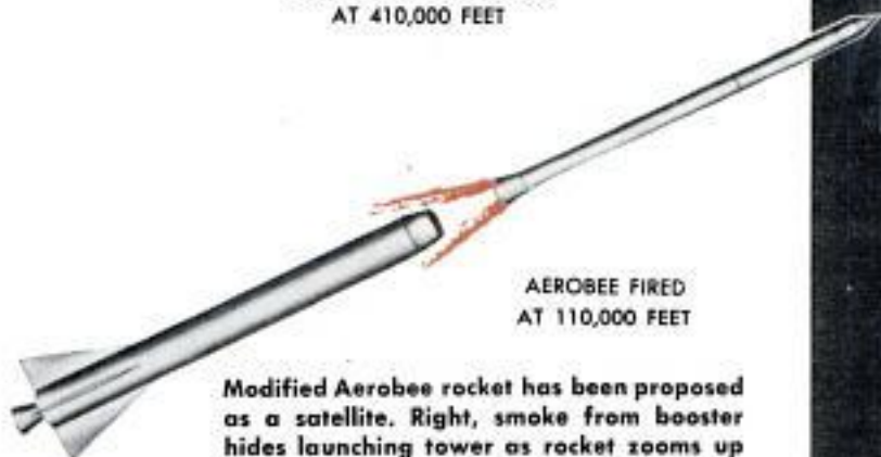
AEROBEE BURNS OUT AND BEGINS COASTING AT 410,000 FEET
