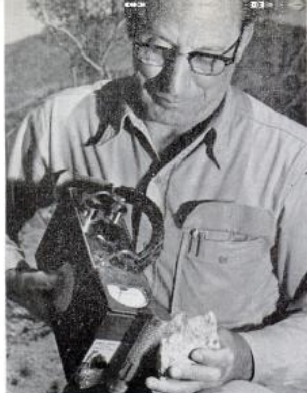
Ashby determines value of ore sample by holding it against tube of his assay counter, watching needle
