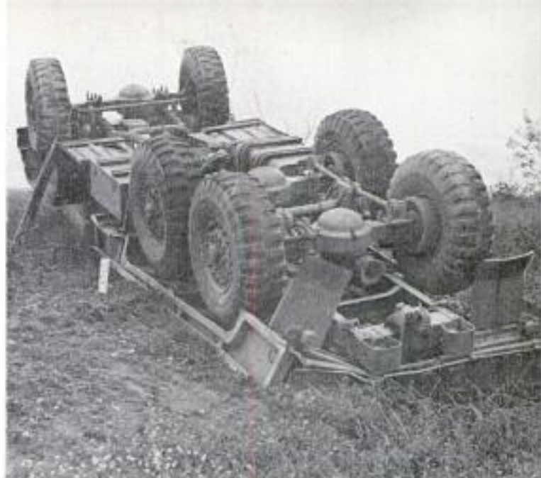
M41 cargo truck flipped over after the steering failed on a speed run at Perryman. Driver was unhurt
