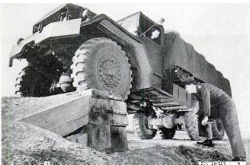
New supply carrier must be able to climb over the 30-inch vertical barrier at Munson. Test also proves clearance of truck
