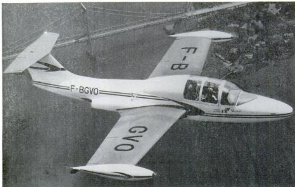
Morane Saulnier 760, French twin-jet executive transport, cruises above East River on demonstration flight
