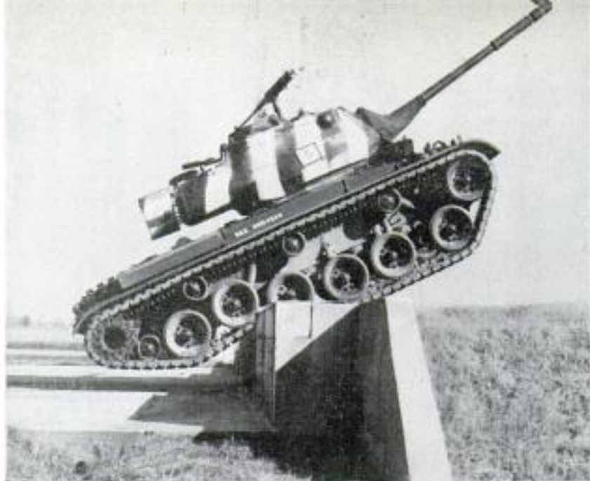
Before a new tank such as this M47 can qualify for service, it must be able to leap three-foot vertical wall at Munson without coming apart
