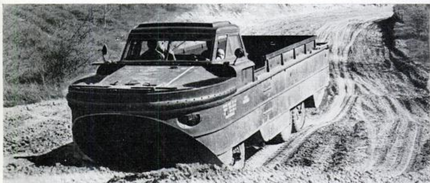
Amphibious Super Duck, like fish out of water, bucks a mud wash on four-mile torture course at Churchville
