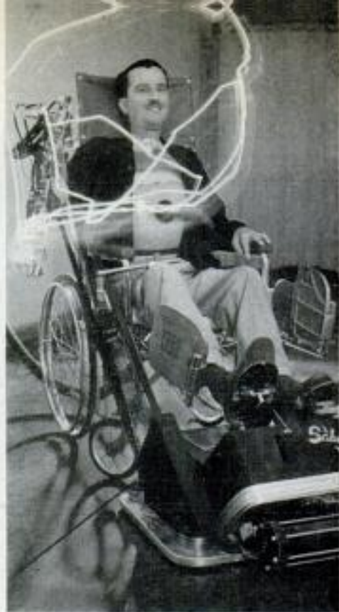
Path of light bulb in photograph traces the extent of the hydraulic arm's reach
