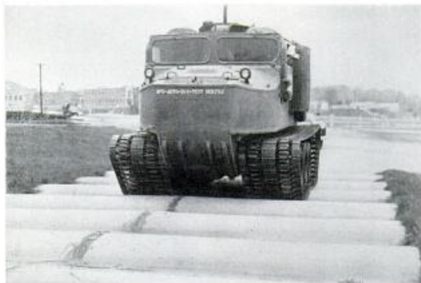
Amphibious Otter must withstand 10 or 20 miles of these concrete bumps before taking other tests. Below, rotary plow keeps roads unpleasant
