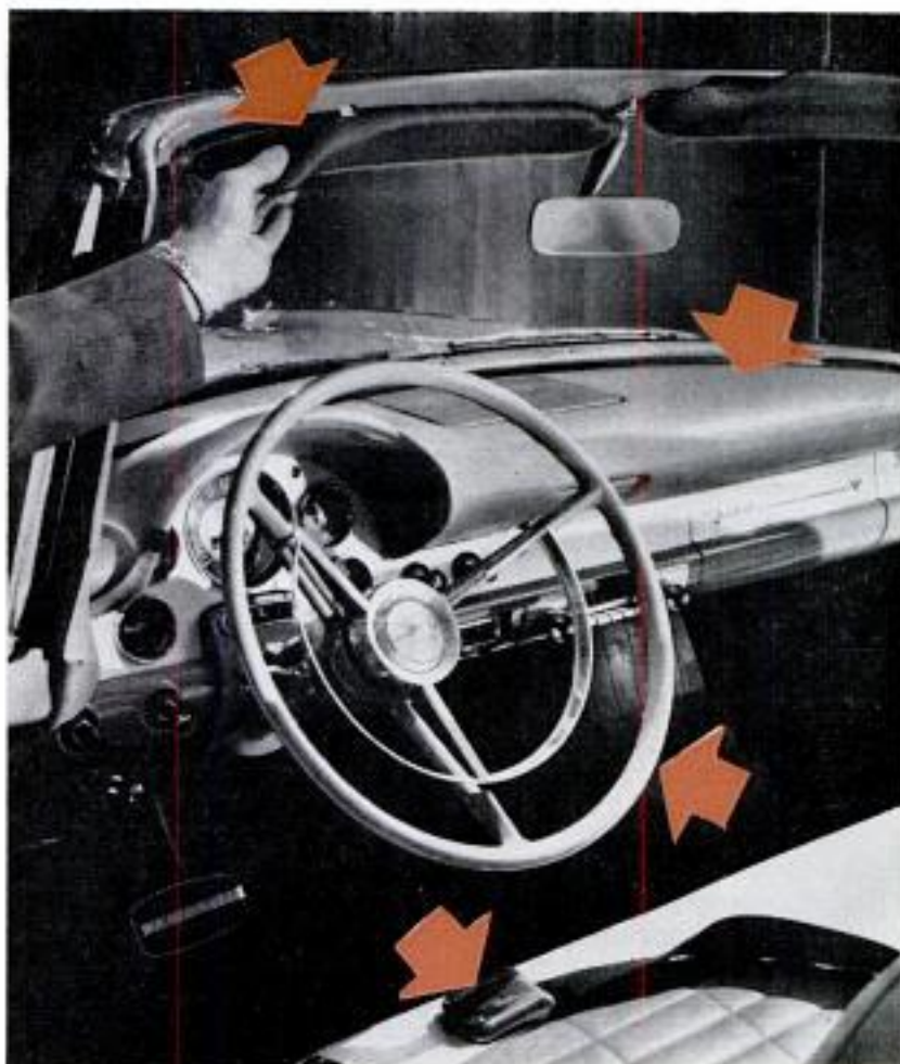
Ford's safety equipment (arrows) includes padded sun visors, padded dash, concave steering wheel and seat belts. Rear-view mirror is shatterproof
