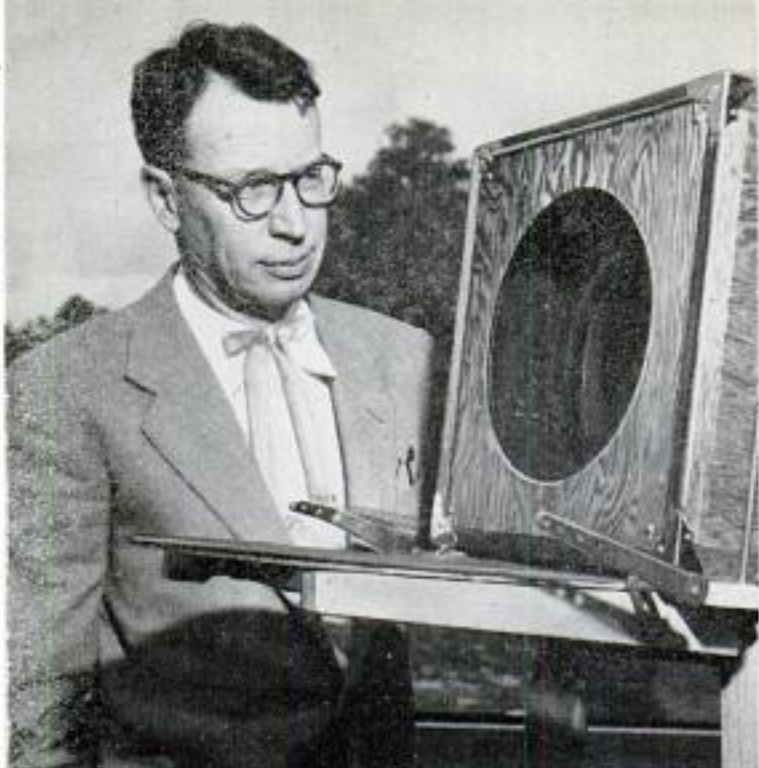
Plain wooden box houses Schmidt telescope so powerful it could spot a tennis ball 1000 miles away
