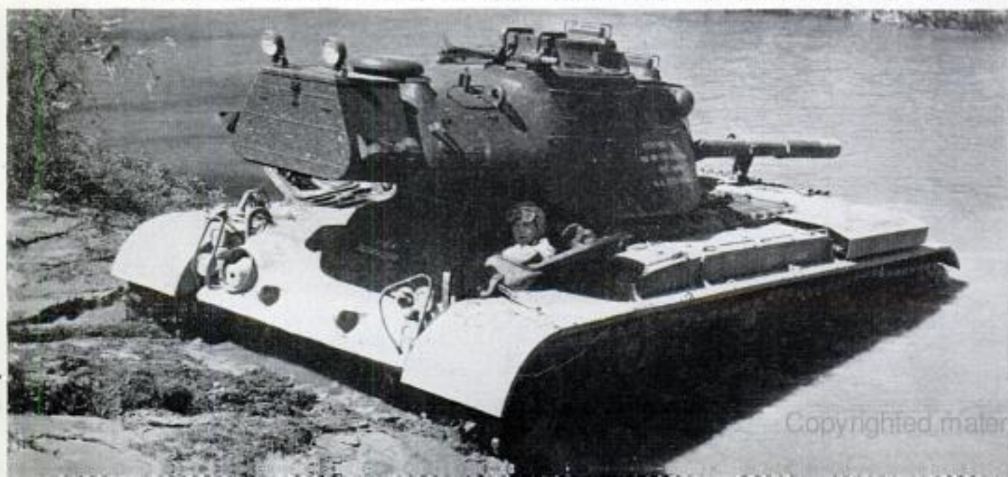
Churchville's rutted route takes vehicles right through a stream to test fording ability. This is an M47 tank
