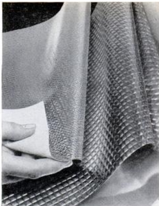
Transparent Mylar has one third the tensile strength of steel. Right, film can be metallized with aluminum
