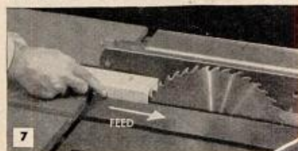
TEST CUTS SHOW FENCE OUT OF ADJUSTMENT
