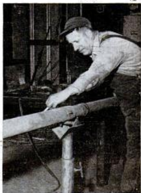
Machine cleans dirt and rust from old pipe before it is bolted together, telescope fashion, into TV masts
