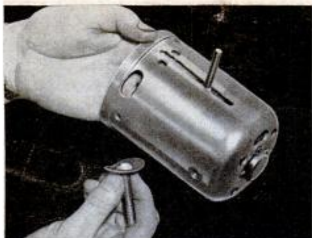
Motor housing is slotted to take two \frac{1}{4} -in. bolts which permit vertical adjustment on mounting block
