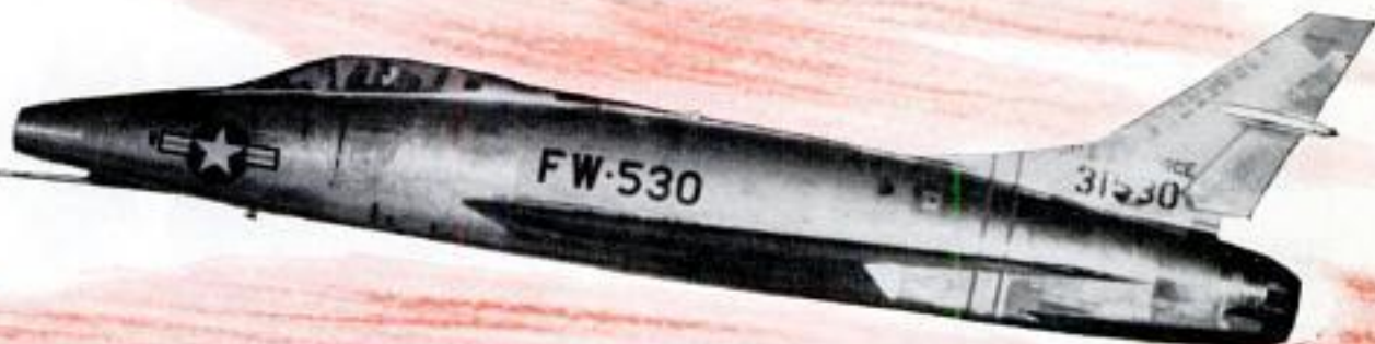
Two views of North American F-100, Super Sabre, one of latest and fastest jets in military service. A supersonic fighter, it is made of heat-resistant metals and equipped with automatic cockpit air conditioning
