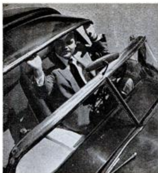
Stylist Flajole demonstrates the sliding roof. Right, with the roof retracted, the car is an open sportster
