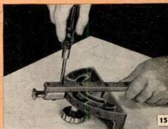
Miter gauge should permit an accurate 90-deg. cut. Cuts made halfway through test stock indicate error as above. Parallel cuts show that gauge is properly set. Miter gauge is reset by backing off screws holding index pin, right
