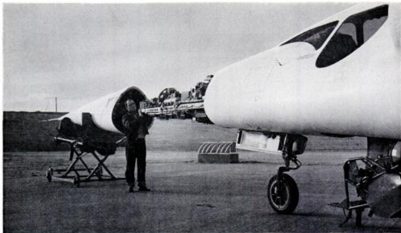
Test instruments are carried in the needlelike nose of the X-3, jet designed for "heat barrier" experiments
