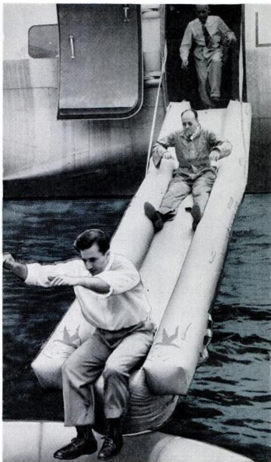
Garrett Corporation photo Passengers demonstrate escape from plane via pneumatic slide, originally designed to evacuate people from high doorways of planes on land. After evacuation it can be detached from plane and used as a life raft.
