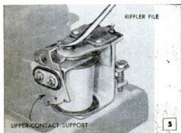
Above and below, always use a riffer file to clean the contact points of current and voltage-regulator units. Never use sandpaper or other type of abrasive
