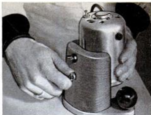
Mounting block is of hardwood shaped to fit curve of motor housing. Block is bolted to the base plate
