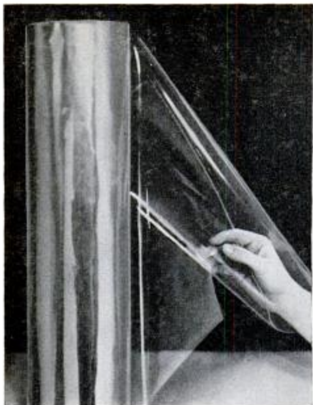
Transparent Mylar has one third the tensile strength of steel. Right, film can be metallized with aluminum
