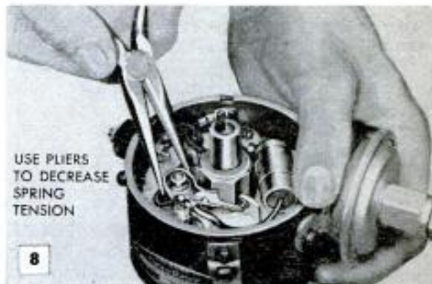
Usually the spring tension can be altered slightly simply by bending the spring with long-nose pliers. Correct tension is important in high-speed operation
