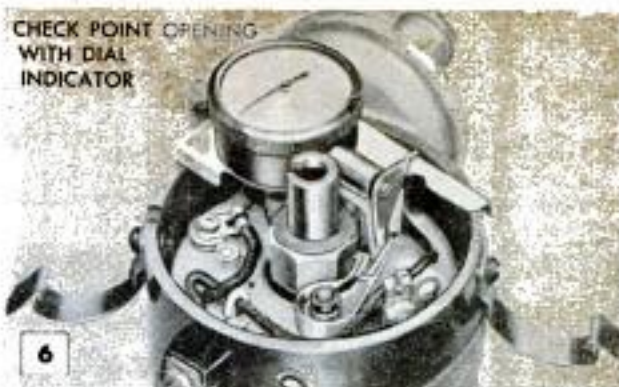
There are various methods of checking distributor-point opening, but a dial indicator is most accurate
