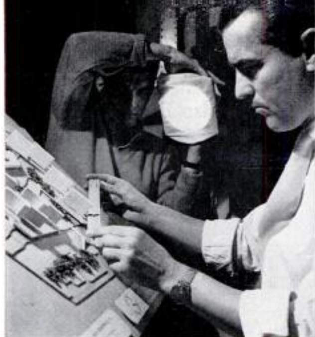
Powerful spotlight simulates the sun. Architects move board to determine sunlight, winter and summer
