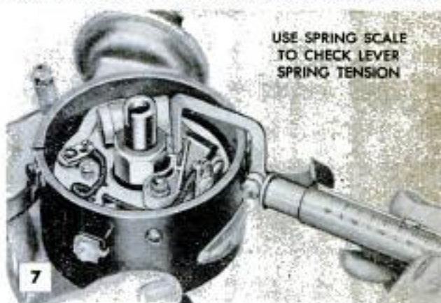
Whenever a new breaker arm, or lever, is installed always check the spring tension with spring scale
