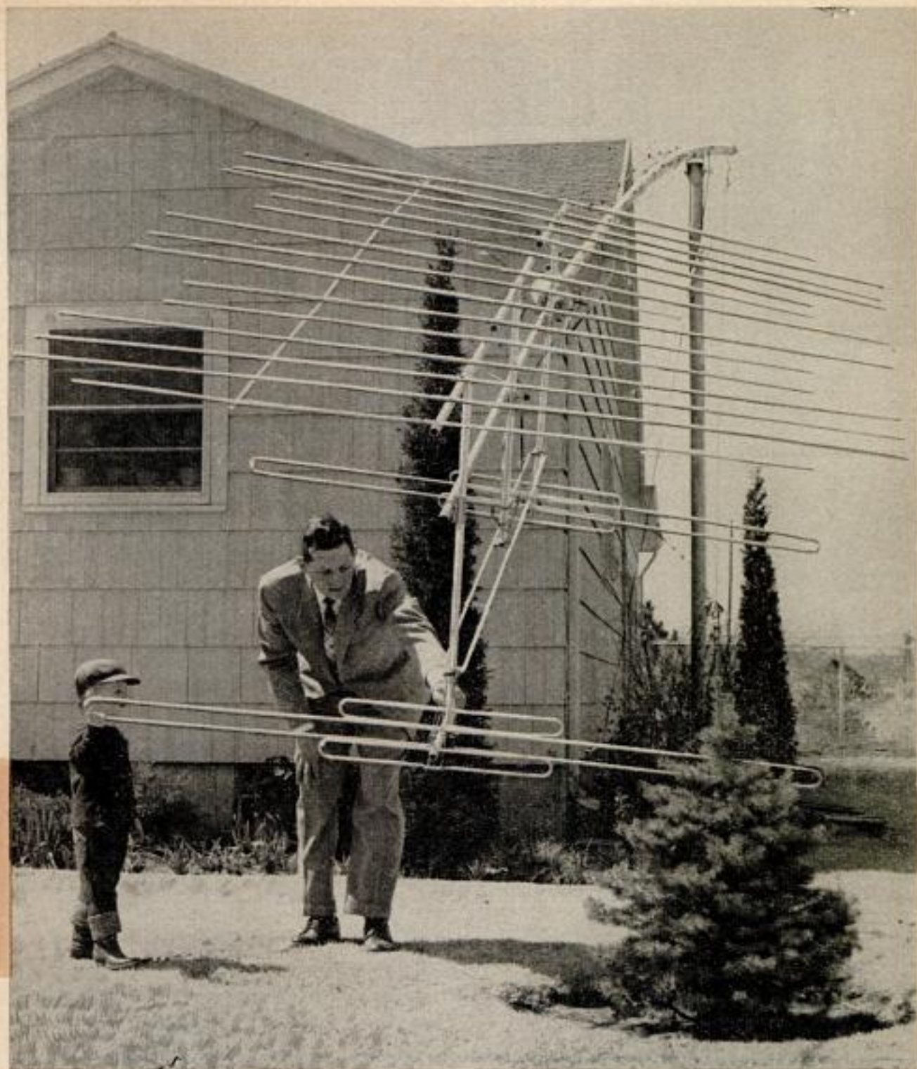
Antenna adjustments are easy when mast is tipped over. Motor on top of pole turns the antenna for tuning
