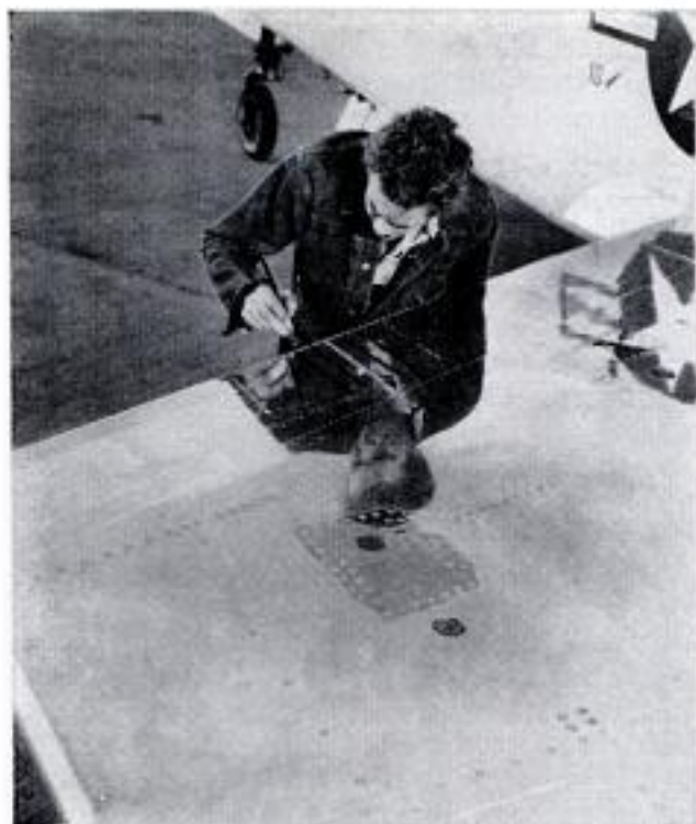
Speed stripes painted on wing, above left, change color as heat rises to warn pilot of temperature changes on wing surface. Right, pilot is raised into cockpit by small motors. In emergency, pilot in seat is ejected downward and fins visible on side of seat unfold to act as air brakes to slow descent
