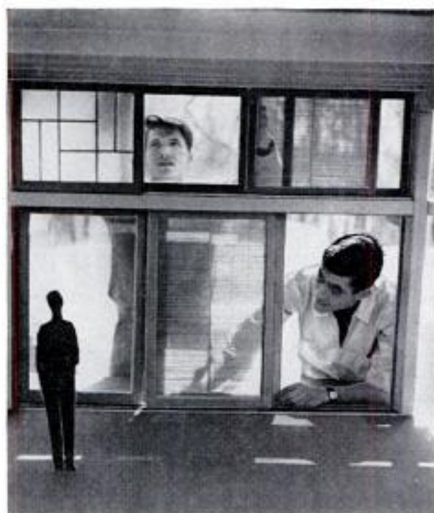
Panels of shading material close off a model room. Cardboard man shows how sun would strike human in the full-size room. Below, plastic bubble in roof offers plenty of sunlight for checking a house model
