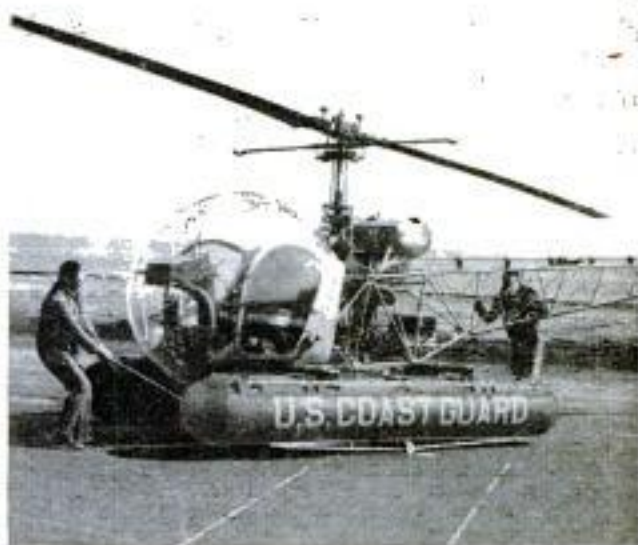
Copter on platform can be towed by hand. Below, the unit weighs only 66 pounds. Framework is of molybdenum-steel tubing
