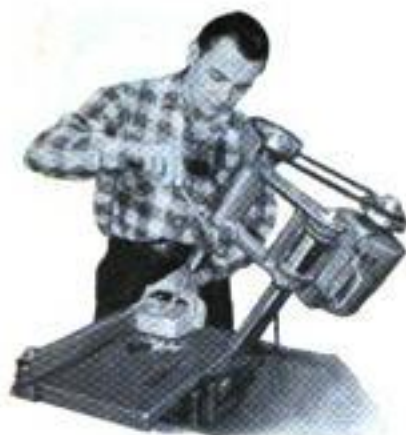
Above, drilling at an angle without blocking the work is an exclusive feature. Below, "chop sawing" short stock is fast and safe
