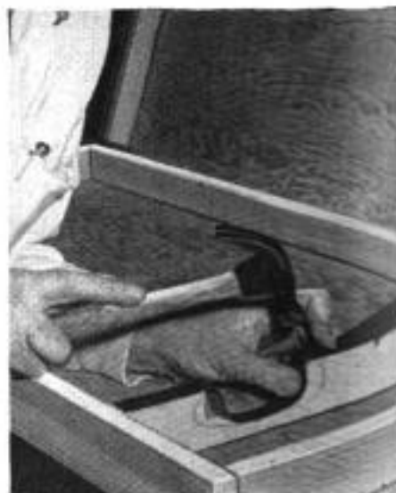
Lower right, the crosspieces are lined with strips of rubber held in place with broad-headed tacks
