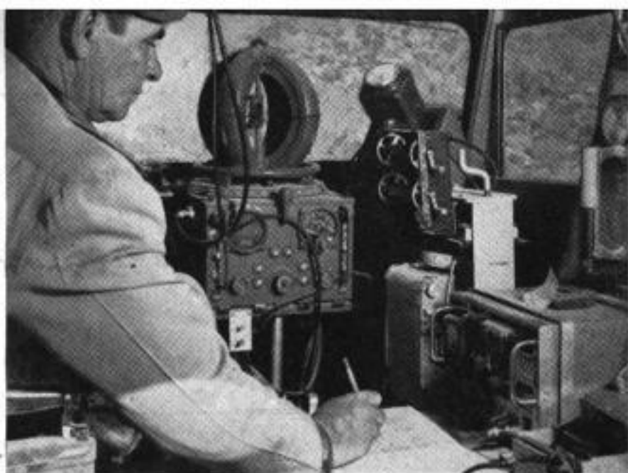
Jeep's interior is packed with instruments. Beside the driver is a moving graph that continuously records the radioactivity. ↓ Campbell subjects a rock sample to a check with a fluoroscope. Jeep also carries a microscope and chemical assay kit
