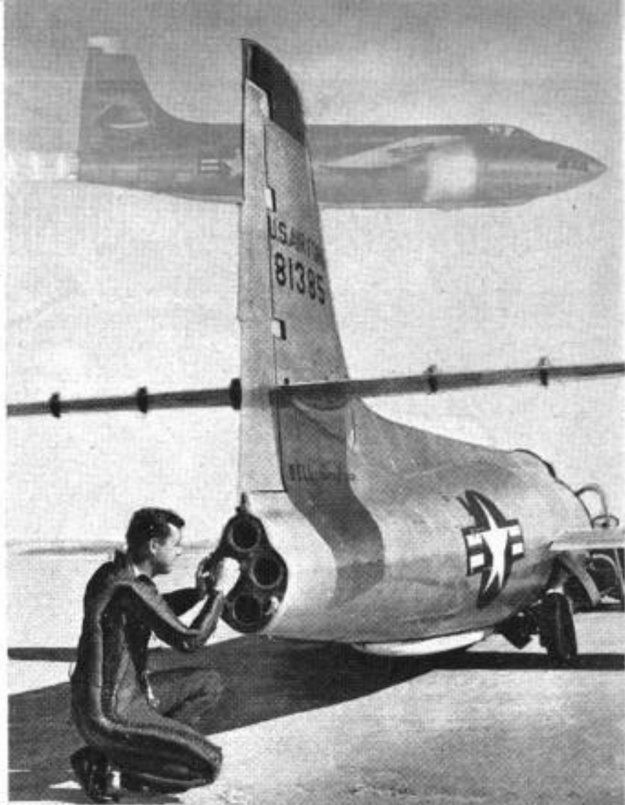
Major Murray examines the exhaust nozzles of the four rocket motors after a flight. The four motors can be fired one at a time or simultaneously
