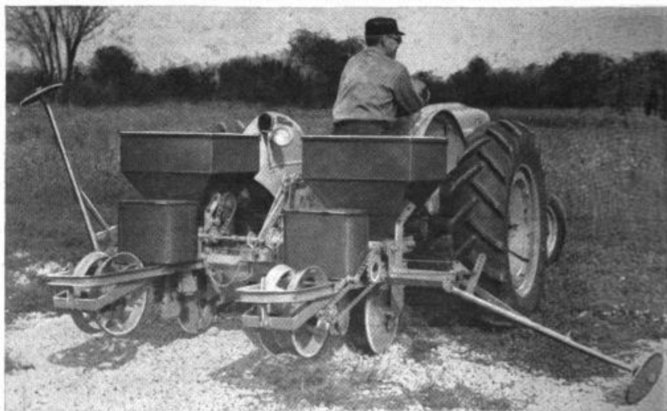
Four-inch saber and eight-inch saber on opposite sides of rolling colter lay fertilizers at different depths
