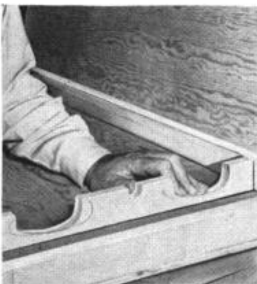
Lower left, cutouts are made on a jigsaw. Center, attaching screws must not be driven through cutout
