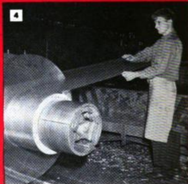
across waist. 3. Scratching his cheek is operator's way of saying "Adjust scratch brushes." 4. Cupped hand means "Adjust to align rolled edge of sheet"
