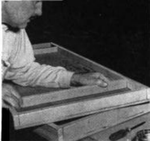
After box is assembled, top and bottom are separated by making a saw cut all around, shown above left
