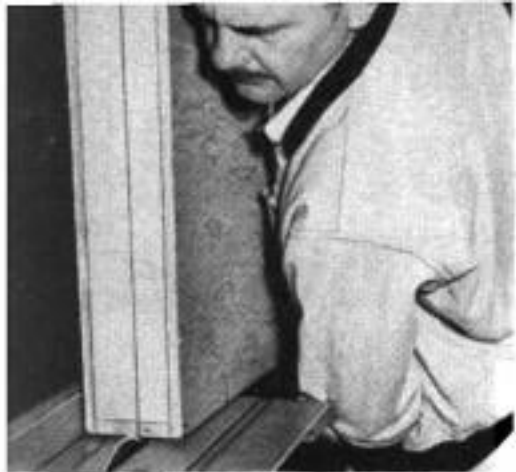
After box is assembled, top and bottom are separated by making a saw cut all around, shown above left
