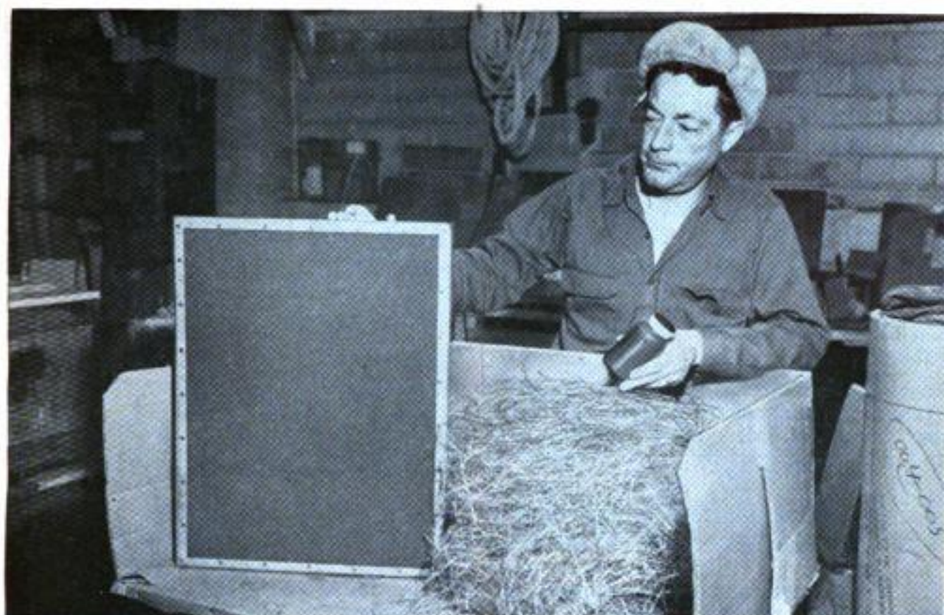
Norbert Ruff holds a catalyst element. It is made of resistance wire coated with platinum and palladium derivatives in bottle
