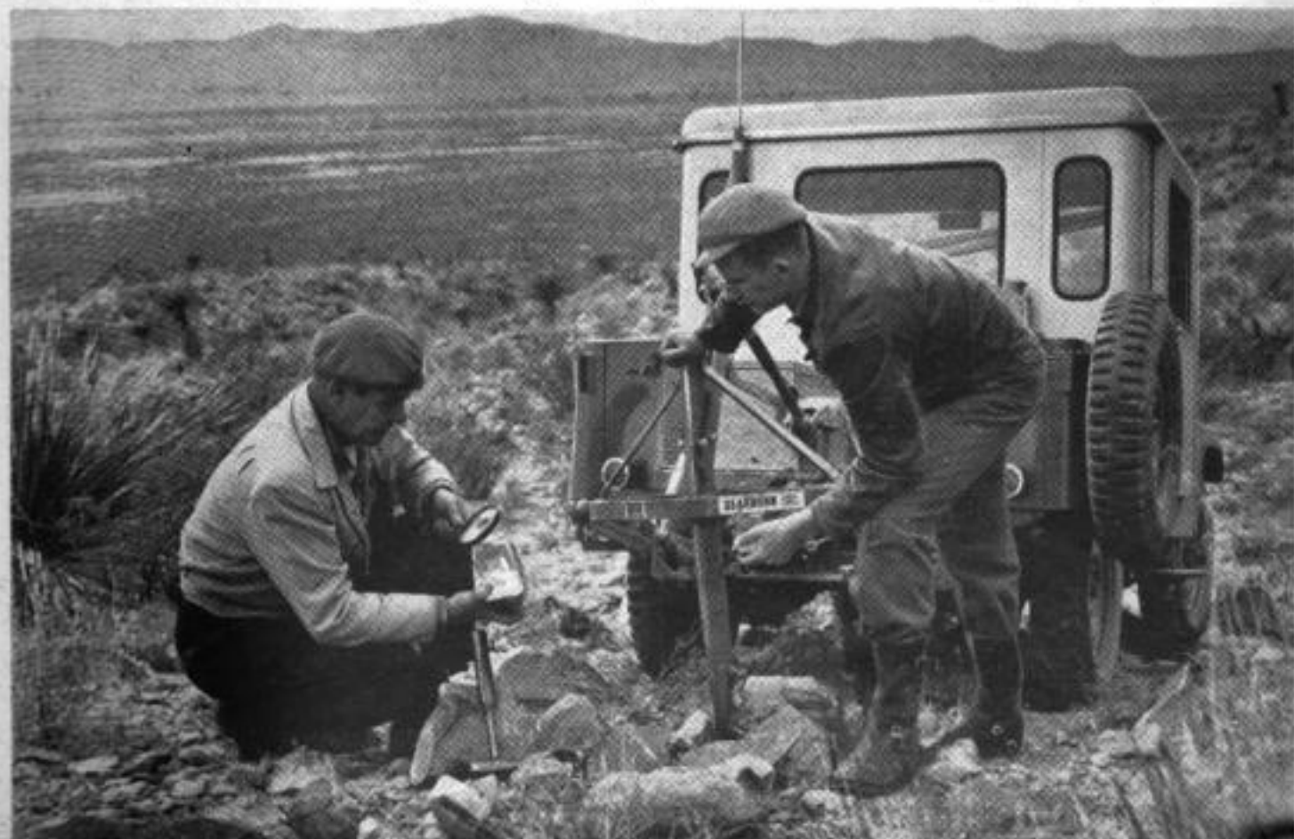
Plow on second Jeep is used to turn up rock samples. Prospectors use diamond drill to bring up deeper samples
