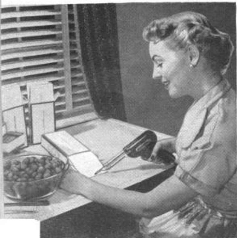
Here's a gun in use with a pad tip. Works perfectly for sealing plastic containers of the type pictured
