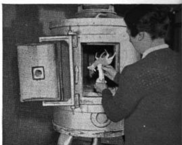
Color is applied and deer is placed in gas kiln for firing. Upside-down position helps prevent antlers from warping. This firing takes seven to nine hours
