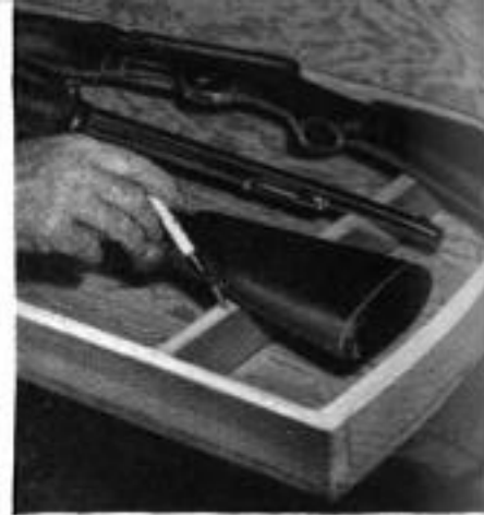
Above center, the 1 x 4 crosspieces are fitted in place. Next, at the right, gun positions are marked
