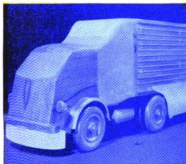
Partial streamlining (mostly closing the gap between tractor and trailer) would save $700
