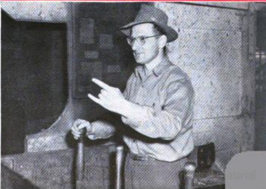
Hand signals used by sawyers in Pacific Northwest indicate inches of cut to be made. Below, George Crouch, head sawyer in Weyerhaeuser sawmill, tells setter he wants 6½-inch cut
