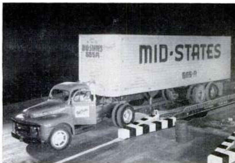
Trailer is backed right up terminal ramp and onto the flatcar, then down length of train to its own berth on one of the special cars
