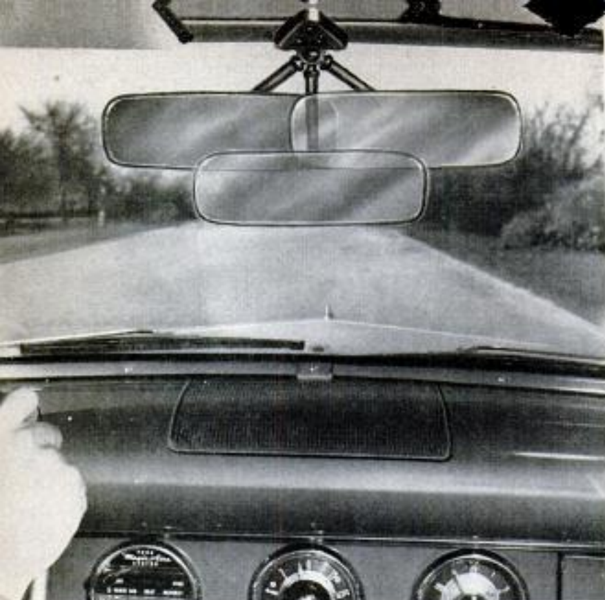
Retouched photograph, above, demonstrates how Ford's rear-view mirror has a double-swivel action to adjust to fit any driver
