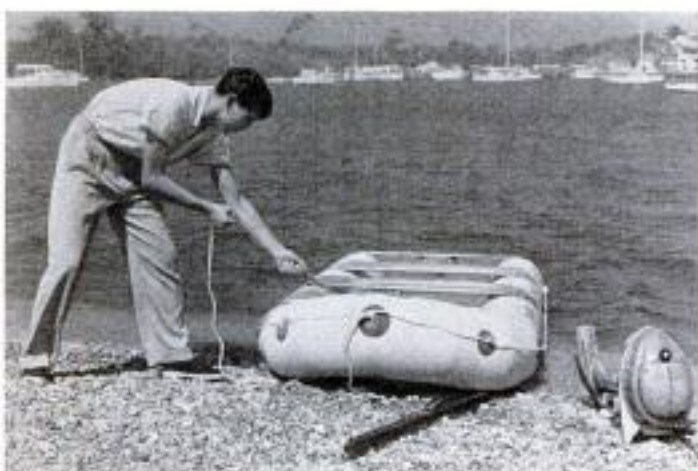
Pulling a lanyard attached to the carbon-dioxide cartridge causes the boat to inflate within seconds
