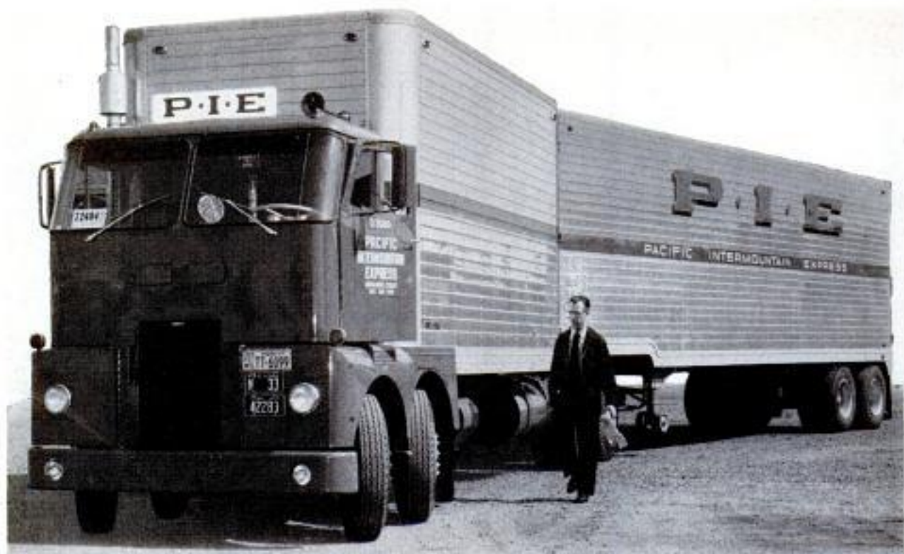
All four front wheels steer. The tractor not only pulls a load, it carries a 10,000-pound load on its back
