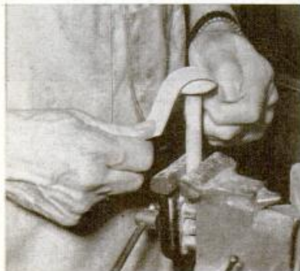
Third, Gray clamps the handle in a vise and works the blank into the desired form with abrasive cloth
