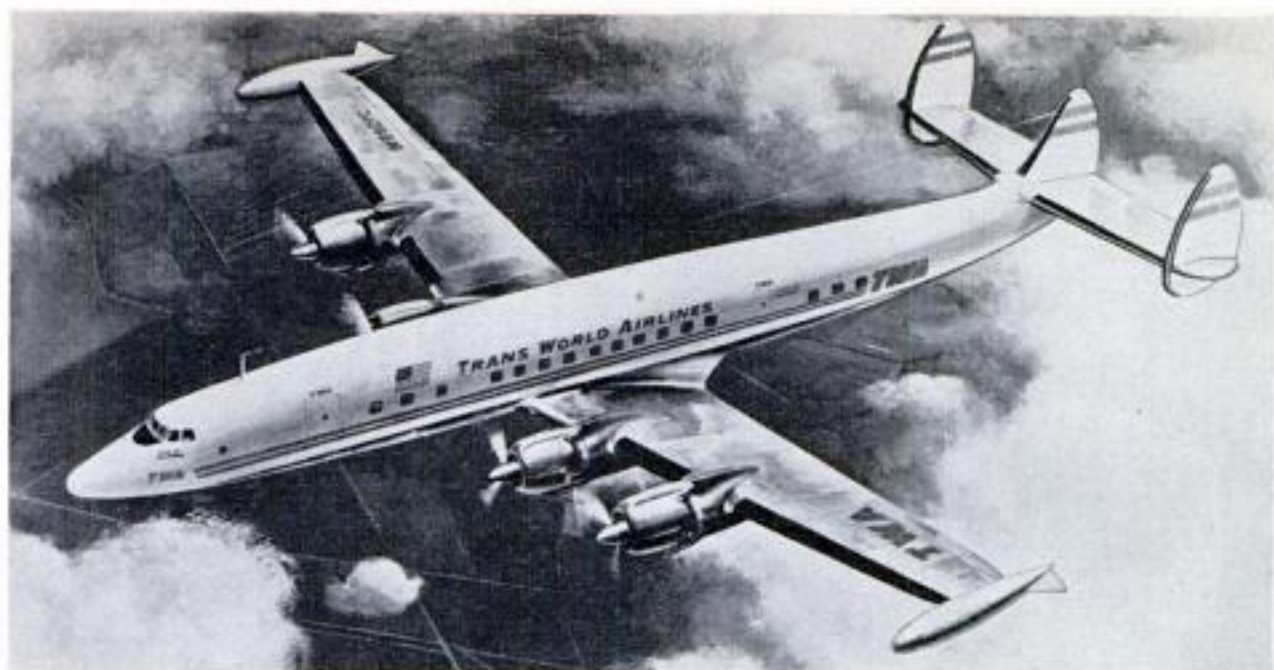
Permanent wing-tip fuel tanks mounted on some of the new Constellations will add two hours of flying time
