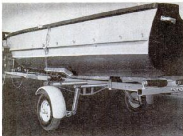
Boat is tied down on the trailer as in photo above. Note that the transom-support rollers should be raised for this particular hull
