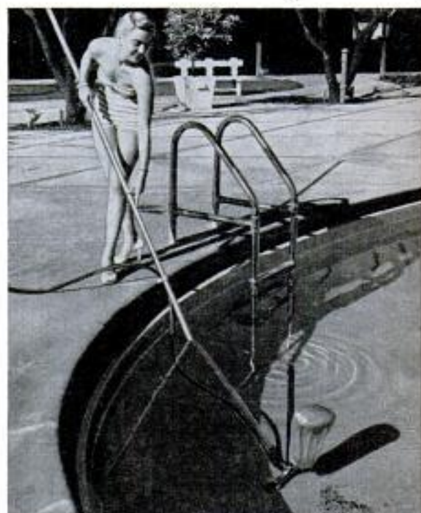
Water pressure of garden hose operates vacuum cleaner for pool. Suction behind nozzle draws refuse
