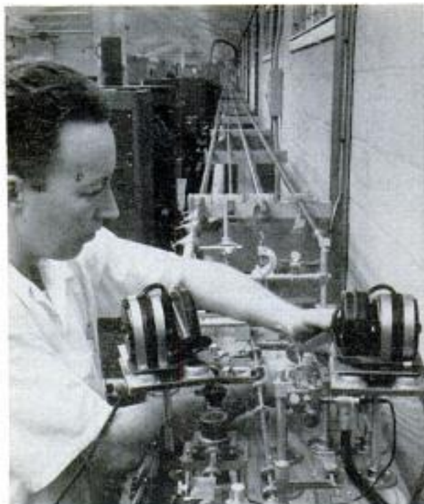
Bell scientist checks test equipment used to bounce microwaves back and forth for 40 miles in metal tubes
