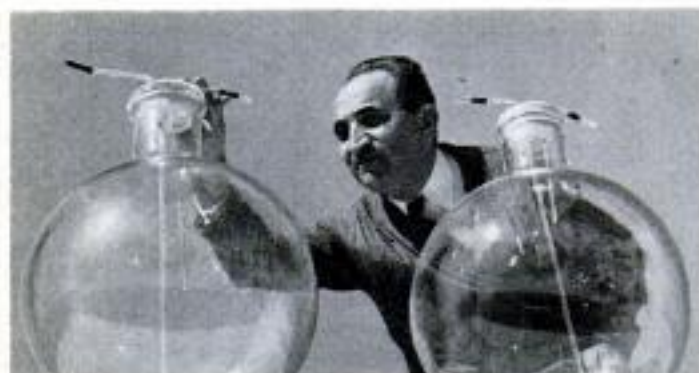
Exhaust is pumped directly from car into greenhouse to determine effect of automotive smog on growing plants
