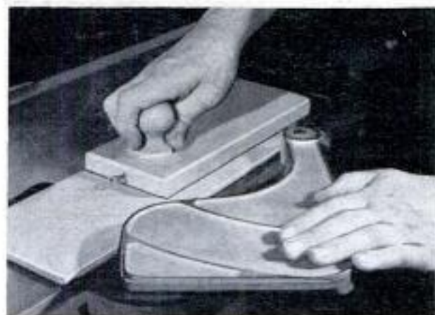
Make a hold-down pusher block and use it whenever you plane thin stock on jointer. It will save your hand
