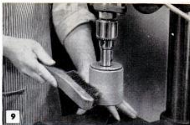
9 Wire-brushing the abrasive sleeve occasionally will prolong its useful life and produce smoother work
