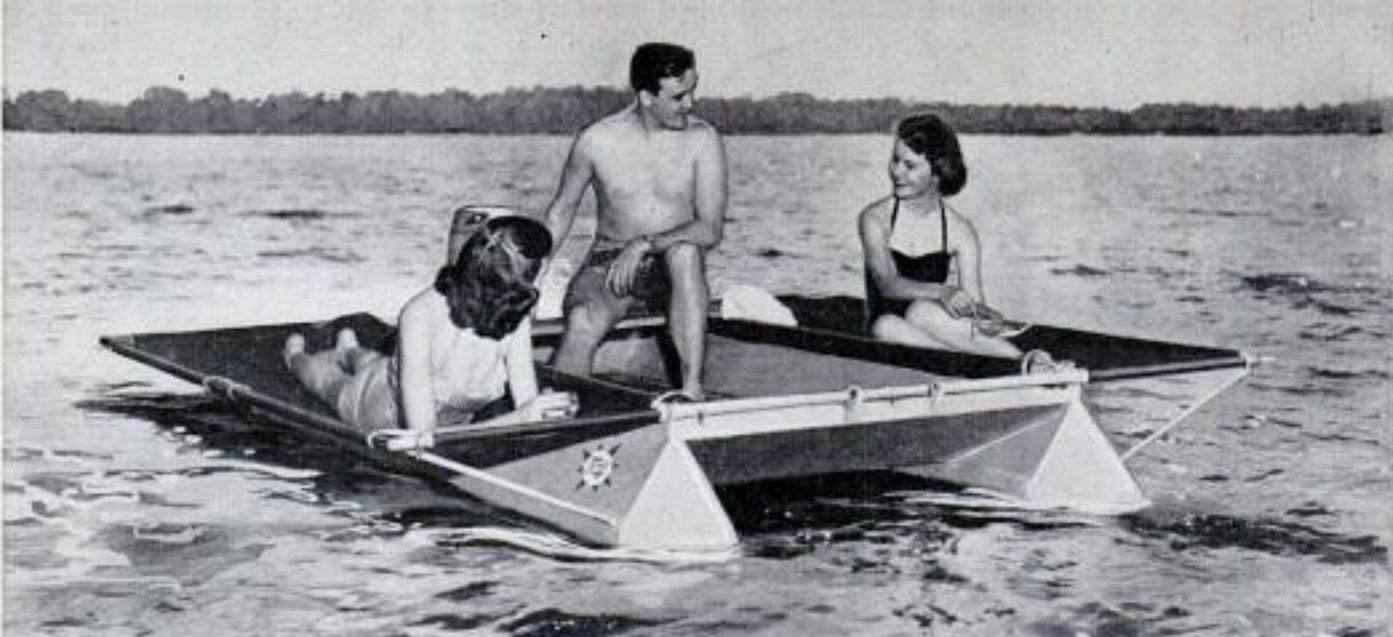
When the unit is used as a swimming and diving raft, cots unfold to provide a comfortable canvas sun deck
