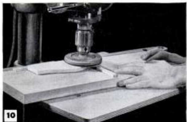
8 Coating the soft-rubber drum with commercial talcum powder will prevent sticking of the abrasive sleeve
