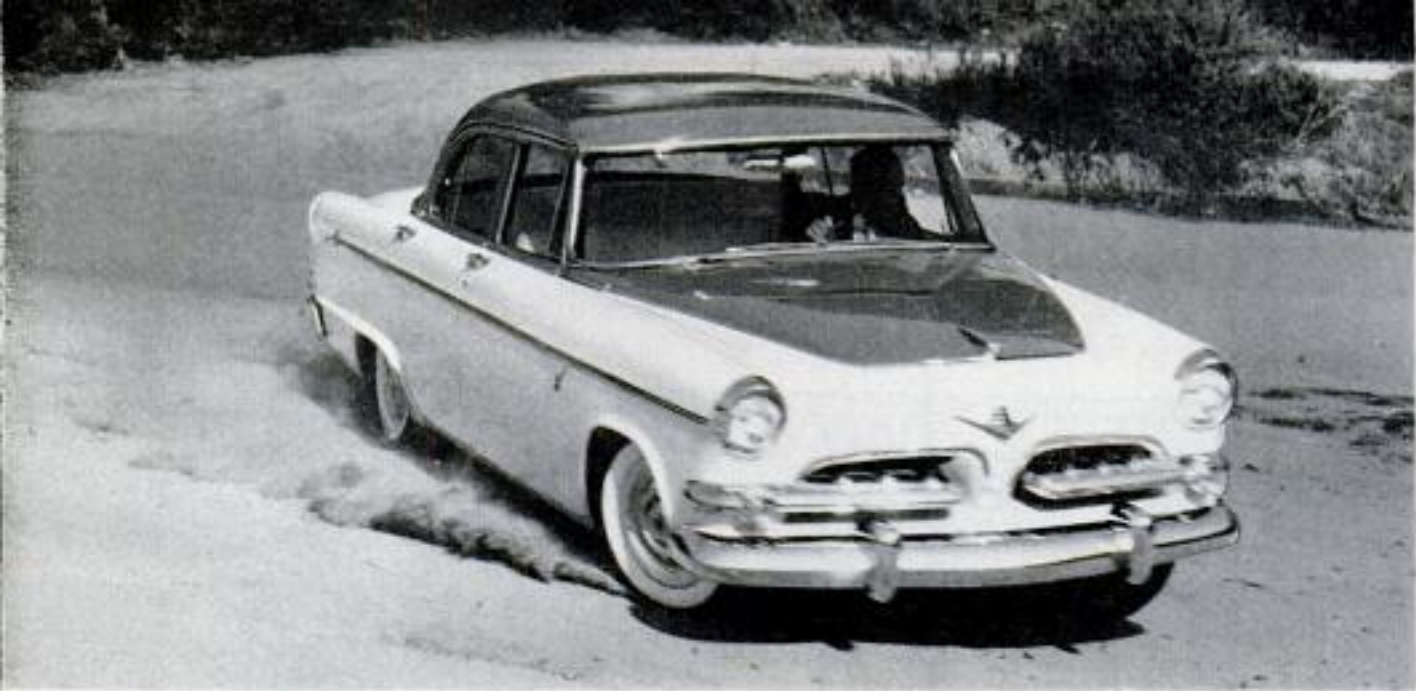
Dodge's unusual two-toning lets you put a dark color on top of the hood of a light-colored car to reduce glare
