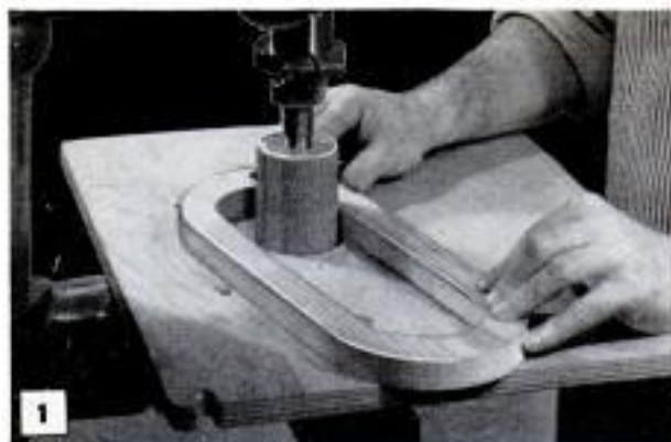
1 For best results, drum-sanding should be done with an auxiliary table bolted to the drill-press table
