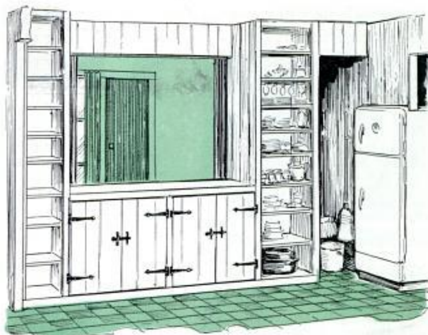
Open-face modular closets in kitchen frame pass-through opening. Cabinet doors are cleated redwood panels hung with wrought-iron strap hinges
