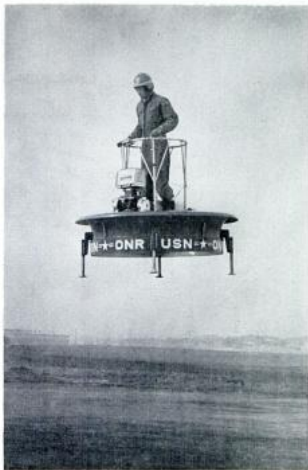
The platform goes straight up, down or sidewise. Pilot changes direction just by shifting his weight. Below, safety tether used in test flight saves pilot and craft from sudden letdown if trouble develops
