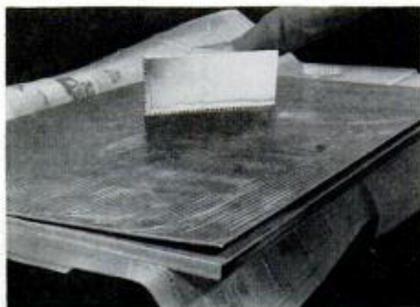
Below, the right amount of mastic is applied to the laminate and plywood with a notched applicator
