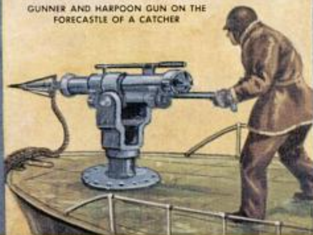
A Dutch "corvette" catcher approaches its target, a spouting blue whale. Gun on forecastle fires a harpoon that explodes and snaps open in whale
