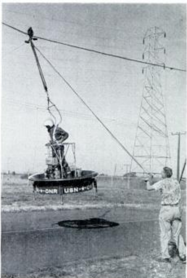
The platform goes straight up, down or sidewise. Pilot changes direction just by shifting his weight. Below, safety tether used in test flight saves pilot and craft from sudden letdown if trouble develops
