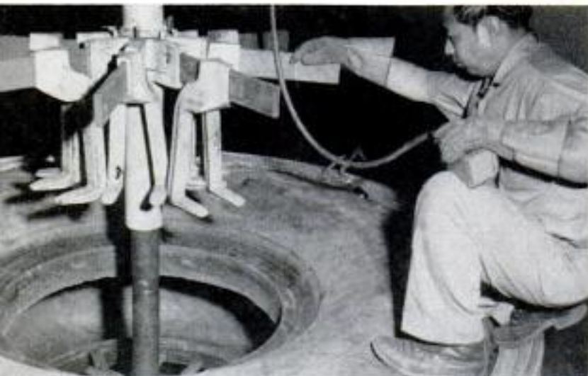
New tread is formed in a big mold, shown under man's right foot. Below, the mold is pulled upward, exposing "new" tire
