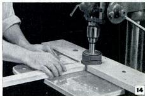
When squaring the end of a narrow strip use a follow block to guide end of strip past fence opening. This precaution assures a square end on the stock
