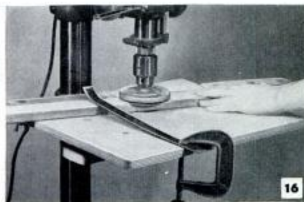
Above, a shaper fence can be used with drums 2 in. or less in dia. Fence is adjustable to proper offset. Below, disk sander is efficient unit for surfacing either hardwood or softwood to a uniform thickness
