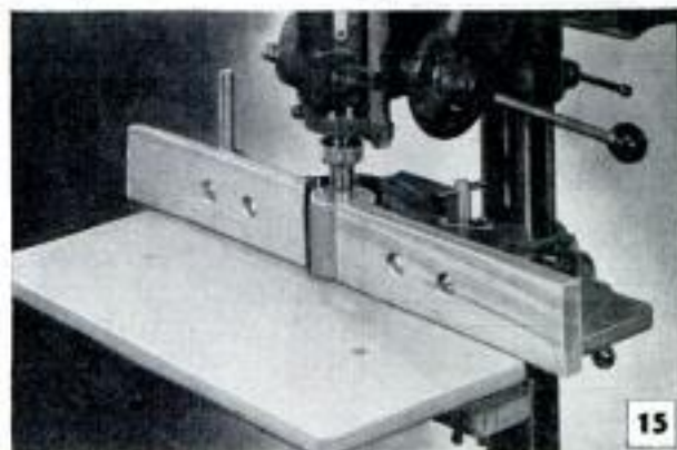
Above, a shaper fence can be used with drums 2 in. or less in dia. Fence is adjustable to proper offset. Below, disk sander is efficient unit for surfacing either hardwood or softwood to a uniform thickness
