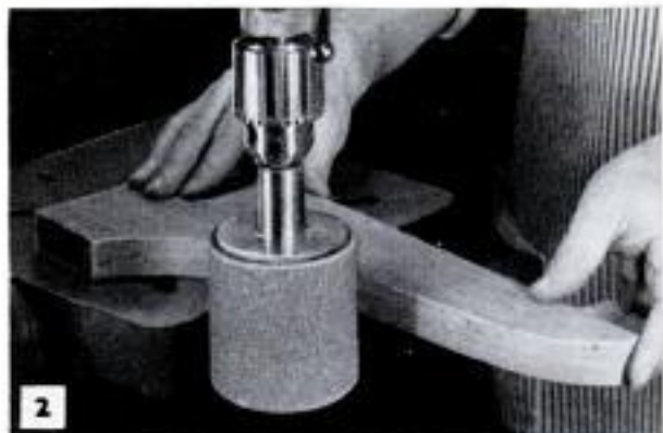
2 In some cases where work is small size, drum can be worked off edge of machine table in manner pictured. Lower end of drum should be below surface of table
