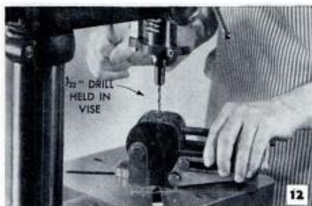
When drilling spindle, place drill bit in vise and lower spindle onto it slowly. Use very light feed
