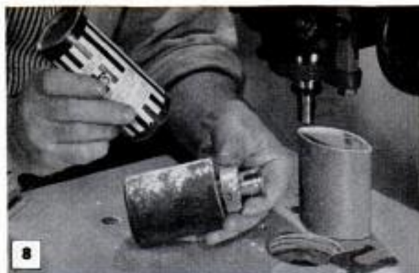
8 Coating the soft-rubber drum with commercial talcum powder will prevent sticking of the abrasive sleeve
