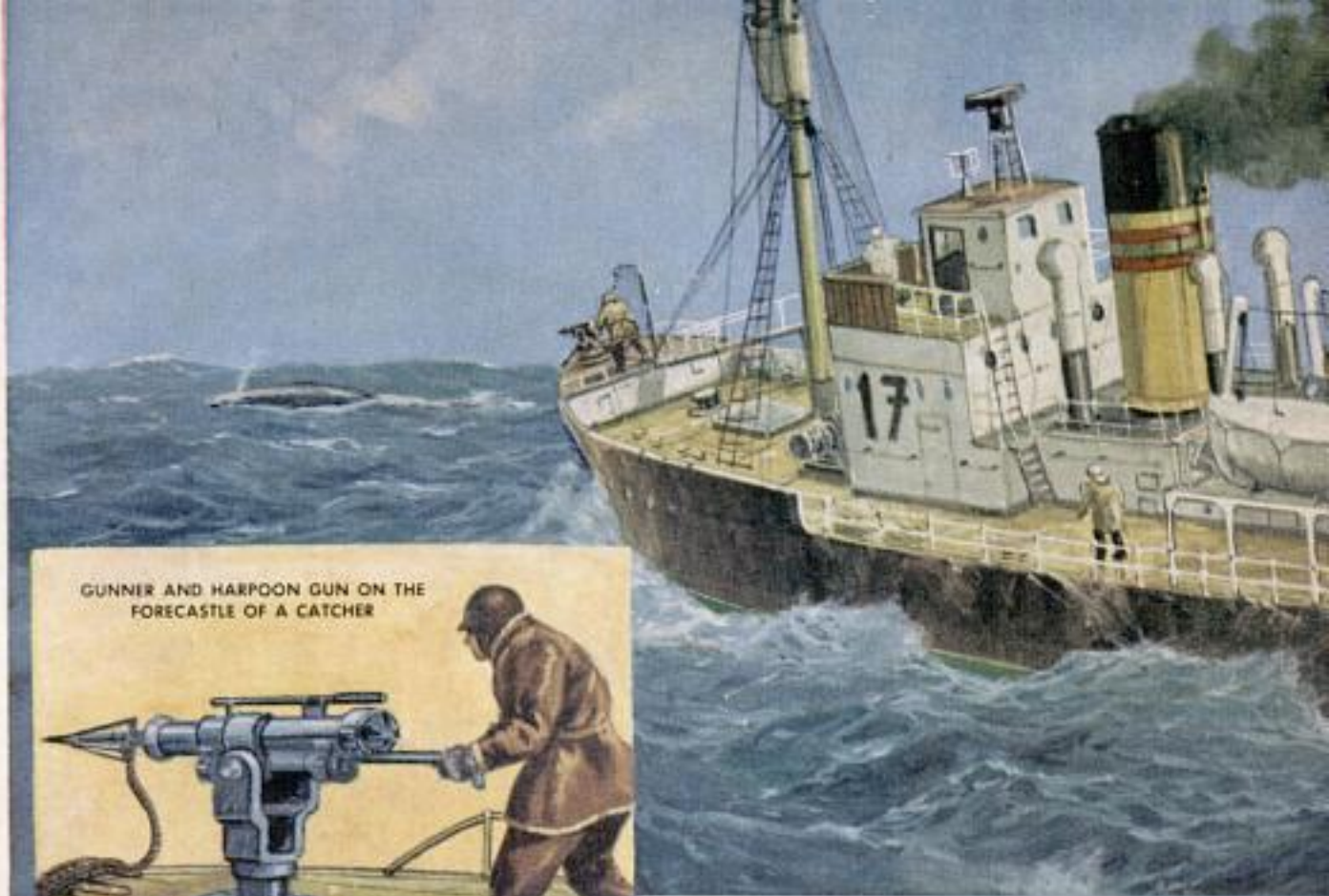
A Dutch "corvette" catcher approaches its target, a spouting blue whale. Gun on forecastle fires a harpoon that explodes and snaps open in whale
