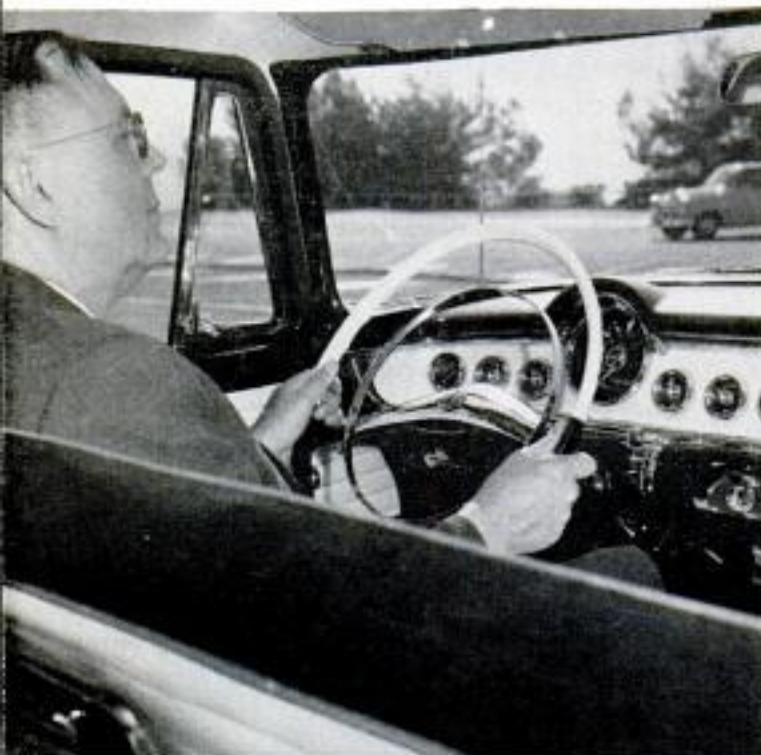
Driver's position and dash are fine, says Clymer, but he still objects to horn ring blocking view of panel
