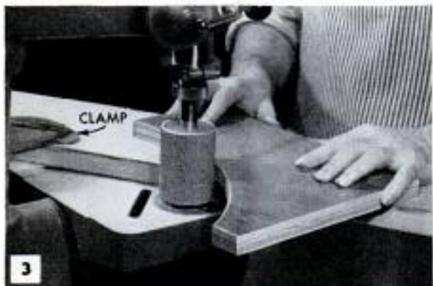
3 Above, purpose of auxiliary table is to permit running drum with its lower end below surface. Below, table with raising cleats allows drum to be adjusted up or down to equalize wear on the abrasive sleeve
