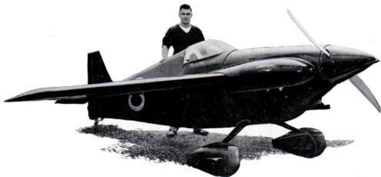
Many homebuilders seek more speed than that built into ordinary light planes and turn out slick racing jobs like the 180-mile-per-hour Pitts Special , below. Engine turns up only 85 horsepower
