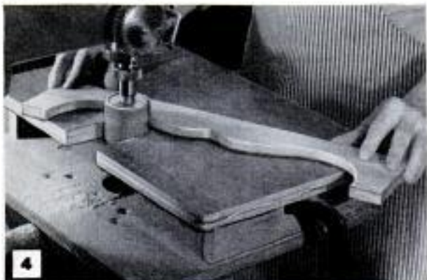
3 Above, purpose of auxiliary table is to permit running drum with its lower end below surface. Below, table with raising cleats allows drum to be adjusted up or down to equalize wear on the abrasive sleeve
