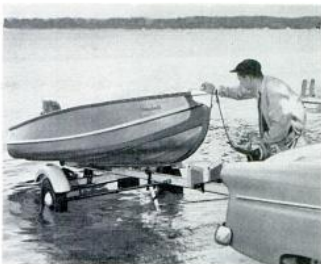
Launching boat is easy. Back trailer so end of boom is at water, release winch lock and push boat into water
