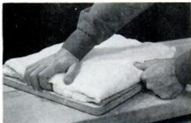
Above, three layers of roll cotton, or the equivalent in foam rubber, are used as padding. Below, the material covering the backs of the chairs is held in place by large-headed, decorative furniture nails
