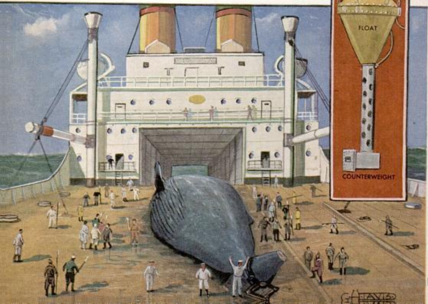
Radio beacon in buoy transmits a distinctive signal that helps a retrieving vessel locate a floating whale carcass. Dead whales may drift for miles after killer vessels cast them loose. In background is one of the latest Norwegian catcher ships. Below, a blue whale just after it has been pulled from sea up slanting skidway to ship's deck
