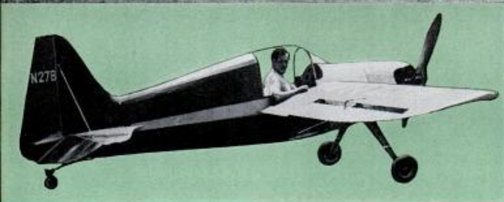
Many homebuilders seek more speed than that built into ordinary light planes and turn out slick racing jobs like the 180-mile-per-hour Pitts Special , below. Engine turns up only 85 horsepower
