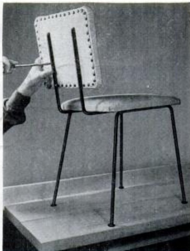
Final assembly is completed by attaching the seat and back of the chair to the metal frame with screws
