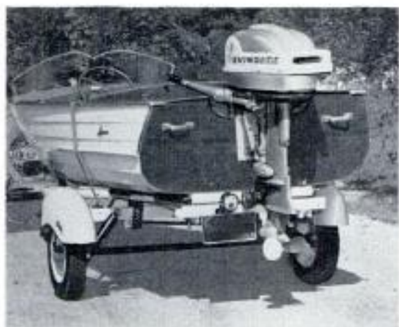
To bring boat out of water, fasten winch rope to bow, line up boat with the trailer boom and reel in the boat
