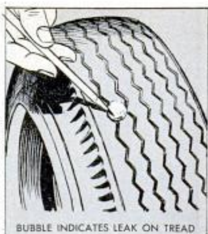
SOAP SOLUTION LOCATES LEAKS
