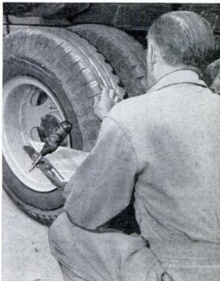
Above, gouged tread is a clue to how driver handles his truck. Below, dual tires must be mates. Towner's square shows they are
