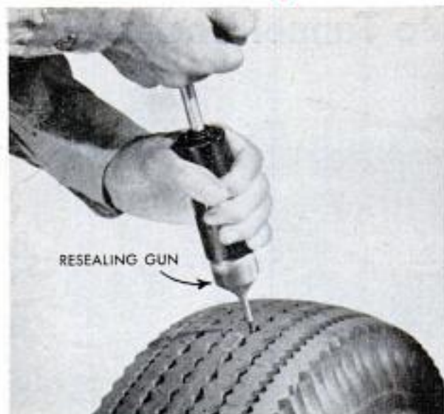
Small punctures up to 1/16 in. in dia. can be repaired with a gun containing fire-resealing compound
