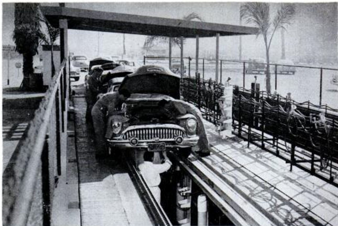
Men, cars and equipment move at the same speed on the endless conveyor, which handles five cars at once
