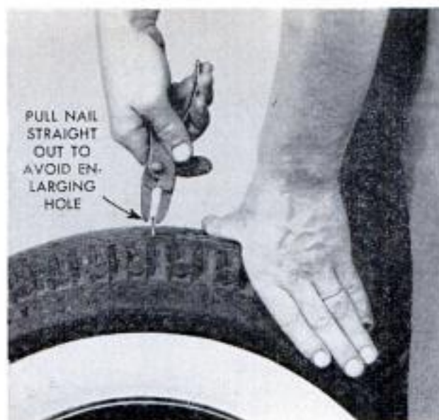
Small nail usually causes a leak even though it remains in tire. Use care in removing with pliers
