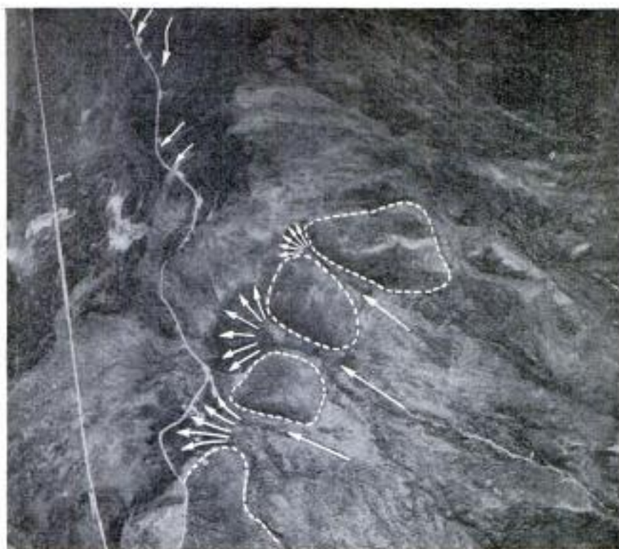
White arrows indicate natural erosion that might destroy old Canadian road. As result of study, new straight road was built as shown at left. Dark line (below) indicates Belcher's recommendation for pipeline route to reduce costs and repairs. Corrosive areas may cause trouble in future
