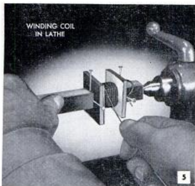
Coil for the electromagnet is wound on a form to assure correct size to fit over center leg of core
