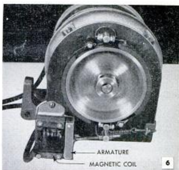
The electrically operated brake is controlled by the motor switch which is supplied with the lathe
