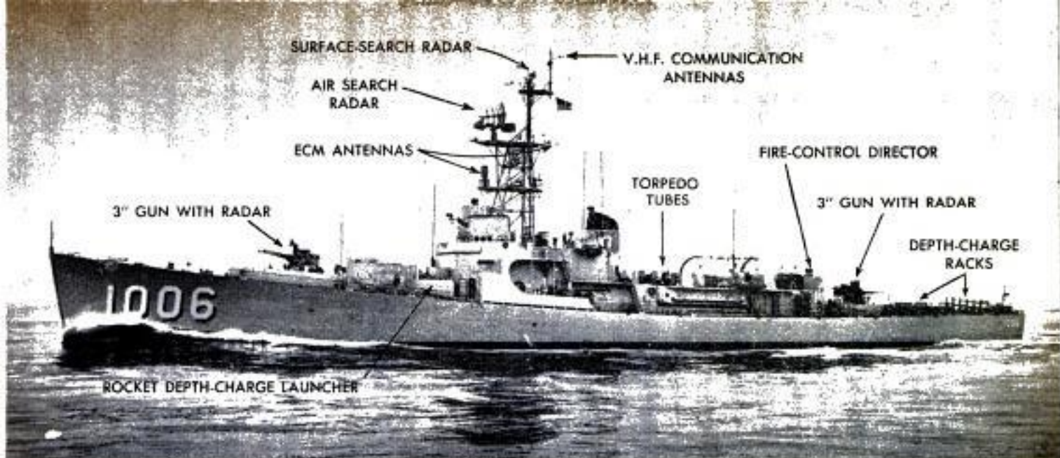
USS Dealey, first of the new destroyer escorts, bristles with armament and radar. It's longer and faster
