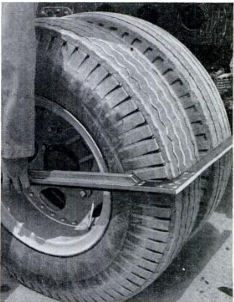
Above, gouged tread is a clue to how driver handles his truck. Below, dual tires must be mates. Towner's square shows they are
