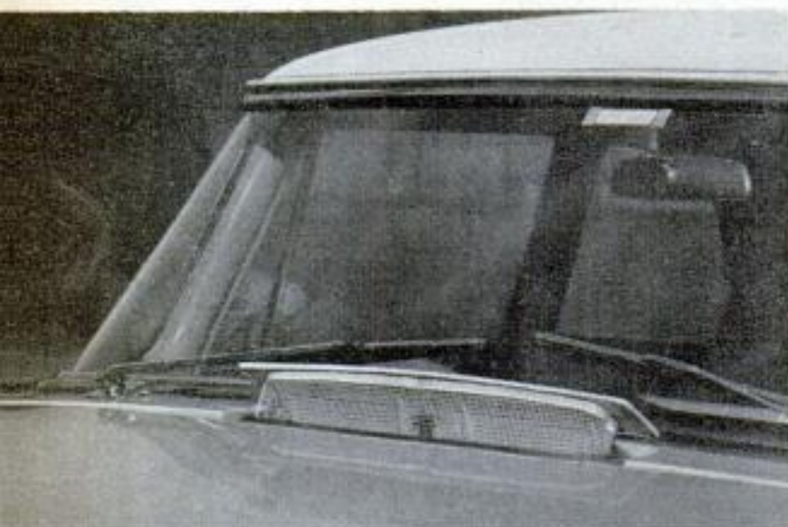
Plymouth, like other Chrysler-built cars, keeps the push-up cowl vent. Clymer likes it. Some of the Plymouth owners don't
