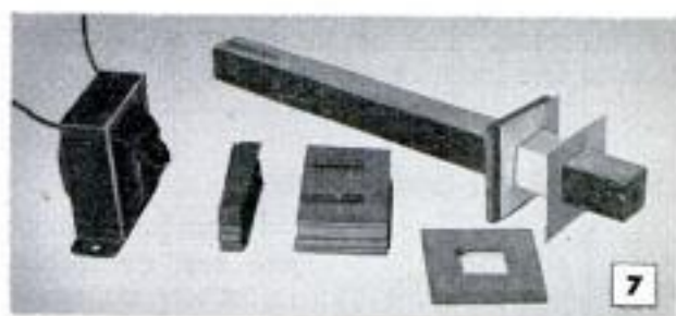
A discarded radio transformer supplies the iron core for the electromagnet. Note coil-winding form
