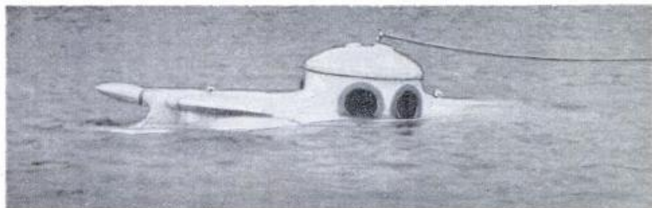
With its two "eyes" above water, the sub moves under own power. Telephone line leads to the mother craft
