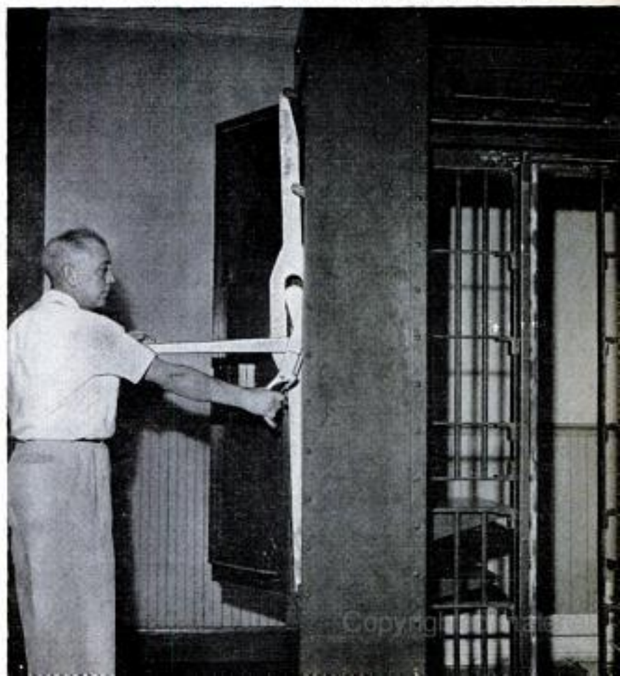
Engineer with full-scale model of maximum-security cell shows how door control works. One man can easily open or close any combination of up to 50 doors. All doors are operated manually
