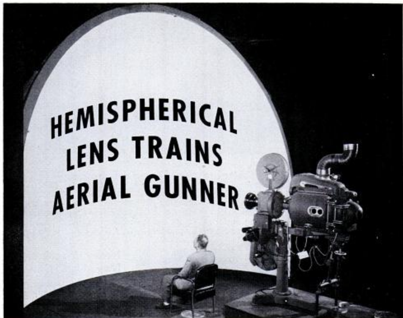
Screen on which movies are projected is half a hemisphere. Larger screens are used for audience presentation
