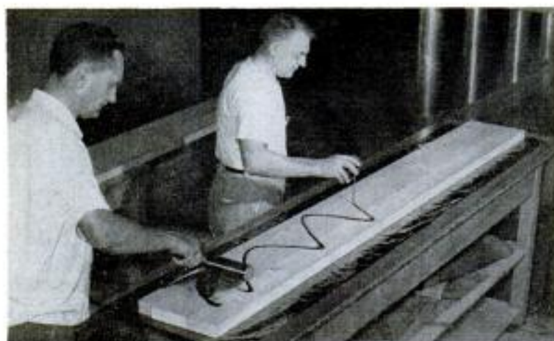
Two-inch plank made up of knotty narrow pieces edge-glued together is spread with synthetic resin. Paper overlay, below, is laid in place on top of glue. The overlay contains waterproofing resin
