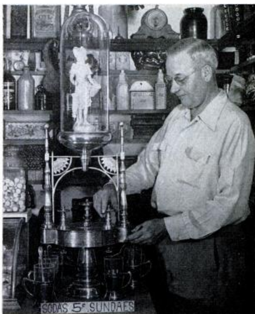
Silver-plated soda fountain was made in 1874. Syrup and other soda ingredients were kept in kegs and forced to spigots by air pressure
