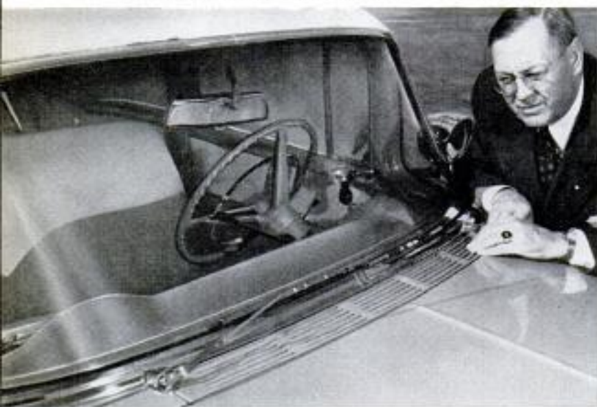
Above, heater intake is on cowl. Below, Clymer likes driving position. Note the slight distortion of wrap-around windshield
