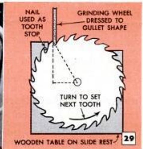
Above, when filing a circular blade it is essential that it be held rigidly to prevent vibration under the file stroke. The vise pictured and detailed is suitable for blades 6 to 10 in. in dia. Below, after blades have been filed several times the shortened teeth will require reshaping and gumming
