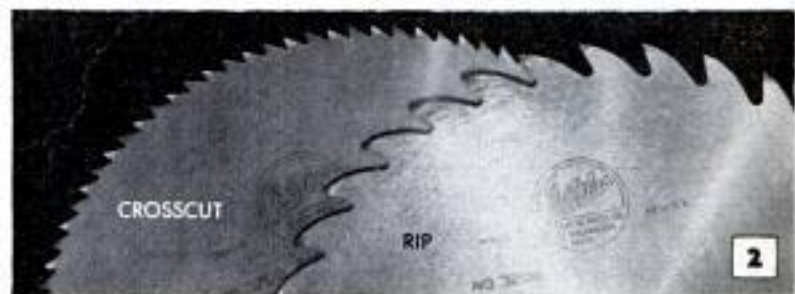
BASIC TYPES OF SAW BLADES—CROSSCUT AND RIP
