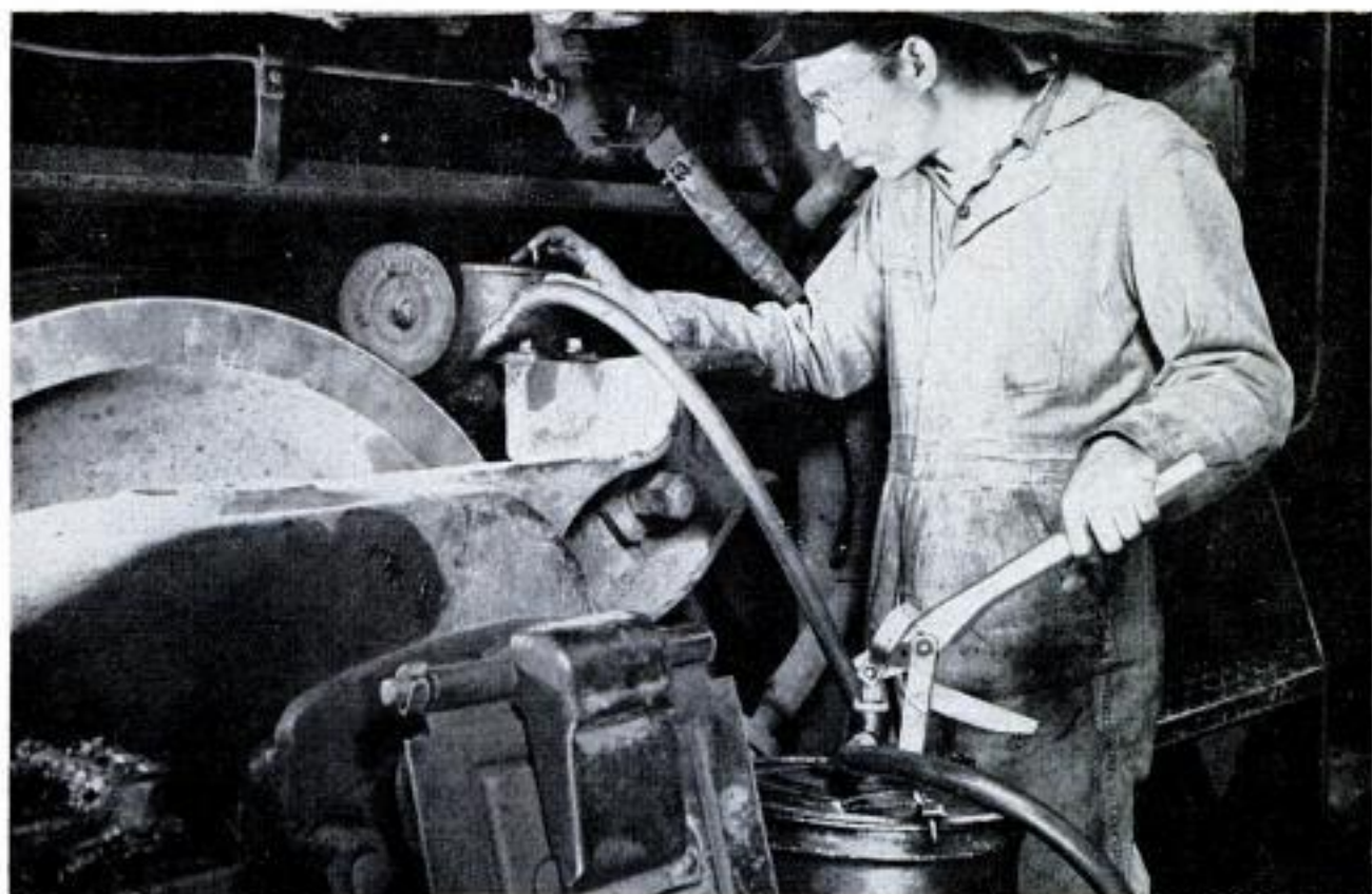
Lubricator, filled every 500 miles, mounts above locomotive wheel and coats wheel flange with graphite grease
