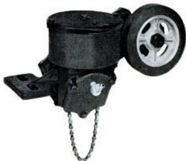
Lubricating chain rotates continually. Swaying motion of train causes chain to slap against wheel flange and deposit its grease
