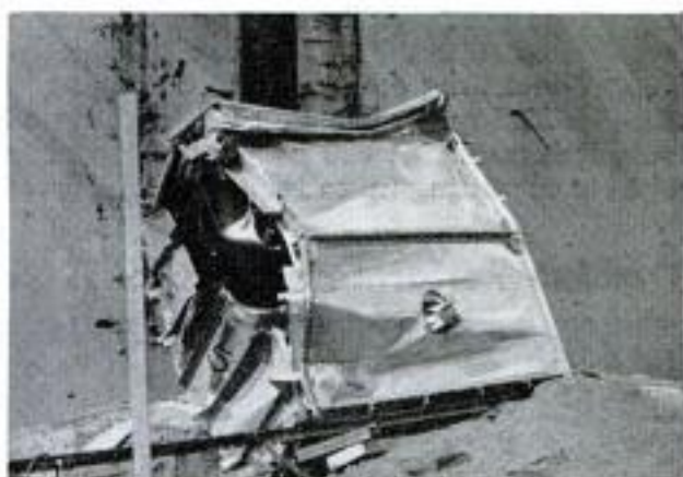
The aluminum wing section was smashed to scrap, but the bladder-cell tank it held did not lose a drop
