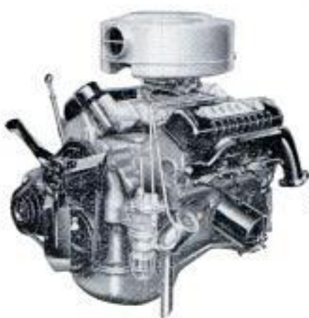
182-h.p. Y-block Special V-8 272 cu. in. displacement, 8.5 to 1 compression ratio.
