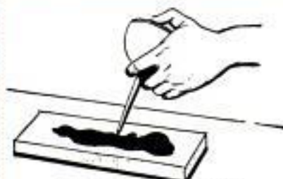
PLACE A FEW DROPS OF OIL ON THE OILSTONE BEFORE USING
