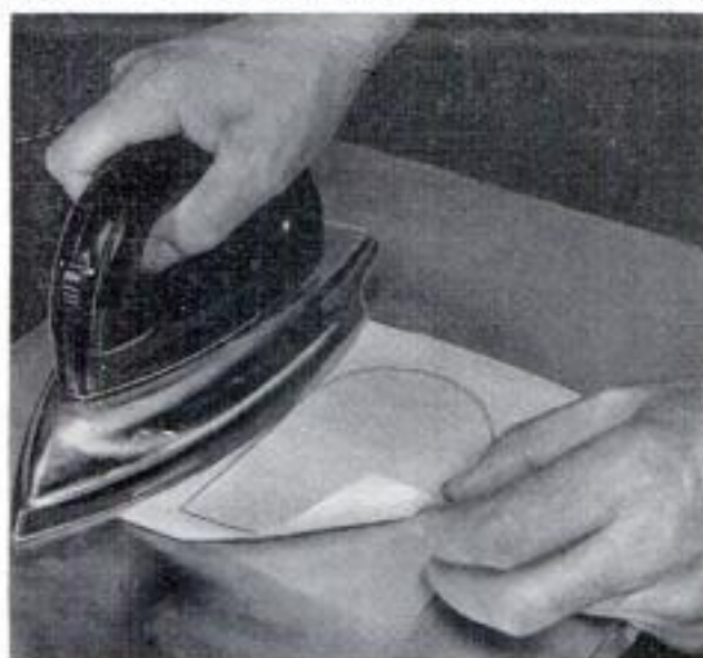
With tracing-paper pattern in position, plastic is heat-welded with iron. The iron is set for low heat
