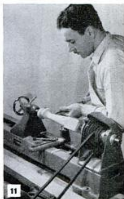
Light filing and sanding are necessary to remove sharp edges and shape foot to the required contour. Waste piece is sawed off
