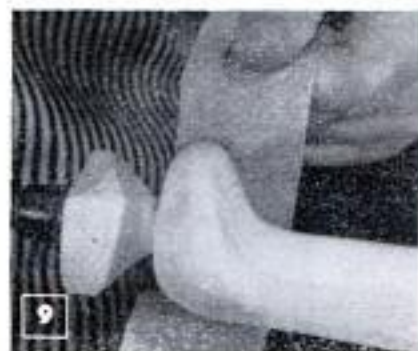
Careful sanding smooths the foot ready for finishing in color desired
