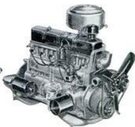
120-h.p. I-block Six 223 cu. in. displacement, 7.5 to 1 compression ratio.
