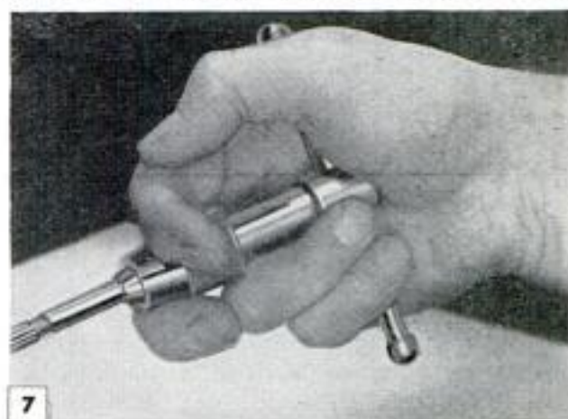
Grip chuck wrench in this manner for accurate work
