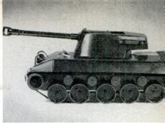
The three photos above show the detailing of the 76-mm. tank. Note the air-intake screen, the headlights and the pivoted gun turret. The idler wheels are made from .38-cal. cartridges, others from sheet metal or wood
