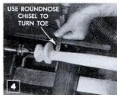
Body of turning and front of foot are turned down on true center
