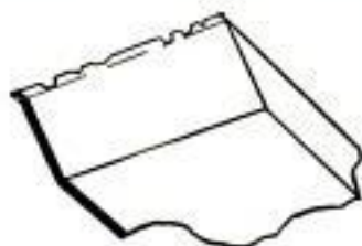
GRINDING FORMS BURR ON EDGE
