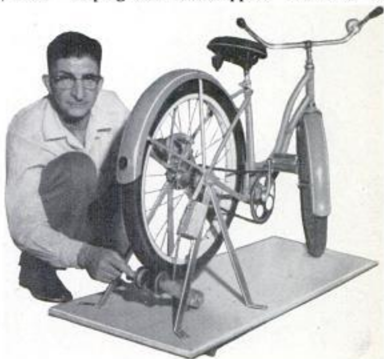
Stationary bicycle permits leg exercise. Roller on rear wheel stiffens pedaling
