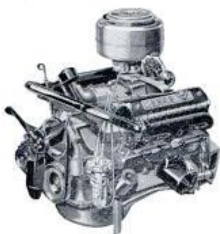
162-h.p. Y-block V-8 272 cu. in. displacement, 7.6 to 1 compression ratio.
