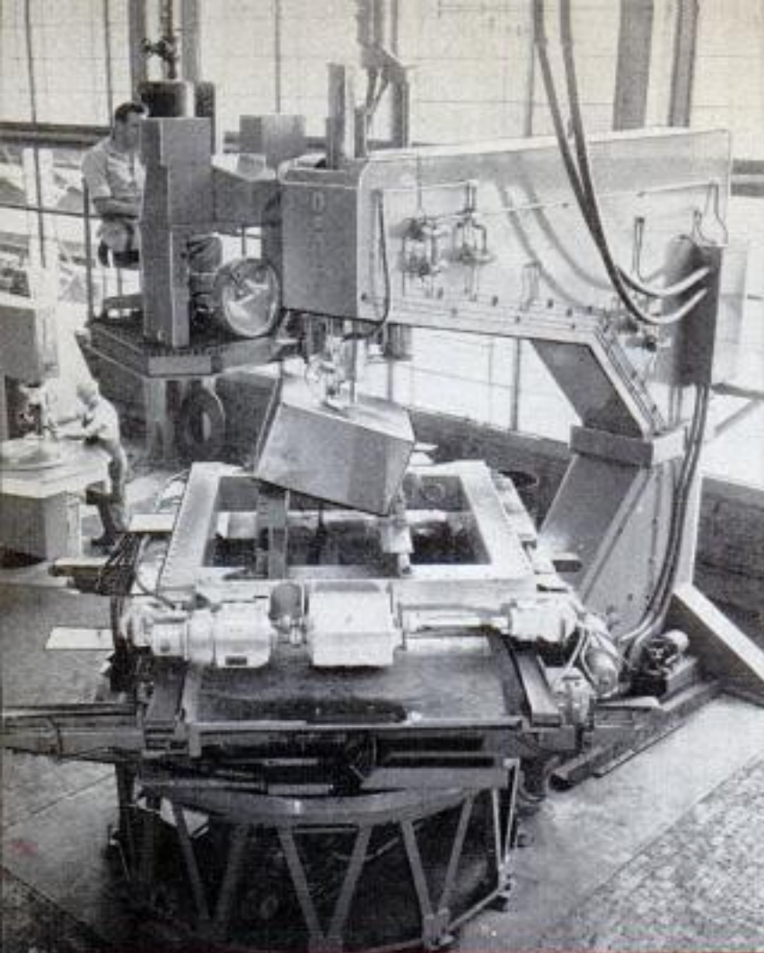
Operator of the world's largest metal-cutting bandsaw cuts die blanks from control station at head of machine
