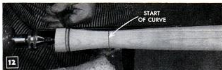
First step in making curved foot is turning into round on true center
