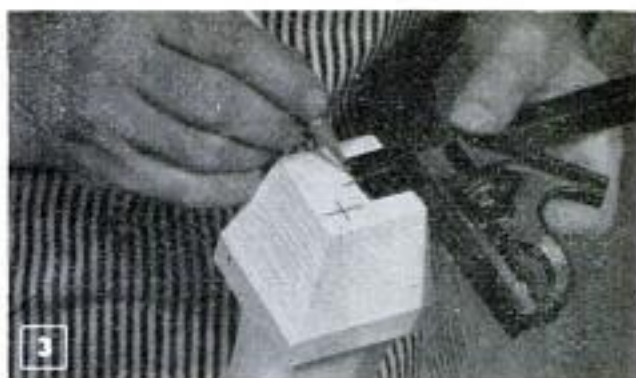
Locate the offset centers from the two flat sides of work. Here the offsets are made on the diagonal
