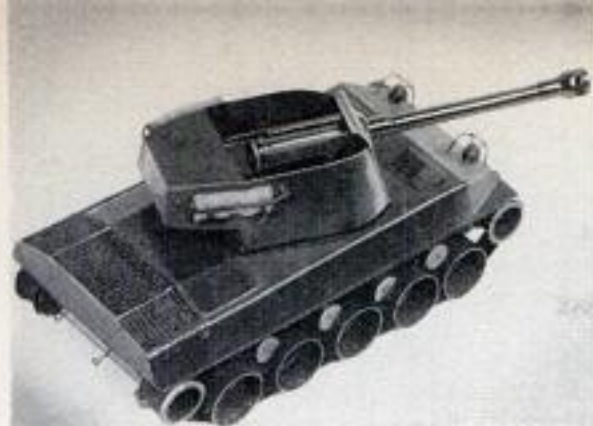
The three photos above show the detailing of the 76-mm. tank. Note the air-intake screen, the headlights and the pivoted gun turret. The idler wheels are made from .38-cal. cartridges, others from sheet metal or wood
