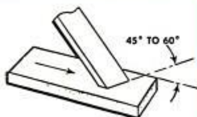
TOOL IS PUSHED EDGE FIRST OVER STONE
