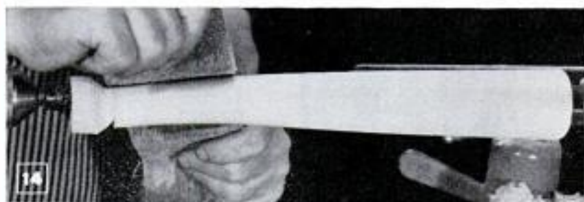
In the final step, ridges are removed by sanding and filing to contour
