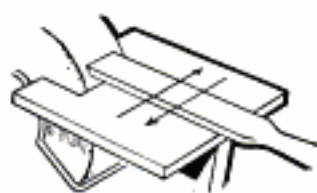
TOOL MOVED BACK AND FORTH ACROSS WHEEL FACE
