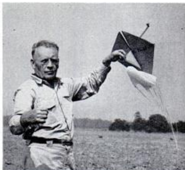
Inventor William A. Pruett demonstrates his kite yacht, which drops parachute or glider from kite altitude
