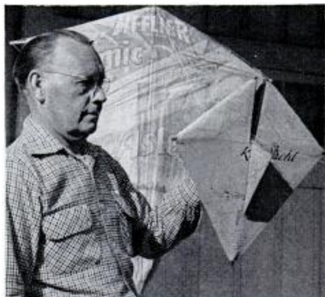
Inventor William A. Pruett demonstrates his kite yacht, which drops parachute or glider from kite altitude
