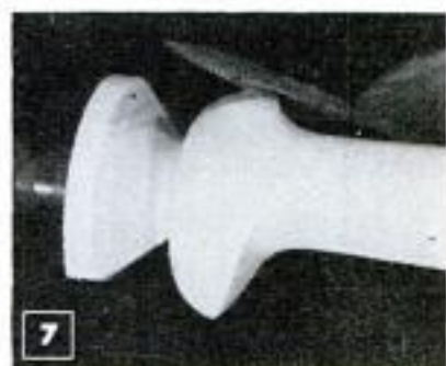
Light filing and sanding are necessary to remove sharp edges and shape foot to the required contour. Waste piece is sawed off
