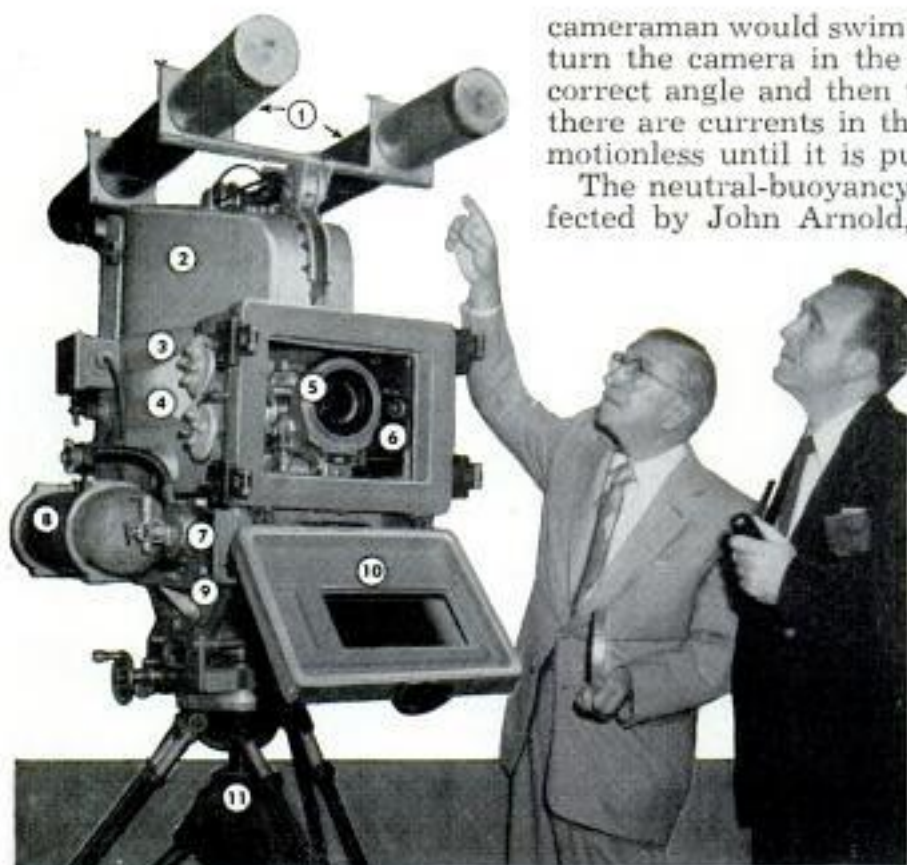
Inventor Arnold and director Sidney inspect underwater camera. The parts labeled are: 1. Stabilizer tubes; 2. Film magazine; 3. Focusing knobs; 4. Different lenses; 5. Wide-screen lens; 6. View-finder lens; 7. Camera's own aqua lung; 8. Compressed-air tank; 9. Self-contained batteries; 10. Front cover of waterproof blimp; 11. Tripod used only when on dry land.
