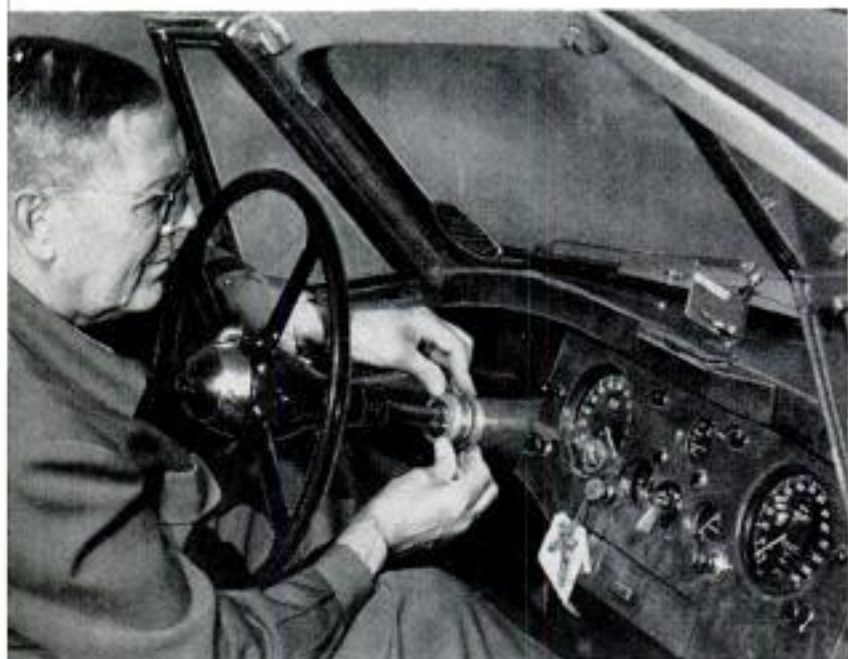
Telescopic column enables the driver to adjust steering-wheel position to suit himself. Instrument panel is made of hardwood
