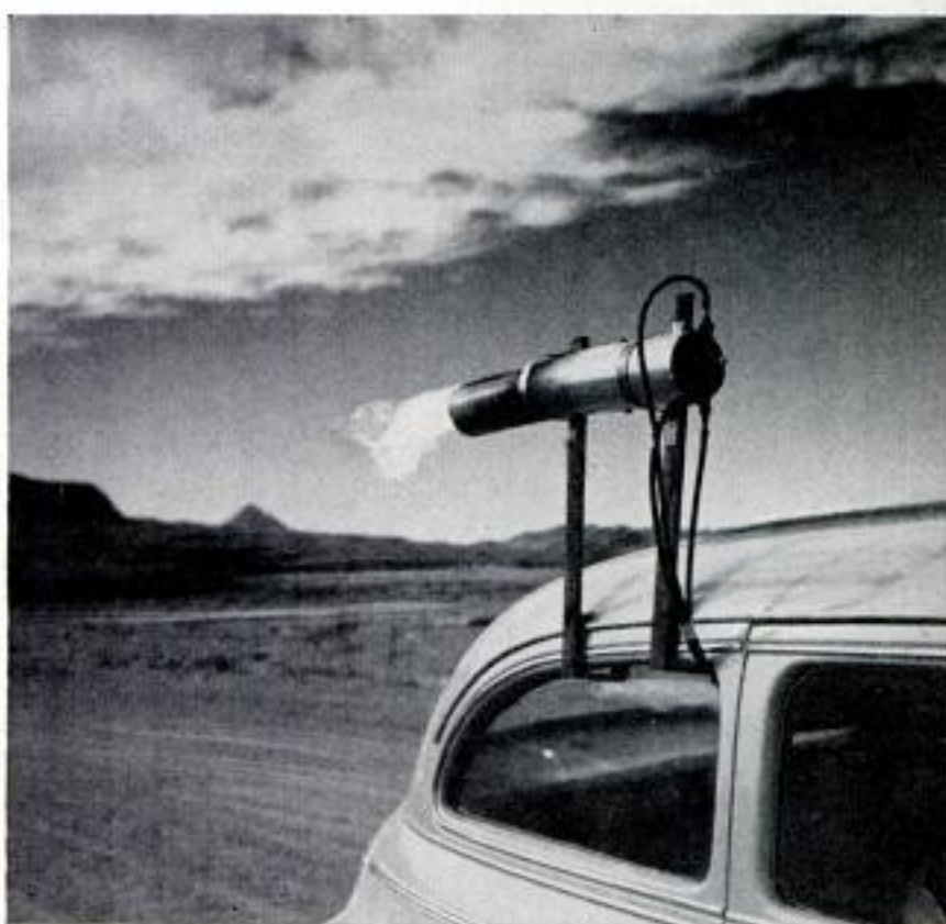
Generator on car creates clouds of silver-iodide smoke, seeding cloud formations in experiments to increase the rainfall
