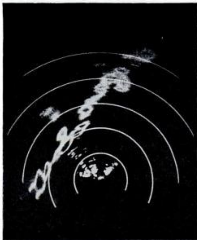
Dark storm centers, invisible on ordinary circuit (left), stand out with special weather wiring (right)
