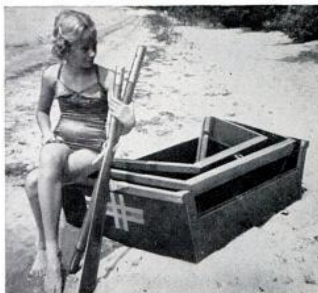
Above, the three sections are nested. Below, the boat is ready to have sides put on. Note that bow and stern are held at proper angle by temporary braces. Next step is to clamp sections together
