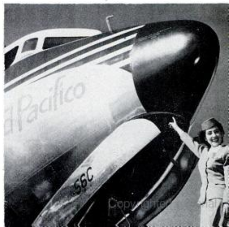
The black plastic radome on the nose of this DC-6 conceals and streamlines the weather-radar antenna
