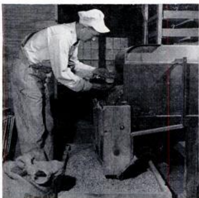
Infrared lamps around belt continue drying process Corn trickles slowly between stone grinding burrs
