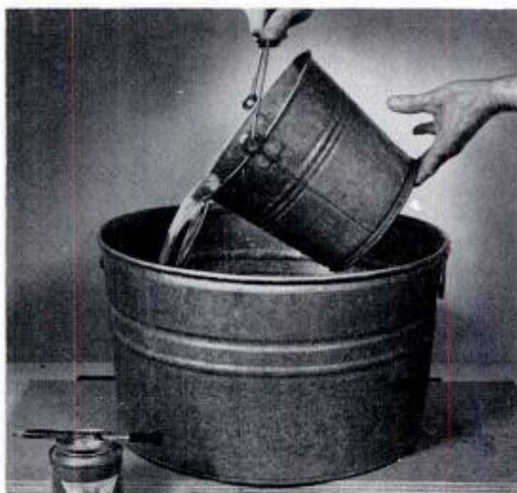
A tub filled with water makes a good "clamp" for flat work such as veneering a small surface. Place a piece of plywood under the tub to distribute pressure
