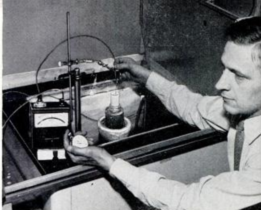
Doctor Reynolds measures the time that water, freezing in cup, generates electricity as indicated on the dial of the voltmeter
