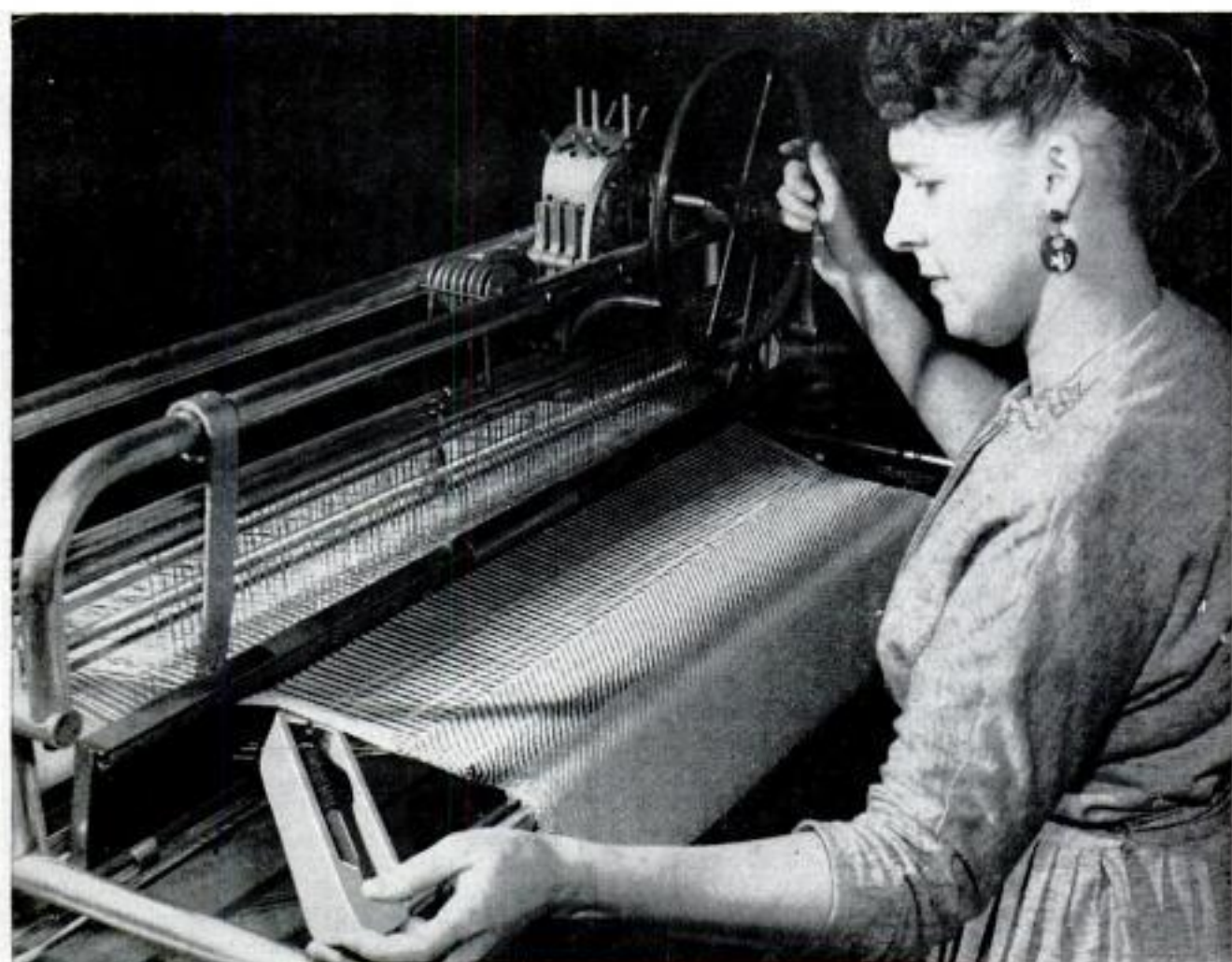
Here the boat-shaped shuttle is being thrown through the shed. Weft yarn unwinds from shuttle as it is moved
