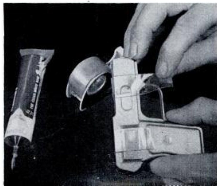
For certain clamping operations requiring light pressure, cellulose tape is useful. Simply spread glue on joining faces, locate parts and wrap with tape
