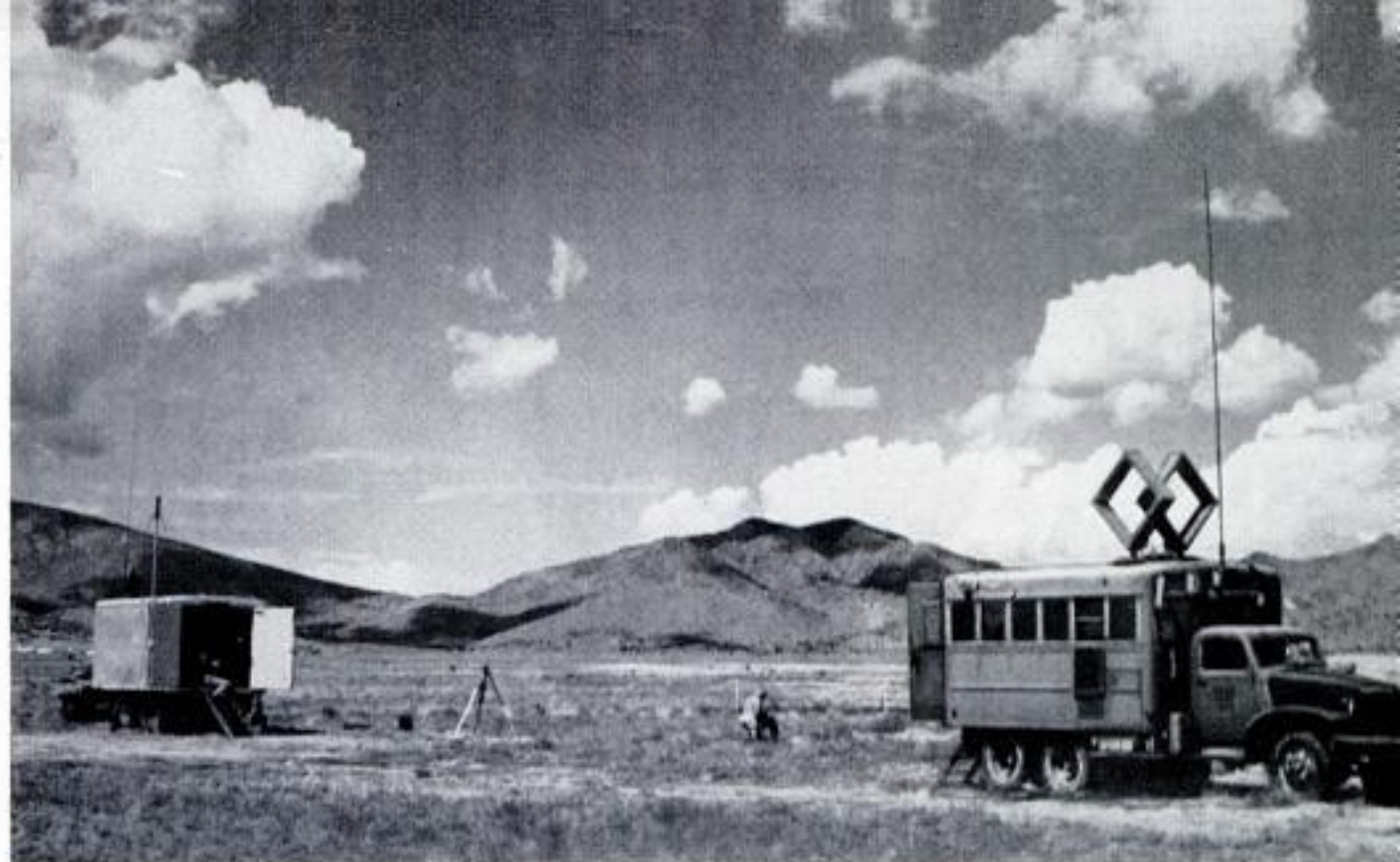
Radar truck tracks cloud formations and radio direction-finding truck records lightning 1000 miles away
