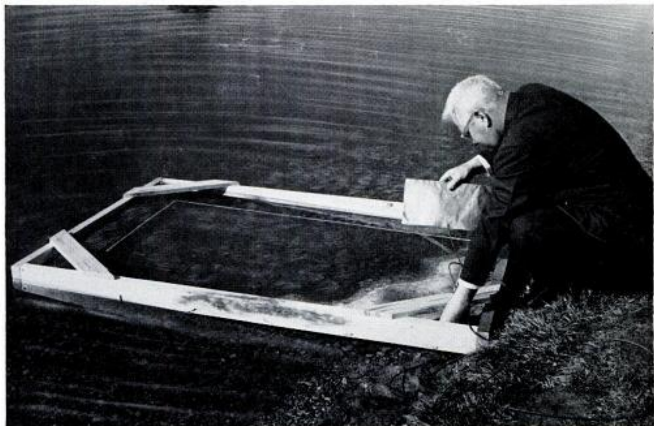
Floating copper screen measures voltage and amperage of freezing water. Metal sheet tests electrolytic action
