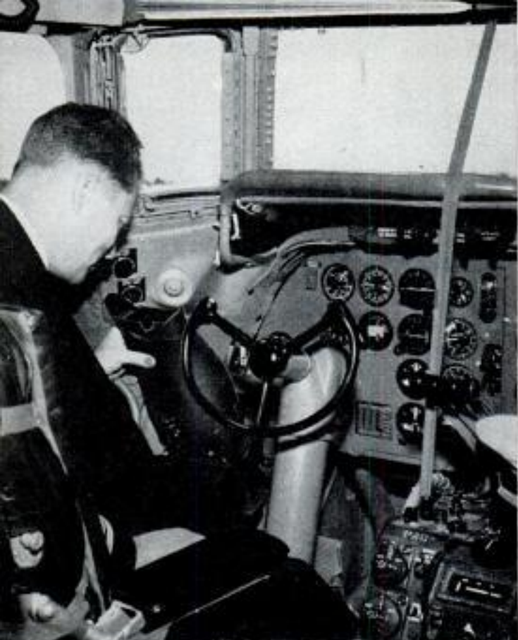
This Panagra pilot (top left) can see a radar "map" of the weather ahead in the hooded scope at his left
