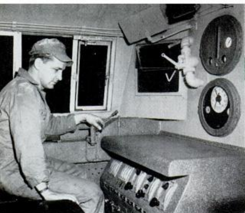
Automatic stoking in this coal burner takes the sweat out of the fireman's job. His cab has a minimum of simple controls
