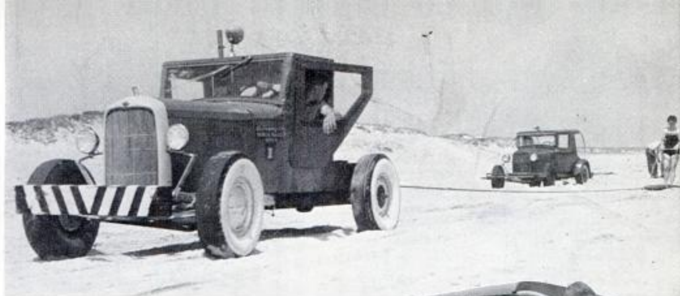
Converted Model A with vertical exhaust and oversize tires tows sledder. Handrails at right protect rumble-seat riders
