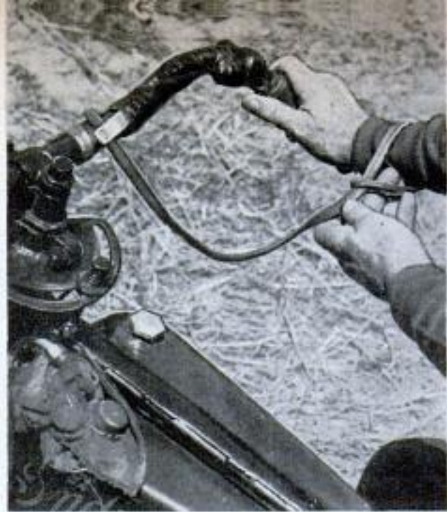
Safety rules require an automatic device to stop the engine if the rider is thrown off. When the thong is pulled from the handle-bar clip, ignition is grounded
