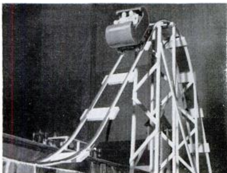
Roller coaster was 1953 addition. A chain pulls it to the top of tallest slide before its one-minute journey around island. A single \frac{1}{4} -horsepower motor beneath the platform powers every part of the display except the Wise Men on the wall above.
