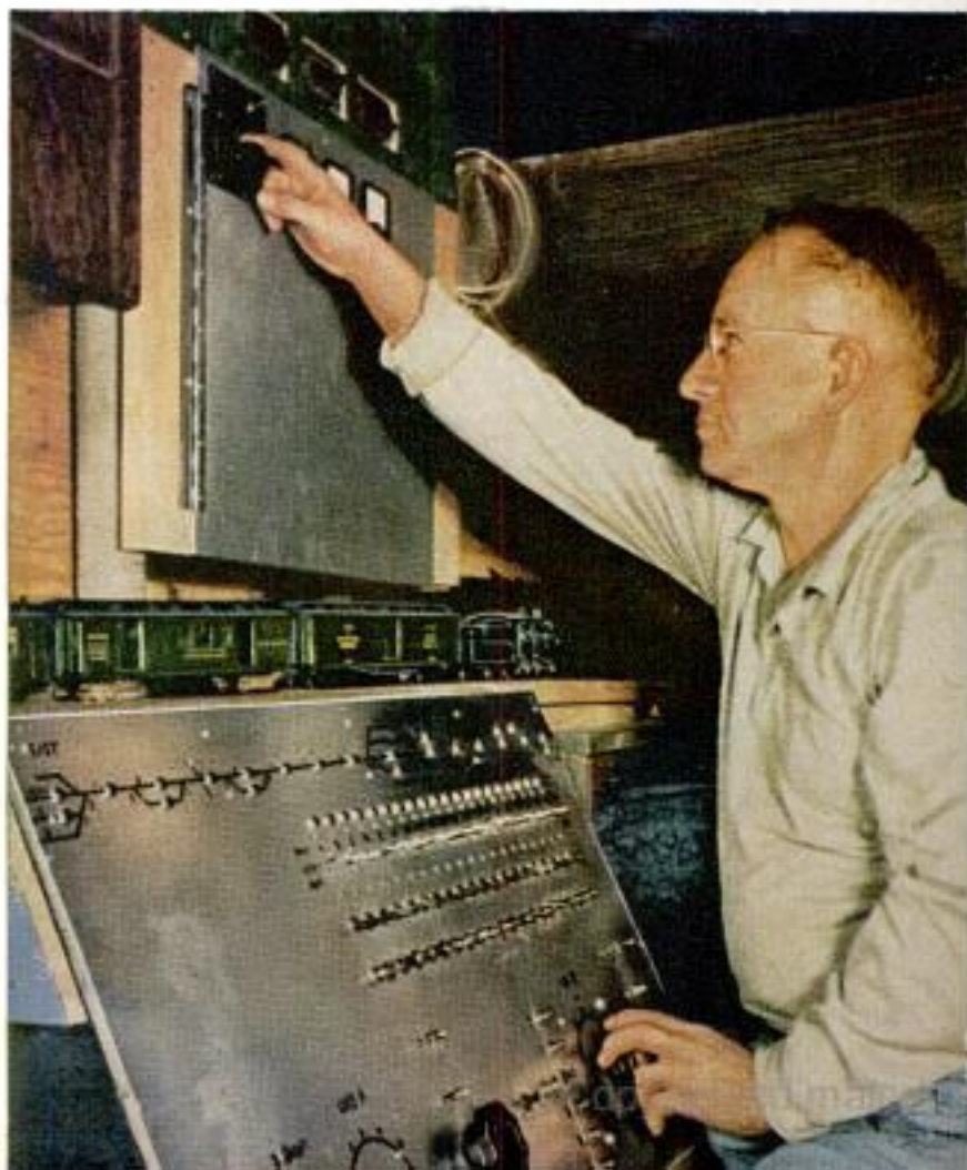
Part of trackage runs right across the top of the main control panel. Panel controls trains, lighting, cloud and sound effects
