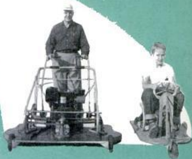
Big mower at left is driven by an eight-horsepower engine. Boy rides car his father designed and built
