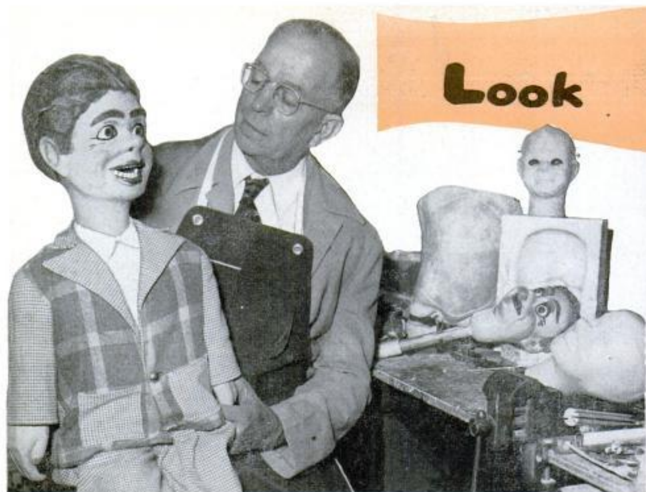
Cecil Gough holds one of the ventriloquist dummies he makes as a hobby. On the bench are examples of the stages of making a dummy head—the plaster molds, the plastic-cloth head and a completed head on stick
