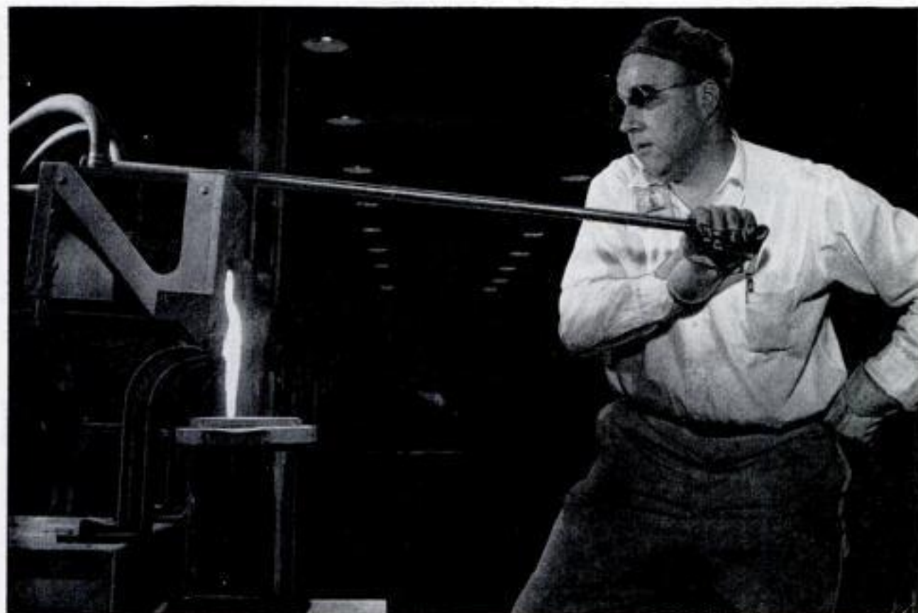
Laboratory worker pours molten Thermenol into mold. Metal is hot rolled and later rolled under moderate heat
