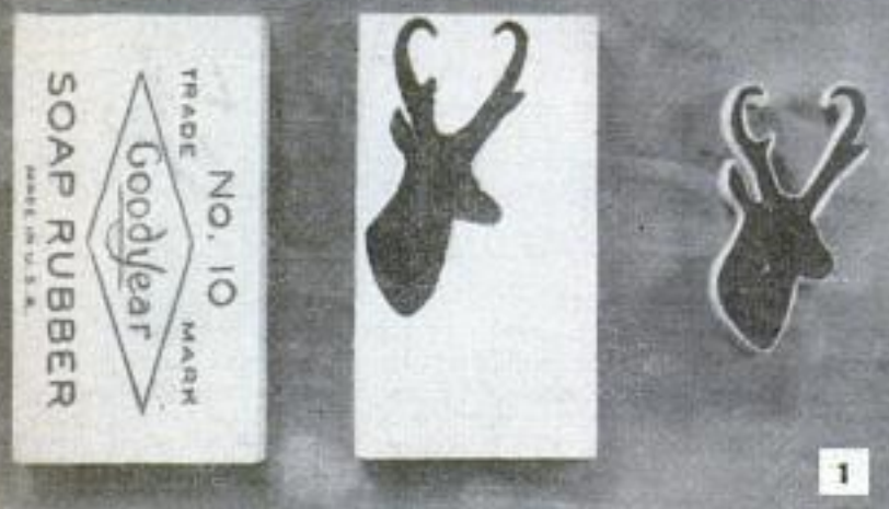
Pattern for plastic-inlay design is traced on soap-rubber eraser and cut out, as above. Sides of cutout pattern must be perpendicular. Below, pattern is placed in bottom of aluminum-foil trough and rubber-mold material is poured over it
