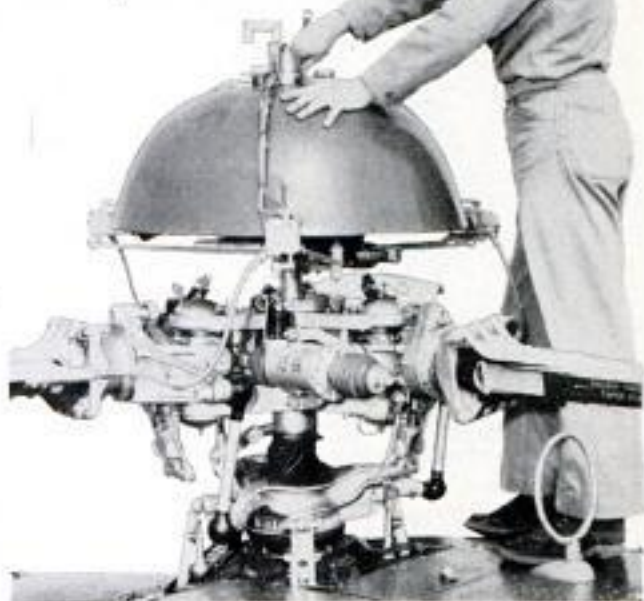
Dome-shaped tank on rotor holds special rocket fuel
