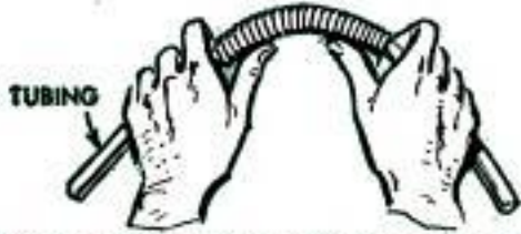
Bending tubing without kinking can be done by using a length of coil spring that fits snugly over tubing. Center the spring on point of bend, shape with thumbs placed as shown
