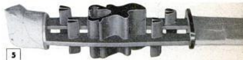
A second aluminum-foil trough is made, this time to enclose the entire knife handle. Holes and joints of trough must be sealed carefully and plastic poured in slowly, as shown below
