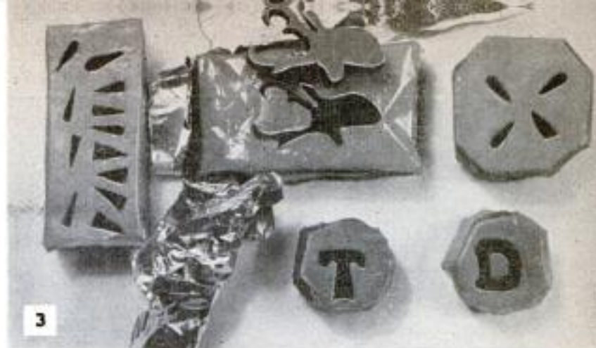
When material has cooled, remove foil trough and eraser pattern from rubber mold. Note various mold designs shown above
