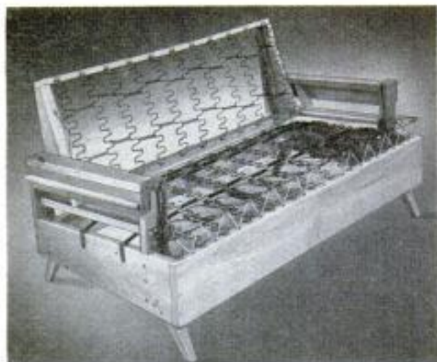
Above, this photo of the Davenette shows it ready for the foam-rubber padding. Note the spring edge wire that is required across front of T-type seat
