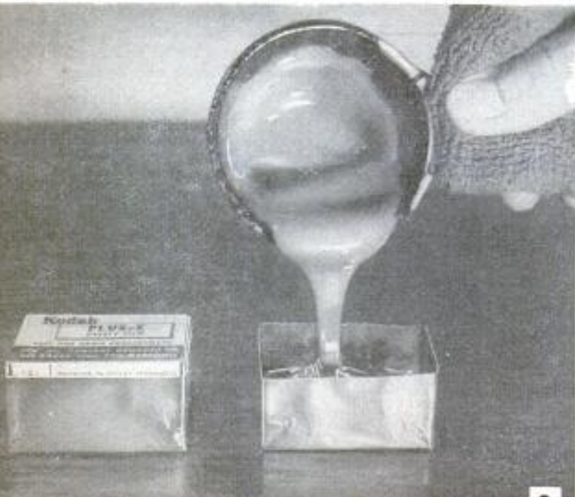
Pattern for plastic-inlay design is traced on soap-rubber eraser and cut out, as above. Sides of cutout pattern must be perpendicular. Below, pattern is placed in bottom of aluminum-foil trough and rubber-mold material is poured over it
