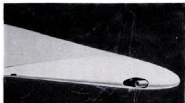
Except for pilot's controls, mechanism is mounted entirely on rotor (diagram, right). The small rocket engine rides inside streamlined rotor-tip fairing (above). Rocket exhaust, which provides thrust, is practically invisible and almost silent
