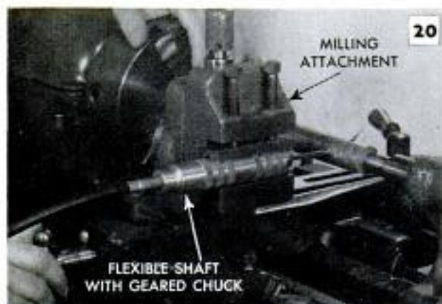
Accurate cross drilling can be done with flexible shaft held in milling attachment. Locate centers accurately
