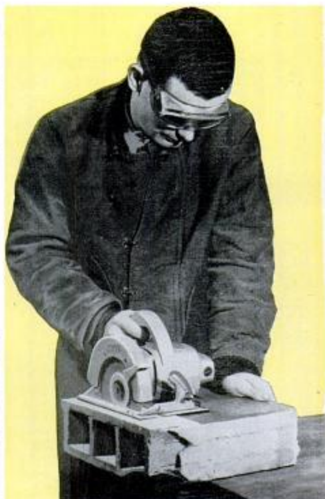
Above, note similarity of operations of cutting wood and clay tile. Saw is held in same manner. Woodcutting blade is replaced by abrasive disk for cutting tile. Right and below, saw squares up broken pieces of hollow tile and concrete for re-use
