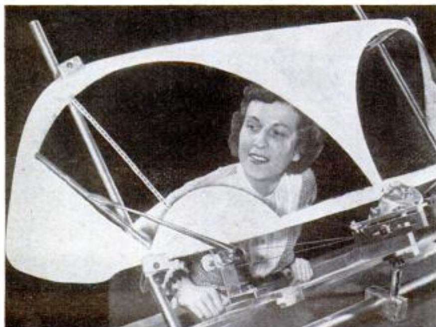
Dotted line is where usual blade stops. New type wiper 5½ inches more
