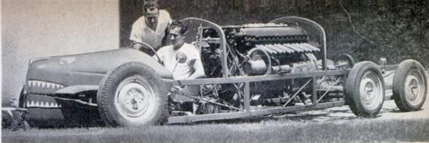
Monster's engine, taken from a fighter plane, is mounted behind driver. Car has a wheelbase of 17 feet
