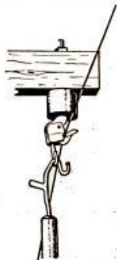
Key to the new "climbless" pole is this insulator. Ground crews use long-handled tools to place the wire in position and then lock it fast.
