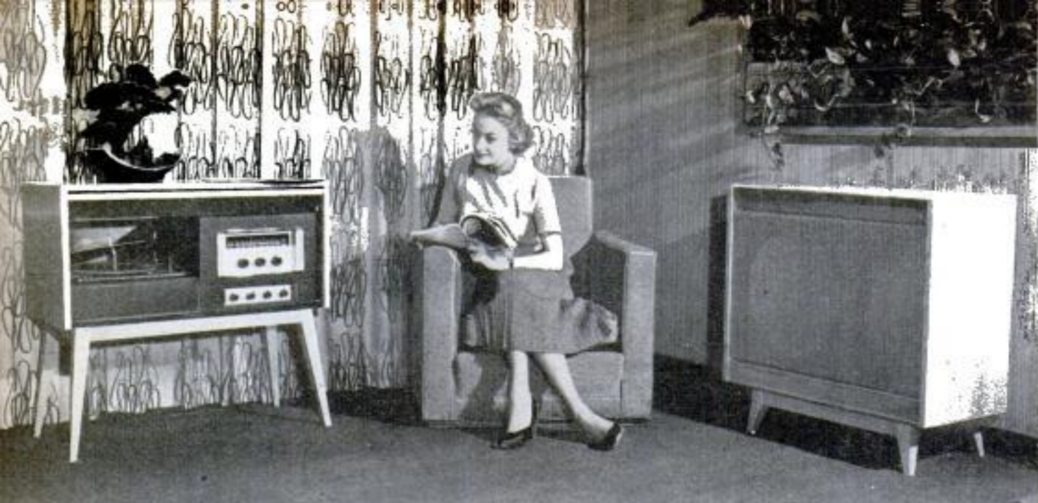
Modern open cabinet holds record player and preamplifier while cabinet at right holds amplifier and speaker
