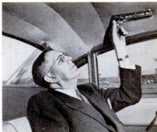
Cadillac's air conditioner introduces cooled air into body through four outlets similar to those on planes
