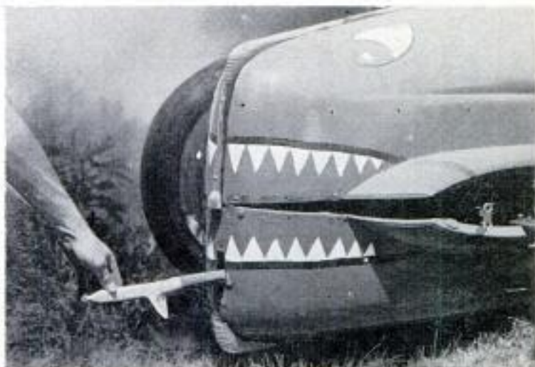
Projecting from the Monster's savage mouth is an air-speed indicator tube. It takes the place of an ordinary speedometer
