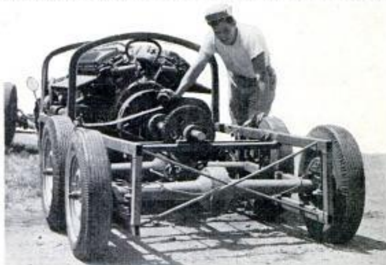
Tandem-wheel drive increases the traction and minimizes the tendency to "fishtail." Car has a clutch from a 30-ton tank
