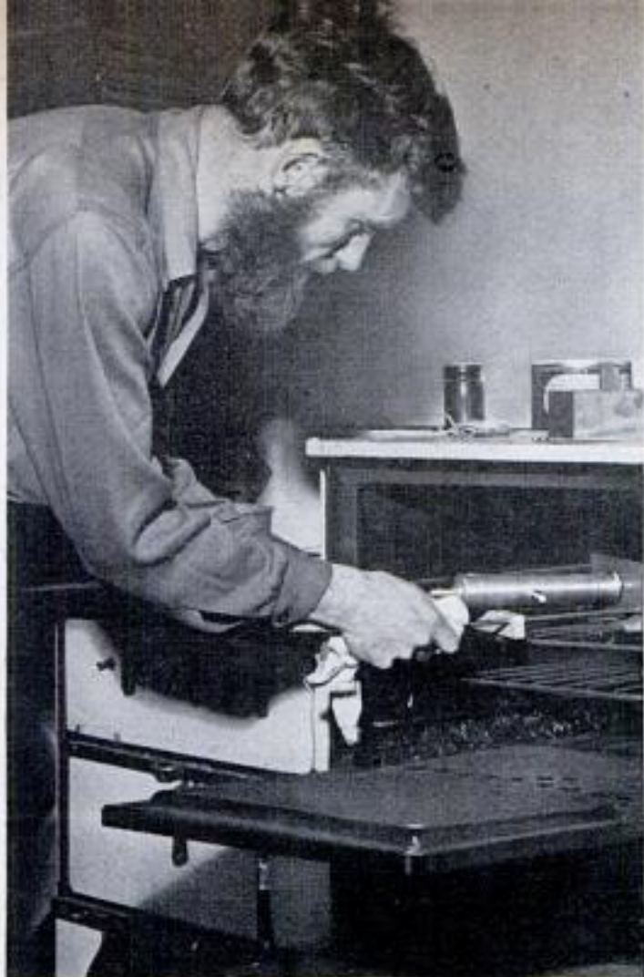
With the trunnions inserted in the holes, the barrel is heated in an oven to assure a good bond of solder
