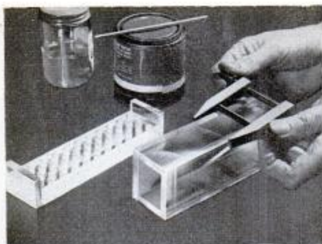
Sliding cover is assembled and clamped. Cellulose paper on block assembly assures sliding clearance
