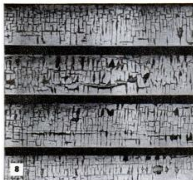
Paints applied must be compatible or cracking may begin within a few months. Above photo shows result of applying finish coat over incompatible undercoat. Below, wire brushing often reveals spots where paint is intact but has lost its bond with the surface. All such paint should be removed before repainting
