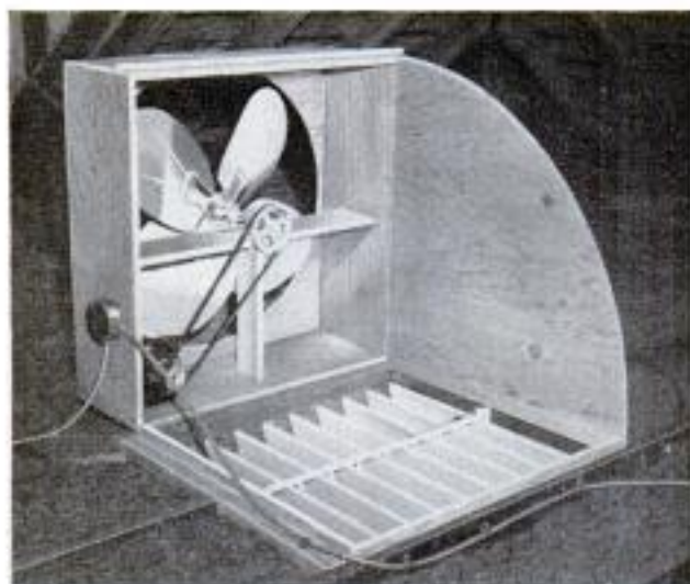
Suction box partially dismantled shows typical vertical installation of fan over ceiling grille. Pillow-block bearings do not permit horizontal mounting
