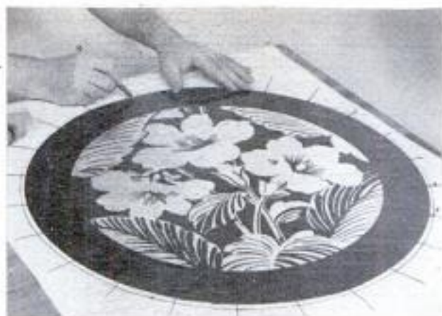
Flutes are spaced equally by laying out paper pattern, above, and transferring to disk. Bend as below
