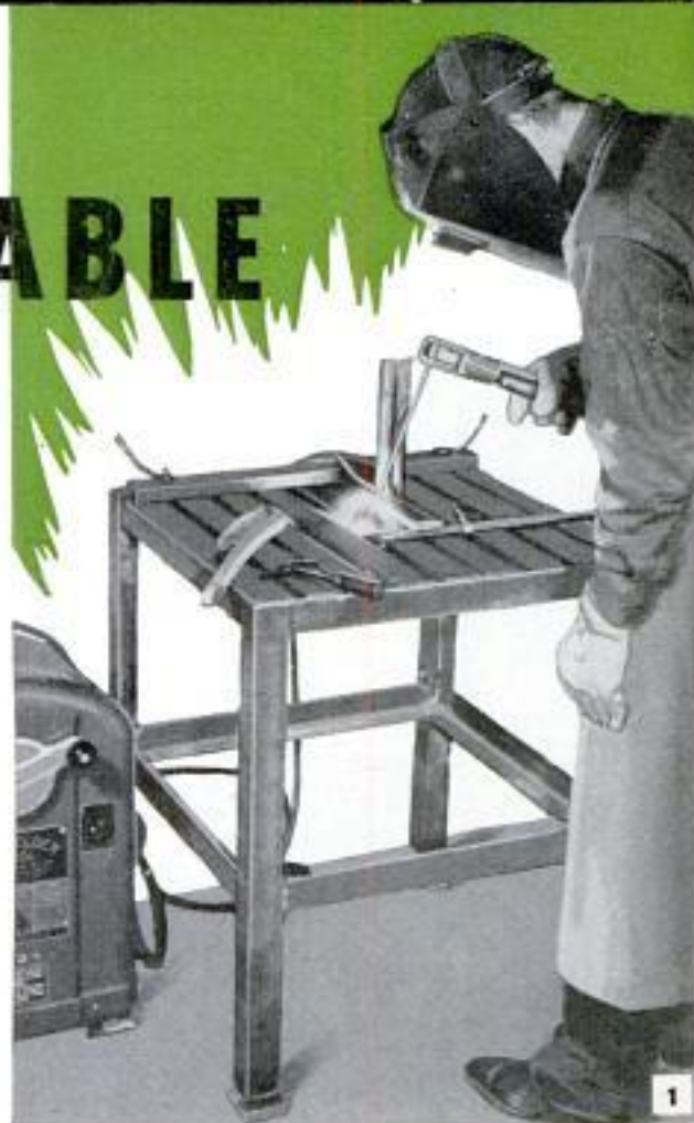
Above, slotted-top welding table in use. Slots permit clamping work in almost any required position. Below, circle, or ring, clamp holding work at angle. Unit is adjusted by means of leveling screws
