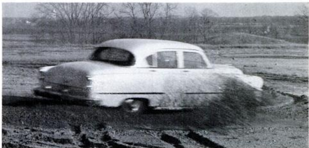
In the sand pit, a DeSoto does a series of figure eights to test traction, running gear and body tightness
