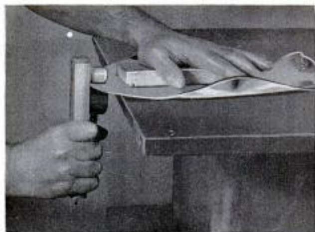
Fluting tool detailed at the right is shown in use in photos above and below. Note how sheet-metal disk is held flat with wooden block while flute is bent
