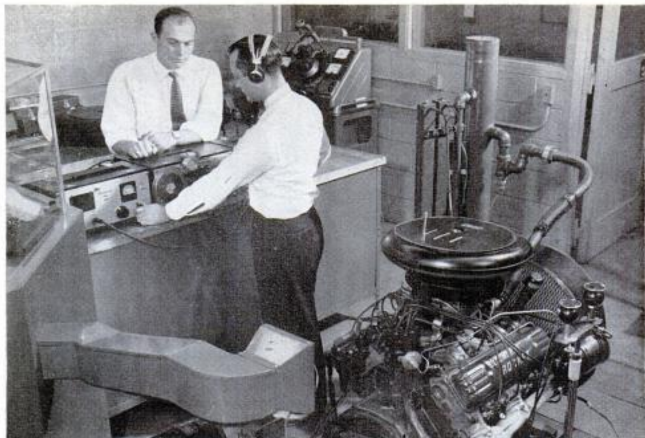
Engineers check valve noise in an Oldsmobile Rocket engine, an overhead-valve V8 first introduced in 1949
