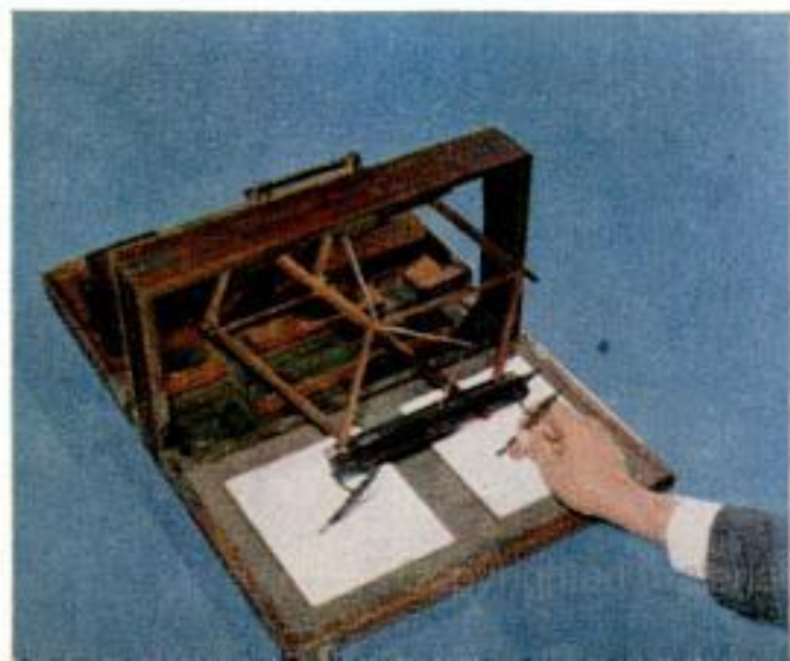
Jefferson used this polygraph to make copies of all his work. Copies have been invaluable to historians
