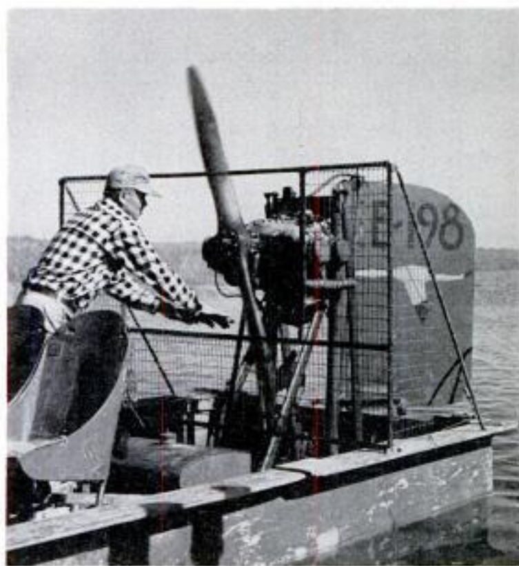
Operator spins propeller to start engine. Protective screen guards against accidents. Most boats are powered by airplane engines which have plenty of power but are no longer airworthy. The boats are usually made by their owners, cost up to $1000
