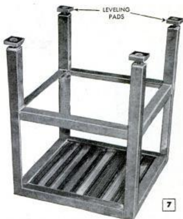
Welding table inverted to show the boxed sections of the four legs and the manner of assembling the leveling pads. By welding a long screw to each pad the table can be raised to any convenient height
