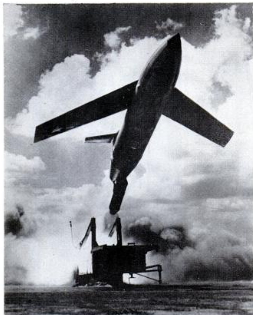
Standardized sections of the bomber are shipped in seven crates and assembled in field prior to launching. Matador roars away from its launcher with the aid of a rocket booster.
