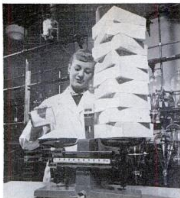
Quantity of beads on left of scales produces foam plastic on right. Twenty-pound plastic raft floats swimmer
