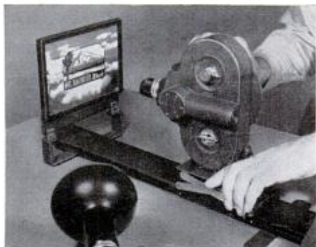
Superimposed decal and background print are placed between two pieces of clear glass before filming
