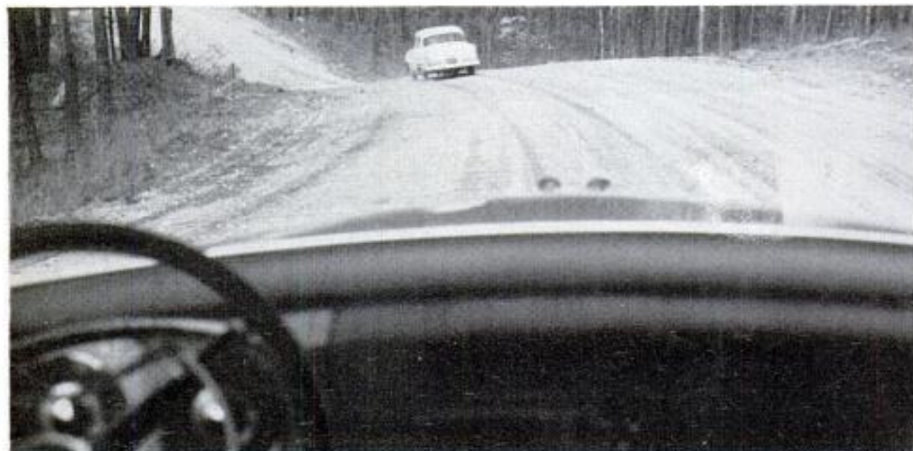
Driver's view of the endurance road. Test cars go around the rugged gravel circuit for thousands of miles
