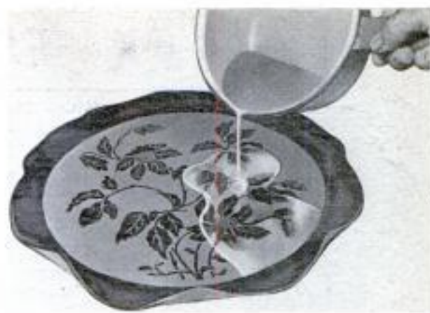
After disk is blocked out with varnish and fluted, etching acid is poured over design to \frac{1}{8} -in. depth
