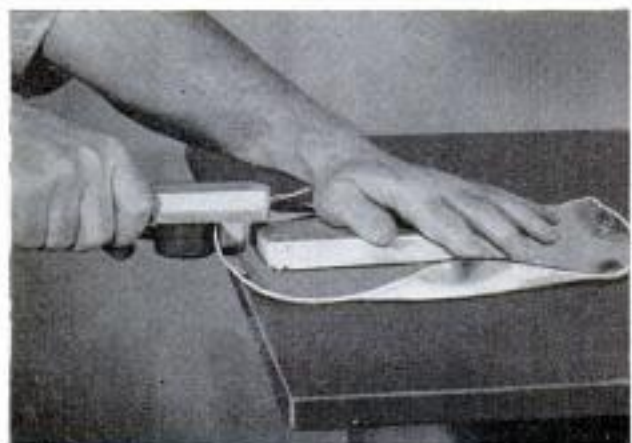
Fluting tool detailed at the right is shown in use in photos above and below. Note how sheet-metal disk is held flat with wooden block while flute is bent
