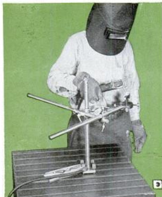
Upright leveling fixture combines with two horizontal arms to hold small work. Below, ring clamp with horizontal arm holds short round stock securely
