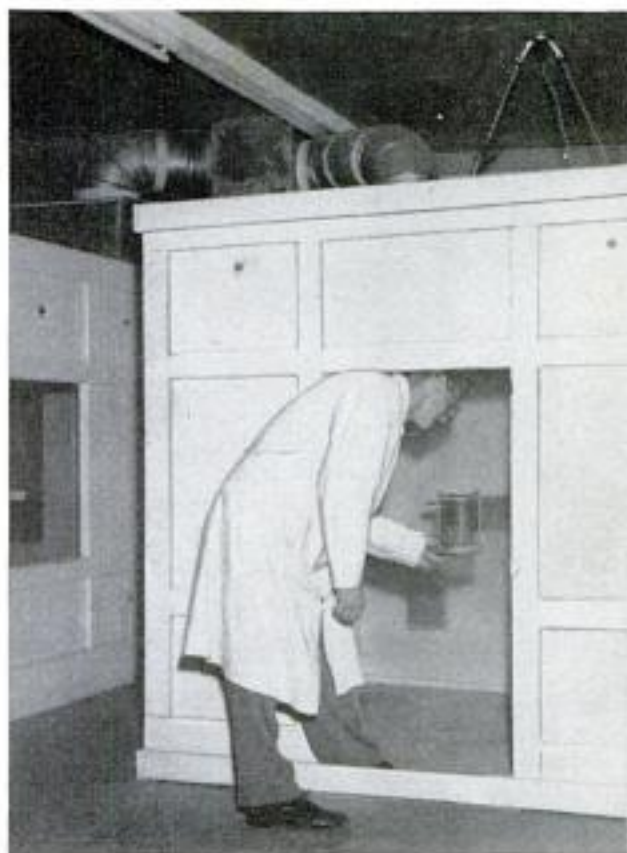
Cage of flies is placed on turntable in test chamber. Table rotates as insecticide is sprayed into the box
