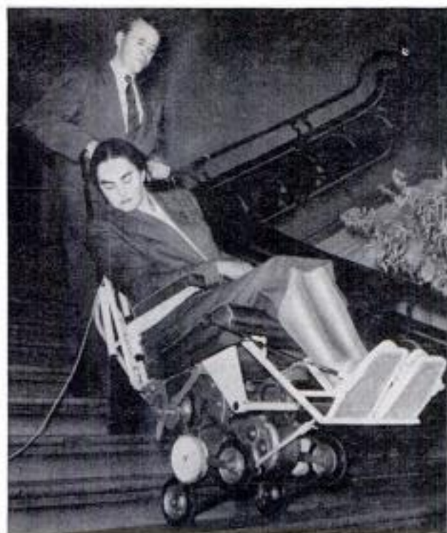
Electric chair is designed specifically for going up and down stairs. Attendant is needed to steady it
