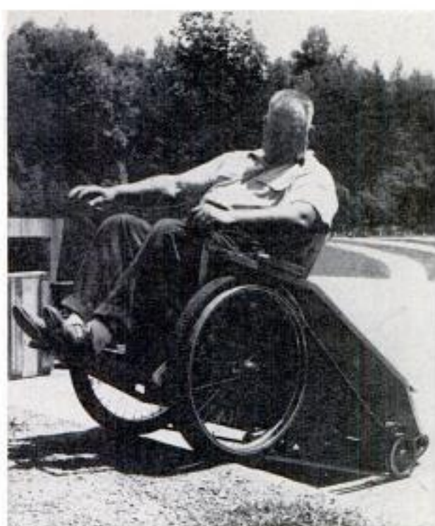
Curb-stepping wheel chair easily climbs over small obstructions when center tail wheel is retracted
