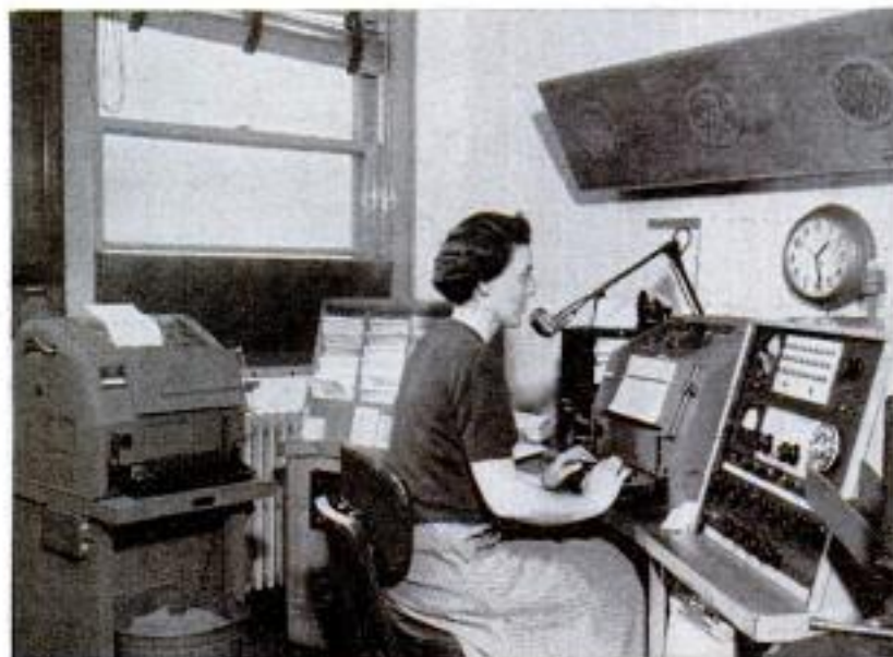
Incoming reports are copied on a teletypewriter for relay to other points. Right, center dial controls primary power to "slave" stations
