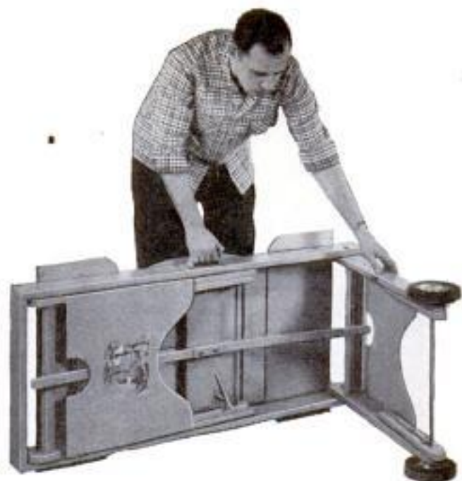
Photos above show the steps in folding the portable wooden barbecue. First, windbreak is folded down and leaves are folded over windbreak, elbow cabinet catches holding them in place. Then the legs are folded, as above, with barbecue resting on its side
