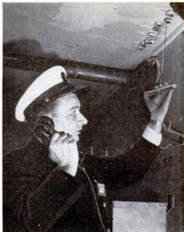
Instructor pulls cable, exposing sample any amount. As the decontamination proceeds, he lowers samples
