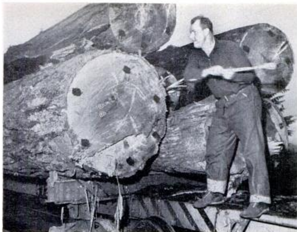
Log is branded with a blow from heavy hammer that is faced with company symbol
