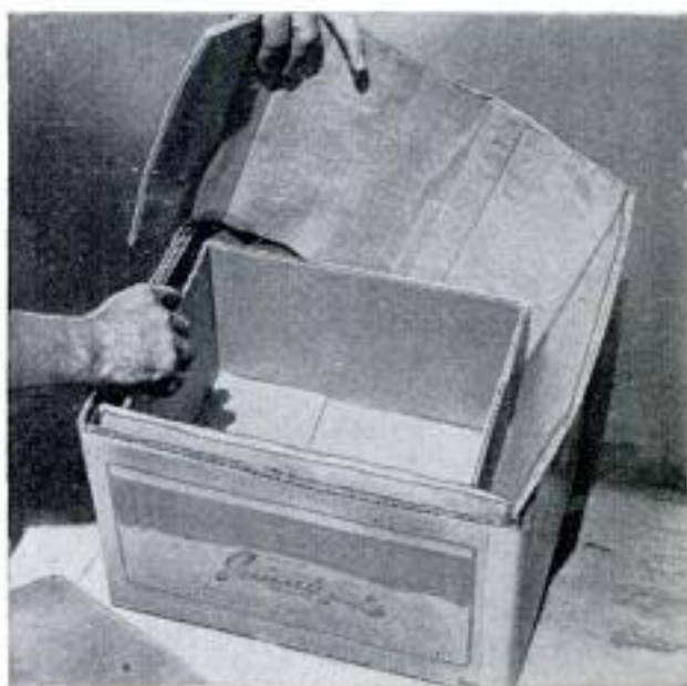
Cardboard from cut-up box is inserted between inner and outer cartons, above, to act as insulation
