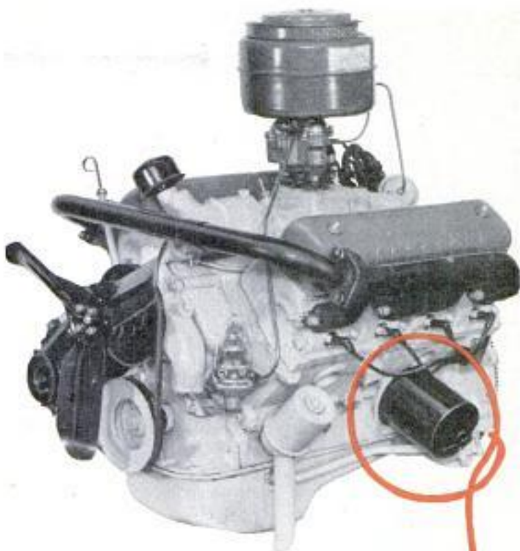
Owners praise the new Ford engine with its overhead valves and high-turbulence combustion chambers. But there were some complaints about the location of the oil filter (in the circle above) and the distributor
