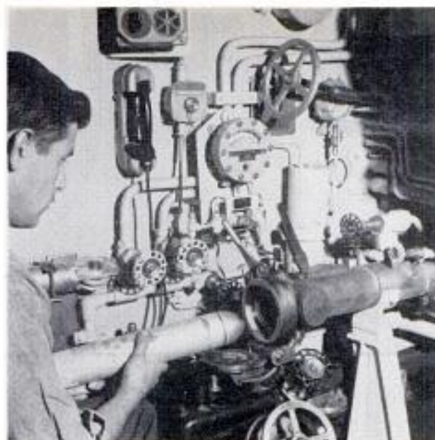
Signal flare projectile goes into ejector. Chief Ott, right, regulates ballast and closes hatches with hydraulics
