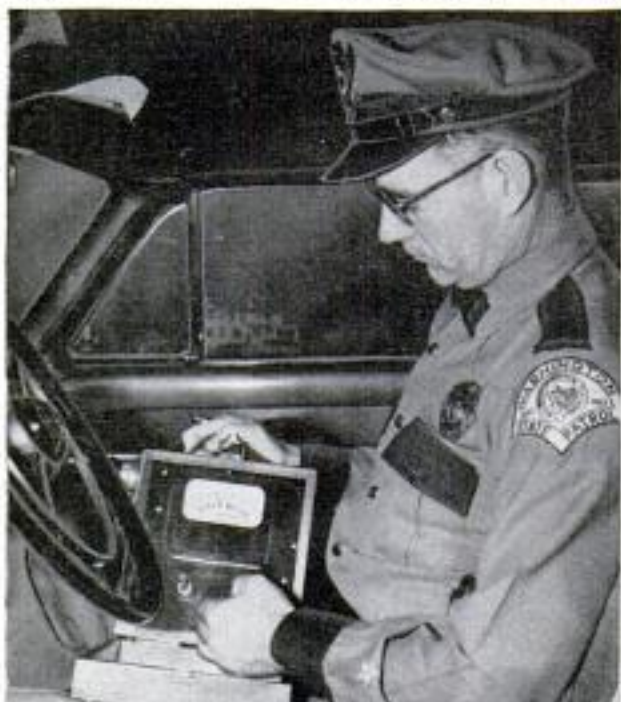
Speedometer of the radar unit gives the speed of approaching cars. A second car picks up violators
