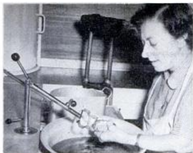
Clamp acts as the "hand" holding a potato peeler
