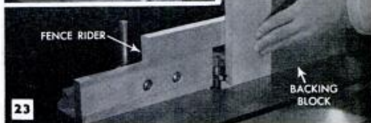
When the molding cut must run across the grain and on the face of the stock, use the setup pictured above. The setup shown at the left is permissible only on stock wider than 6 in.
