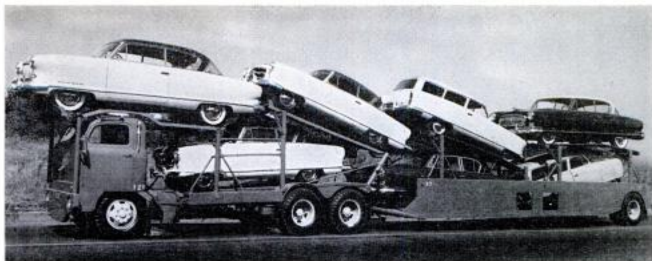
Auto transport with engine between front and middle wheels carries seven cars instead of six. Relief driver, left, sleeps in recessed bunk between seats
