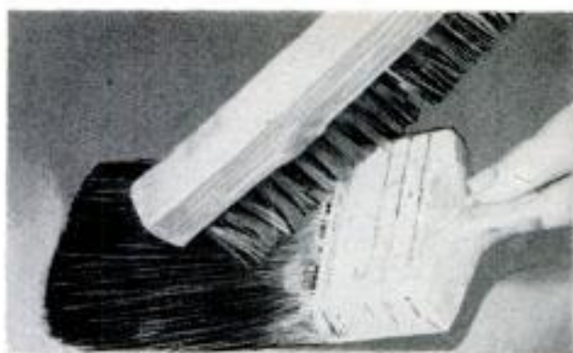
A wire brush can be used to scrape dried paint from the handle, around the ferrule and from the heel. In stubborn cases, wire brush is used on bristles
