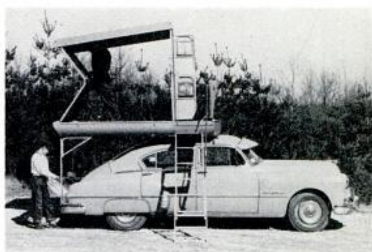
To set up cabin, you remove the ladder from its special storage compartment, climb up and raise roof by unfolding plywood ends.
