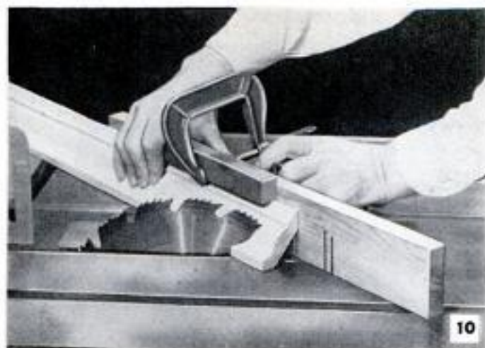
Moldings can be mitered and coped on power tools, using the circular saw for the miter cut and the bandsaw and simple jig for the cope cut
