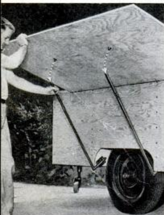
Below, bolt-head studs project from lids to engage ends of pipe supports
