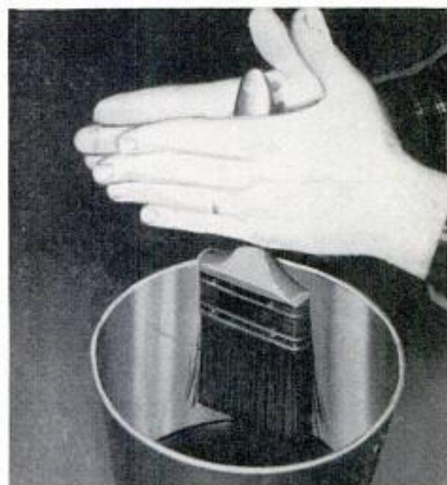
After soaking new brush in linseed oil for 24 hrs., it is spun dry by rolling rapidly between palms. Brush is held well down in empty pail for spinning
