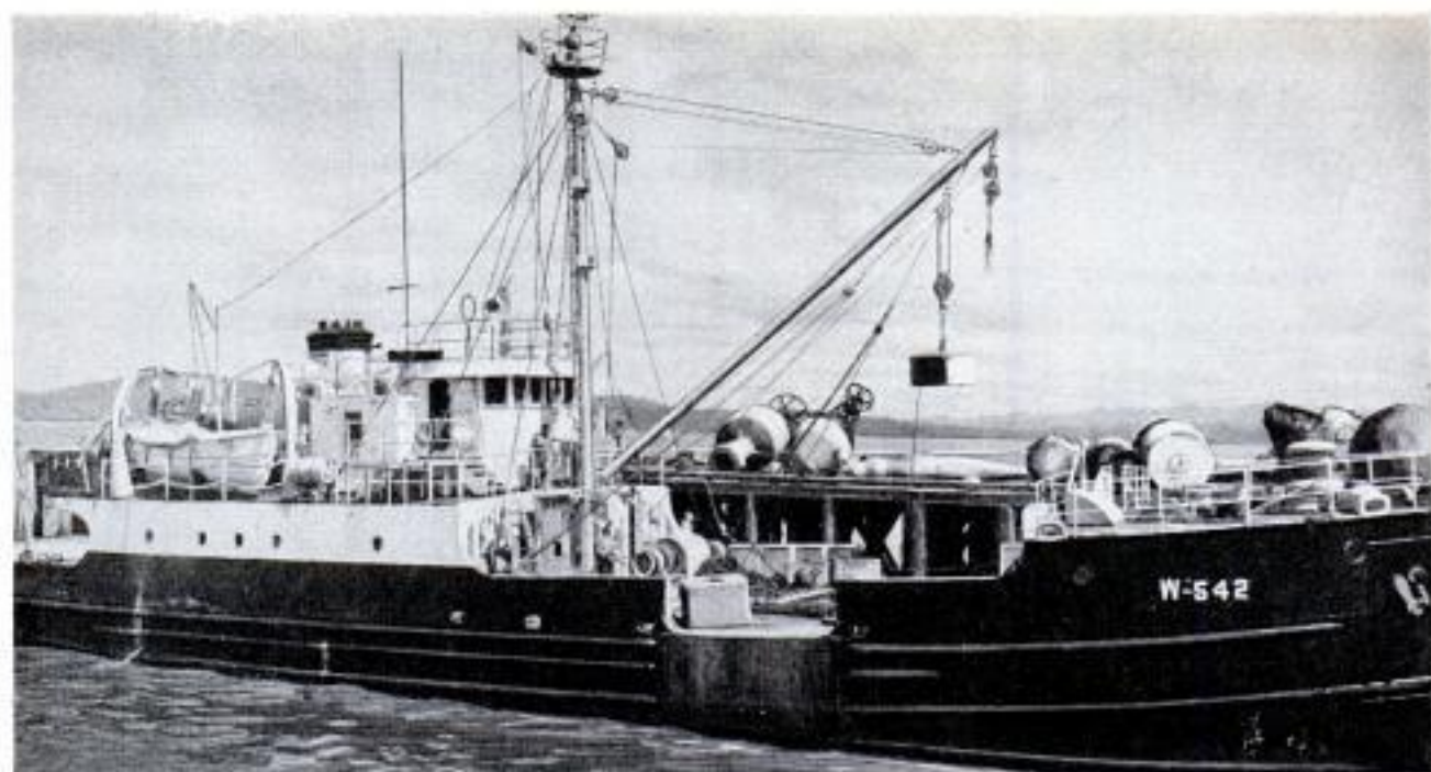
Nine-ton concrete block used in anchoring huge buoys is loaded aboard one of the busy Coast Guard ships
