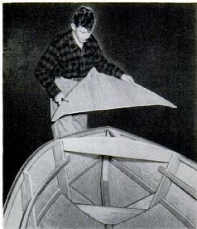
Alternate methods of cutting transom knees and finishing edge of plywood decking. Waterproof deck seam
