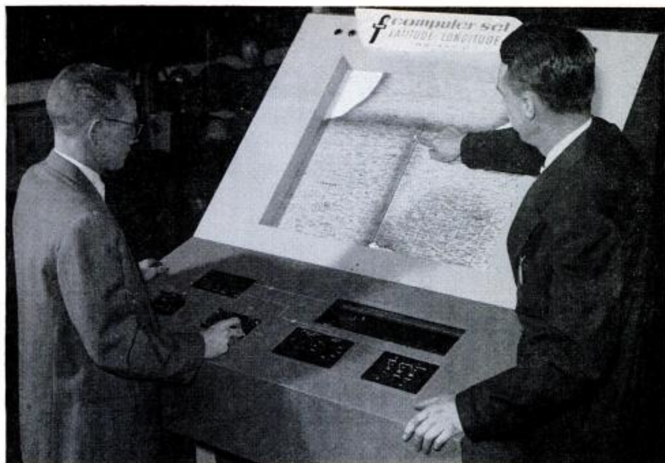
In display built to demonstrate robot navigator, white dot on map simulates aircraft it would be mounted in and its present position is indicated on bottom-left box. Only four boxes mounted on console are in the airplane
