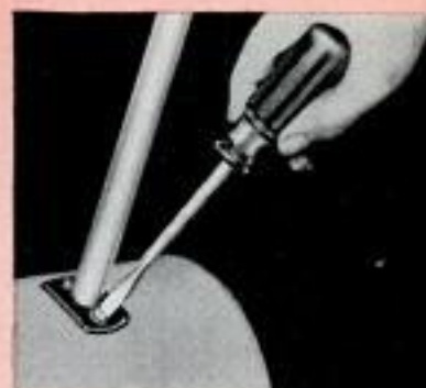
Photo at left shows completed lamp. Those above picture how drapery rod serves as adjustable column. In center photo lower end of rod is being attached to wooden base
