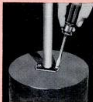
Photo at left shows completed lamp. Those above picture how drapery rod serves as adjustable column. In center photo lower end of rod is being attached to wooden base
