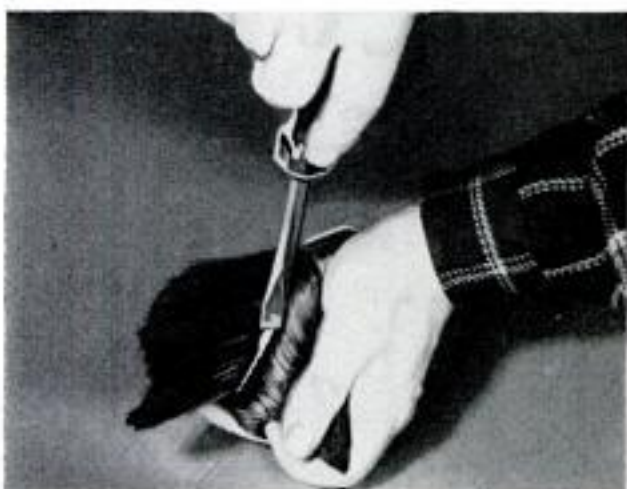
Before storing a paintbrush for a long period, separate bristles as shown above and clean paint from the well with a screwdriver or narrow putty knife
