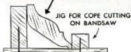
Moldings can be mitered and coped on power tools, using the circular saw for the miter cut and the bandsaw and simple jig for the cope cut
