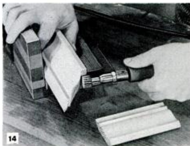
Some workmen prefer to undercut the cope with a rotary file, or burr, driven by means of a hand grinder
