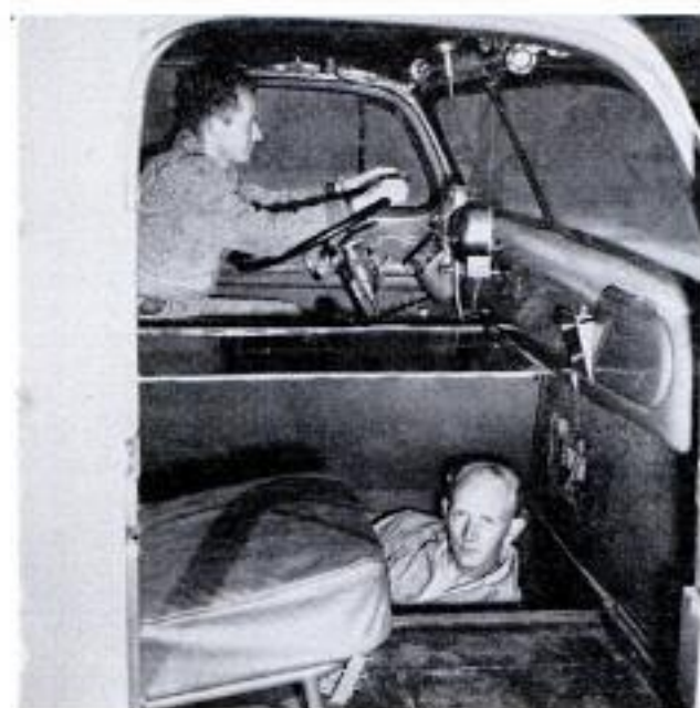
Auto transport with engine between front and middle wheels carries seven cars instead of six. Relief driver, left, sleeps in recessed bunk between seats
