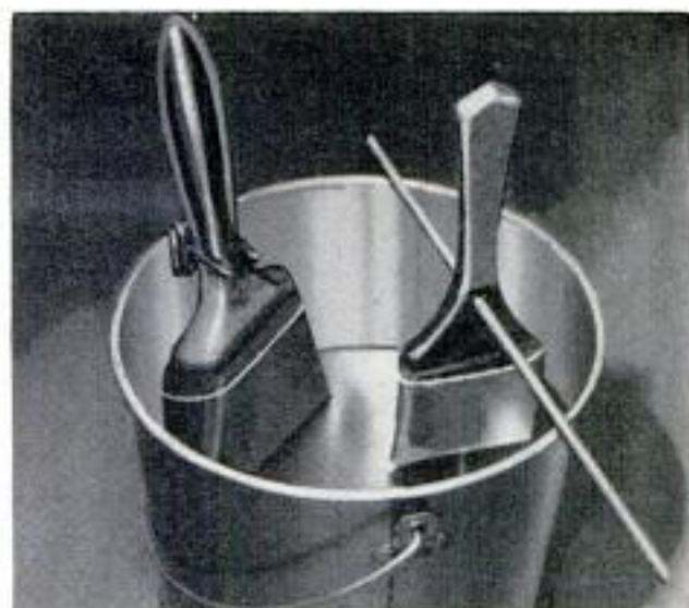
Above, two methods of suspending brushes in solvent. Brushes should not be allowed to rest on bottom of can, as resulting curled bristles cannot be straightened
