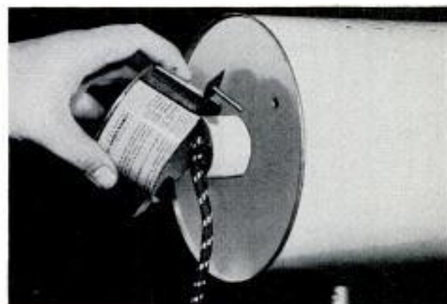
Lower left, No. 1 photoflood bulb gives ample light without excessive heat. Lower right, a hole about 3 in. in dia. in can lid gives fairly sharp spot. Can lid is removed when lamp is used for floodlighting
