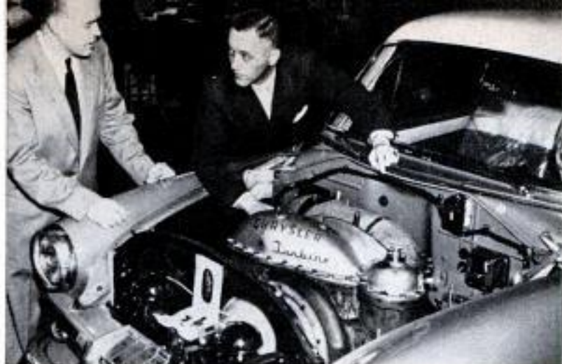
Fitting neatly under the hood of a Plymouth, the turbine is simple, has a fifth as many parts as a piston engine
