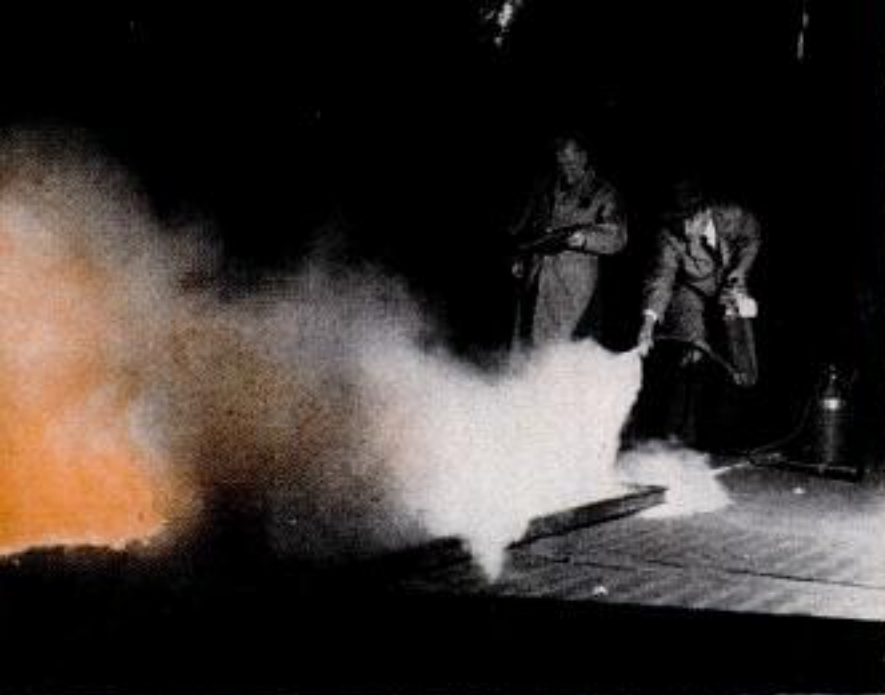
Underwriters' Laboratories photos Underwriters' experts test dry-chemical extinguisher in lab
