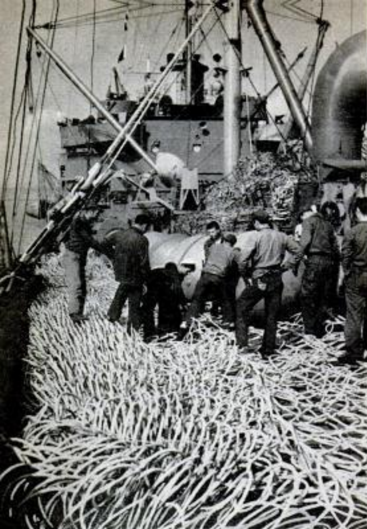
Mass of steel rings is a harbor net strong enough to stop a torpedo. It's made of \frac{1}{4} -inch steel wire
