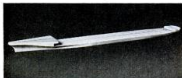
How hull looks when carved according to templates
