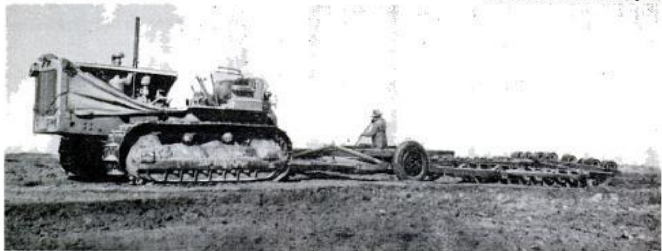
Huge wheatland plow is among the most effective weapons against sage. It cuts a swath of brush 30 feet wide U.S. Bureau of Reclamation photo
