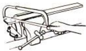
FRAME MEMBERS MITERED WITH HACKSAW
