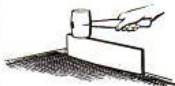
SPLINE DRIVEN IN GROOVE ANCHORS SCREEN WIRE
