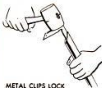
METAL CLIPS LOCK MITERED CORNERS
