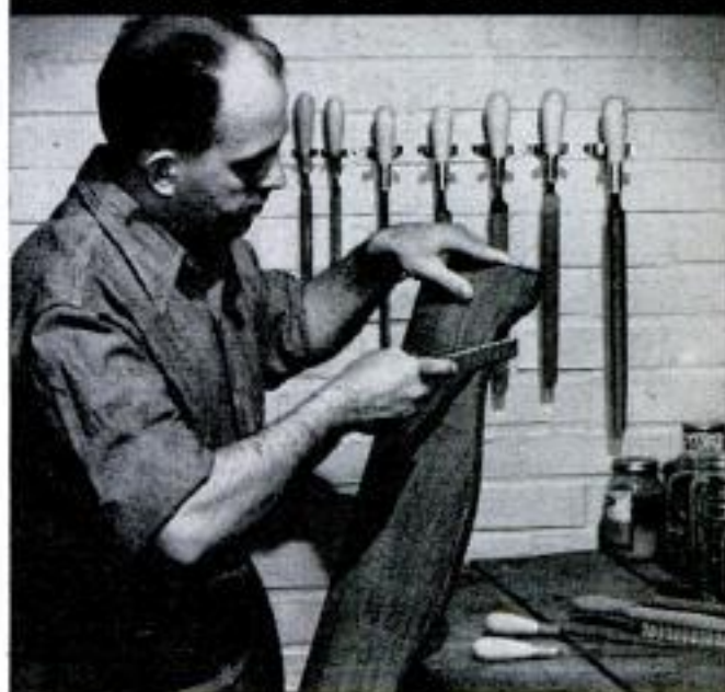
Flat file and rasp on one side; half round rasp and file on other side. (8", 9" or 10" length.)
