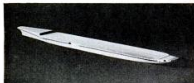
Stern view showing sponson piece in place on hull
