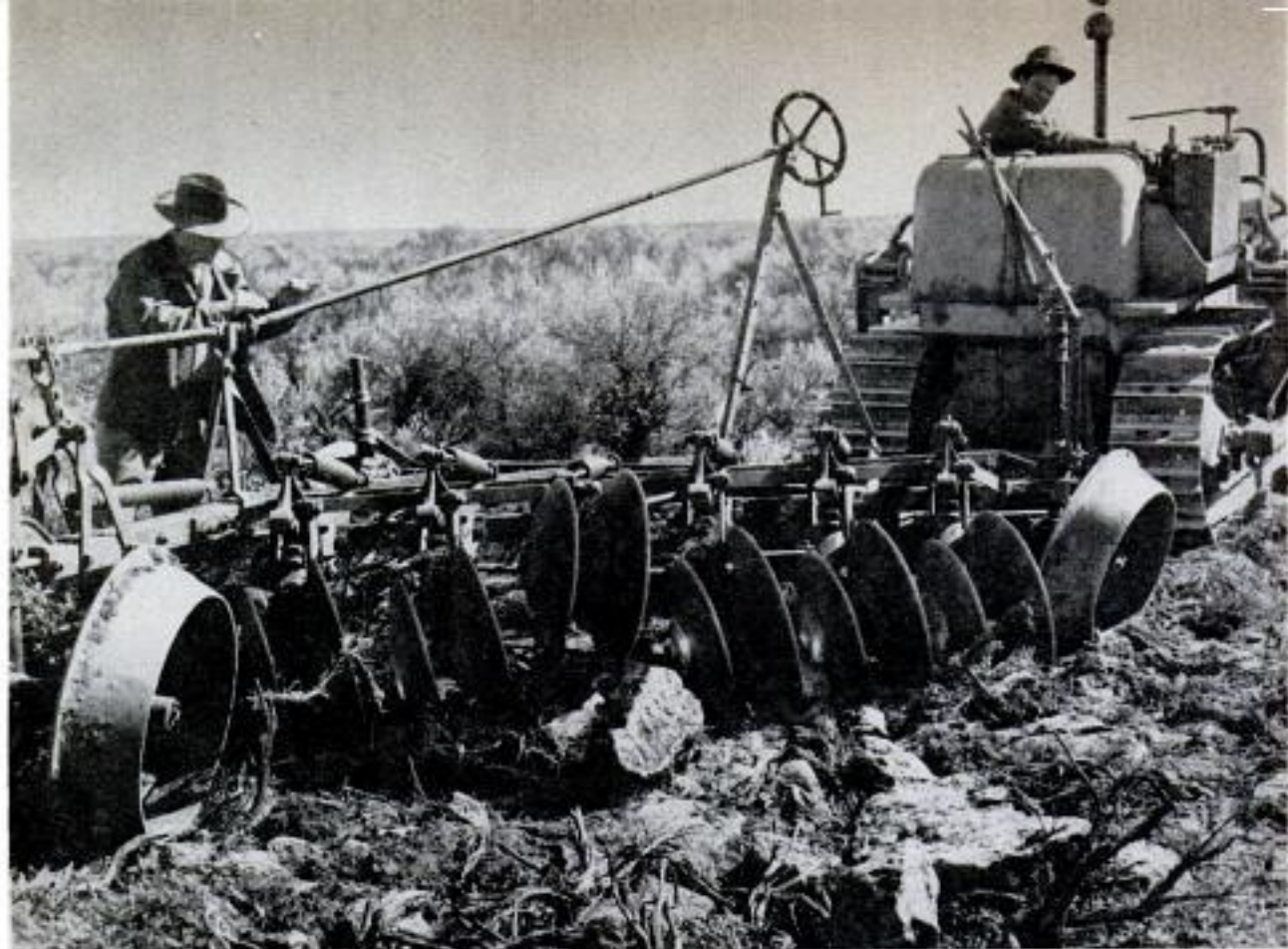
"Stump jumper" for "brush bustin'" has disks mounted in pairs. Each pair can ride right over a big rock
