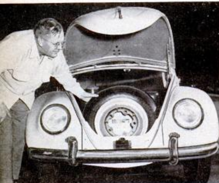
Spare tire, gas tank and some luggage space is under the hood of the VW. Below, the rear engine gives fine traction, Clymer reports, even on rough, sandy roads
