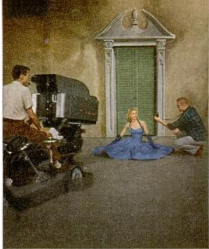
Engineer checks light prior to telecast. Poor lighting can turn blues to reds, give flesh a green tone
