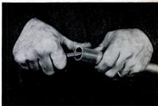
Burrs can be removed from edges of tubing with pocketknife, above. Aluminum sheet is bored with expansive wood bit, as below
