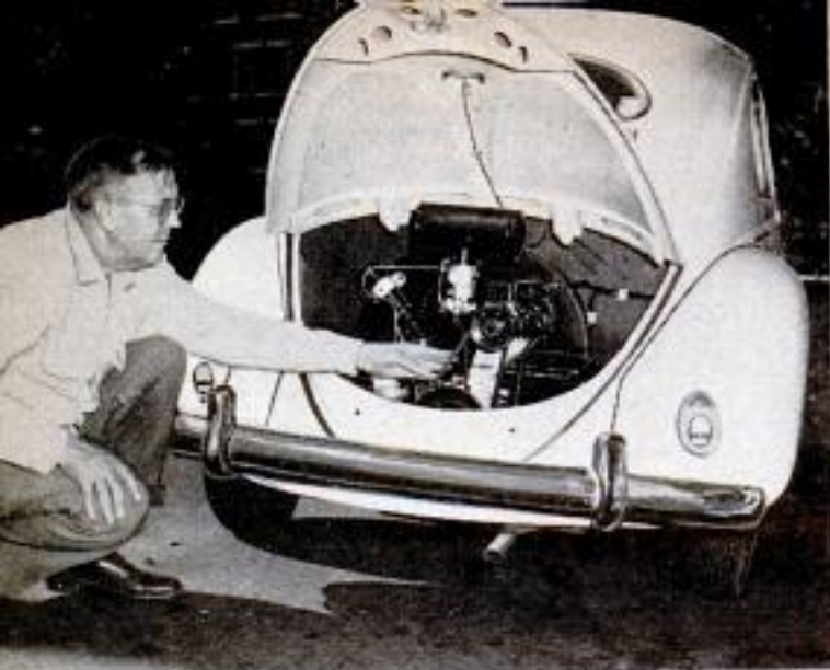
Clymer points to the belt that drives the cooling fan of the rear-engine, air-cooled Volkswagen he tested
