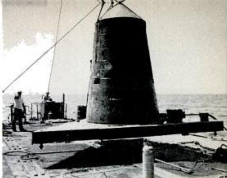
"Heralds," like this one, are placed in row at bottom of harbor entrance and are actually sonar instruments. Their "pings" are monitored at control post
