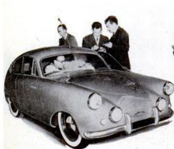
With a body of lightweight plastic, the Morocco-built Reac has won several North African races. Roof and windows can be detached from the body to convert it into a roadster
