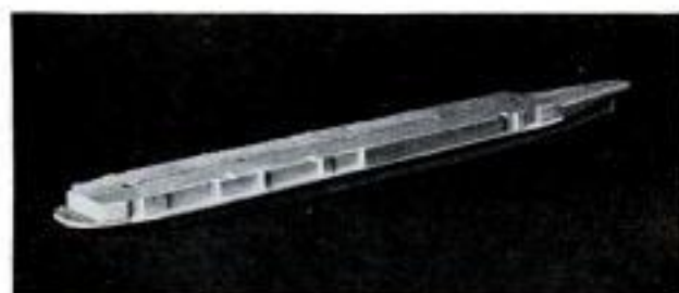
Above, underside view (looking aft) showing overhanging sponson. Below, starboard view shows sponson topped with notched piece. Cover board fits on top
