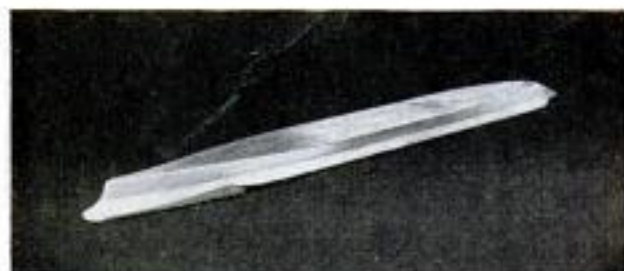
Above, underside view (looking aft) showing overhanging sponson. Below, starboard view shows sponson topped with notched piece. Cover board fits on top
