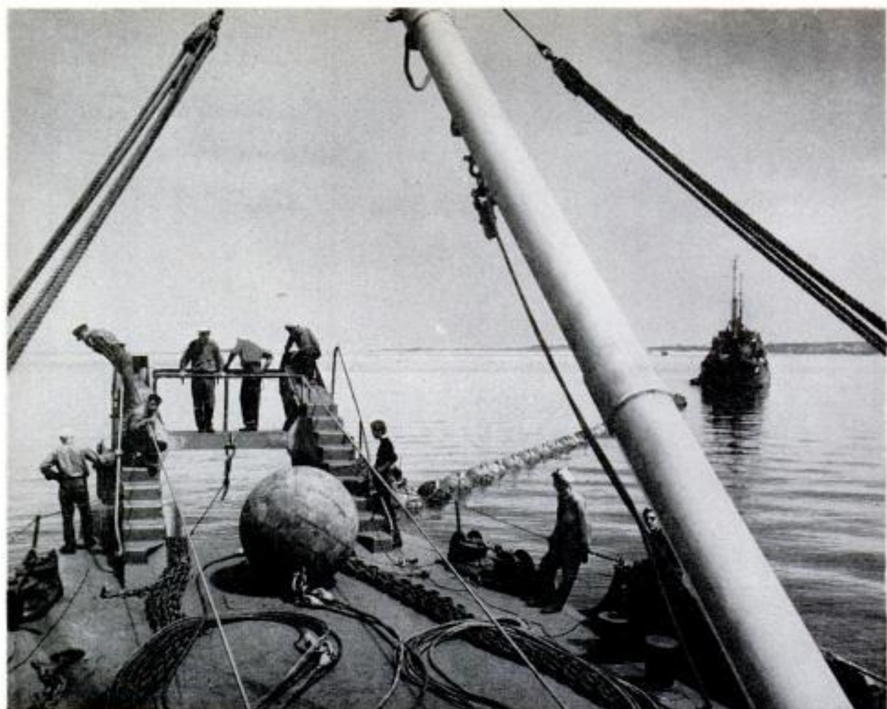
Net tender drops buoys and nets into water while another vessel prepares to tow completed sections away
