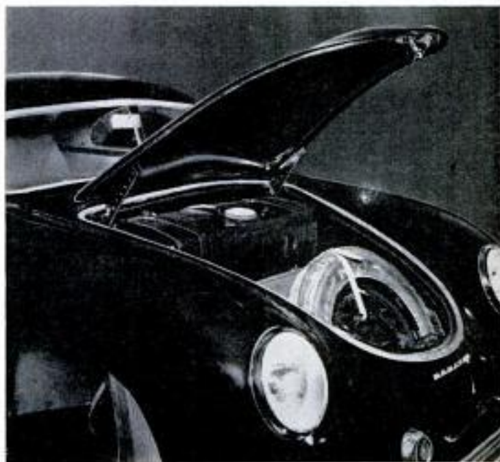
Four-cylinder, air-cooled Porsche engine fits neatly into the "trunk." It has two carburetors, gets expert factory tune up. In front is spare tire, gas tank and little luggage space
