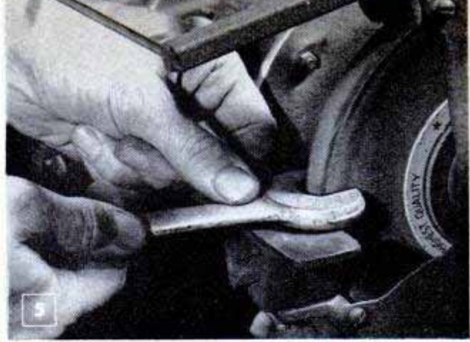
Wrenches with badly damaged jaw faces can be made serviceable again by grinding the jaws so that the spacing between them is equal to the next nut size
