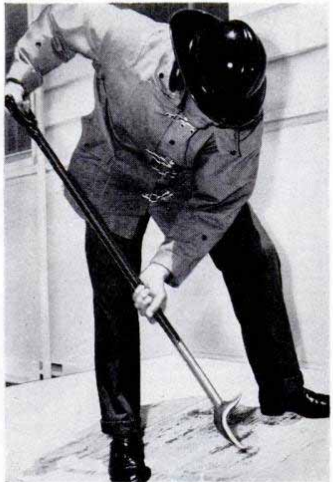
Tin-roof opener works on the same principle as the familiar can opener; just jab it in and rock along
