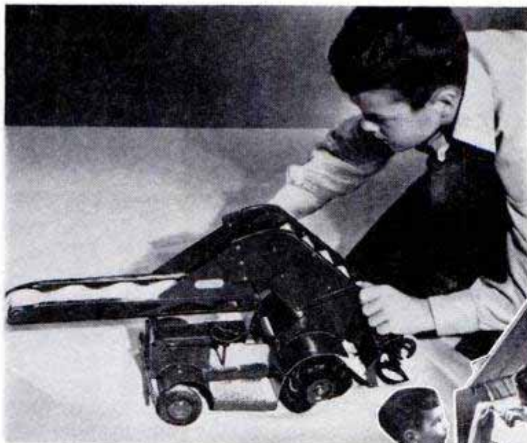
BUCKET LOADER scoops up sand or gravel and puts it in an earth hauler. A crank operates the loading screw, sand buckets, and the rubber conveyor belt
