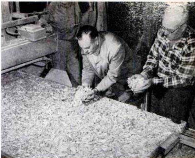
Machine at left feeds cedar chips treated with plastic into moving tray. In the press, tray serves as form for finished panel
