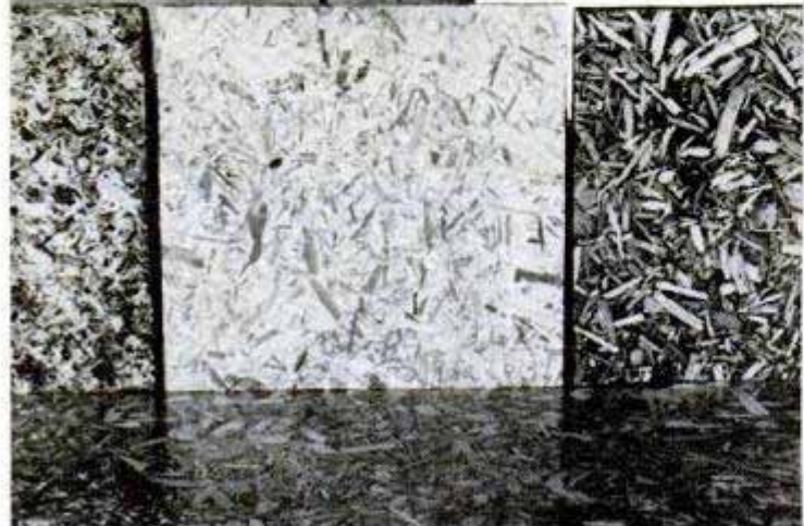
Samples, left, contain cotton stalks (top) and bolts, cedar chips with white and colored putty
