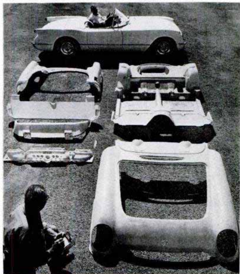
Right, major plastic parts of Corvette. Only metal body part is gas-tank flap
