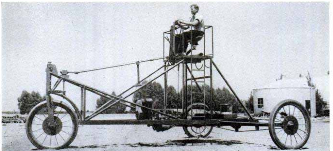
↑Huge spiked wheels are forced into ground to pick up sugar beets and deposit them in a bin. Below, from high perch of this strange machine, operator spots and flame-kills patches of dodder in alfalfa fields
