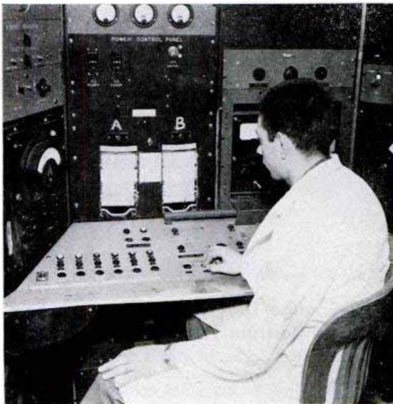
Technician at control board can increase or decrease activity of pile by movement of shields. Test samples are analyzed by recording activity of pile before and after samples are lowered
