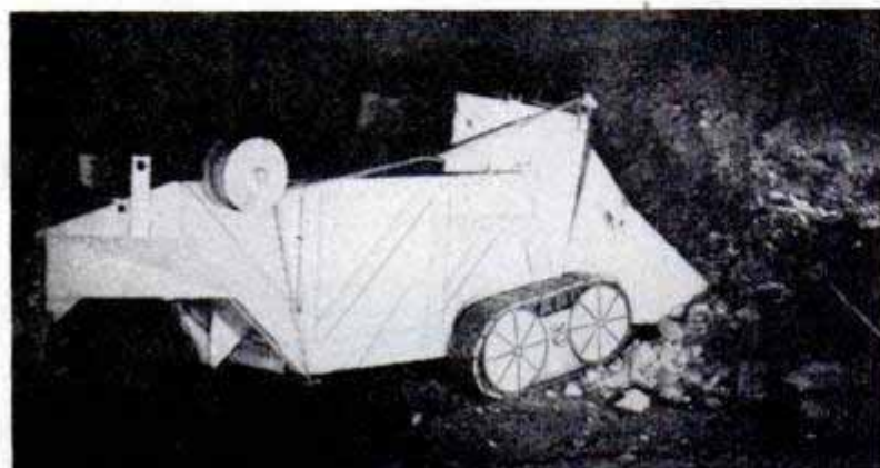
Boom containing rock-drilling equipment is mounted in minutes. [With boom removed, machine scoops up rock, hauls it away
