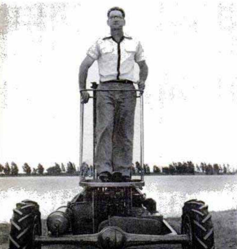
"Steel squirrel" is a self-propelled perch for orchard workers. Below, it's small enough to move easily between trees. Operator guides it by foot and hand controls, has compressed air at hand for pneumatic tools
