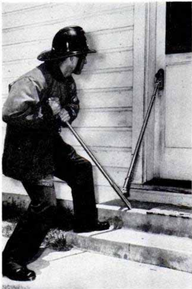
Lever action gives this door opener plenty of the necessary squeeze, far exceeding strength of a man
