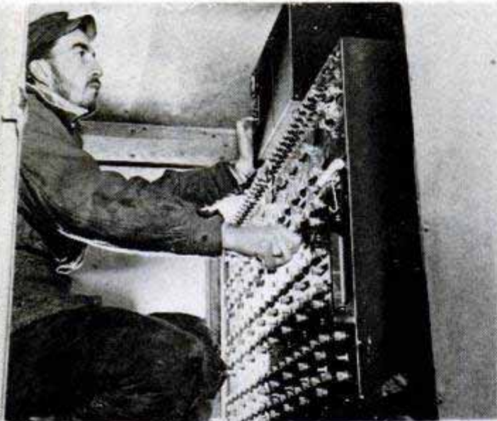
Seismic observer operates a complicated instrument panel inside truck. He determines placement of the dynamite, decides whether a re-shoot is necessary
