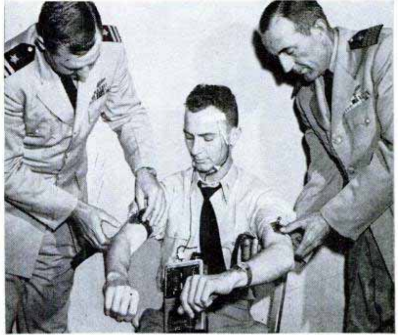
Before a bank of receiving instruments, a technician examines inked graph of pilot's reactions. Beside him is an oscilloscope. At right, doctors tape electrodes to pilot's body. In pilot's lap is relay box. Below, human centrifuge previously used to test reactions of pilot under conditions similar to those of actual flight
