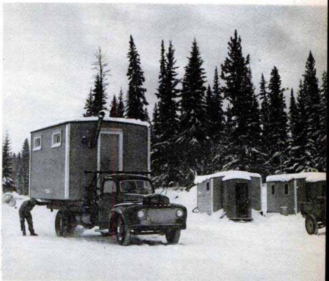
Surveyors who plot the shot holes and Geophone locations have to wade through knee-deep, sometimes hip-deep snow. Below, when it's time to move camp, trucks or bulldozers haul the skid-mounted trailer houses to a new area
