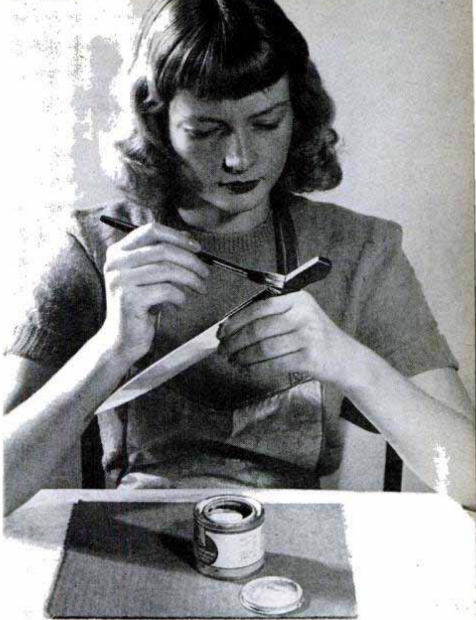
PAINTING THE TOP OF KNIFE HANDLE tells you at glance which edge of blade is the cutting edge. This is especially helpful from a safety standpoint when edges of the blade are curved similarly
