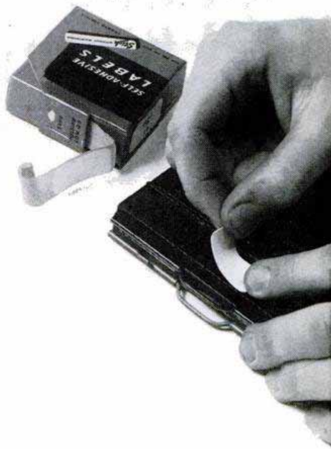
Above, notch patterns filed in edge of holder flap expose film, reproducing pattern as in the inset. Below, numbered holders aid in recording data
