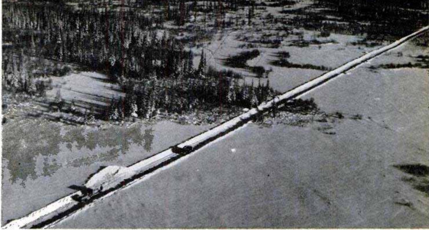
Main street in exploration area is road plowed by bulldozer. Oilmen have cut thousands of miles of such roads
