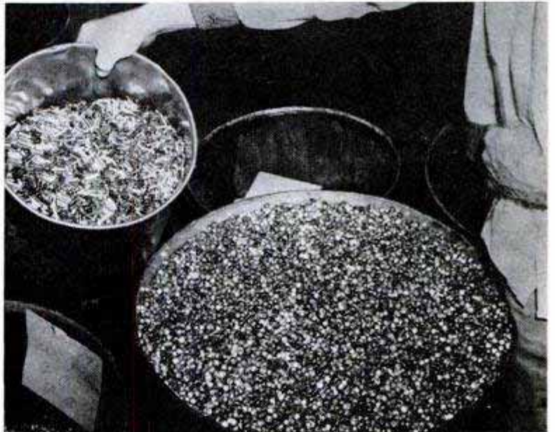
More than 300,000 cups in the large barrel will go through successive drawing operations to shape them to the exact jacket size of those in bucket. Below, precision tools are a necessity. Here a superaccurate die is ground automatically
