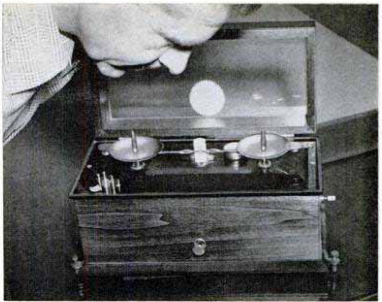
Superaccurate, .30-caliber bullets must be uniform in weight. A bullet which varies more than a fifth of a grain is rejected
