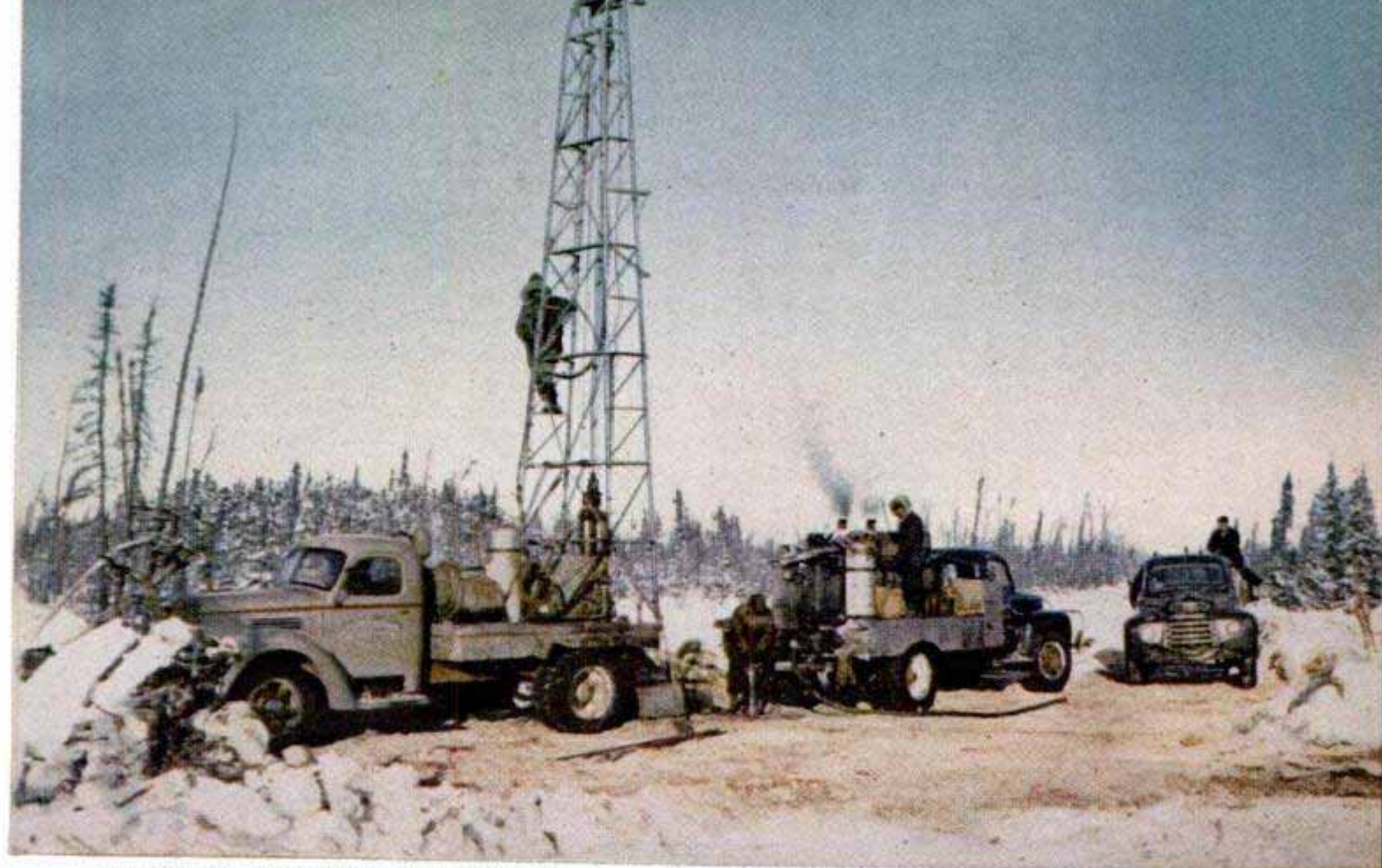
In bitter cold, crew drills hole for dynamite charge that will set off shock wave to map earth's subsurface
