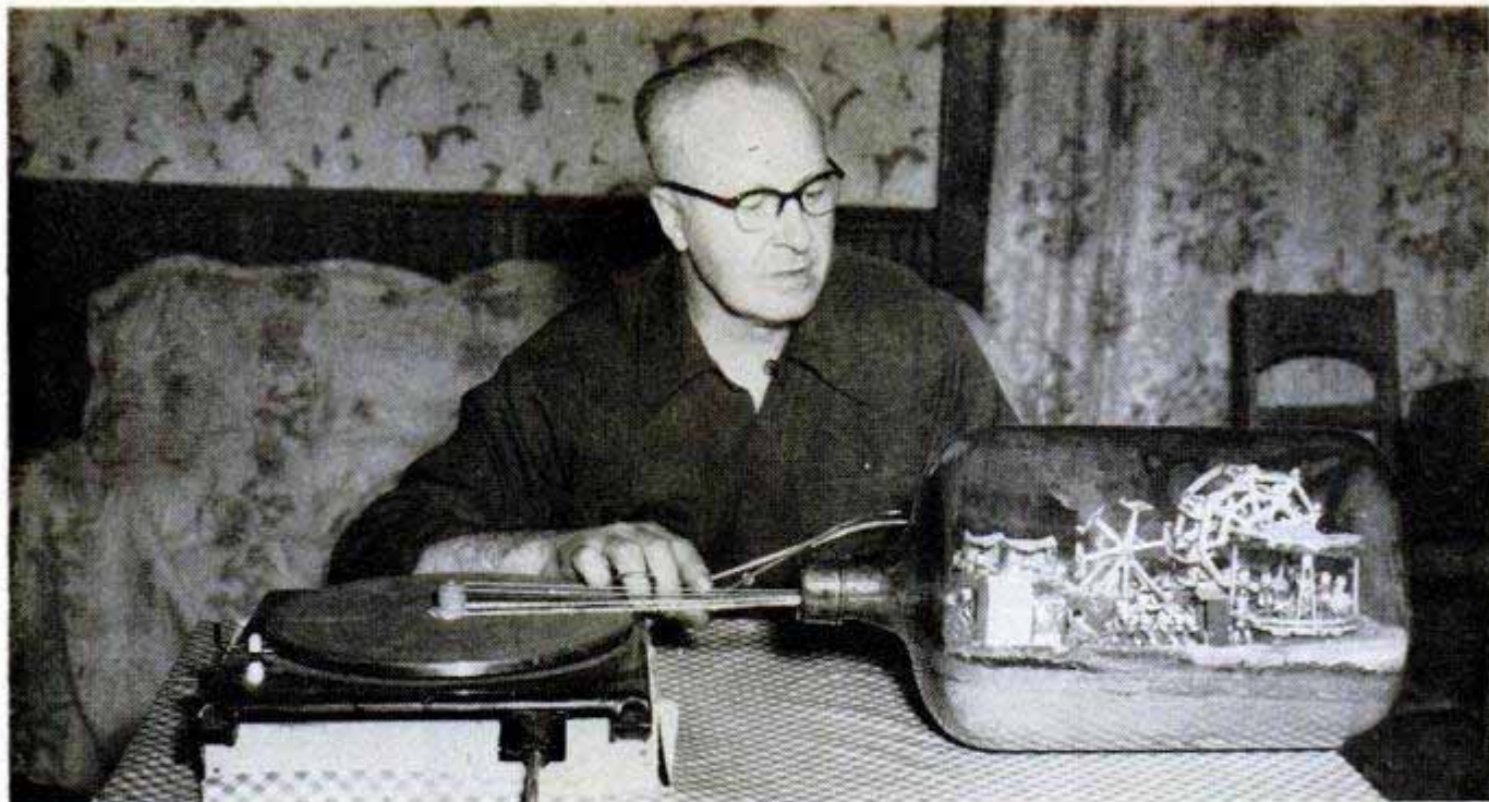
Braided strings looped around the phonograph turntable operate the carnival rides within the five-gallon jug
