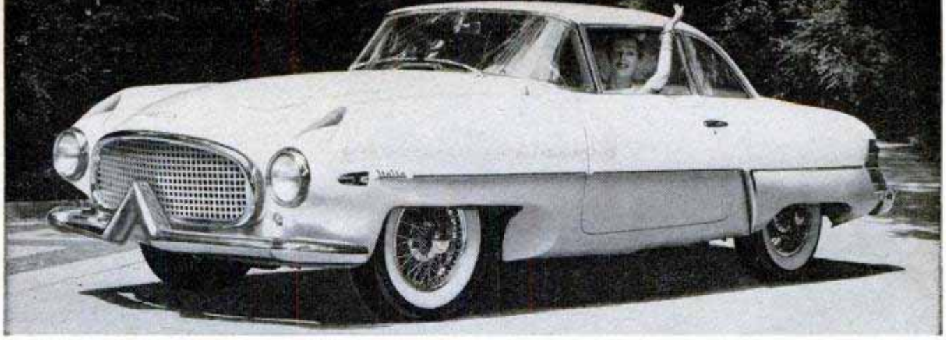
Ten inches lower than a standard Hudson, the Italia has a wrap-around windshield to give full forward vision
