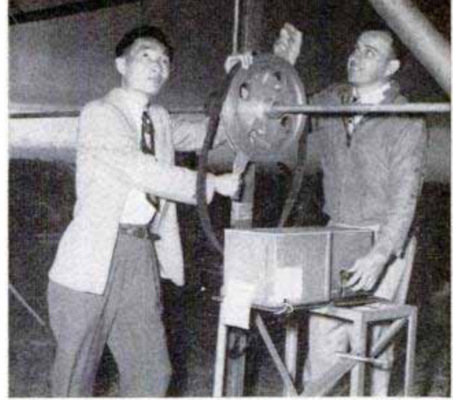
Declination of the telescope can be varied manually as shown here, or by motor controlled from trailer
