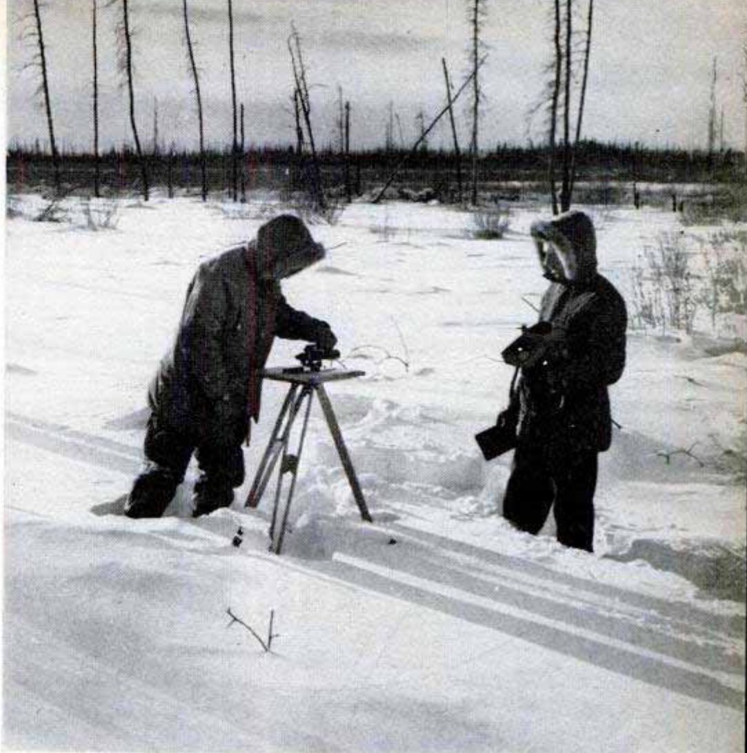
Surveyors who plot the shot holes and Geophone locations have to wade through knee-deep, sometimes hip-deep snow. Below, when it's time to move camp, trucks or bulldozers haul the skid-mounted trailer houses to a new area
