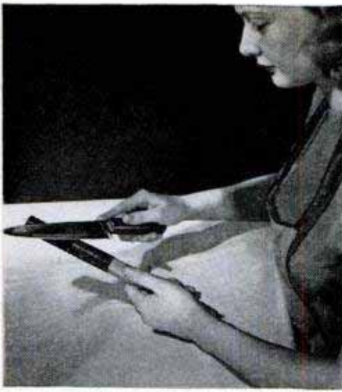
KNIVES may be honed on dowel wrapped with piece of 2/0 emery cloth
