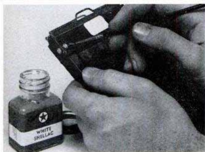
Above, notch patterns filed in edge of holder flap expose film, reproducing pattern as in the inset. Below, numbered holders aid in recording data
