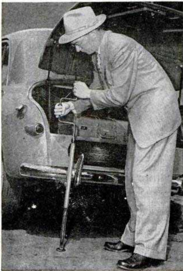
Safe and slipproof is the Minx jack. The arm on the jack slips into a socket welded just under the bumper
