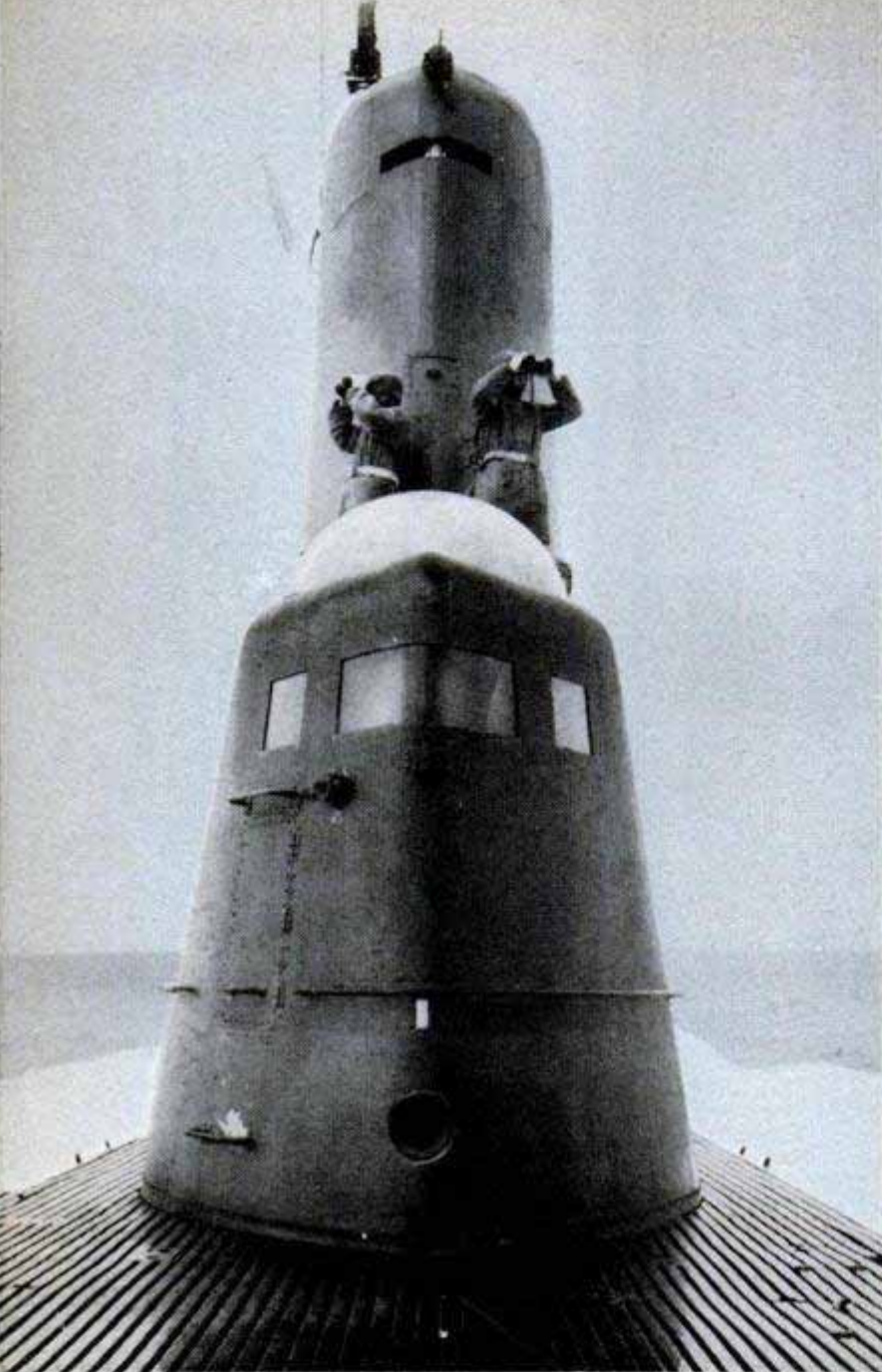
When sub surfaces, lookouts scramble up to their stations beside "sail." Snorkel subs seldom need to surface completely
