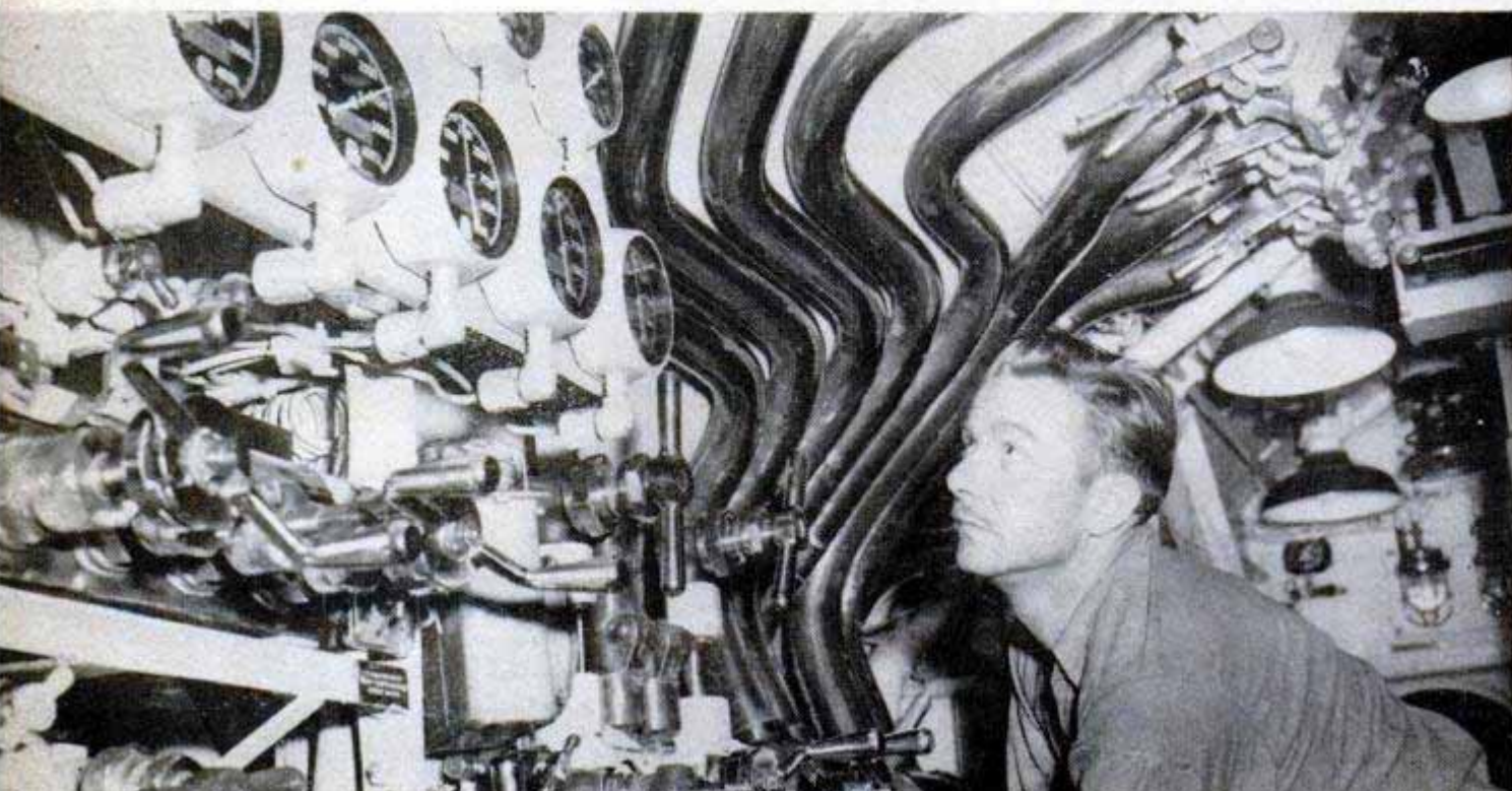
Submarine is literally jammed with equipment. Here the air manifold operator prepares to blow ballast tanks
