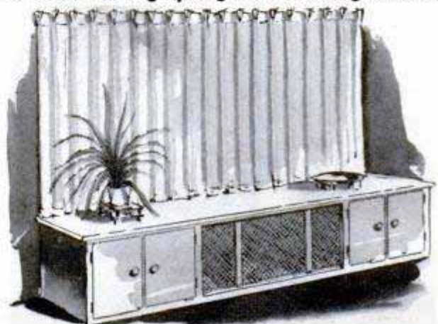
Unightly radiators under wide windows can be hidden effectively, without impairing efficiency, by means of a built-in having open grille and storage cabinets
