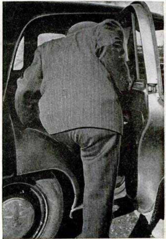
Getting in and out of the rear seat takes practice. The door opening is small and the wheel interferes
