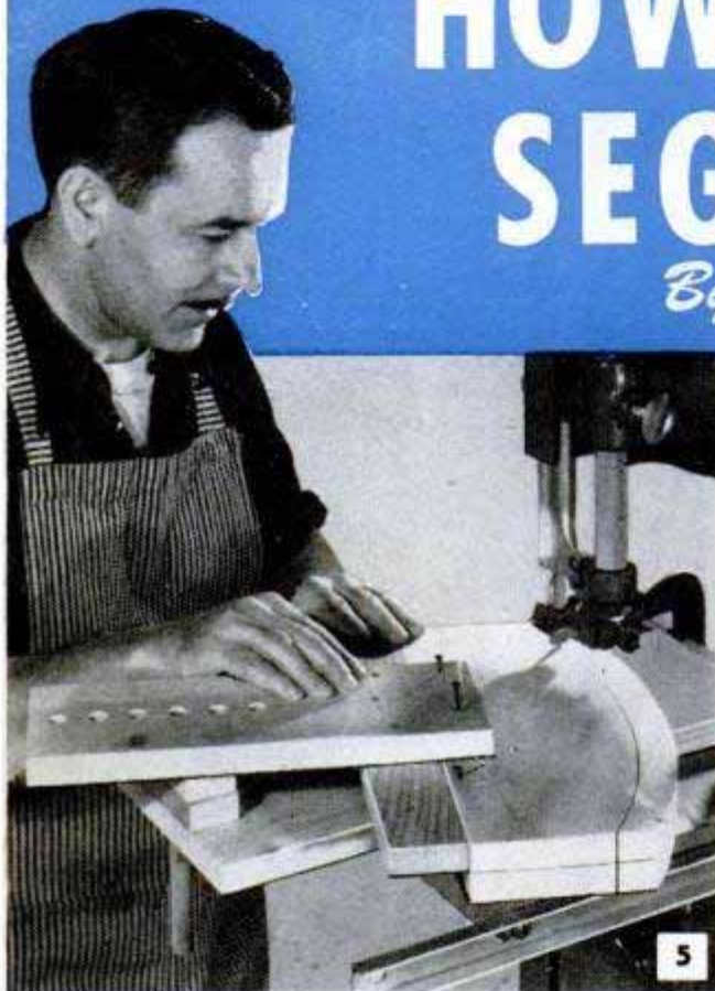
Above, setup for cutting curved segments in two thicknesses of stock. Be sure bandsaw blade is sharp and properly set. Below, an example of the polygonal form is six-sided table built with straight segments
