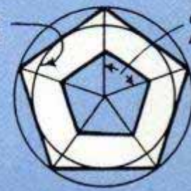
5 SIDES — PENTAGON CENTER ANGLE—72° MITER—54° BEVEL—36° OUTSIDE CIRCLE—1.176 INSIDE CIRCLE—1.454
