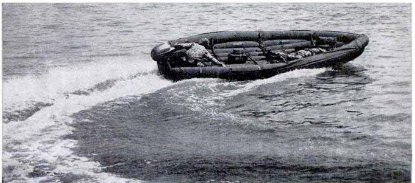
Carbon-dioxide cylinders inflate boat in 30 seconds
