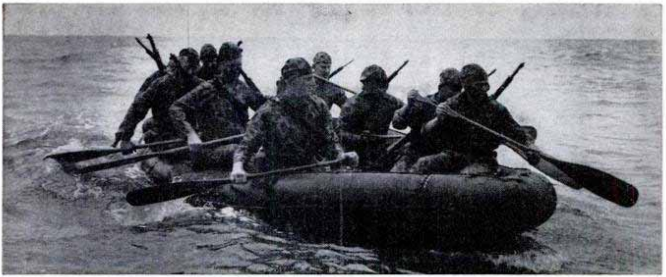
Raiding team cuts 25-hp. motor and switches to oars when close to shore. Large 2450-pound model carries nine
