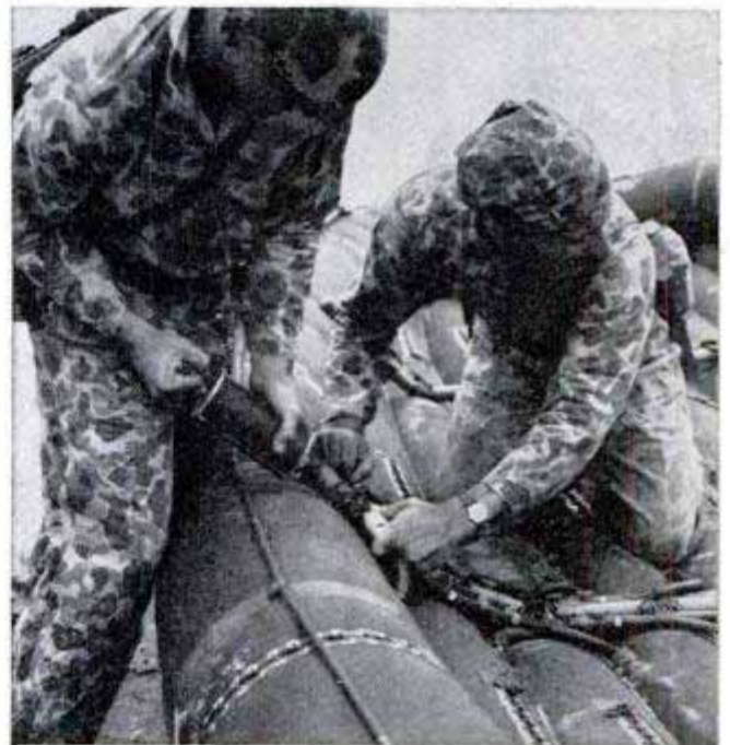
Carbon-dioxide cylinders inflate boat in 30 seconds
