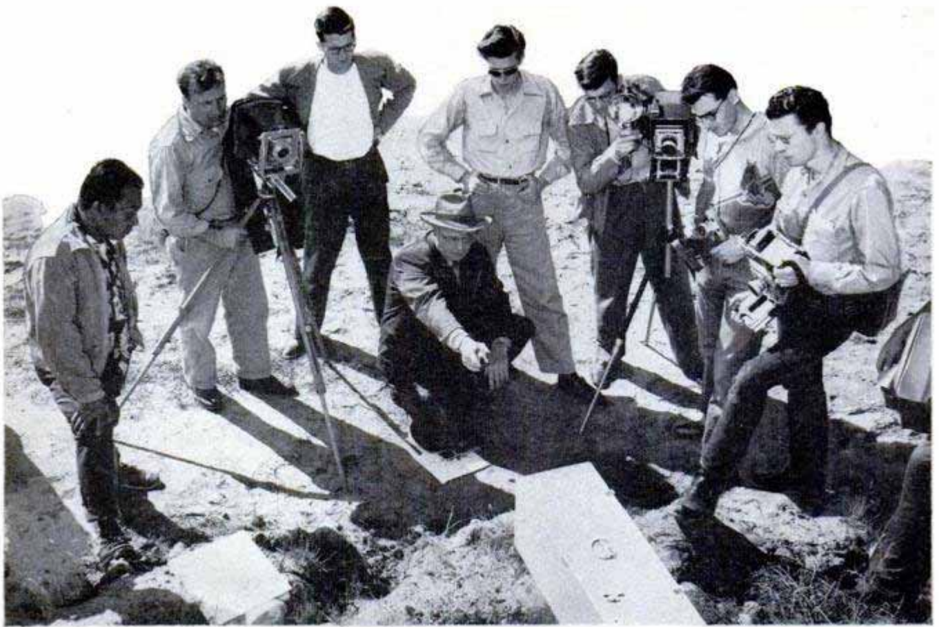
Bullets are fired into a recovery box and rifling marks photographed for matching with those of murder gun
