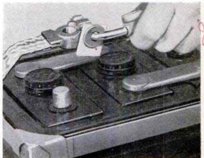
Many car owners equip ground cable with quick-acting clamp so that circuit can be opened in an emergency
