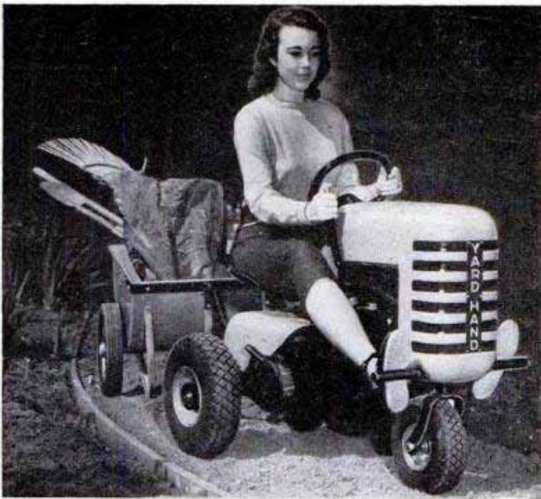
Taking the place of a wheelbarrow, above, the little tractor tows a cart full of tools down a garden walk. Width is 28½ inches. At right, it mounts a 10-inch circular saw and table
