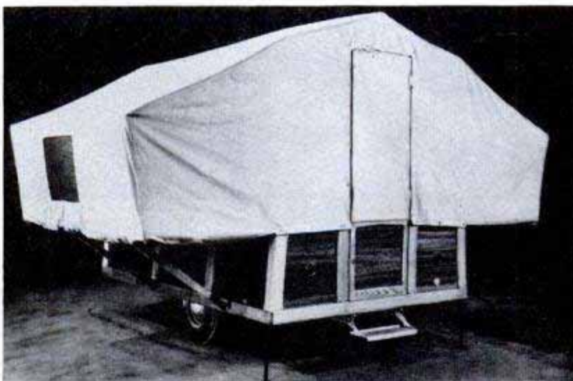
In extended position, the trailer is 7½ feet high in the center, 10 feet long and 12¾ feet wide. Screens cover the side openings
