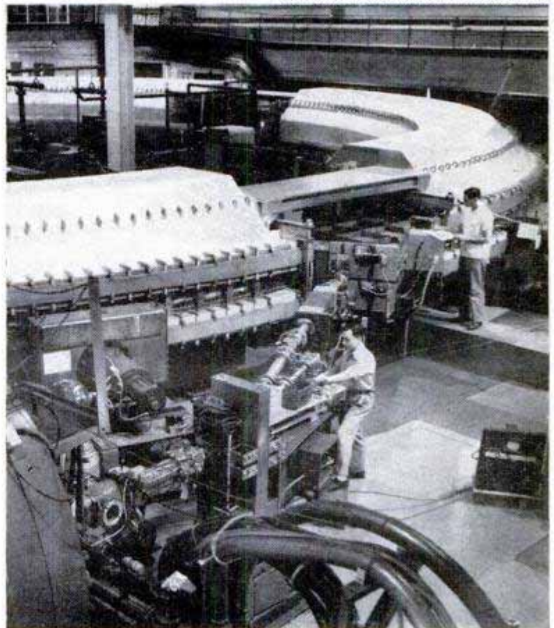
Protons shoot into cosmotron through equipment at lower left. Magnet forces them in circle so they can be given higher energy
