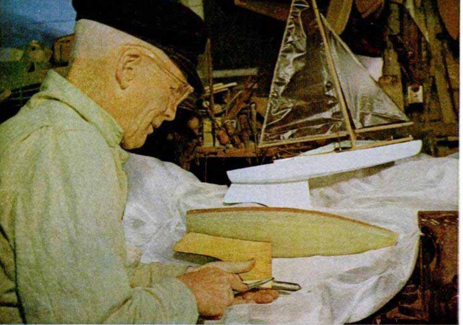
Lassal works on an experimental "finless fin" keel which improves sailing characteristics, making boat faster
