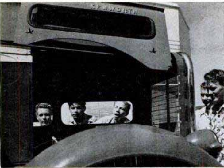
Special windows are provided for the curious. Turbojet takes only 13 percent of space required by diesel
