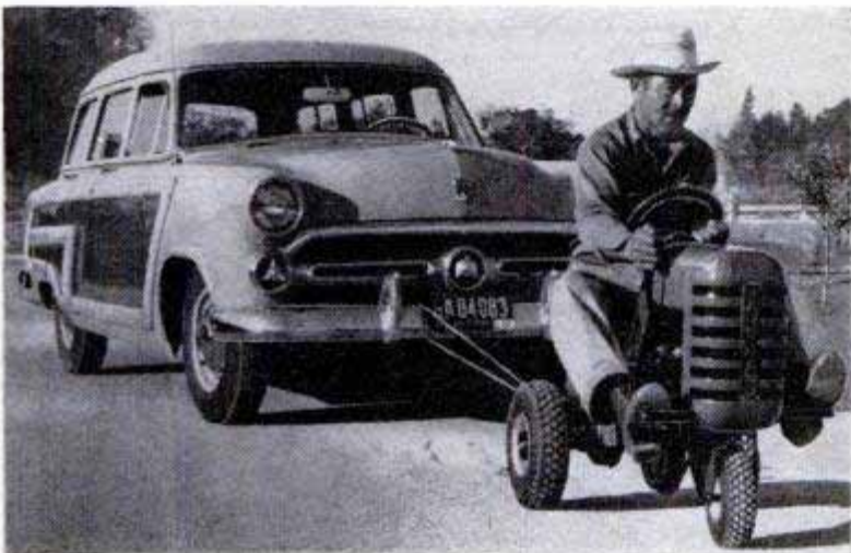
This isn't a gag shot. There's enough power in the midget to pull an automobile up a slight grade. Below, Hiller mows his lawn in comfort, towing a 20-inch mower and grass catcher. Fuel consumption for most yard work is one quart per hour
