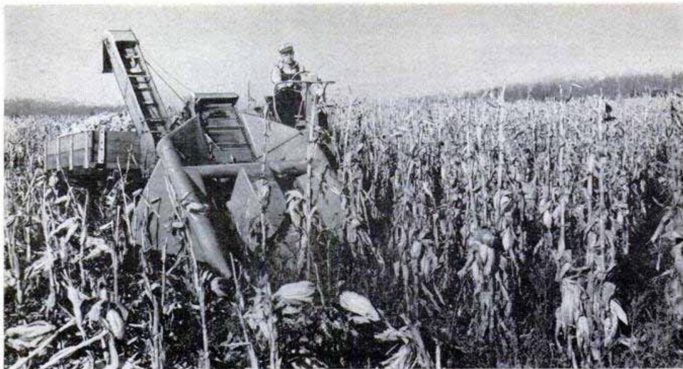
Operator, using corn picker and husker, has full view of the stalks from his vantage point high on the left side of the machine. There are ten 36-inch husking rolls, half of them made of rubber and half of iron
