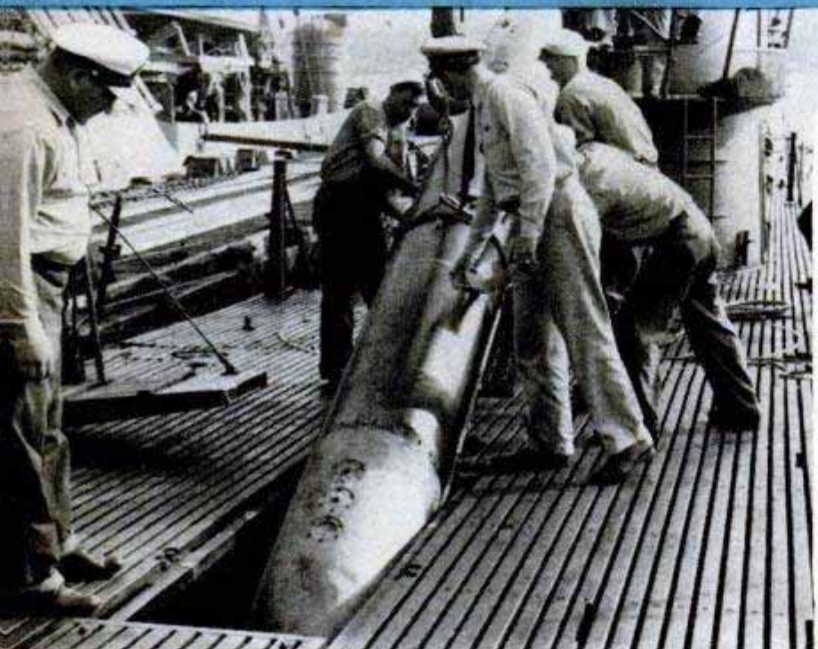
Electric torpedoes are slipped carefully through the hatch and down into the torpedo room. Torpedoes are designed to "home" on enemy craft. Below, submariners prepare to test famous Momsen lungs, named after the author, who is co-inventor of device U. S. Navy photo
