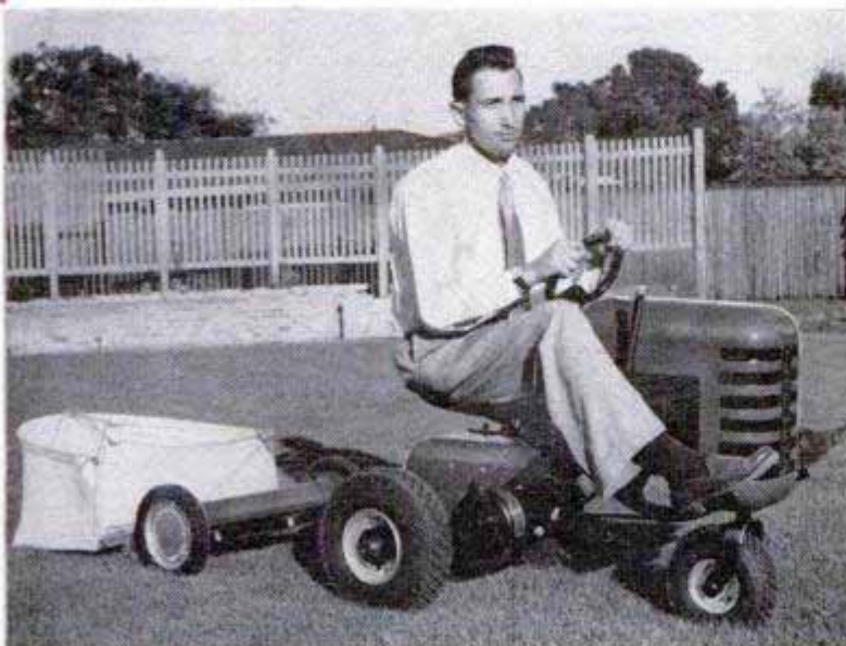
This isn't a gag shot. There's enough power in the midget to pull an automobile up a slight grade. Below, Hiller mows his lawn in comfort, towing a 20-inch mower and grass catcher. Fuel consumption for most yard work is one quart per hour
