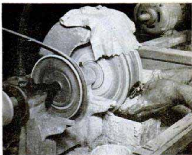
Preliminary polishing operation on wooden wheel is pictured above. Cloth spray apron hangs from hood
