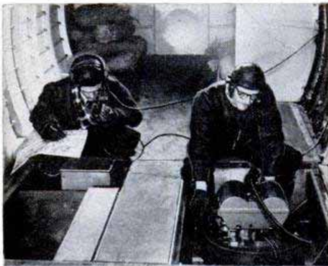
Taking photos for the dot. Man at right operates camera, assistant gives pilot instructions through microphone. Camera, below left, has a magazine of 40 photo plates on each side. Magazine is shown in center. Mechanism shuffles plates through camera
