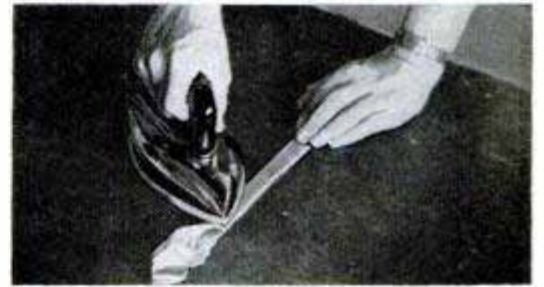
Tapes for tying flaps are made by folding wide piece of plastic six to ten times
