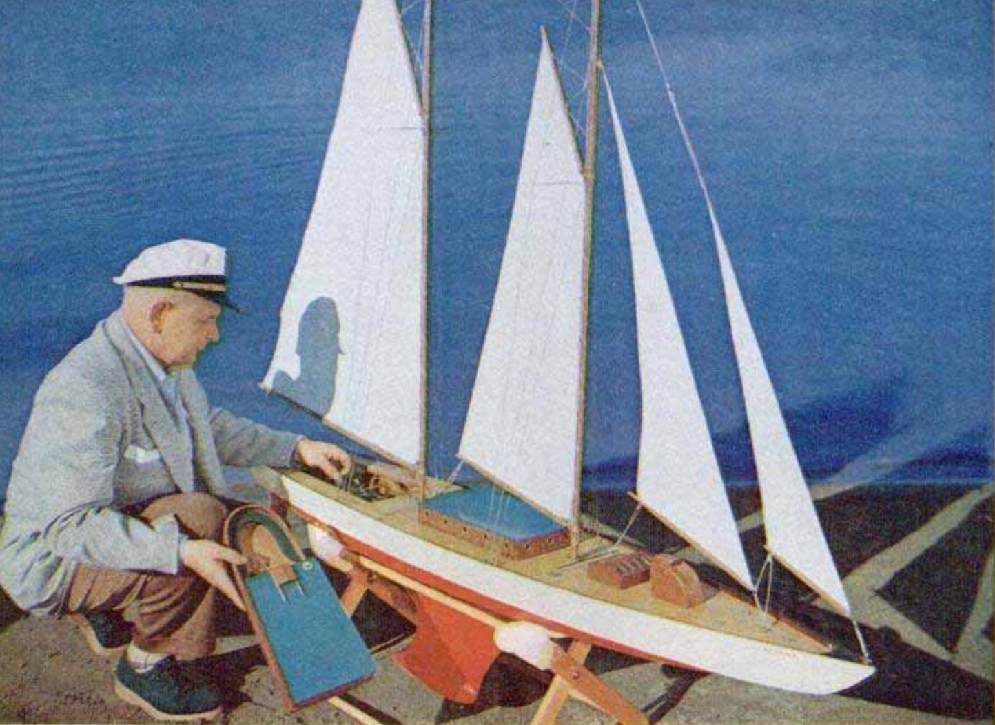
Model yachtsman adjusts radio receiver in schooner. He can control sails or auxiliary motor from shore
