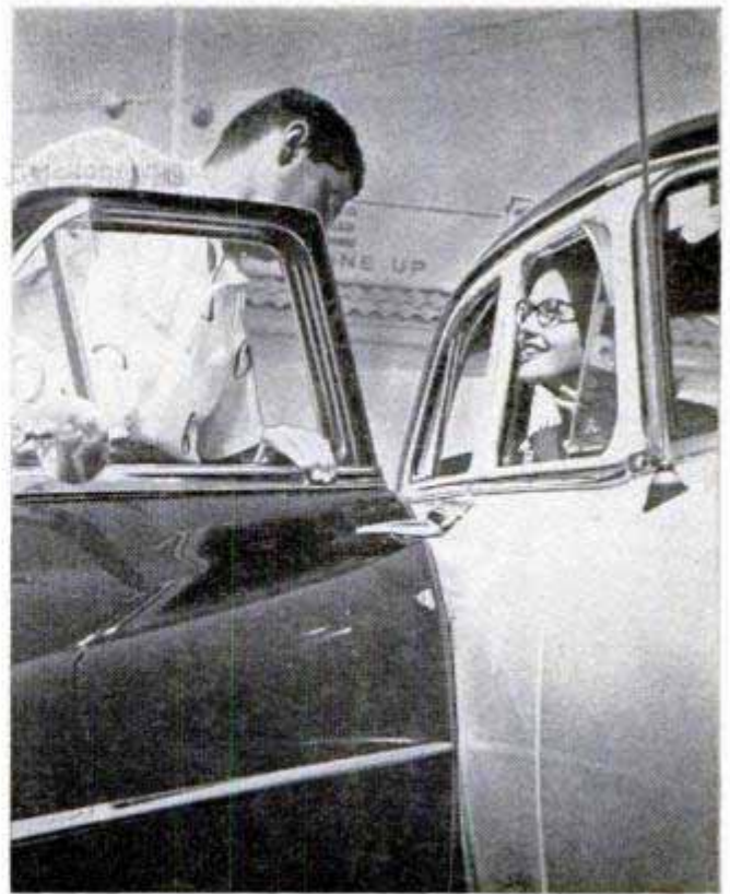
Protective plastic strip, easily applied to edge of automobile door, ends one cause of parking-lot scratches
