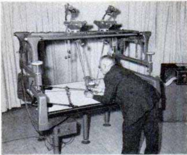
Simpler and less expensive machine than autograph is Kelsh Plotter which also makes maps. It uses red and blue dots. Observer wears red-and-blue glasses
