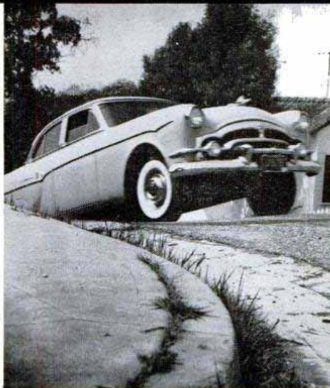
On steep hills used by Clymer for his test of the Packard, the long-stroke, straight-8 Clipper Deluxe showed that it has excellent low-speed lugging power
