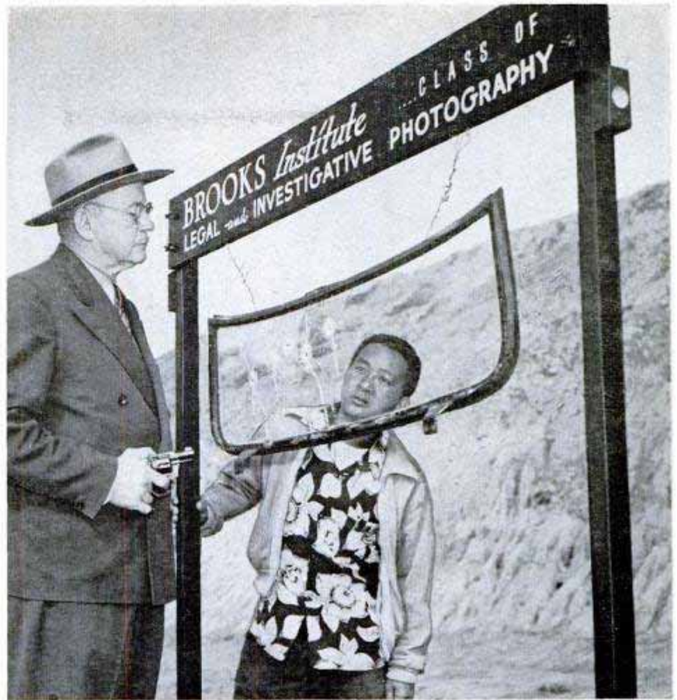
Above, students learn to tell the sequence in which bullet holes were made in windshield and, below, from which side of the glass came the force to break it
