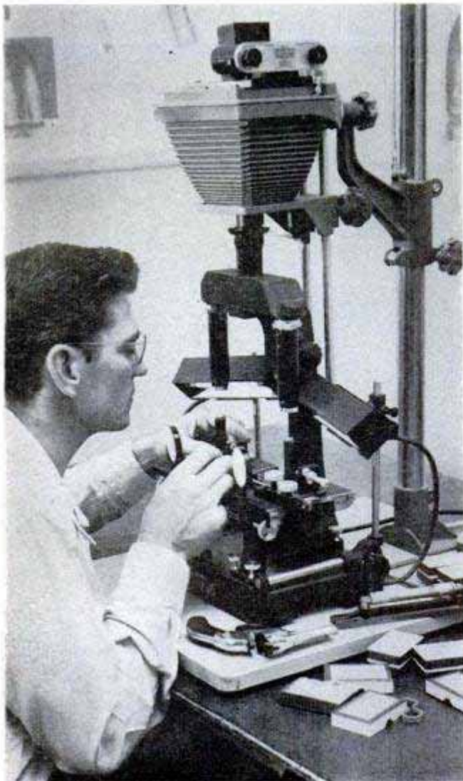
Camera on a microscope photographs bullet rifling
