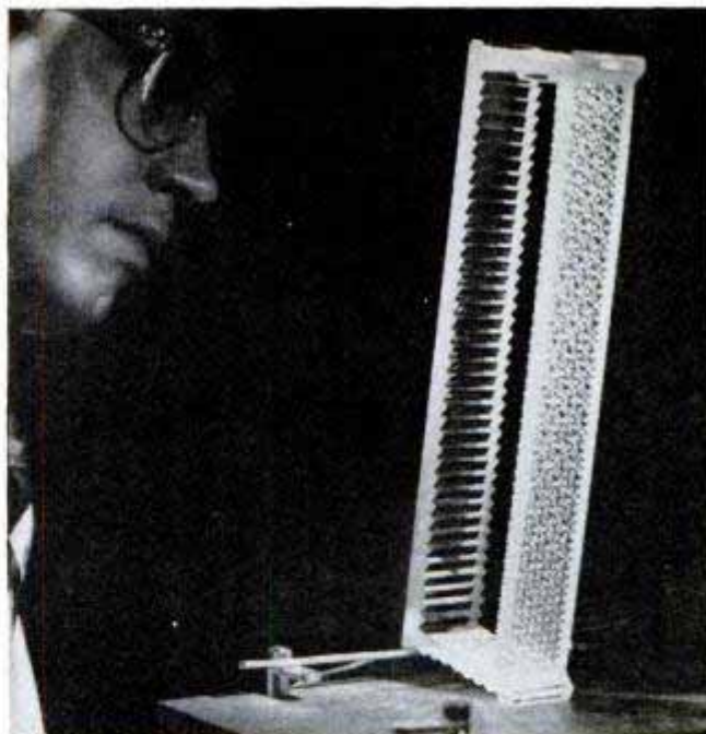
Prisms in top layer let slanting rays through but block overhead light. Bottom layer diffuses rays
