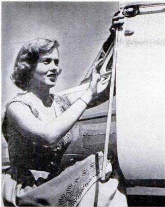
Protective plastic strip, easily applied to edge of automobile door, ends one cause of parking-lot scratches
