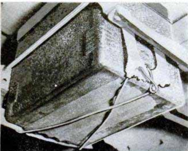
Above, checking brush-spring tension. Worn brushes, weak springs cause arcing. Below, check battery carrier often. If defective, it should be replaced
