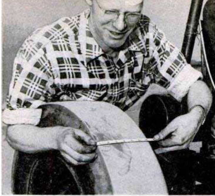
Rear tires, called asphalt slicks, provide maximum traction. Contact area is almost seven inches wide
