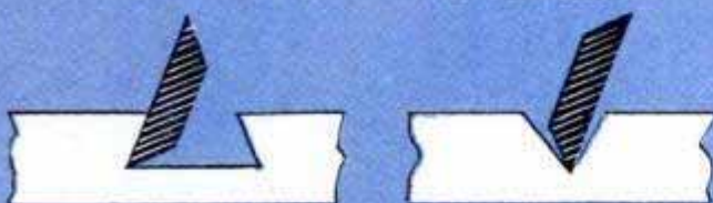
BEVELED BLADE USED FOR UNDERCUTTING AND TRIMMING V-GROOVES
