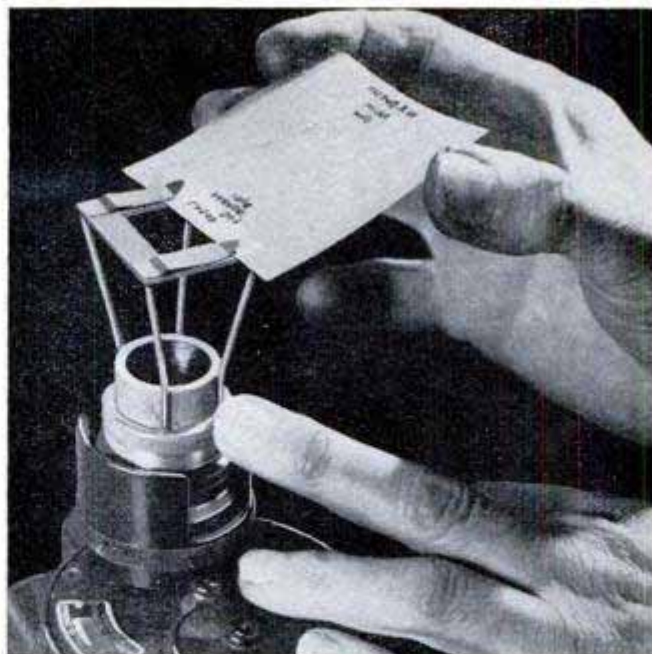
When title card is inserted beneath clips, lettering is positioned so it will read correctly when viewed through lens. Title is aligned with camera aperture
