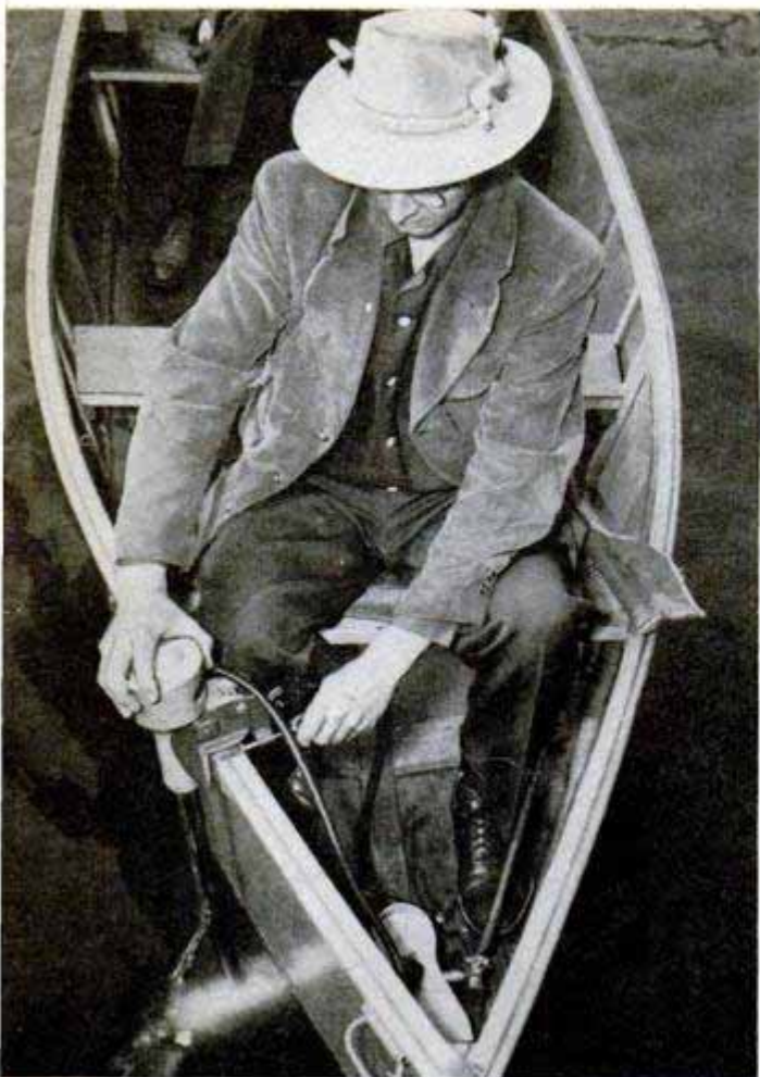
Clamping the motor, left, to the boat's side. Right, unfolding the foot-steering unit prior to installation
