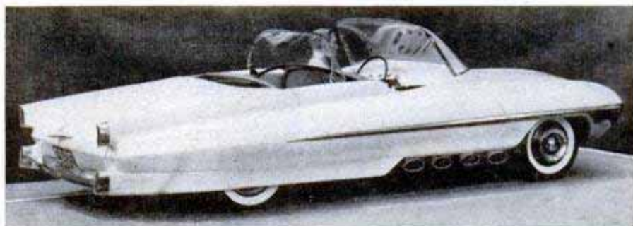
Rear window swings forward as tonneau windshield or back out of sight
