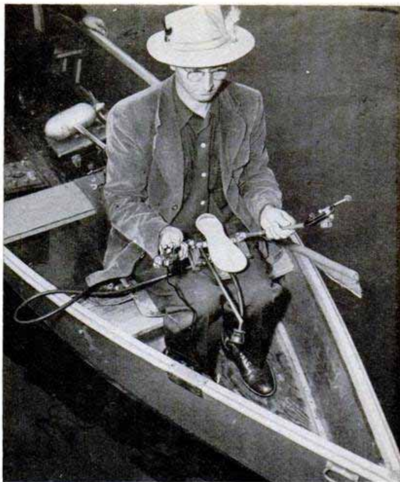
Clamping the motor, left, to the boat's side. Right, unfolding the foot-steering unit prior to installation
