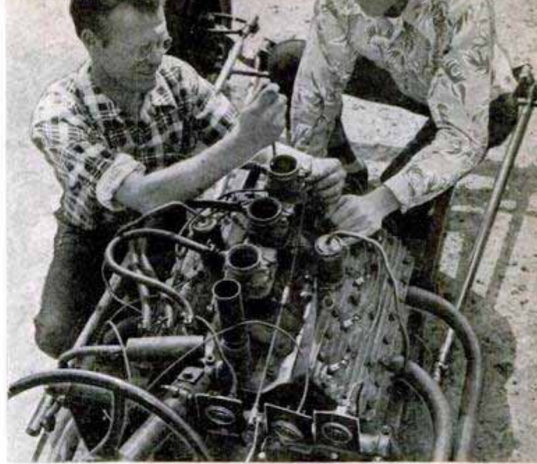
Three carburetors feed this V8. It has no radiator. If it boils, hoses deflect steam down to pavement
