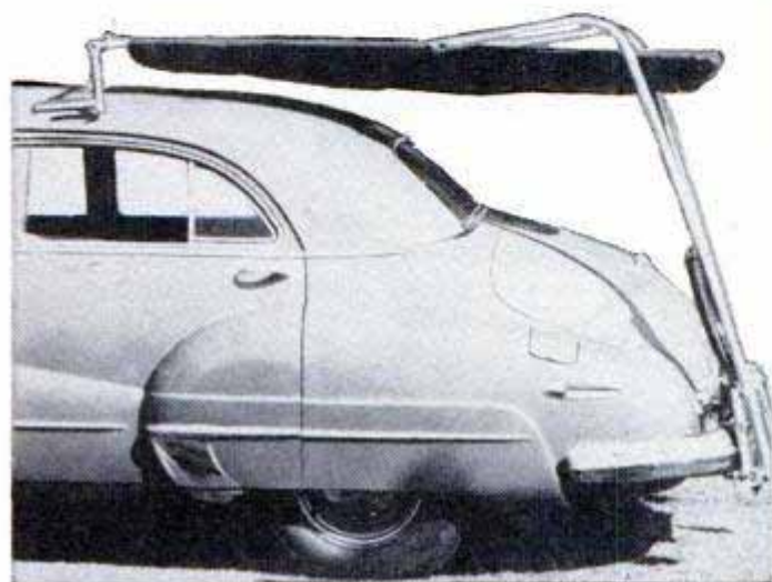
Carried atop car, the tent and bed swing down as a unit, below. In five minutes, it's ready for use, above
