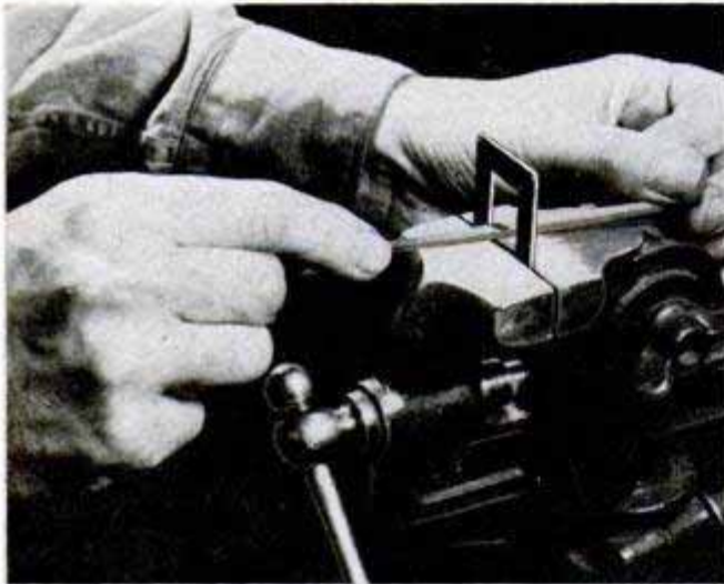
Size of the frame opening is determined by the focal length of the lens used. The edges of the frame are filed to remove burrs after cutting out center
