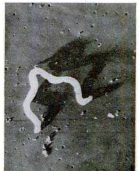
Left photo shows, as a flat specimen, an organism 1/2000 inch long that was air-dried before examination under an electron microscope. Freeze-drying of specimen, right, reveals its original three-dimensional shape
