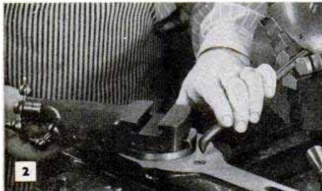
1 Sighting to a line is a simple and accurate way to set threading tool. Below, how the line is marked
