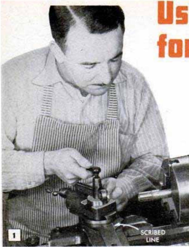
1 Sighting to a line is a simple and accurate way to set threading tool. Below, how the line is marked
