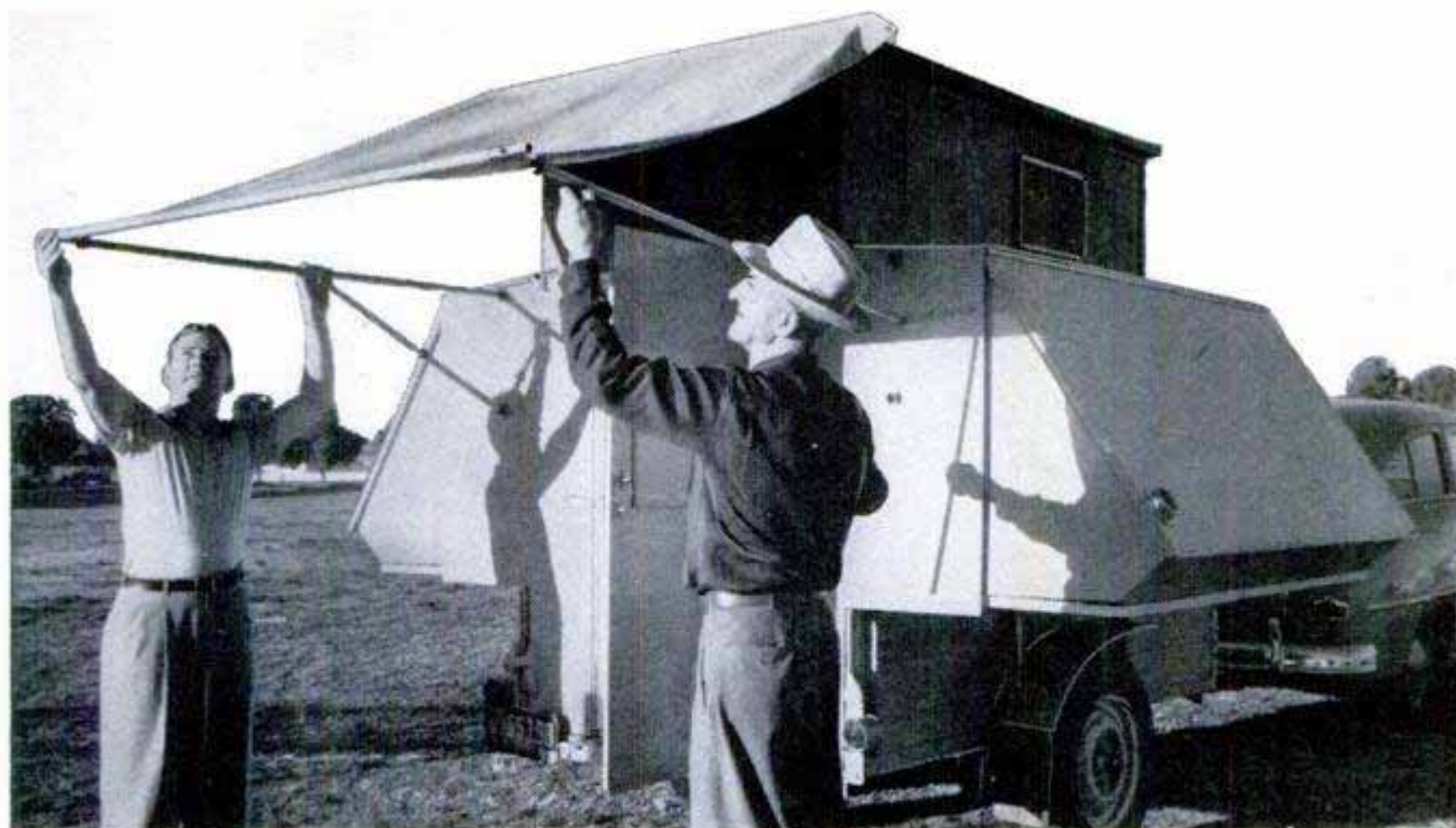
Top telescopes to standing height and the sides swing out to accommodate bunks. Rear awning supplies shade
