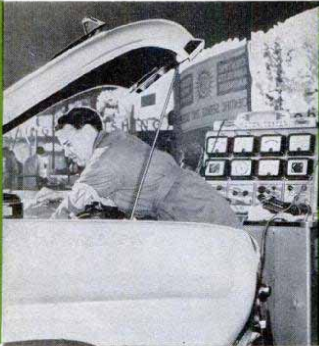
Technician making final inspection of timing and carburetor settings with test stand. Cars are under constant official supervision after selection
