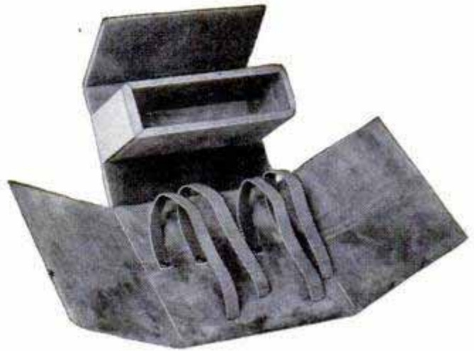
Left-hand photo shows the finished case with camera and accessories in place. Right-hand photo pictures lined metal box and pull-out straps attached to metal liner, which has been partially bent to shape. Note that the liner is lined inside with a pile plush
