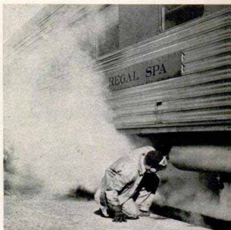
Meanwhile another crew member inspects valves of the air-conditioning systems, which blow off surplus steam while train is at rest. Below, temperature of wheel bearings is checked by feeling them with hand
