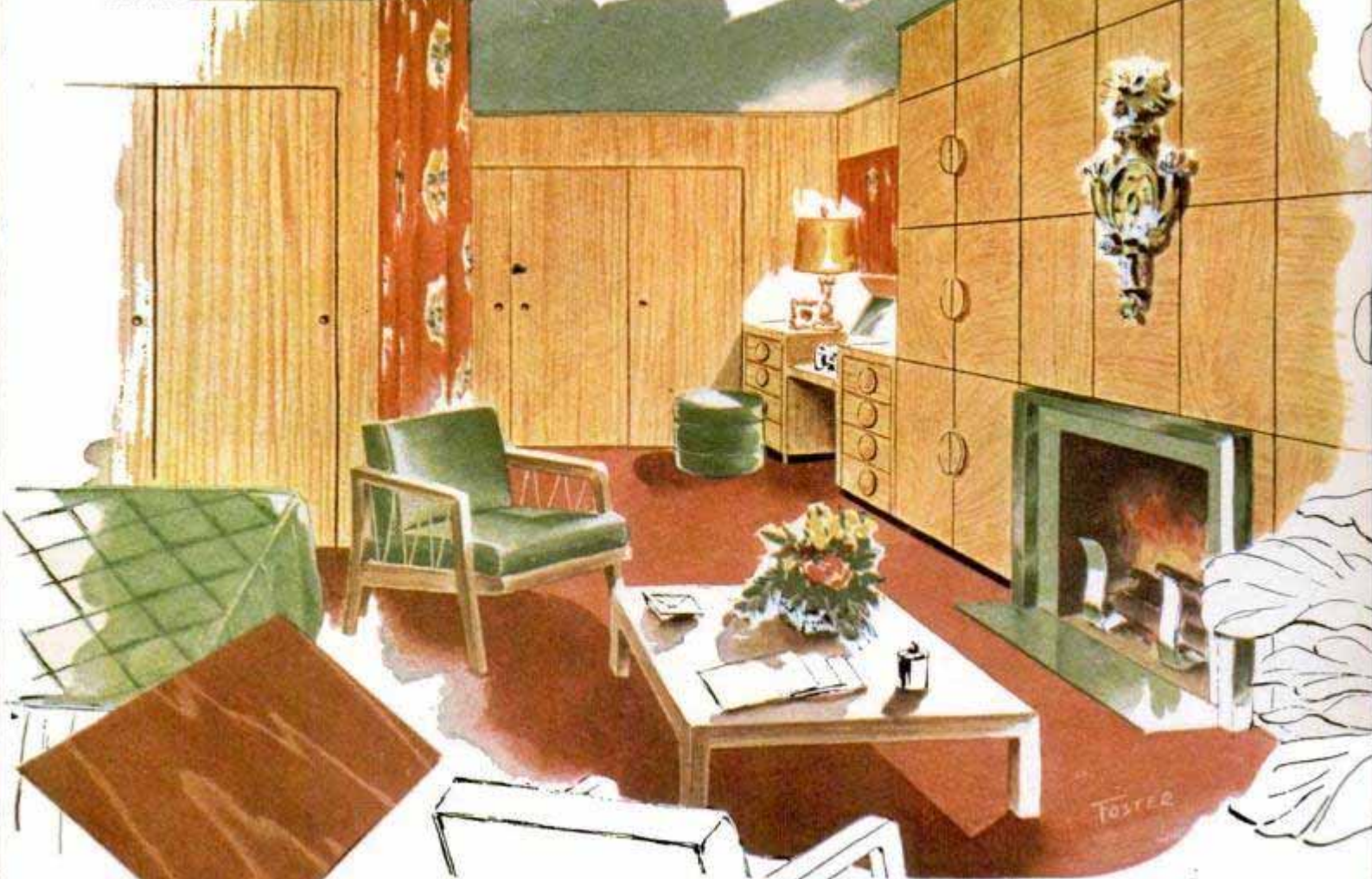
Fireplace wall of modern bedroom is of 24-in. squares of \frac{1}{4} -in. birch plywood over \frac{5}{16} -in. underlayer. Other walls are of full-sized panels
