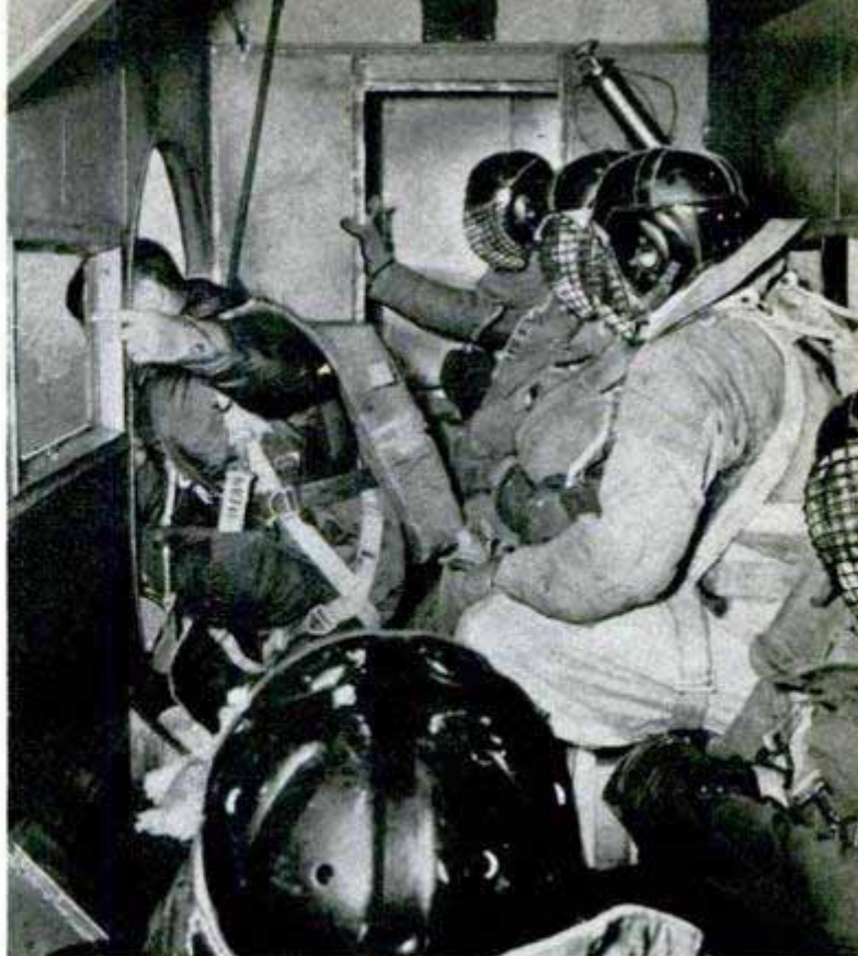
Photos on this page by Robert M. Catlin for Johnson Flying Service Inside a Ford, a crew chief, above, helps direct the pilot over the jump spot. Smoke jumpers like the Tri-Motor because its stabilizer is high and there is no danger of snagging their chutes as they leave
