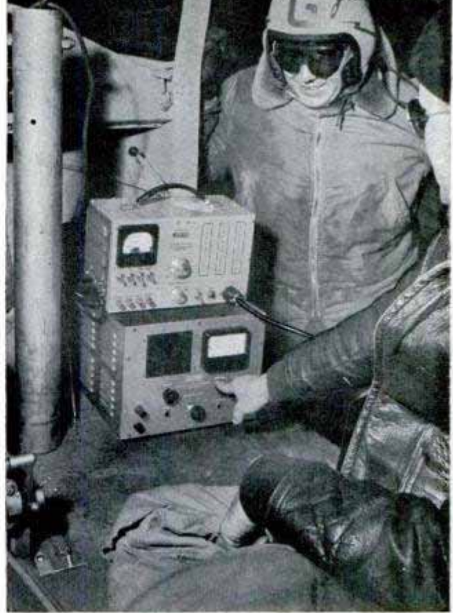
Instruments inside helicopter show radiation picked up by trailing detector, here retracted before take-off
