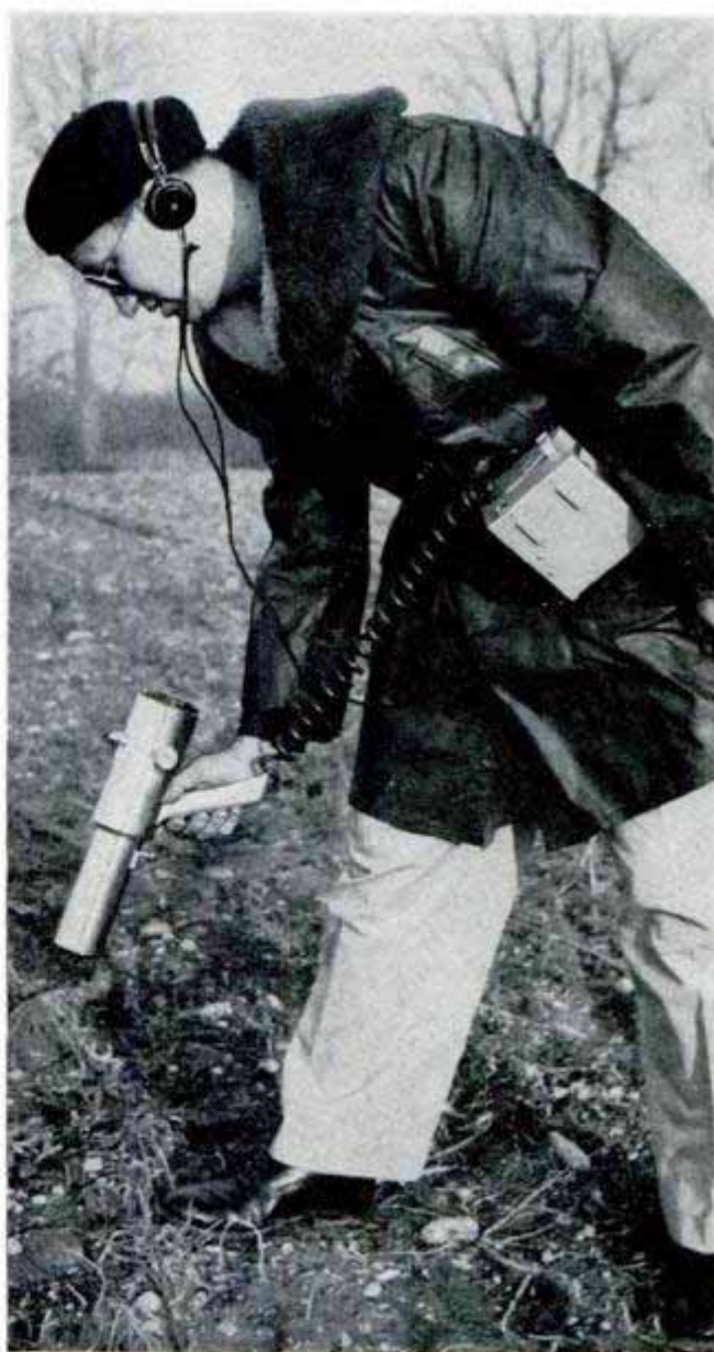
Hand scintillometer for ground surveys registers nuclear bombardment on dial at base of instrument
