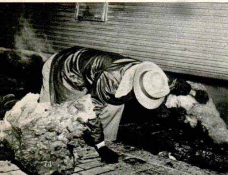
Electrician swings aboard as soon as streamliner pulls in, unlocks and inspects each air-conditioning unit. Below, in winter, ice piles up beneath diesels. Here an inspector pulls off chunks to check valves
