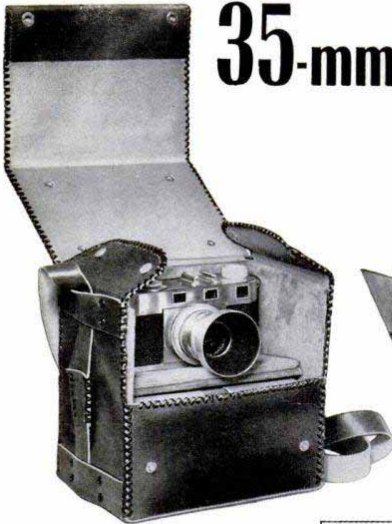
Left-hand photo shows the finished case with camera and accessories in place. Right-hand photo pictures lined metal box and pull-out straps attached to metal liner, which has been partially bent to shape. Note that the liner is lined inside with a pile plush
