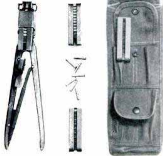
Stripper on handle of tool, left, scrapes ends of wire. Bare wire ends are then put into cartridge and crimped. Below, tool and carrying case
