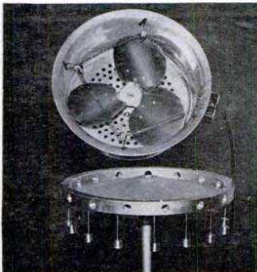
Fan and heater are in top. Plugs block openings to divert flow of air. Right, the drier has 30 feet of "line"
