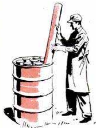
Above, three gal. of preservative in oil-drum tank will treat about six 4-in. posts
