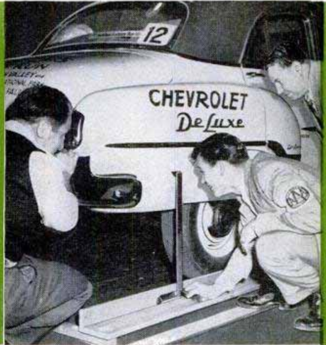
Checking leveling mark for filling fuel tank. At end of Run each car was placed in same position to obtain precise check on the amount of fuel consumed
