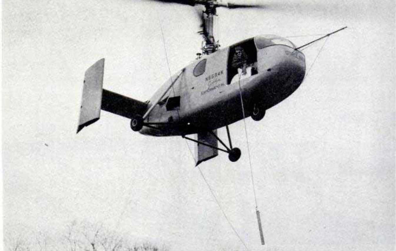
Scintillometer is suspended by cable so it can skim along close to ground and pick up only direct radiation
