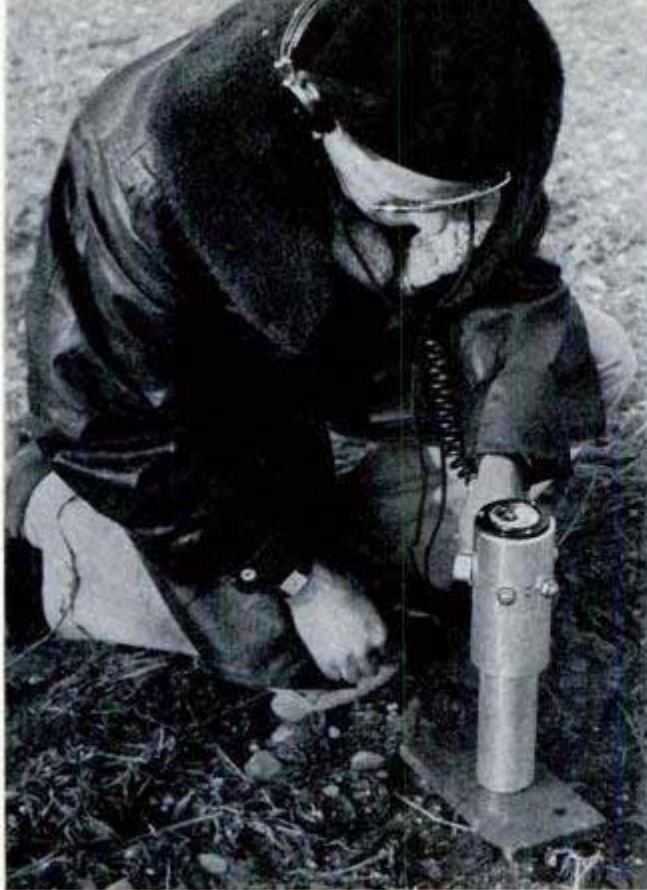
Checking influence of cosmic radiation, Scherb places "gun" on lead shield to block radiation from ground
