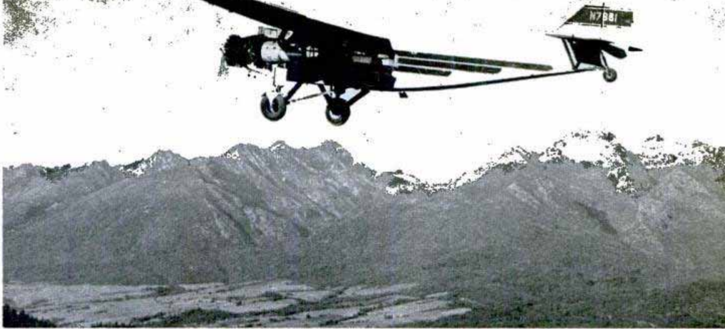
Flyable on two or even one engine, Tri-Motors are still sought for hauling jobs in mountainous regions
