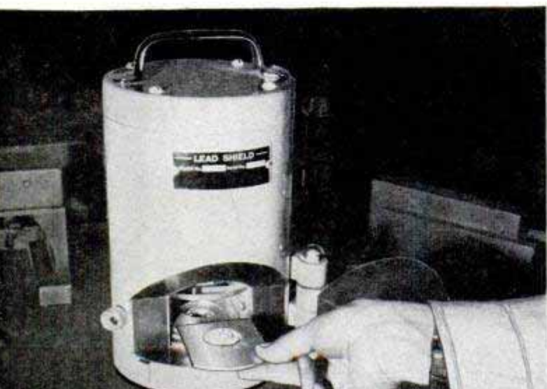
Soil sample from field is placed on tiny metal disk and shoved into "castle" which measures beta rays
