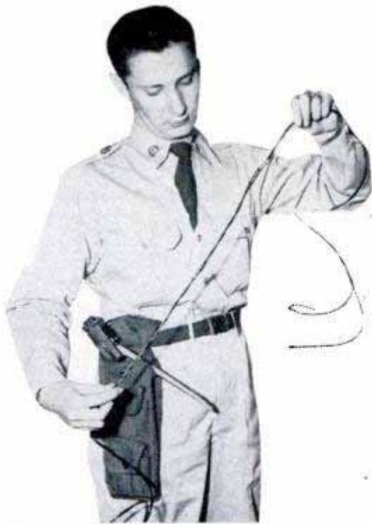
U. S. Army photos Soldier holding wire with two completed splices. Crimped connector cartridge is shown at the right
