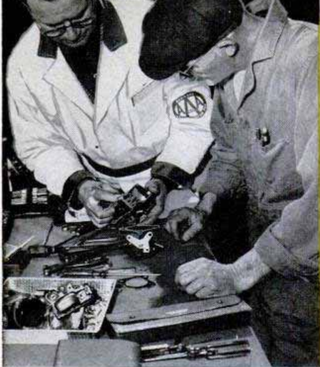
Technicians dismantle and inspect a carburetor to make certain that all parts and adjustments meet factory specifications for each car entered in the Run
