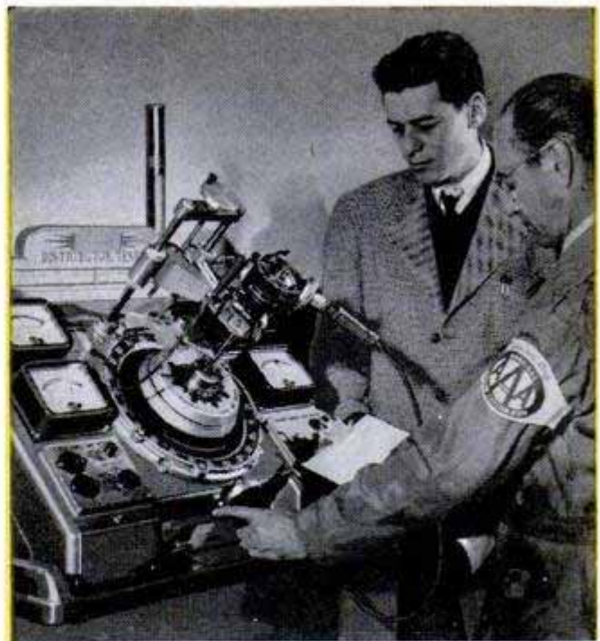
Members of technical staff verify distributor adjustment and vacuum-spark advance. Careful check is made of spark as it must fall within certain tolerances
