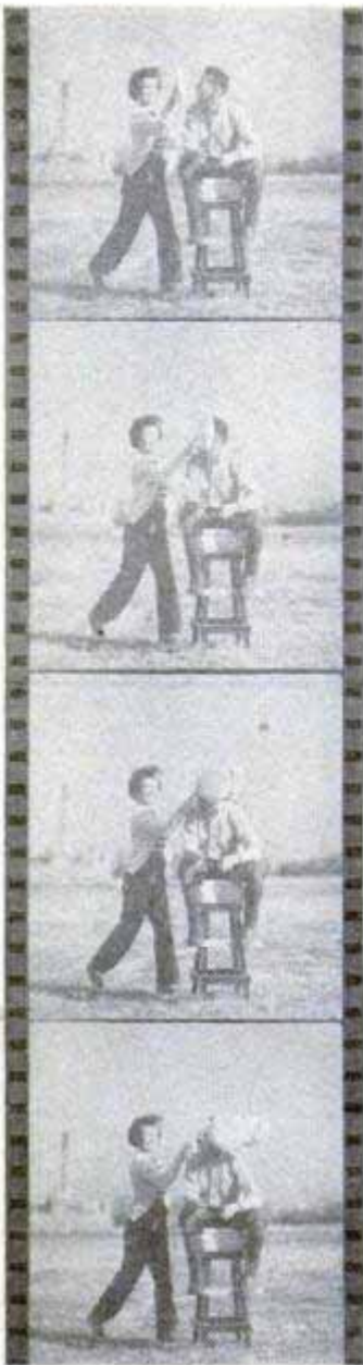
Fast-sequence camera takes roll film about 2¾ inches wide. Series at left was taken at 50 shots a second
