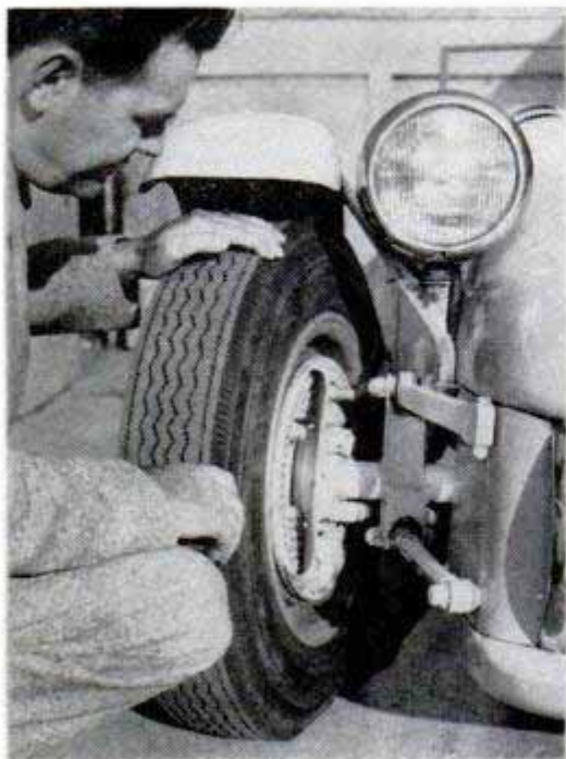
Left, scoops cool front brakes. Right, engine is mounted well behind wheels for good weight distribution
