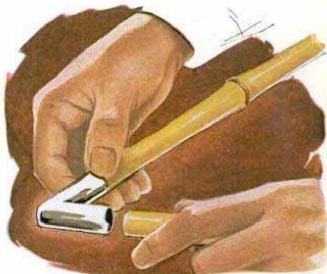
Coffee-table legs, above, and chair legs, below, are joined with brackets made of scrap sheet metal
