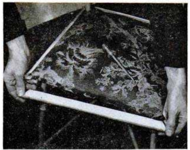
After fabric is tacked to chair frame, bamboo edging is fitted around seat, photos above. The mitered bamboo edging is backed with half-round molding
