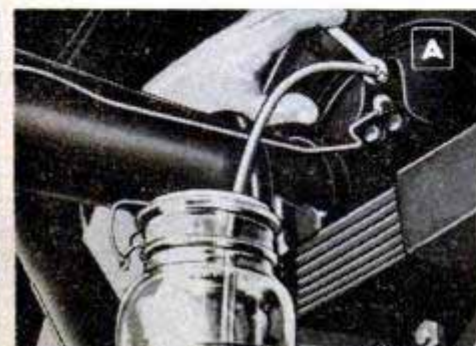
Leave reconditioning and servicing of hydraulic brakes to your serviceman as he will have special equipment required. Dismantled master and wheel cylinders are shown above. Below, bleeding air out of brake lines
