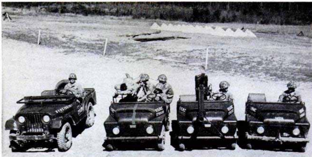
At left is a Jeep. Three other vehicles are Marine Mites, rigged as ambulance, gun mount, signal truck
