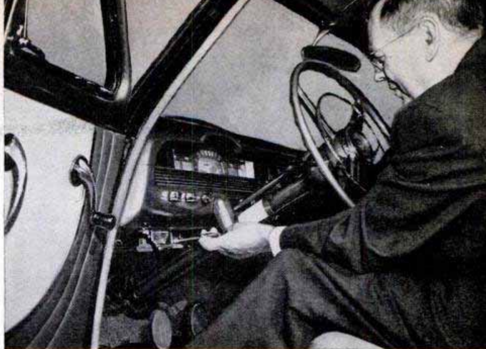
Clymer pulls out overdrive control. A fluid torque converter is now available for Plymouth. Instrument panel is neat, easy to read
