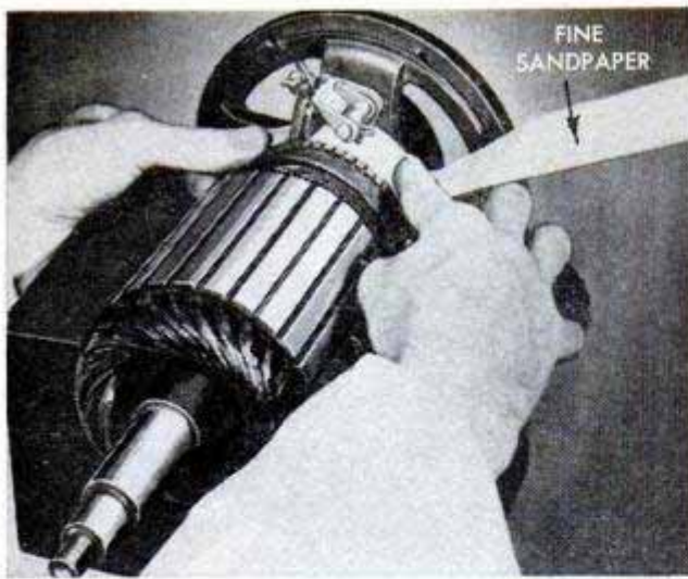
When generator and starter are removed it may be necessary to clean commutators. Use fine sandpaper
