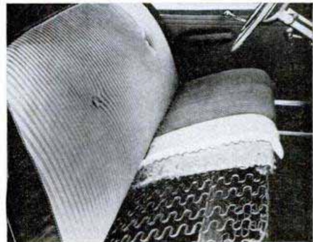
Above, glass channels may still be serviceable even though immersed. If not they are easily replaced. Below, usually a thorough washing and drying will recondition seat cushions. Then vacuum-clean the fabric
