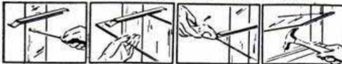
Screw on SUN-SASH fittings to side of window frame. Slide glass louvres to rattle-proof clip holders. Close end of clips over firmly in position. Install 3/4" stop top and bottom. (Window stool may be used for bottom stop).
