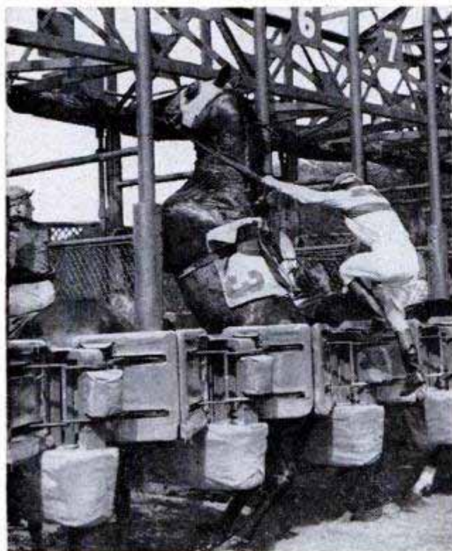
Starter on control stand with complete view of horses presses button connected by cable to main switch to open doors of gate. They're off!
