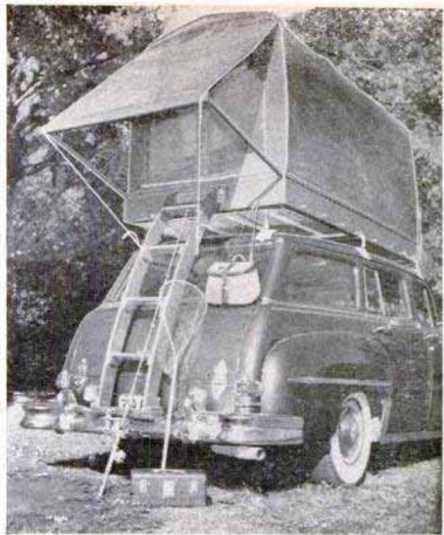
Ladder leading to entrance has curved stiles to fit over car trunk. Ladder is hinged to car bumper
