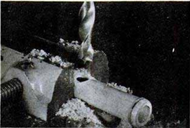
Use spur bit, above, for drilling large holes. If screw-tipped bit is used, first drill pilot hole. Preheat stems over low flame, below, before bending them
