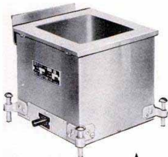
↑ HEAVY-DUTY SOLDER POT takes large units for soldering by immersion and is available in varying sizes and temperature ranges. Has long-life ceramic-embedded element and thermostatic control for fast recovery. The unit is fitted with adjustable legs and dross tray
