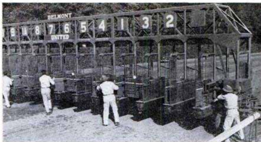
Starting gate is set into position five feet from rail and doors are being closed before horses reach post. Man at right sets control switch
