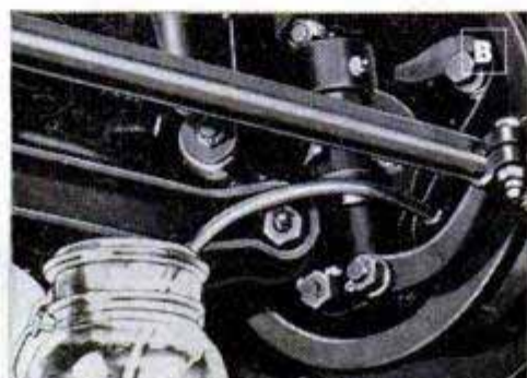
Leave reconditioning and servicing of hydraulic brakes to your serviceman as he will have special equipment required. Dismantled master and wheel cylinders are shown above. Below, bleeding air out of brake lines
