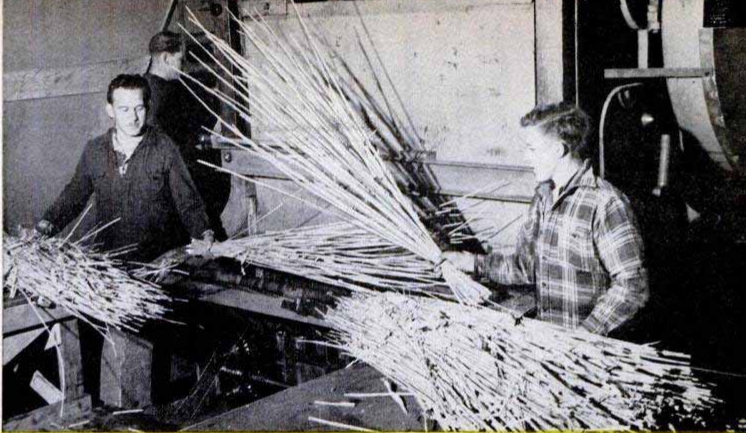
Two men feed reeds into machine, placing stalk butts in opposite positions to make boards of even thickness
