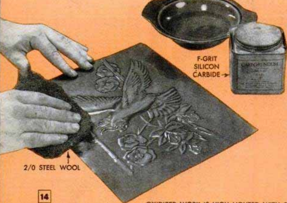
OXIDIZED WORK IS HIGH LIGHTED WITH 2/0 STEEL WOOL OR F-GRIT SILICON-CARBIDE ABRASIVE WITH WATER
