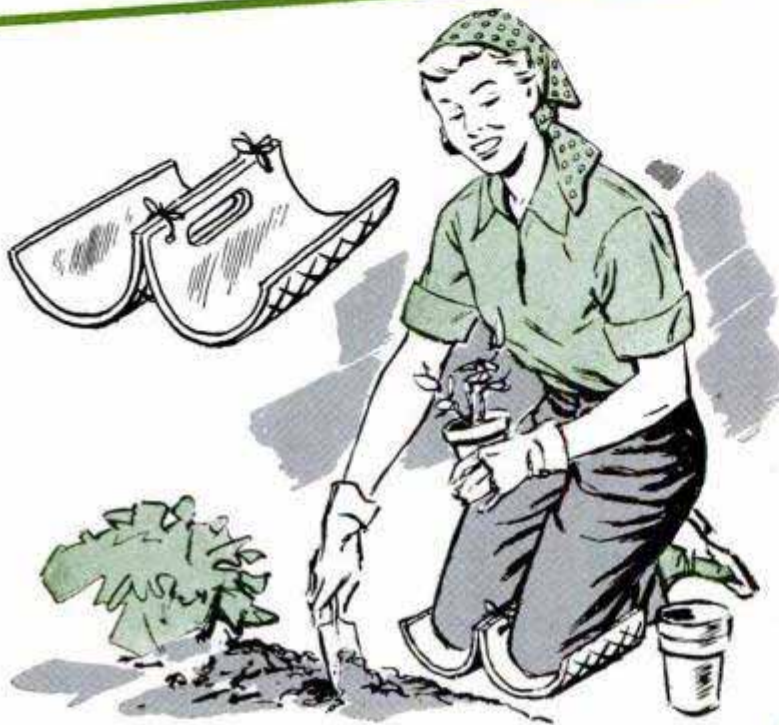
RUBBER KNEELING PAD for working in garden is made from sections of tire casing. Slots cut in sections form handle and casing is drilled so the two parts may be wired together or tied with heavy twine
