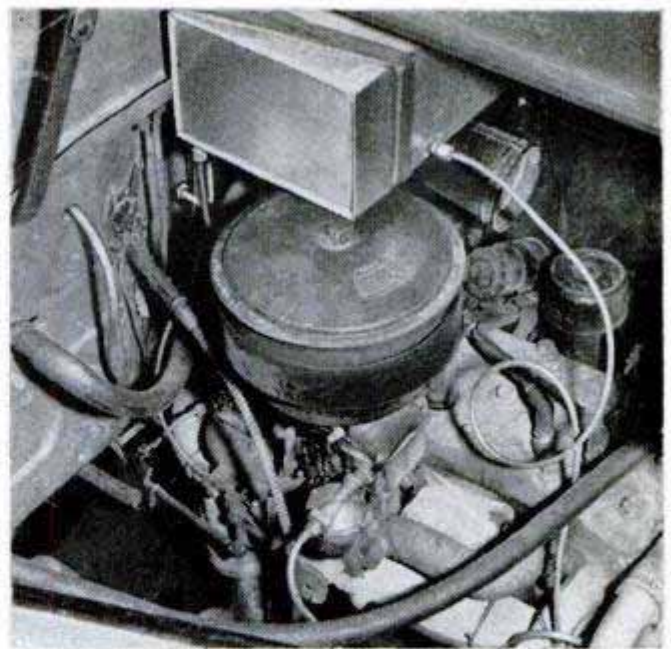
Faucet is mounted within easy reach of driver. Water is heated by passage over hot manifold of the engine
