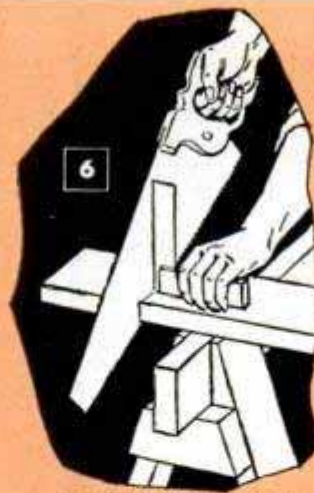
CHECK SAW WITH TRY SQUARE FOR RIGHT-ANGLE POSITION
