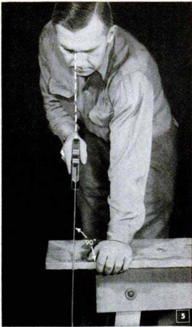
START WITH SLOW BACKSTROKE FROM HEEL OF SAW
