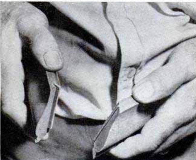
Spline joint, ready for the glue, is neat and strong
