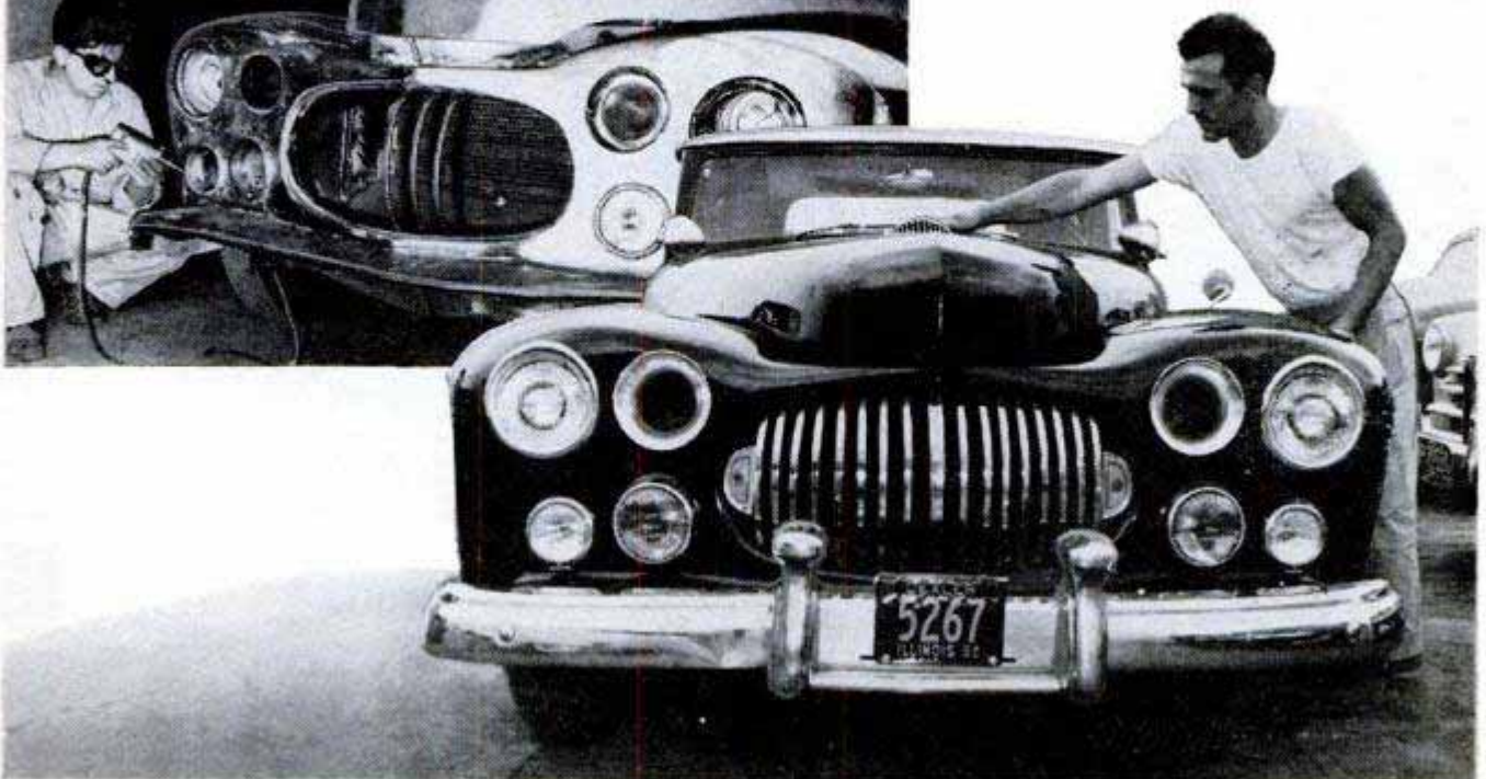
Left, mechanic at work making front-end changes shown in completed job below. Changes include grille, holes for air horns and the various lamps
