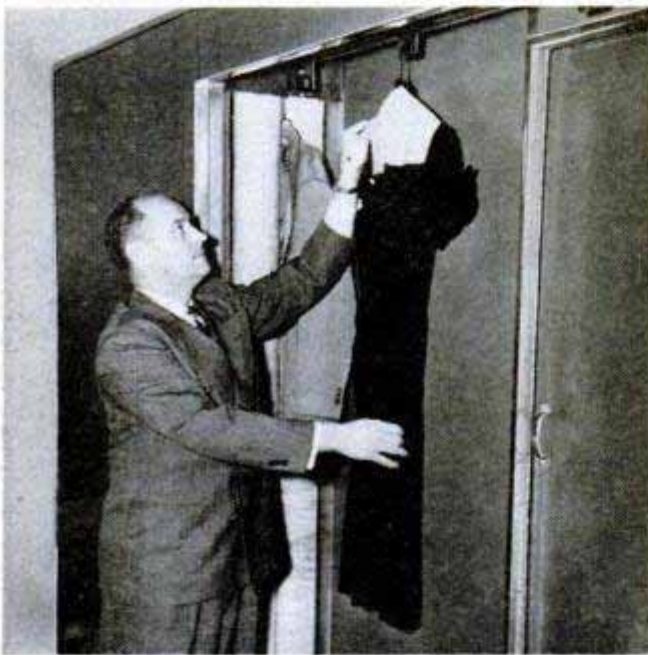
Dress is placed on conveyor as coat disappears between closure rollers which keep heat and spray inside
