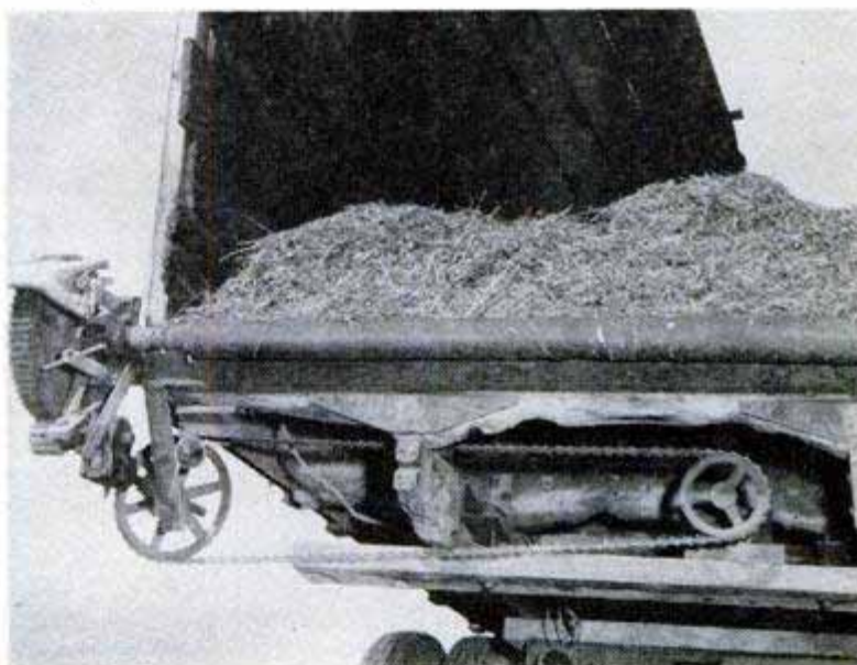
Old truck's motor turns roller to move a canvas belt on bed of vehicle. Belt slowly unloads field-chopped hay. Below, the axle of an old Buick, cut in two and lengthened with a timber, becomes tractor-drawn trailer for moving bulky range shelters
