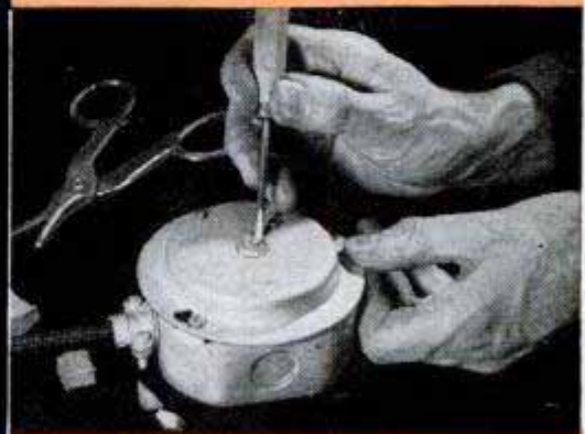
Foam rubber around switch pin keeps dirt out of box. Note tape wound on cord to increase size for connector
