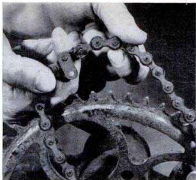
Special repair kits are available for replacing worn parts of the drive chain. Rollers and links which show excessive wear or rust pits should be replaced
