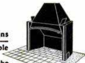
Fireplace form set on foundation includes firebox, damper, down draft shelf and smoke dome.
