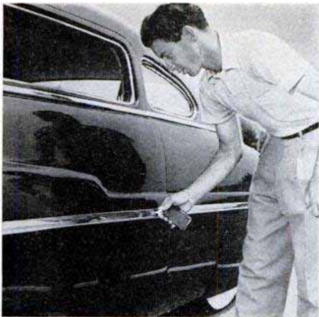
Ignition-type lock for door with handle removed is concealed in chrome strip; it operates electrically
