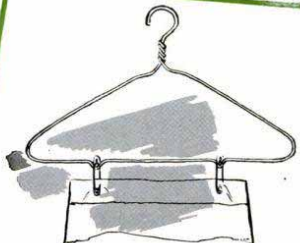
SKIRTS PINNED TO COAT HANGERS won't pull together and wrinkle if the lower wire of each hanger is crimped at two points as shown above
