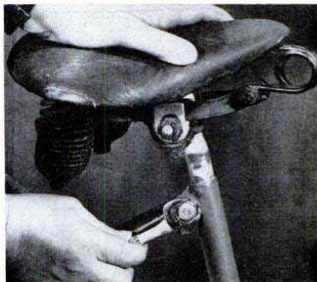
Above, as a final part of service checkup tighten saddle bolts to uniform tension. Below, final step in disassembly of crank bearing. Note that one bearing is being held in the left hand while crank is passed through housing. Clean these parts thoroughly
