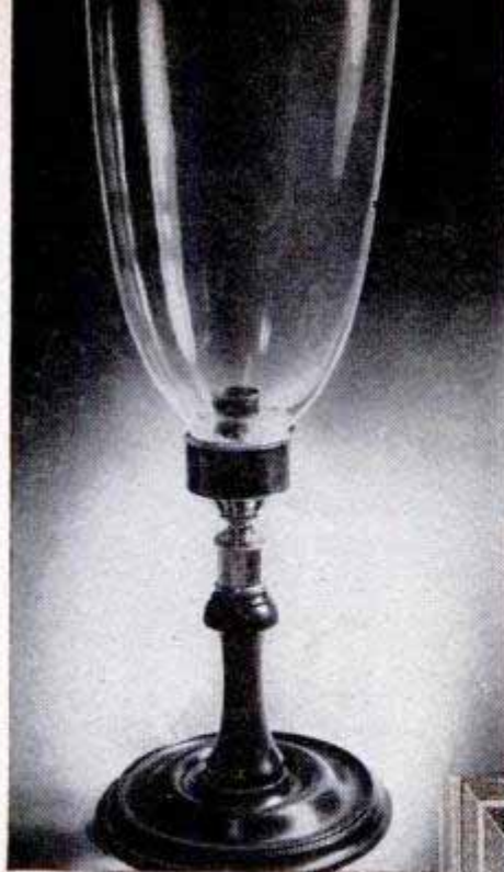
Base and stem of hurricane candleholder are connected by a threaded wood joint. It's tight but comes apart easily
