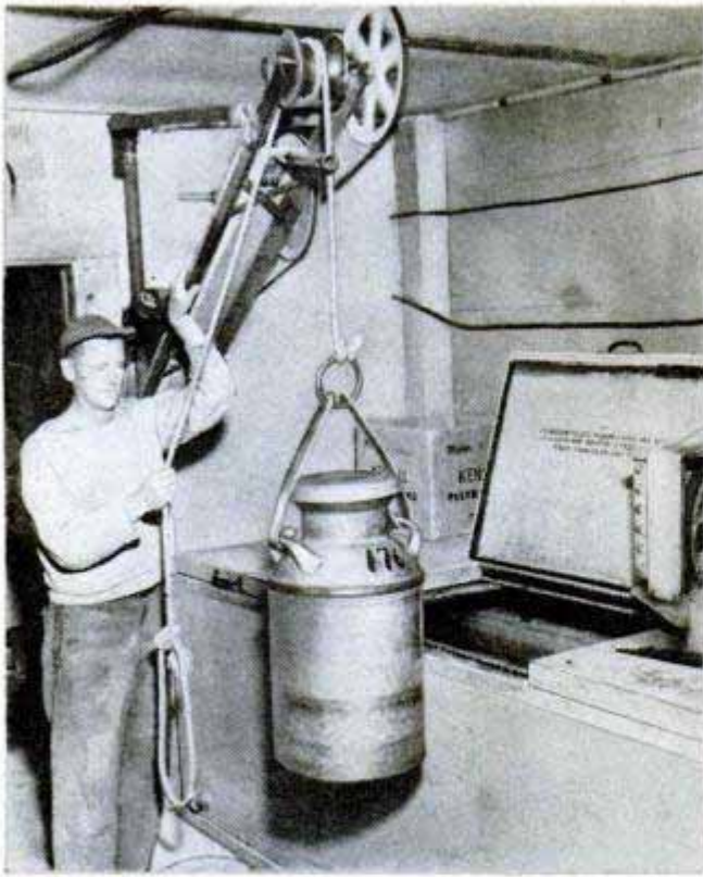
Hand pressure "throws in" clutch on electric hoist which lifts milk cans. Wall pivot is Nash drive shaft
