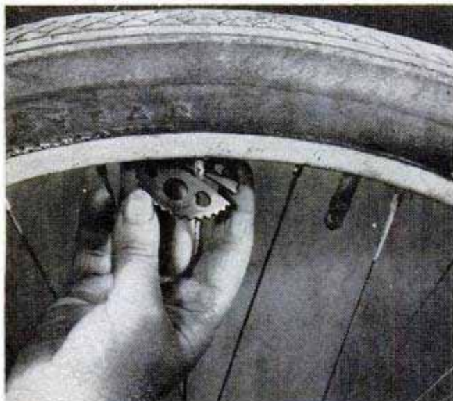
Above, after reassembling the wheel bearing, tighten adjusting cone just sufficiently to take out all end play, yet permit wheel to turn freely. Below, adjust wheel tension with spoke wrench, drawing spokes to a uniform tension. Be sure the wheel rim is true
