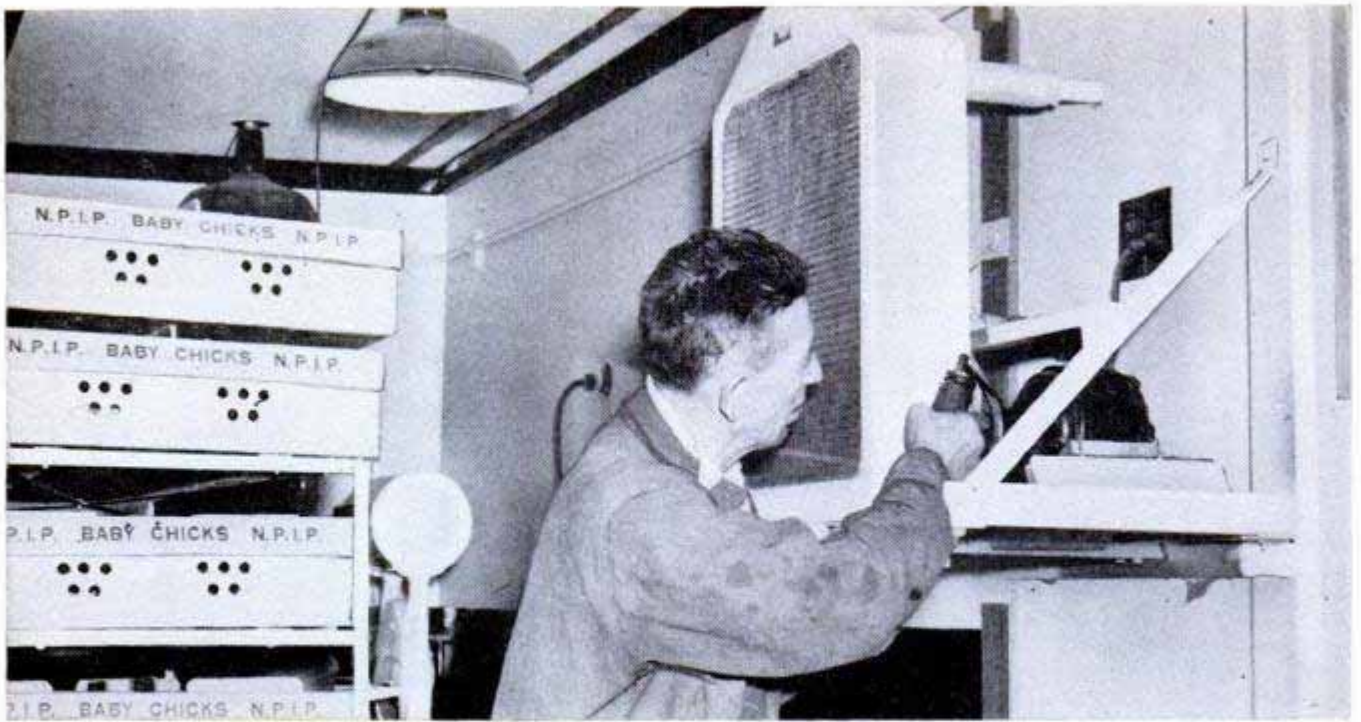
No heat in the hatchery, so this farmer piped hot water through an old Pierce-Arrow radiator to make heater
