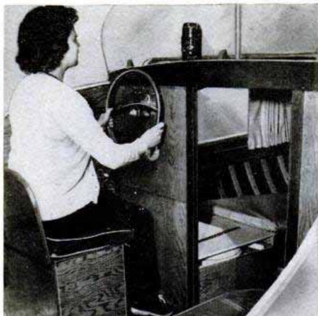
Above, remote controls enable the pilot to sit up front as on inboard cruisers. These motors put out a combined 50 horsepower. Below, Mrs. Ewald at the wheel. The base of the seat contains extra gas tank
