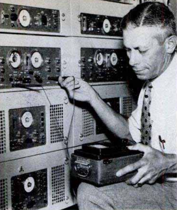
Newton checks filament voltage on amplifier panel
