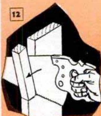
DON'T USE SAW TO PRY OFF WOOD BEFORE FINISHING THE CUT
