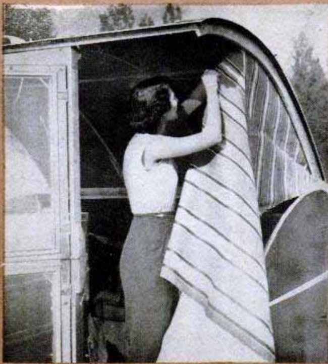
Fabric walls enclosing kitchen area are attached with grommets and turn buttons. Use heavy awning cloth
