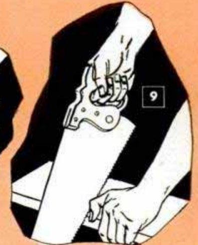
USE THUMB KNUCKLE TO SUPPORT SAW BLADE WHILE STARTING
