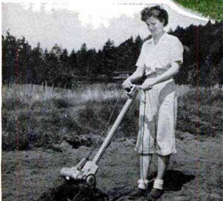
Motor is controlled by combination switch outlets mounted on mower and cultivator handles
