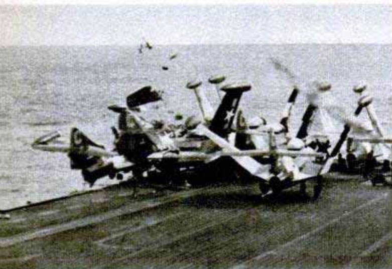
The crash — four other jet aircraft are damaged Damaged jets afloat alongside carrier. Cause of accident: Pilot tried to land despite "wave off" signal
