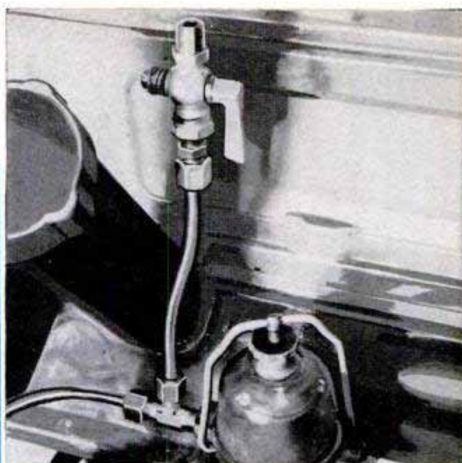
Air bleed can be installed on intake side of fuel pump by running tubing from fuel line to shutoff valve. T-fitting and valve are pictured above, valve normally is located as shown below, left
