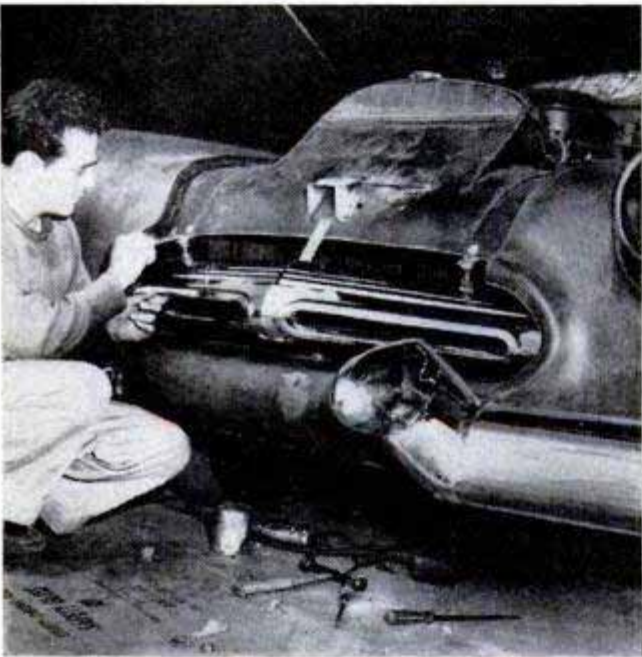
Above, attaching custom grille of "floating" type in front of radiator. Split two-piece bumper will complete the assembly. Below, in building one-piece body, construction joints are first welded together and then smoothed over with plenty of body solder
