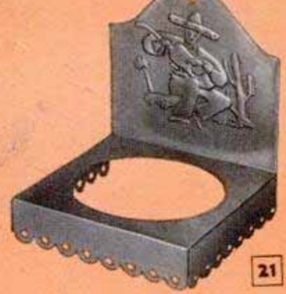
CUT WITH SCISSORS AND HAMMER OVER EDGE
