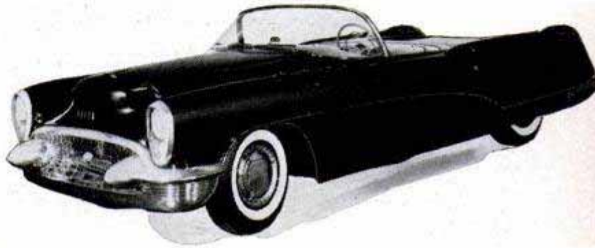
Buick's dream car is the plastic-bodied Wildcat that has a sleek elegance enhanced by the fact that it uses little chrome ornamentation. The interior is trimmed in brilliant green leather. "Roto-Static" front-wheel disks remain stationary while the wheels revolve about them for sparkle
