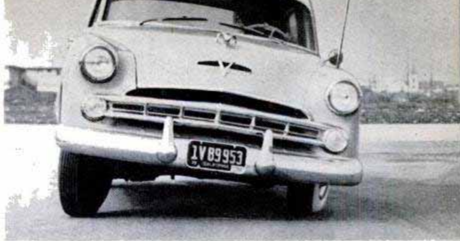
Front-end springing could be stiffer, according to Clymer. It is so soft that there is a tendency to "roll" on sharp turns
