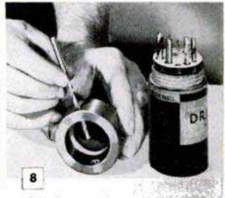
Lacking other means, determine size of internal thread with tap drill
