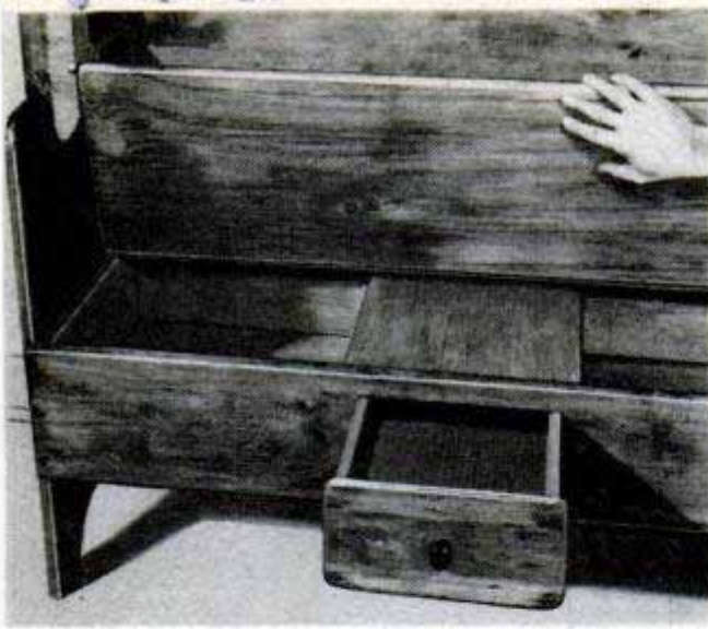
One of the unusual features of the hutch-table construction is the fully housed drawer at the center of the storage compartment. This construction divides the main compartment into two separate storage spaces
