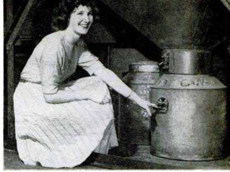
Air circulating through the gold-using plants is filtered and the metal collected in cans like this
