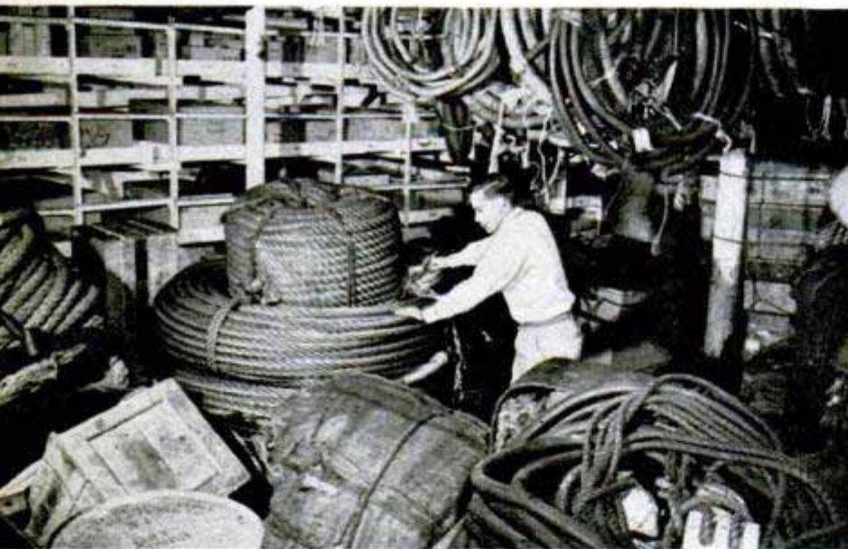
Stored in the honeycomb of the Curb's hull are miles of steel cable and rope for pulling wrecks off beaches. Below, how far ashore can a ship go? Hurricane deposited SS Phoenix on edge of highway. She was relaunched by digging trench under hull
