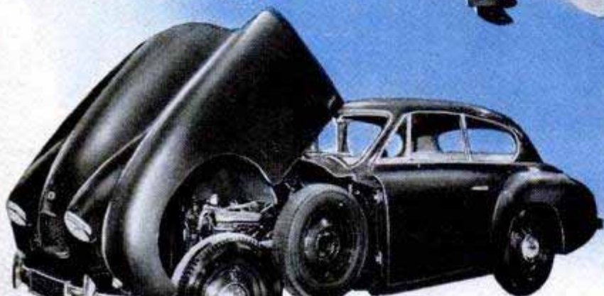
Above, Allard's Palm Beach three-seater comes with four or six-cylinder engine. Below, another Allard, the Monte Carlo, has a bonnet that opens hydraulically
