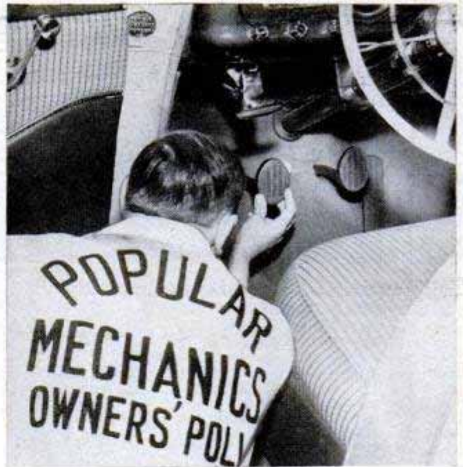
Even with Dodge's torque converter, you must use the clutch pedal when shifting from neutral into drive
