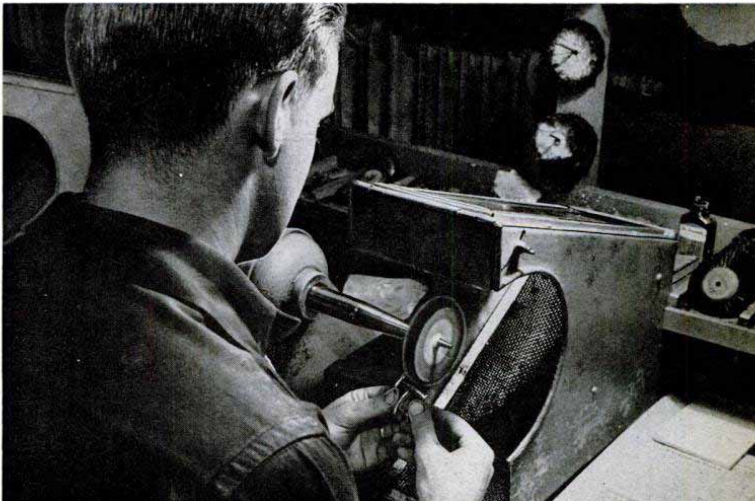
During polishing operations the gold dust is sucked through screens directly below the operator's hands
