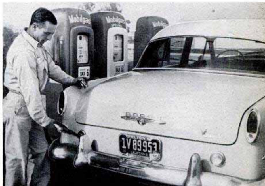
Gas-filler opening in the rear is more satisfactory, but some owners said the pipe didn't have enough slope to handle flow
