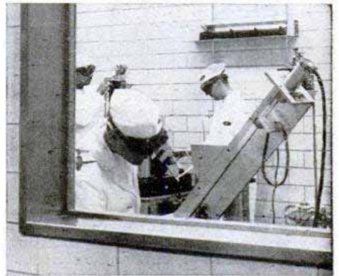
Plasma from tanks is shot in a thin film through ultraviolet tubes in order to kill jaundice virus
