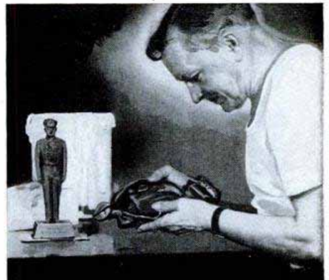
Above, after the first half of the casting shell has set and is coated with soap solution, the box is ready for pouring the second half of the shell. Below, the rubber mold has been cut from crown to base and the plastaline figure removed. Mold is now washed
