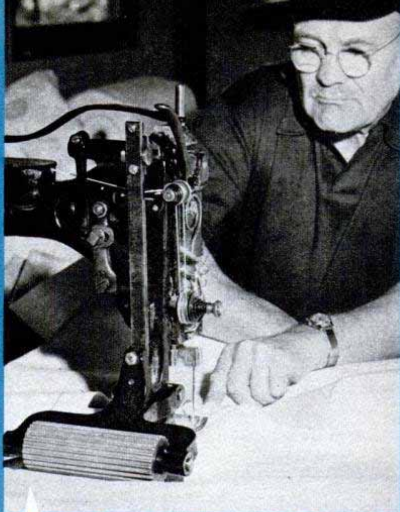
Heavy-duty sewing machines handle all the large work in sailmaking today. In the old days all sails were hand-sewn, but the cost of a hand-sewn job now is prohibitive
