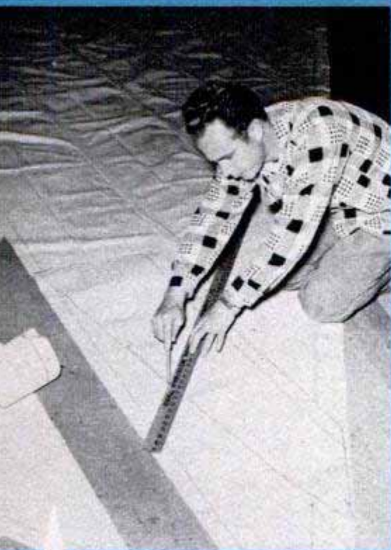
Corners and head of the sail are reinforced by patches. Here a corner is being measured and the patch cut to fit. Right, when sail is sewed it is laid out on floor of sail loft
