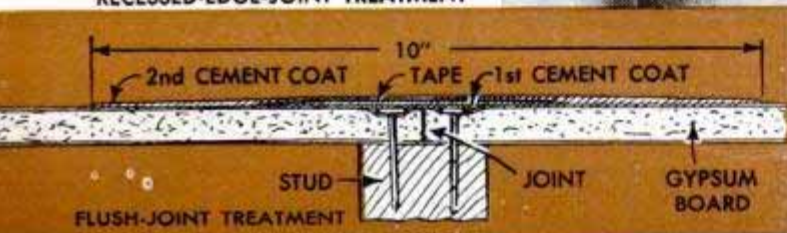
Details above show how easily the joints in the wallboard are hidden with special tape and the cement
