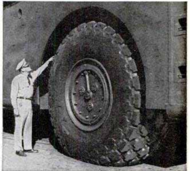
Pressure in the huge tires can be varied from within the cab to meet changing ground-surface conditions
