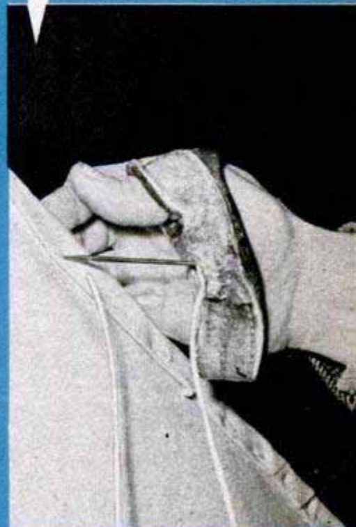
Sail is "roped" with stainless-steel wire. This is a hand-sewing operation. Below, sail-maker's palm is made of an extra-heavy leather
