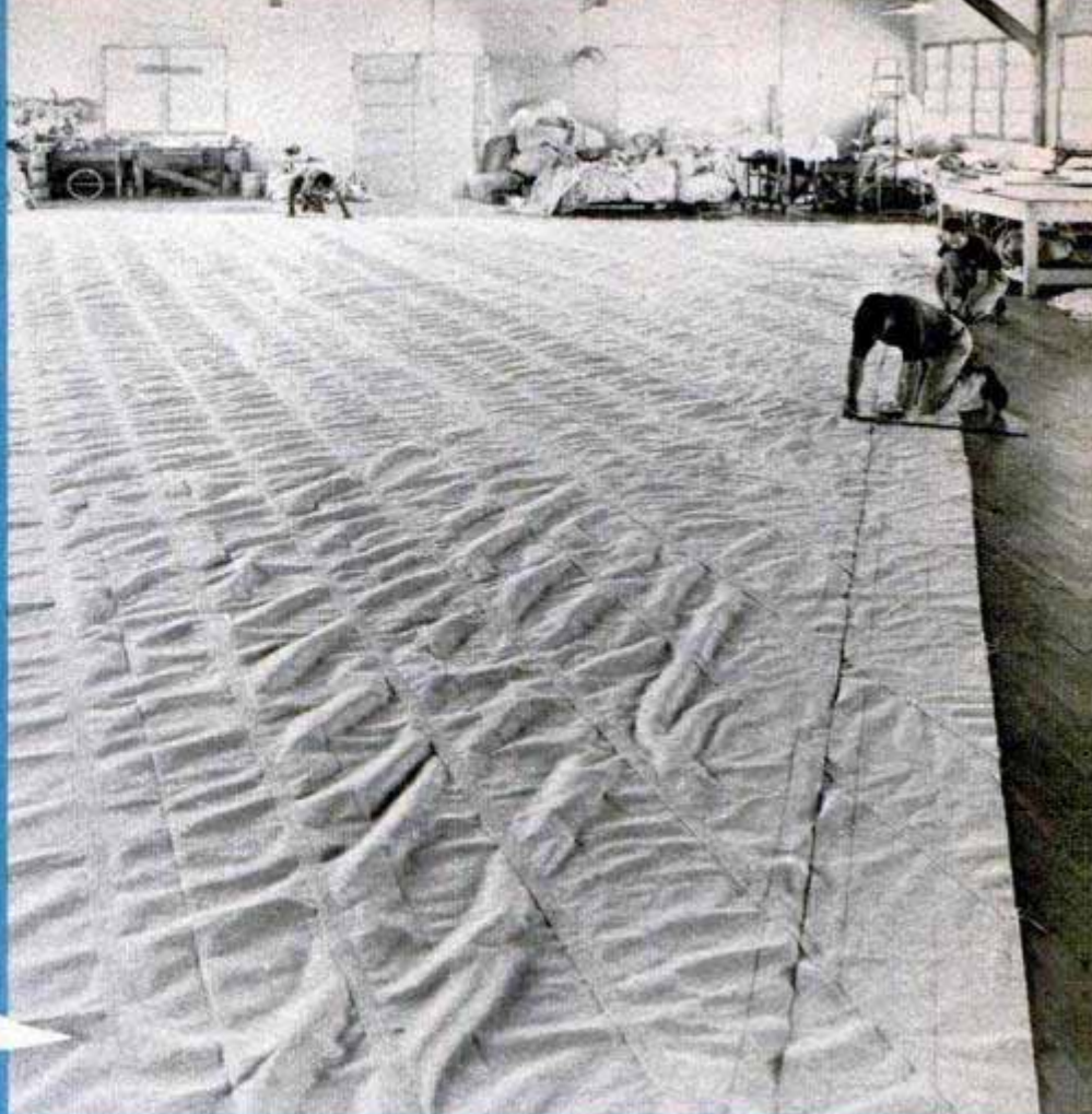
Corners and head of the sail are reinforced by patches. Here a corner is being measured and the patch cut to fit. Right, when sail is sewed it is laid out on floor of sail loft
