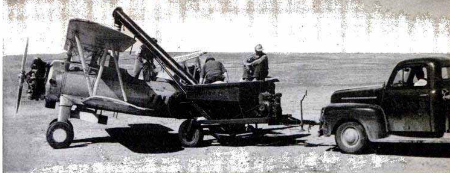
Rig moves wheat seed to the hopper of a plane. Seed is sown in broad swaths from altitude of 25 feet
