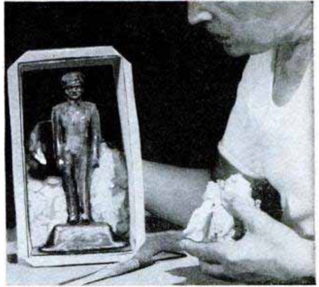
The cured mold, mounted on glass base, is shown in casting box as the clay dam is built up. When back half of mold is filled with clay, plaster will be poured into front half to make first section of shell
