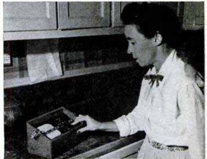
Controlling unit mounts "listening" and "speaking" switch. Unit at other end is equipped with buzzer
