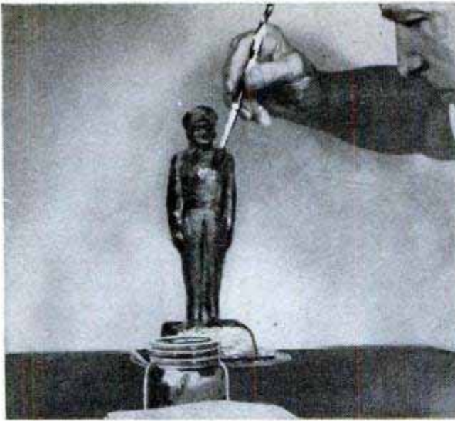
Liquid rubber is brushed over carved figure to form the rubber mold. From 10 to 15 coats are needed to complete the mold. Cheesecloth is embedded in rubber to strengthen the mold and prevent buckling
