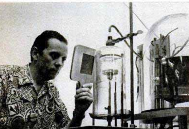
Engineer watches heating coil as it is used to silver-braze titanium parts inside a helium-filled jar
