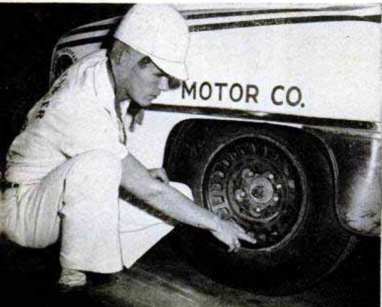
Air scoops on the wheels helped to keep brakes cool
