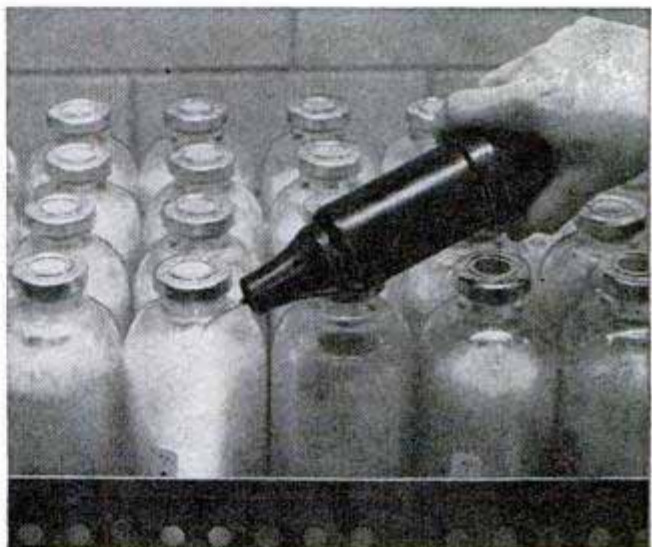
Dried plasma sealed under vacuum is tested for any leaks with spark producer. Purple glow means okay
