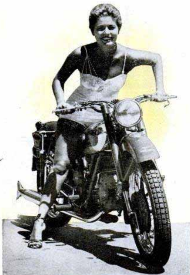
Italy's best-known motorcycle in this country is the Guzzi. It has a horizontal 500-cubic-centimeter engine
