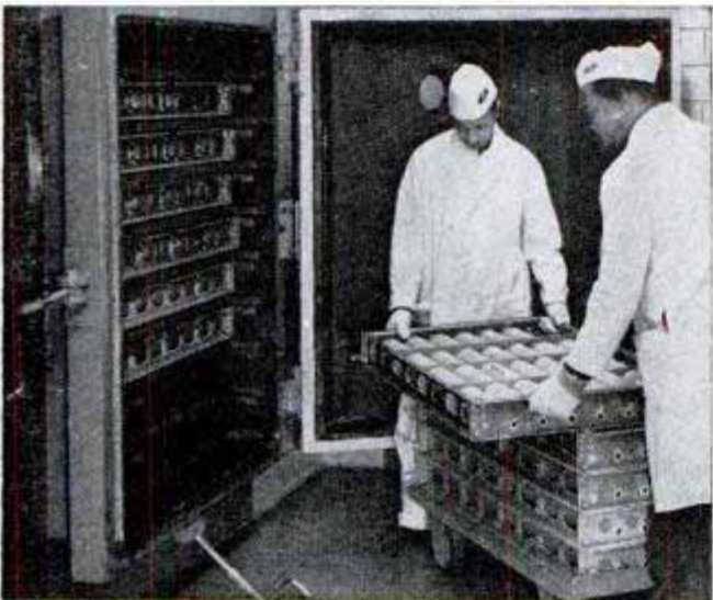
Trays of frozen plasma are rolled into a high-vacuum oven where the fluid is reduced to a dry powder
