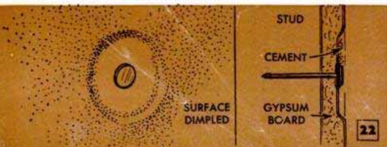
Nails not covered by joint treatment are sunk by dimpling board surface and then cementing over them
