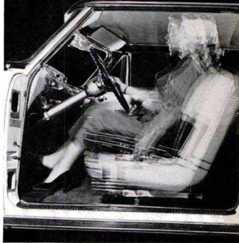
LINCOLN front seats move up and down as well as forward and backward. Electric motors do the work!
