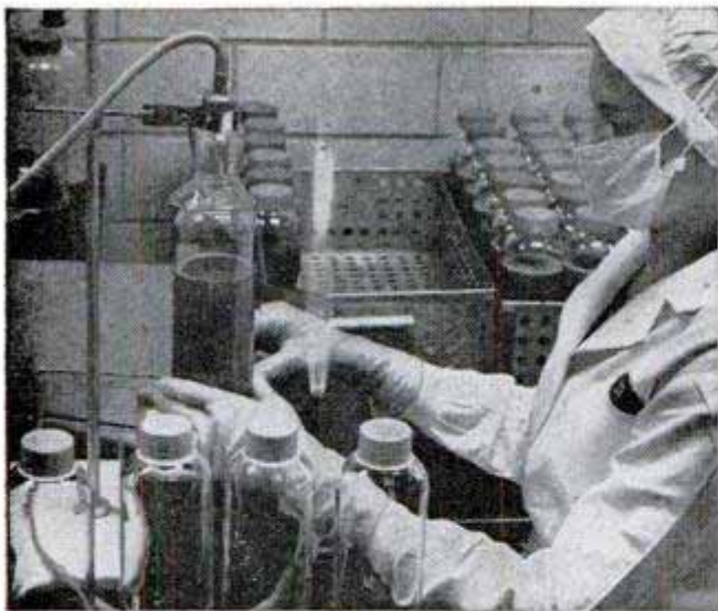
After ultraviolet-ray bath, the irradiated plasma is fed into its final container under high pressure
