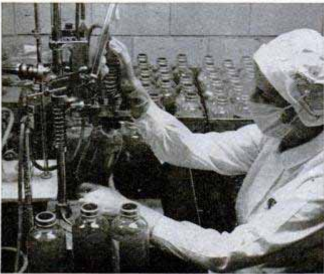
Plasma is drawn off by vacuum from individual donor bottles and is fed into large "pools" or tanks
