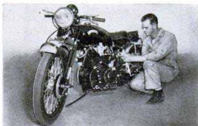
One of world's fastest is the 61-cubic-inch British Vincent. It has no frame below and ahead of engine
