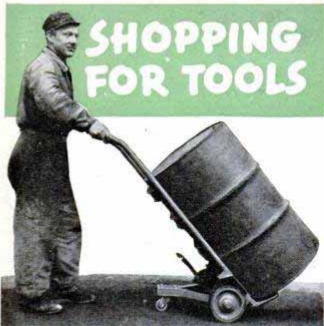
TRAILING CASTER on warehouse truck supports part of the load and permits operator to release handles of the truck which remains in traveling position. Caster frame is sprung to the truck frame and pivots on axle
