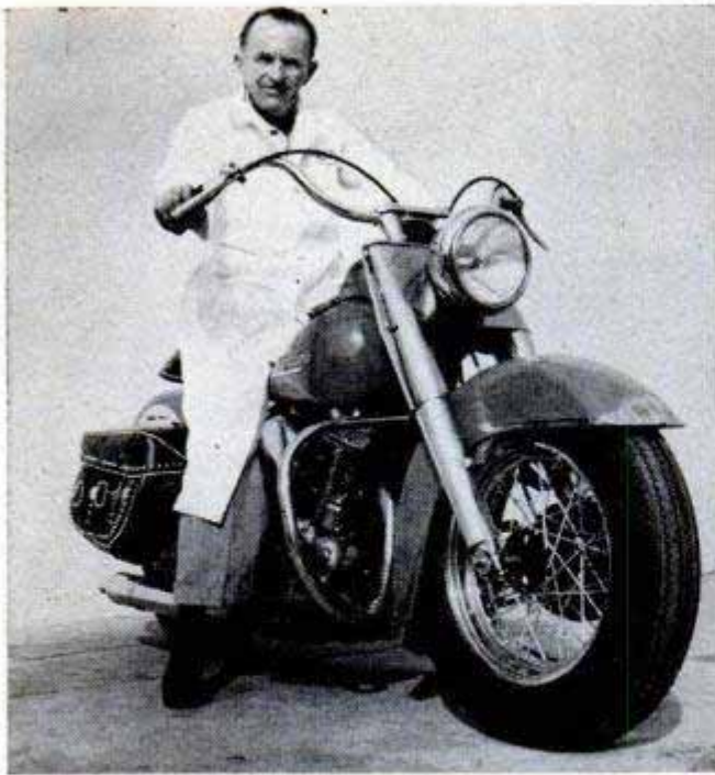
Front view of the Harley-Davidson Big Twin. Note the massive fork that contains springs for smooth riding
