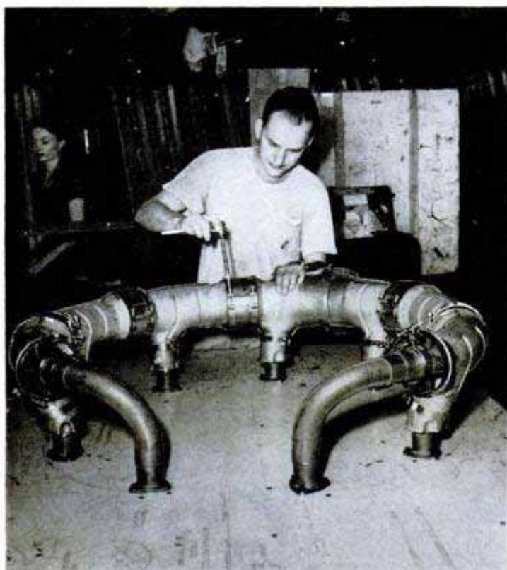
Airplane-engine exhaust system is given a titanium shroud that serves as a heat shield to protect other engine parts
