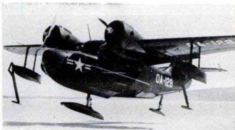
Above, JRF-5 hydro-ski test plane has single ski on a fixed strut below hull. This plane was tested for multibase operations and additional skis were added (below) for use on snow and ice. The ice tests were too rough on the airplane
