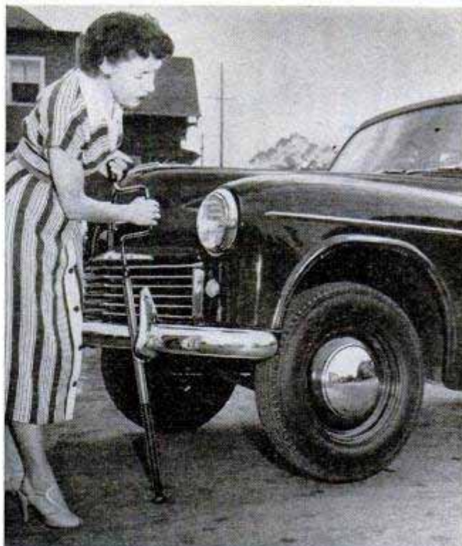
Tire changing on a Minx is easy. The light car is easy to raise and the jack fits in a slipproof socket
