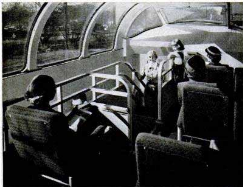
Center aisle stretches the full length of spacious dome car with stairways at either end. The curved-glass window sections are five feet high. Seats have lower backs than the ordinary coach seats for better forward visibility and are nonreclining type
