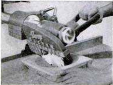
As Ball Bearing Circle Saw Mitres, compound mitres, cross-cuts, dados, rips, cups, grooves. 8" blade, 2 3/16" cut.
