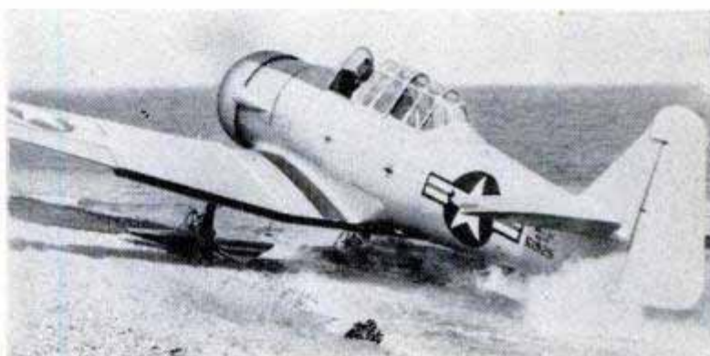
SNJ used in tests is equipped with ski gear and wheels. Here the plane has taxied out of the water for take-off from beach
