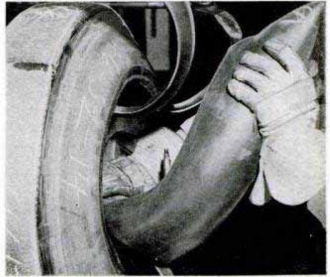
Prior to putting the casing in the mold, a vulcanizing inner tube is inserted in it. Care must be taken to see that the tube and the mold are the correct size for the tire. Otherwise buckling may occur
