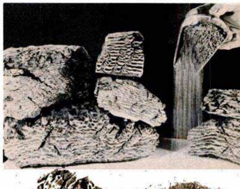
Left, a six-inch ruler indicates percentage of bark on a small fir. Thick cork layers in chunks of Douglas-fir bark, right, are evident as light-colored bands. Needlelike fibers and fine bark powder are being poured
