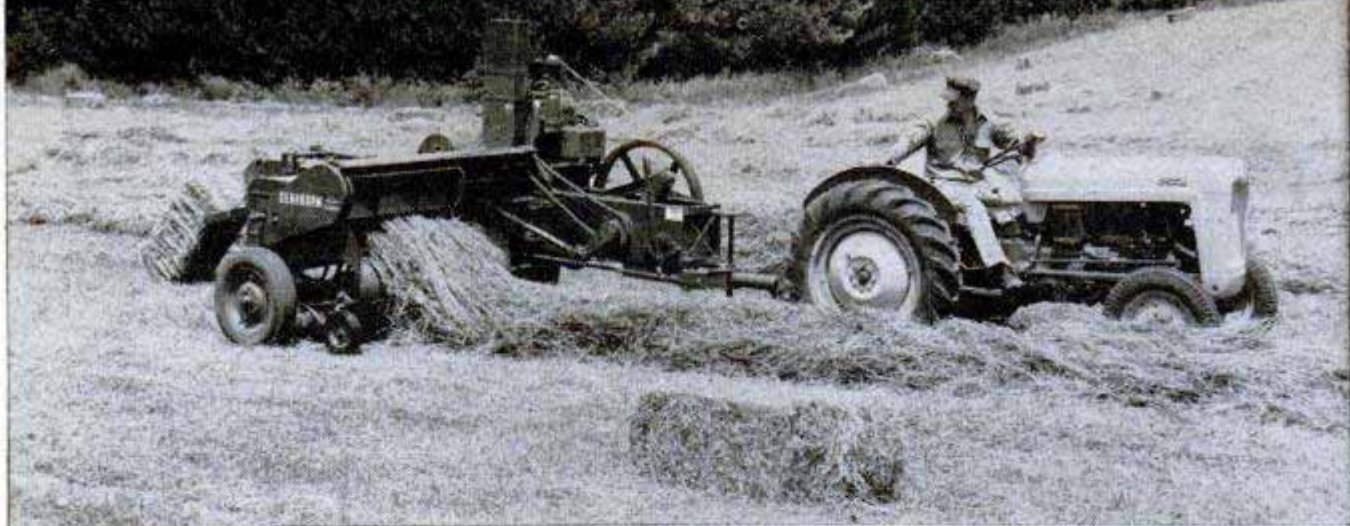
Streamlined tractor pulls the new hay baler, which will turn out three to eight bales per minute
