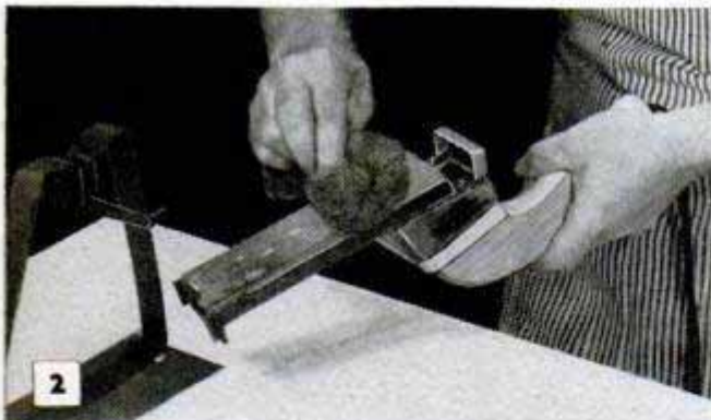
Electric paint peeler, above, shown with scraper mounted in front to permit working up to shoulders. Scouring of heating element with steel wool, center, removes paint accumulations. Rear scraper, bottom, is quicker and allows continuous forward scraping
