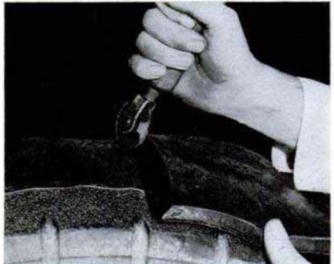
The camelback or tread rubber is stitched down with a roller as it is applied to the prepared casing. Cement has been previously put on with a stippling action which works it down into roughened surface
