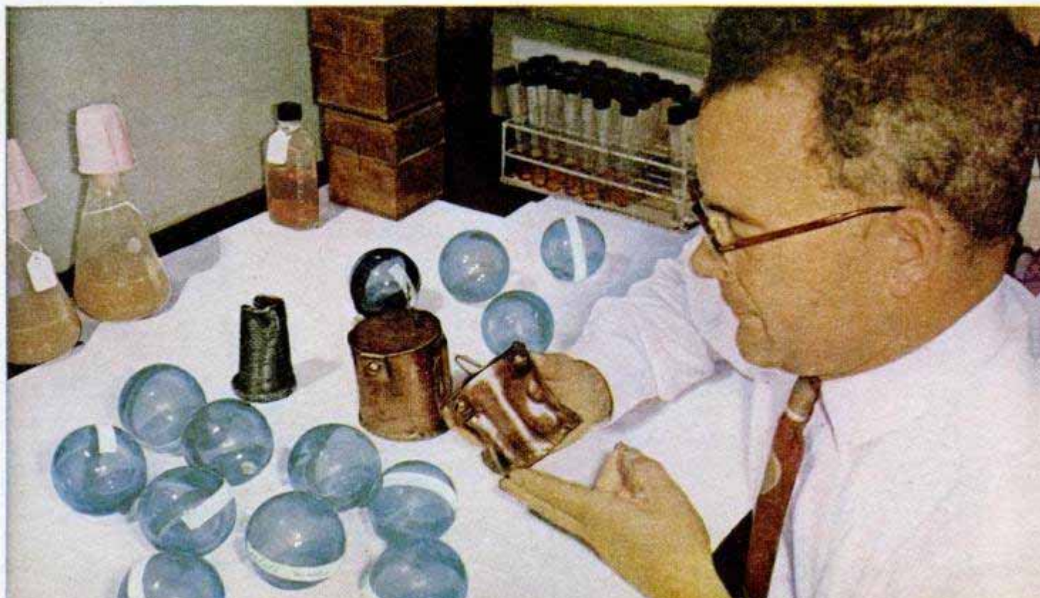
Professor ZoBell examines copper vessel dented by pressure at great depth; glass balls fit in containers
