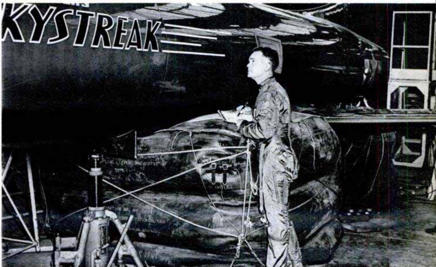
Heinemann and A. M. Mayo, right, chief of equipment design, inspect arrangements in a mockup. During vibration tests, plane below rests on inflated bags to simulate free flight
