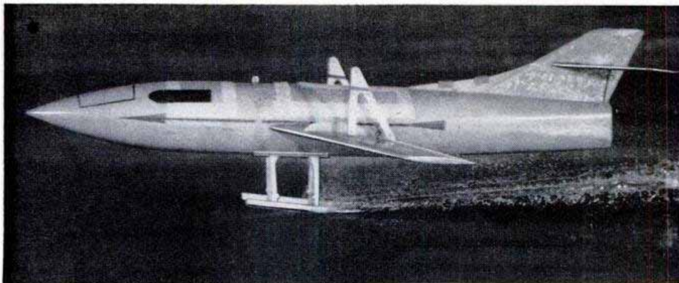
First hydro-ski tests were made by the NACA on this modified D-558 model and proved that the water skis were practical for high speed and could be retracted. Model is shown coming in for landing on its skis
