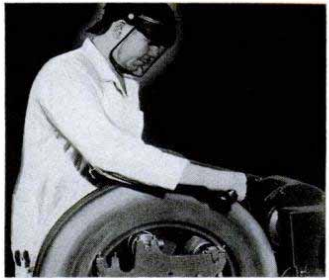
The outer surface of the casing is cleaned and roughened with a special rasp as the next step in the re-treading process. Careful preparation is essential for a job that will stand up satisfactorily in use
