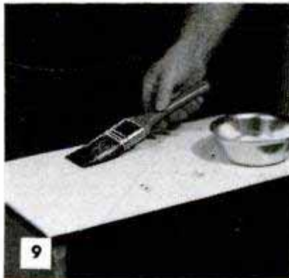
Left, apply remover with flat side of brush, but do not brush out. Right, let work stand until soft, then apply second coat if needed
