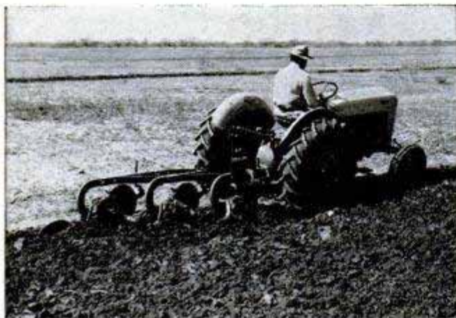
Four-cylinder engine produces ample power to operate three-bottom plows in many types of soils. At end of the field or over grass strips the live-action hydraulic system will quickly lift the implements
