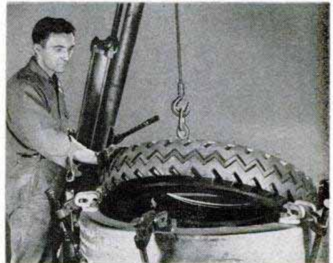
Fleet operators have found that a tire with a good casing can be recapped several times, and that the recapped tires match the service and performance of new casings. Operational costs thus can be cut sharply
