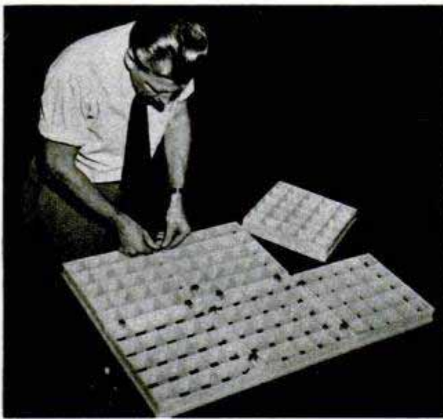
Clamping the plastic squares together is easily accomplished with a slight press on the small clips
