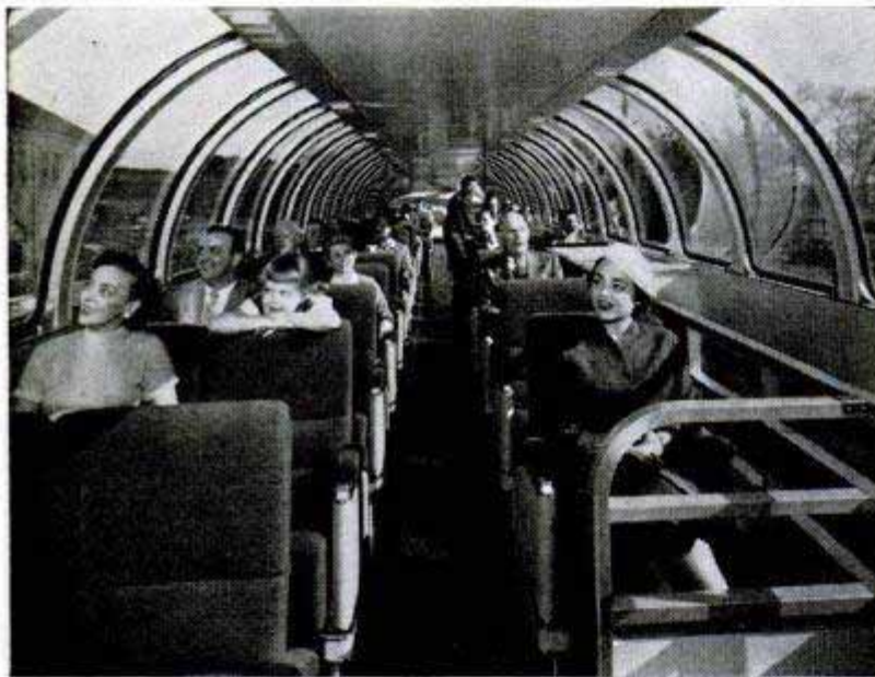
Center aisle stretches the full length of spacious dome car with stairways at either end. The curved-glass window sections are five feet high. Seats have lower backs than the ordinary coach seats for better forward visibility and are nonreclining type
