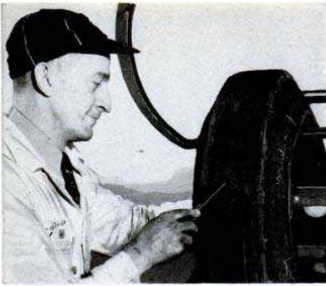
Prior to recapping, tire man removes all foreign matter from casing with a bradawl. Tacks and small nails which will eventually lead to punctures and slow leaks are frequently found embedded in casing
