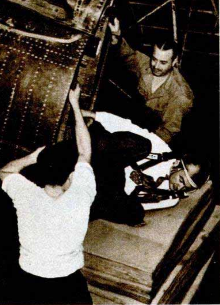
Engineers test pilot's means of leaving demountable nose of the Skyrocket in a simulated emergency escape
