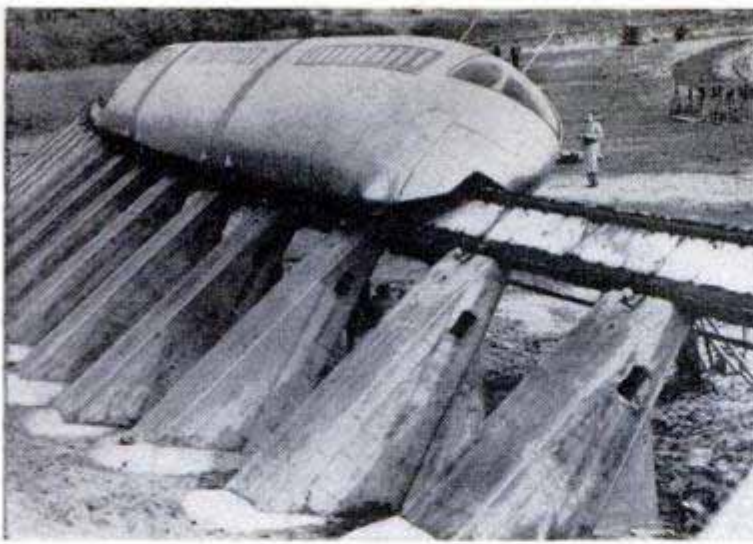
Racing at high speed, test train takes a curve which would normally demand slowing to 18 miles per hour. Switch consists of huge concrete platform containing two sections of rail which is turned by electric motors
