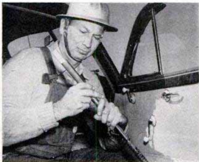
As the instrument is lowered a counter registers its depth. Below, inserting the temperature chart
