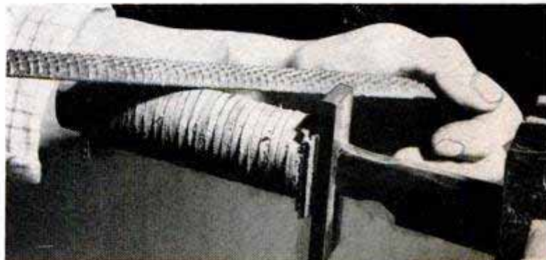
Leather handle is roughed out with a coarse rasp and the hilt and butt piece are filed to the rough shape. Finish with emery wheel and a stitched buff
