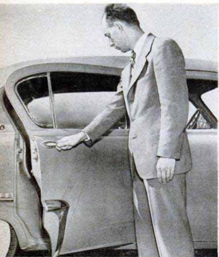
Above, the rear door of the '53 Plymouth is much wider at the top so a back-seat passenger can see out without leaning forward—a real innovation
