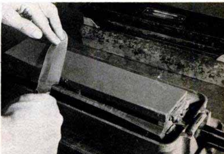
Above, the rough and finished handles of the all-purpose knife. Below, honing the blade by hand on a three-part professional-type hone. Note blade angle
