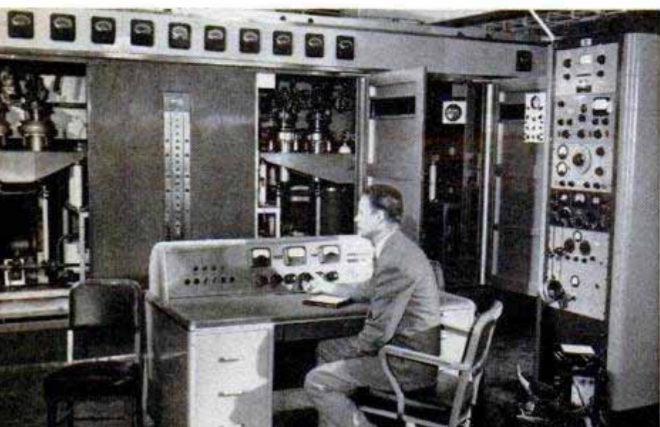
Engineer in main control room on Courier faces water-cooled tubes
