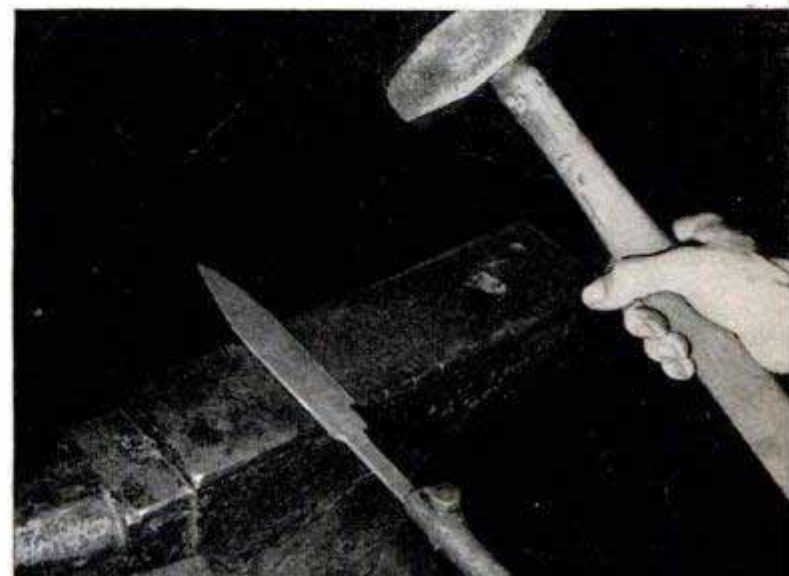
Above, one of the first steps in making a knife is heating the blank in a blacksmith's forge. Below, after heating, the blank is hammer-forged on an anvil to draw the blade to the rough form for grinding
