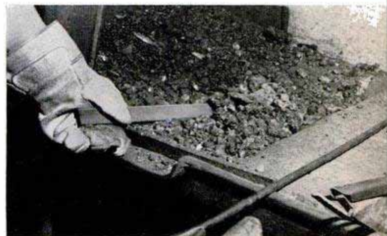
Above, one of the first steps in making a knife is heating the blank in a blacksmith's forge. Below, after heating, the blank is hammer-forged on an anvil to draw the blade to the rough form for grinding
