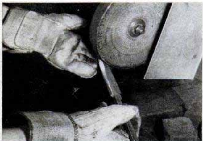
Above, rough-grinding the blank on a coarse emery wheel. Below, polishing blade on stitched cloth buff
