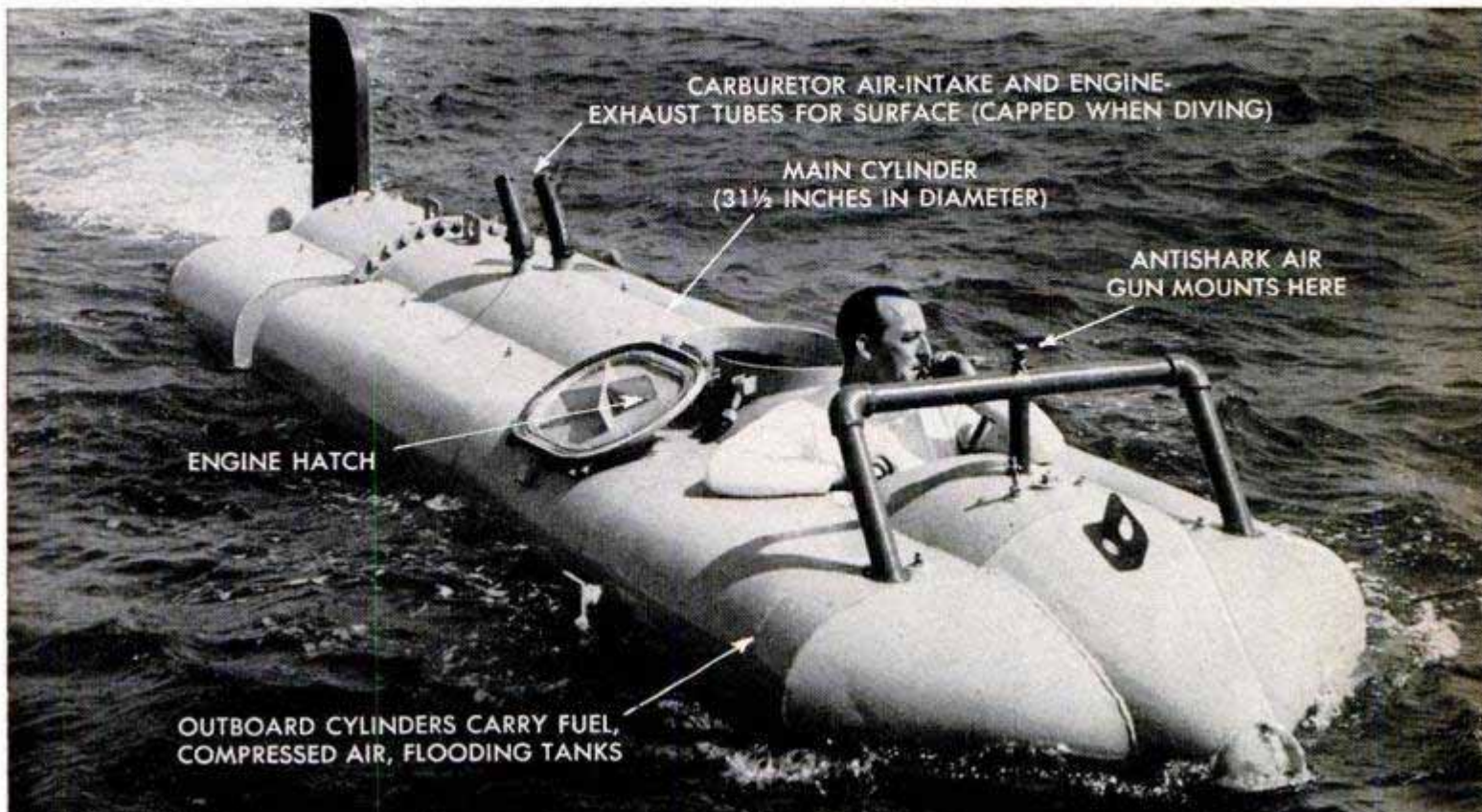
Sub operator rides in an open cockpit containing steering wheel, engine controls, air and water valves
