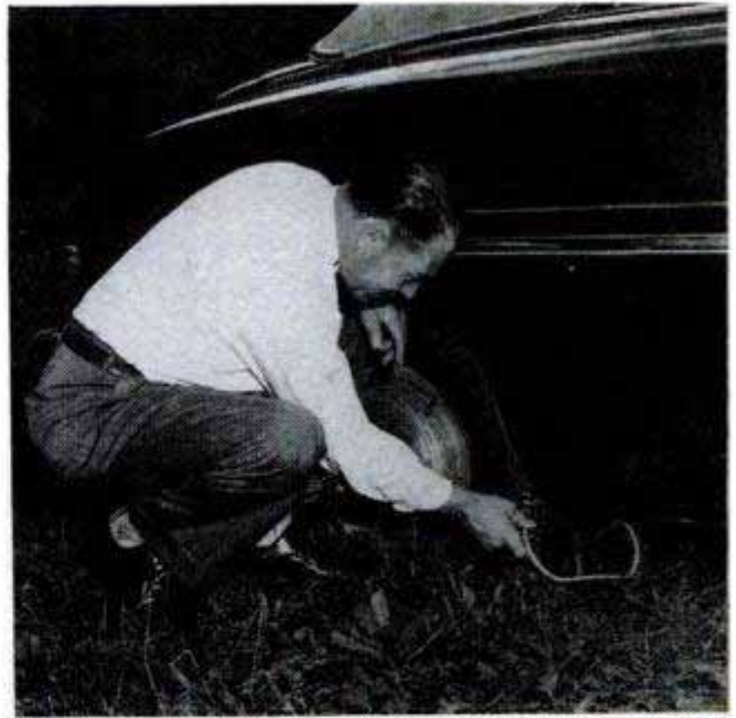
Traction tire clamp, easily placed on wheel after car is stuck, enables automobile to work itself free
