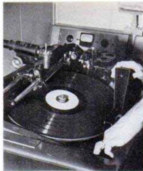
On board Courier , turntable for recordings stays level even when the ship rolls
