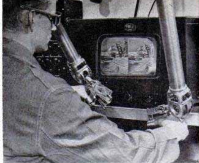
Samples of plant life are taken, left, to determine radiation in vicinity of tests. With three-dimensional television, right, dangerous experiments can be conducted remotely thanks to accurate depth perception
