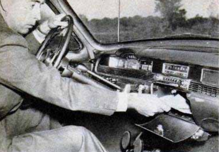
Driver convenience has been improved by mounting the glove compartment in the center of the dashboard
