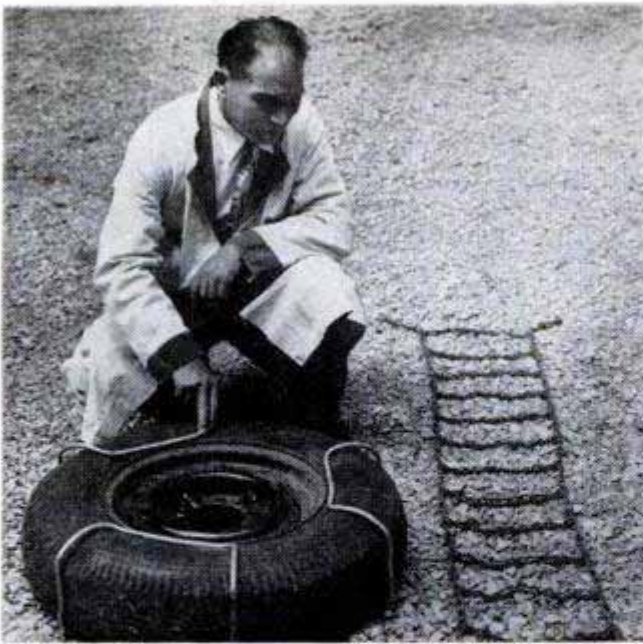
Simple tire clamps may replace conventional chains as standard equipment. Only one is needed per tire
