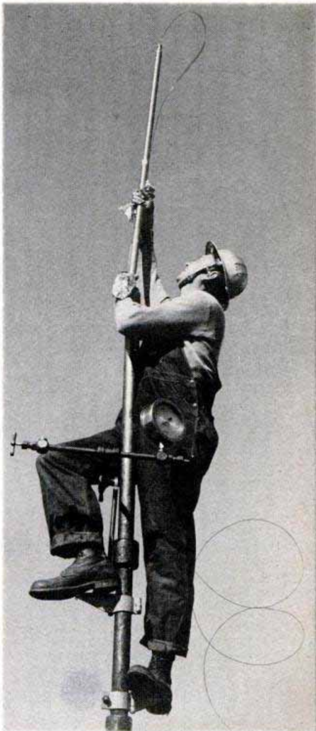
Putting thermometer into a bore. Below, up from the depths, metal strip is a record of well's temperature
