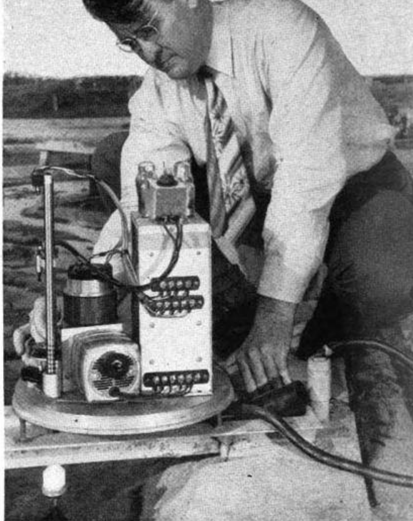
One of many instruments that measure the height of water at various points along the rivers and relay this information to recorders in the control houses
