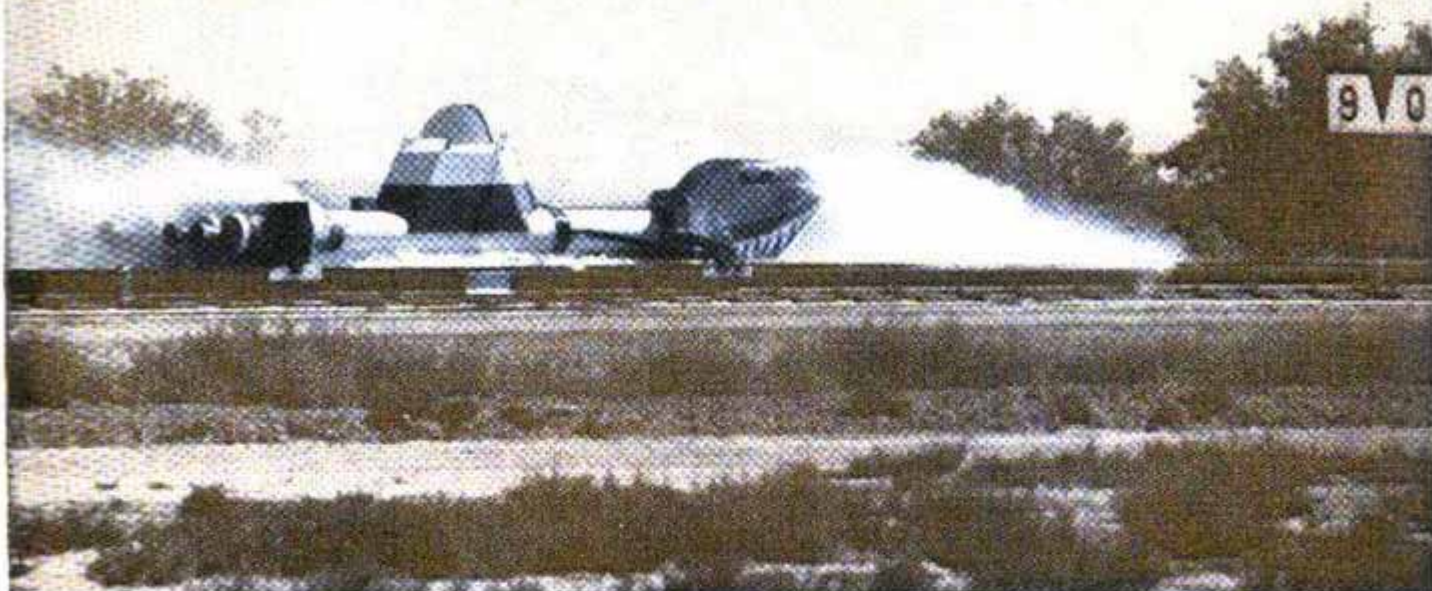
Small sprays of water are still shooting out ahead of a rocket sled just before it comes to a full stop. Water in the trough between the rails, entering an orifice under the head of the vehicle, supplies braking power
