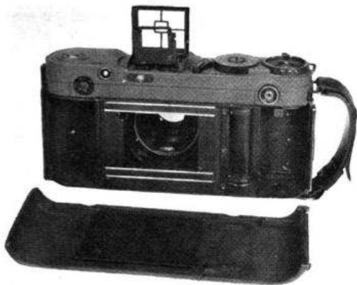
Chassis of new combat camera, left, is easily accessible. Right, plunger at top slices off needed exposures
