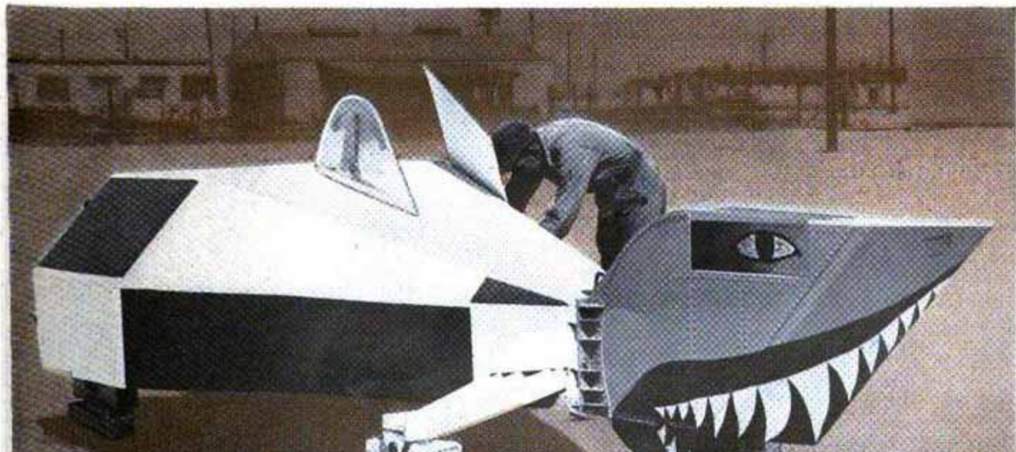
Bug-like high-speed sled uses slippers instead of wheels to remain on rails along which it travels at speeds of up to 1000 miles an hour. Here a technician is installing a radiotelemetering unit inside the body
