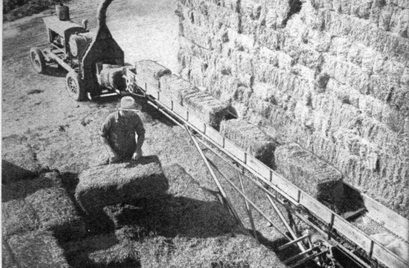
Hay elevator has been rigged so it can be flipped over and run downhill to feed bales into the chopper
