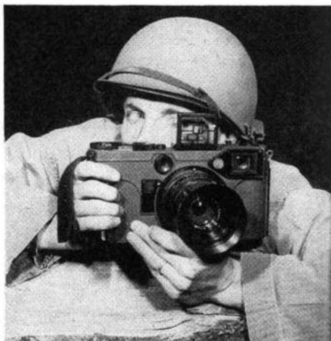
When no film remains, a red flag automatically pops into the combined view-finder-range-finder peephole
