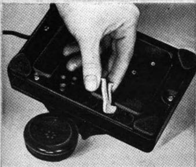
RING HUSHER inserted in "bell-in-set" telephones quiets the sound to stage as low as a gentle purr
