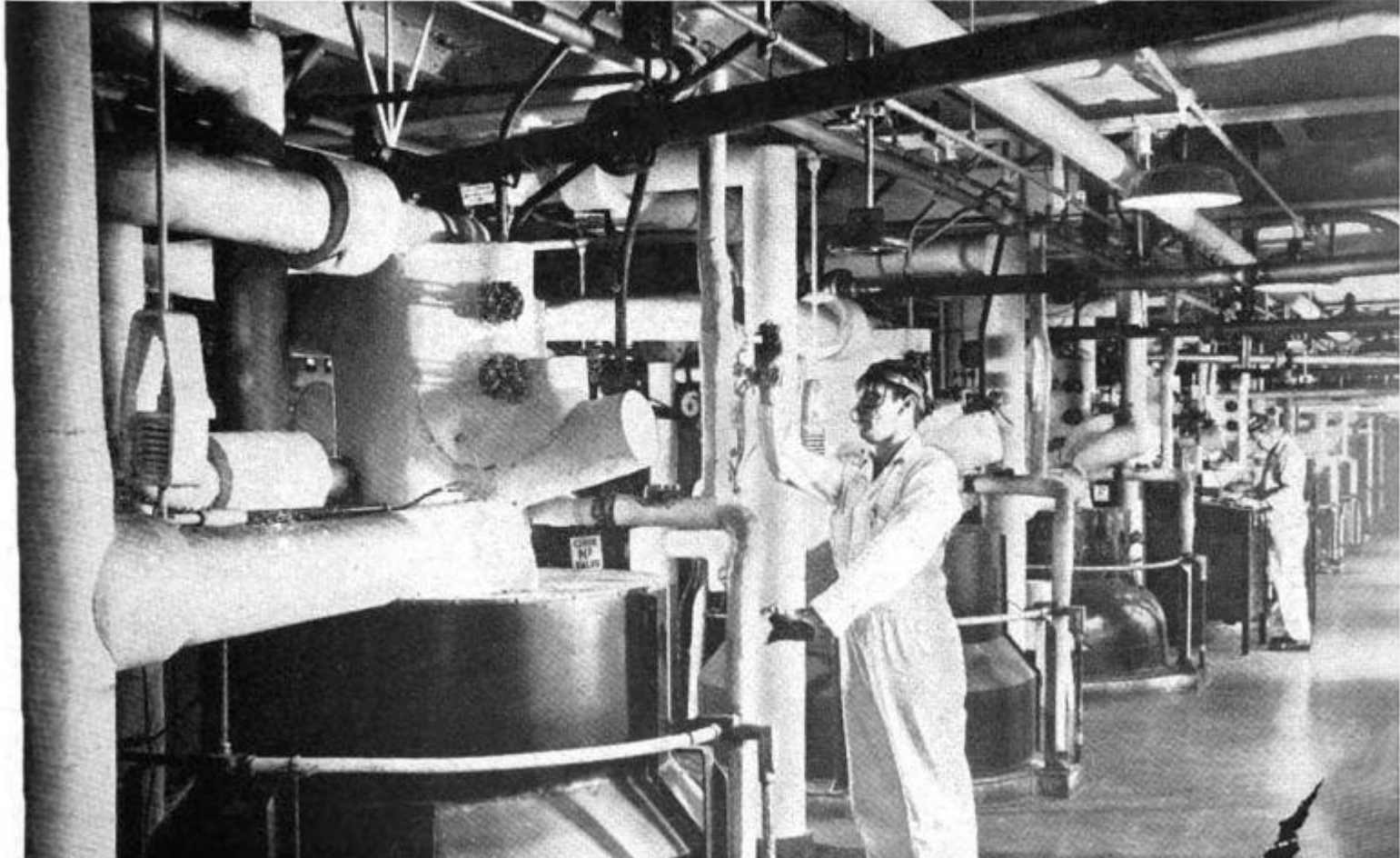
These machines are autoclaves in Du Pont nylon plant where small molecules are joined to make large ones
