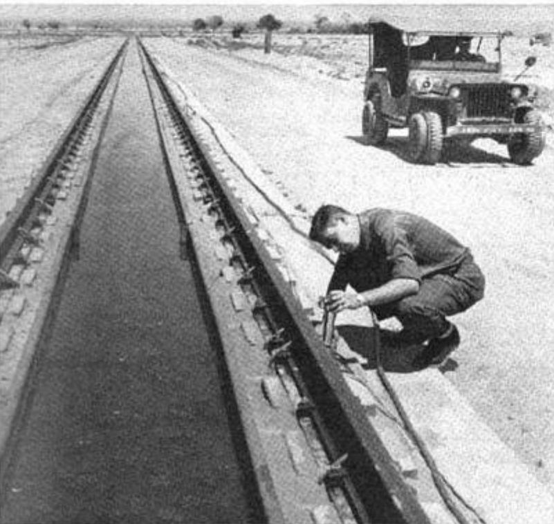
Closeup of water-filled trough in the braking area. A worker is examining one of the electrical trippers along rail by which speed of the sled is measured
