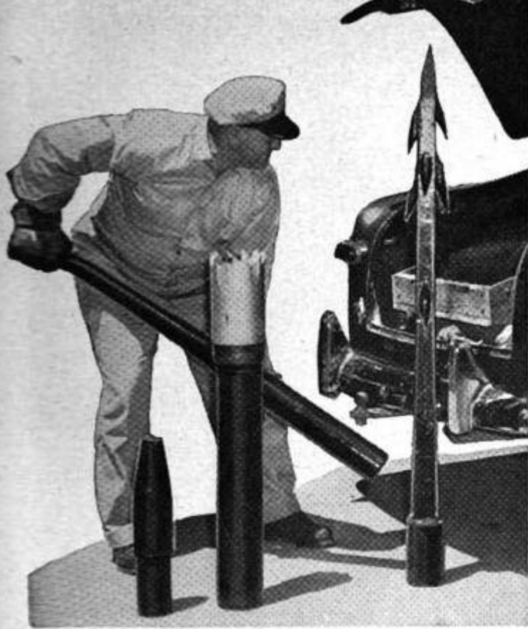
Fishing tools — a short mill for grinding objects; center, "junk basket" for scooping, and spear for seizing and lifting. A taper tap is being loaded
