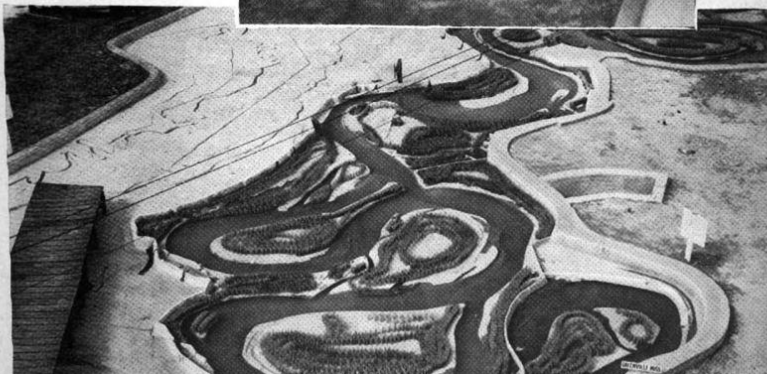
Below, model of Mississippi at Greenville, Miss., shows how it meanders. Present channel (it runs almost straight down the center of picture) is only 30 miles long; 20 years ago, the channel meandered for 58 miles
