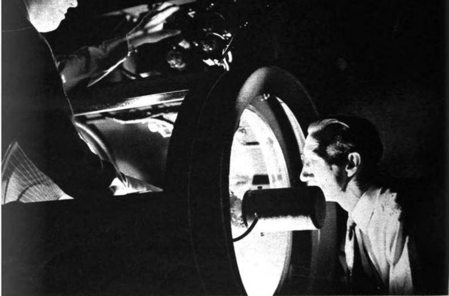
Inspecting the 80,000-volt connections to the projection kinescope tube for possible high-voltage arcing
