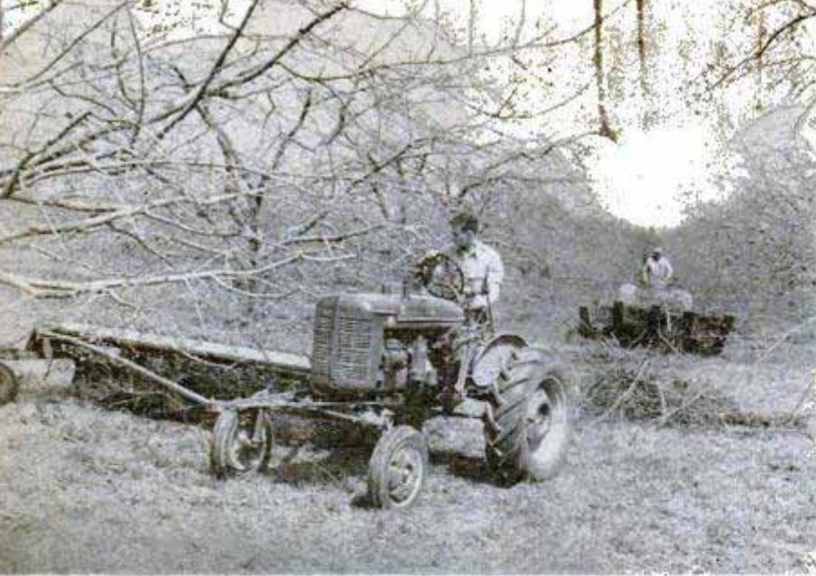
Cross-braced to the tractor, an old hayrake is put to work gathering brush after orchard pruning. The rake's 10-foot reach gathers brush under tree limbs as the driver circles and a second tractor scoops it up and carries it to bonfire
