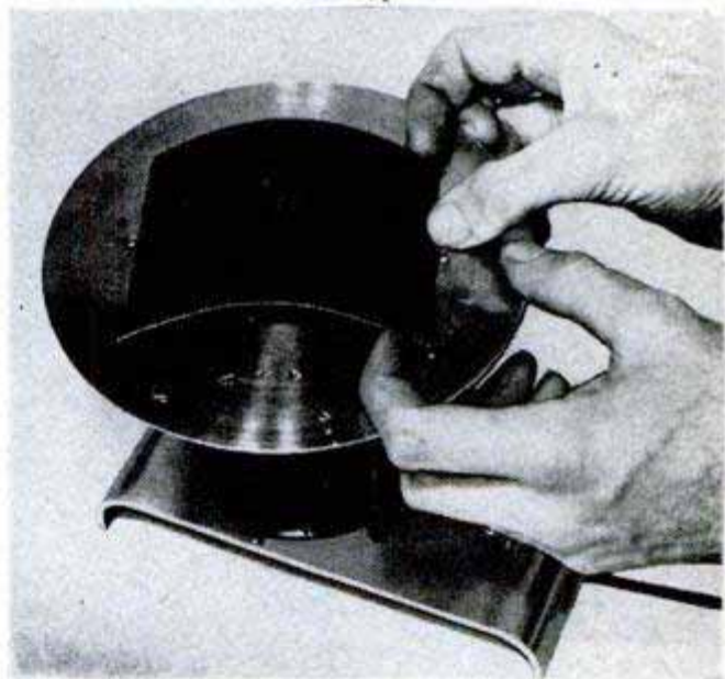
Negative is mounted on drying disk by inserting edges under heads of small machine screws. When drier is spinning, centrifugal force holds film against both screwheads in addition to throwing off water
