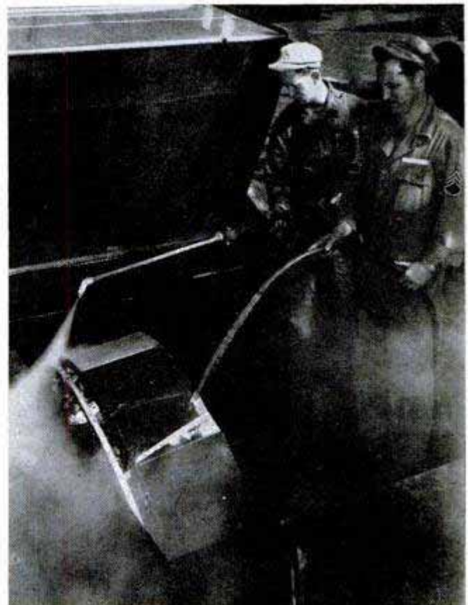
Water and steam being used on a B-29's engine cowling remove dirt and grease prior to paint-removal process that restores brightness to metal
