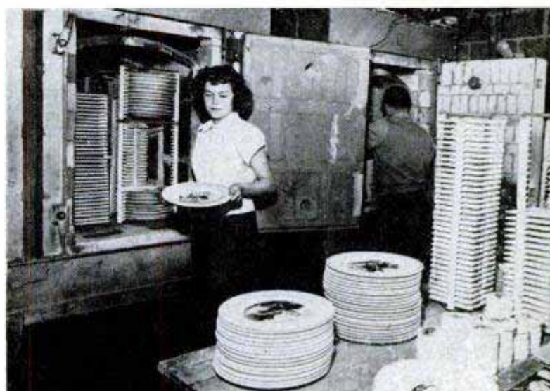
When gummed paper is dampened, design can be slipped off in its protecting film of lacquer and applied to the plate. Below, when plates are baked, colors seep down into the china
