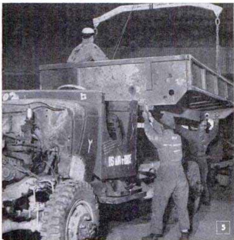
Typical of many vehicles requiring remanufacture is "junkie" above. Excessive damage ruled out the possibility of repair
