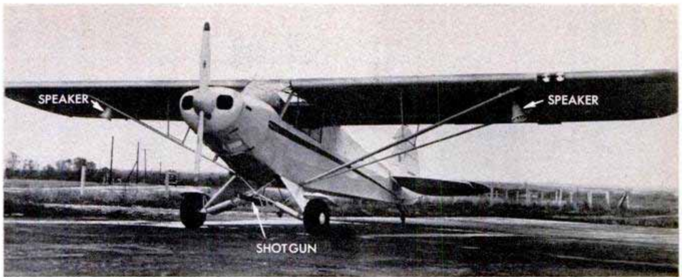
Loudspeakers located at wing struts enable rancher to relay instructions to cowboys during roundup operations. Automatically fired shotgun mounted on landing-gear V, right, is aimed by pointing plane
