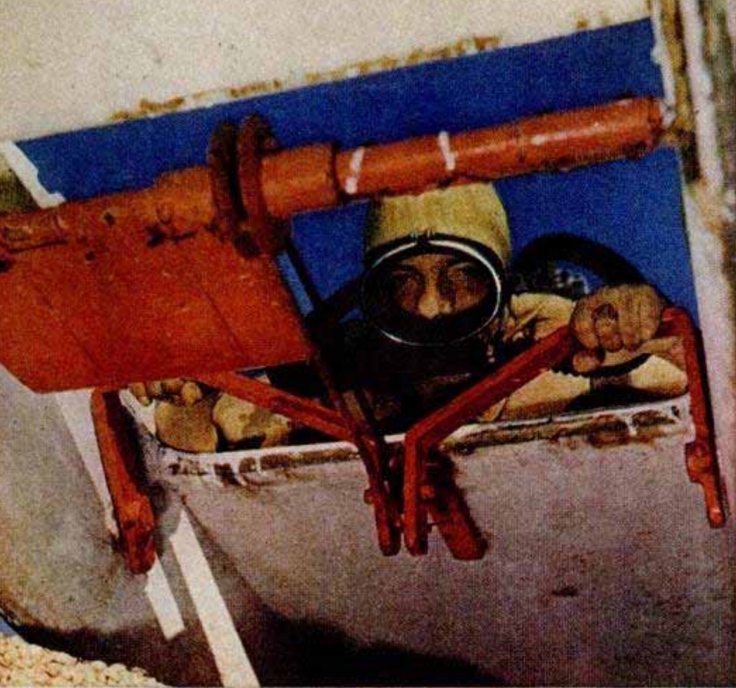
Goggled and helmeted, the prone pilot grips the controls that operate ailerons to make the wing dive or bank. One red aileron is seen at left
