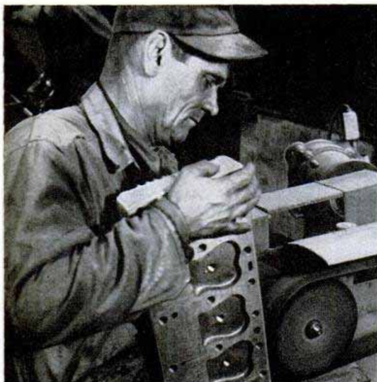
Above, aluminum-alloy manifold is carefully fitted into a jig to be drilled. Below, all Edmunds parts are thoroughly buffed and polished to improve appearance and increase heat transmission
