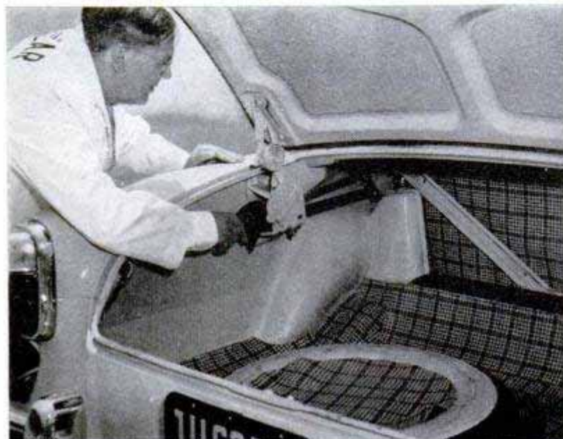
Above, sloping hood gives excellent vision ahead of car and permits driver to see both front fenders. Crash pad across the dashboard is too narrow for real protection, the report shows. Below, recessed spare tire is inconvenient when trunk is full
