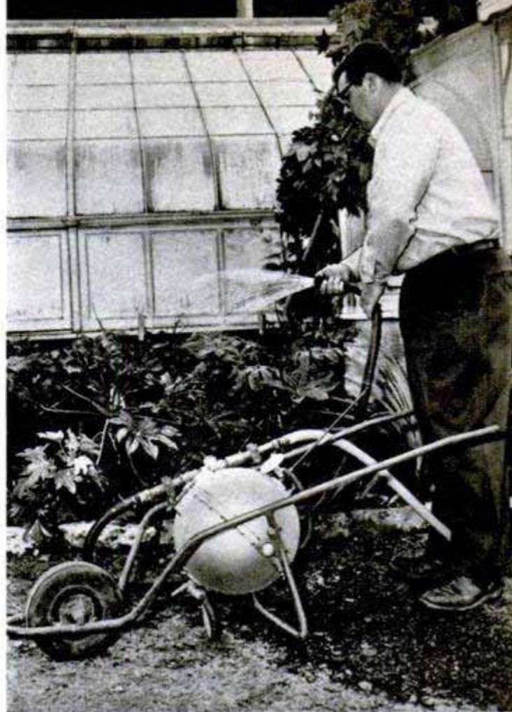
Proportioning dispenser mixes liquid fertilizer and insecticide with water flowing through garden hose
