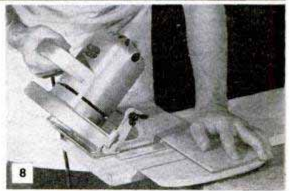
ANGLE CUTS can be made accurately with a special T-guide. Use separate notch on saw
