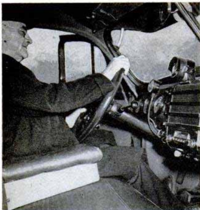
Special antifatigue car has solid armrests, chrome painted flat black, steering rim as big as ax handle
