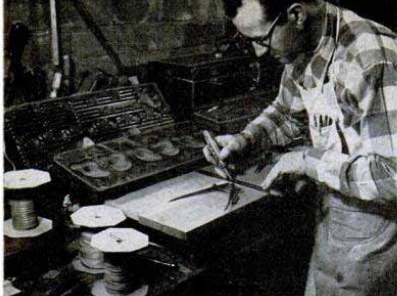
Patternmaker works on a new model for the Edmunds Nash cylinder head. Fluted head in background is the current modification
