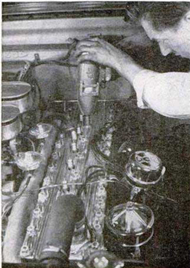
Mechanic tightens down an Edmunds cylinder head on a 1951 Packard engine. Fluting carries off more heat
