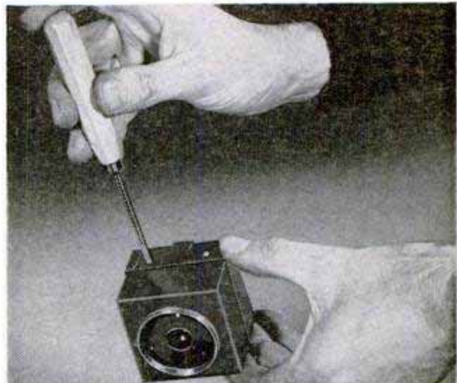
Above, tightening three machine screws locks parts in position. Shanks of screws engage slots in slide holder, as in upper detail. Below, clips bent from sheet metal and soldered to box hold slides in place
