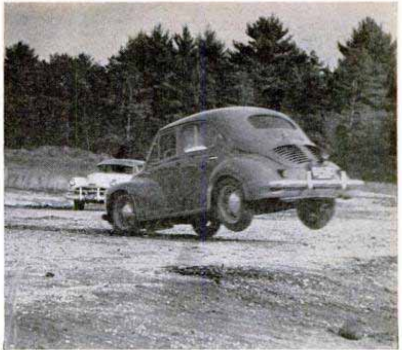
In a test at M.V.R. proving grounds, French Renault leaps across a ditch. On this particular car the front wheels didn't buckle
