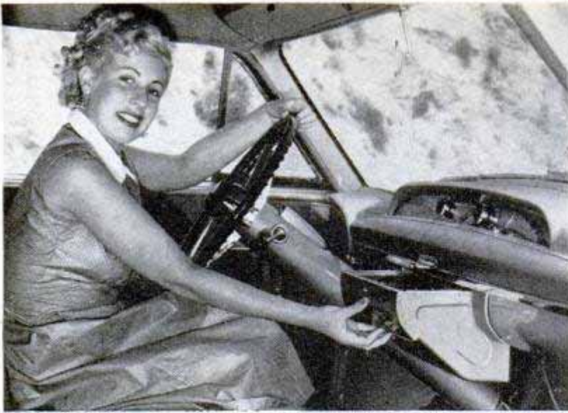
There is room plus accessibility in the sliding-drawer glove compartment mounted below the center of the new Nash dashboard
