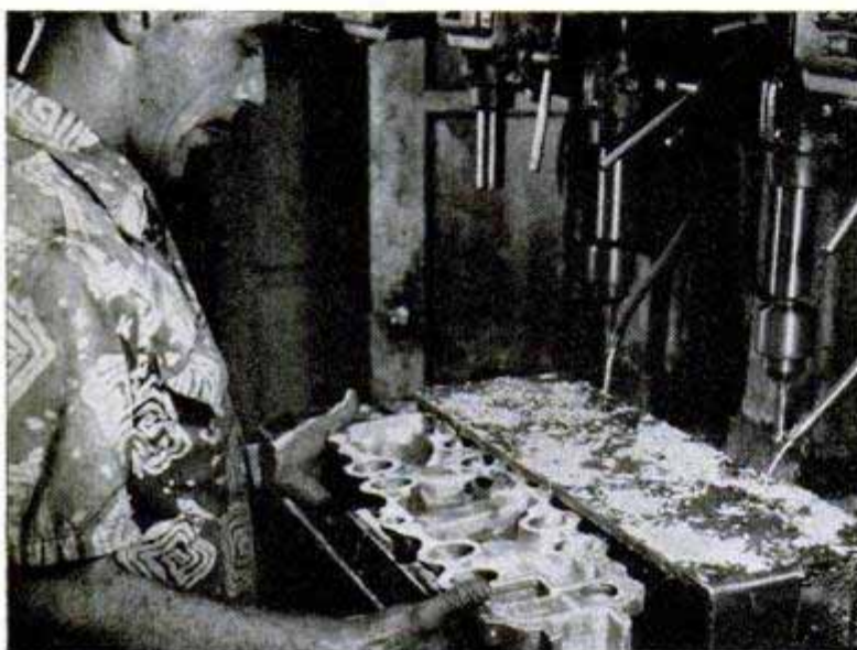
Above, aluminum-alloy manifold is carefully fitted into a jig to be drilled. Below, all Edmunds parts are thoroughly buffed and polished to improve appearance and increase heat transmission
