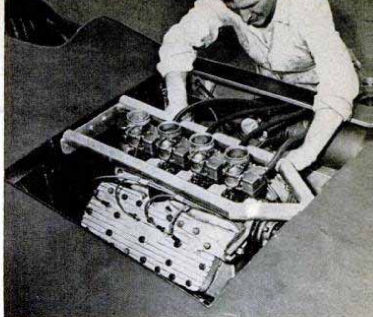
Full-race Mercury engine is used in some trials, but in unlimited competition, a Chrysler V-8 replaces it
