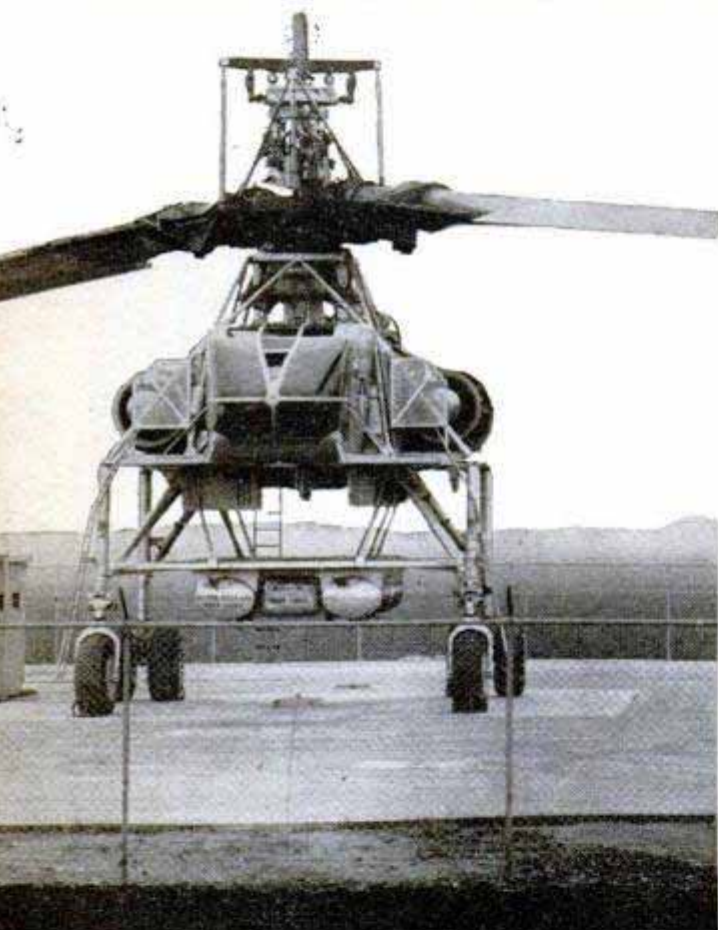
Air from compressors run by two turbojet engines is lifted up through the rotor shaft, above, and out to the rotor-blade tips. Fuel is burned at the exhaust outlets, providing a jet effect that turns the blades
