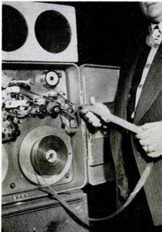
When viewed by the audience, the 1100 overlapping strips of the Cinerama screen look solid, but from an angle you can actually see through it. Below, the sounds are recorded by six tracks on a single tape
