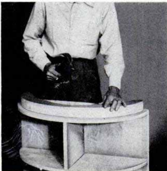
Above, compartment frontpiece is glued and nailed in place with brads. Heads are set below surface and holes filled. Below, after bandsawing to contour and applying facing, bottom frame is nailed to shelf
