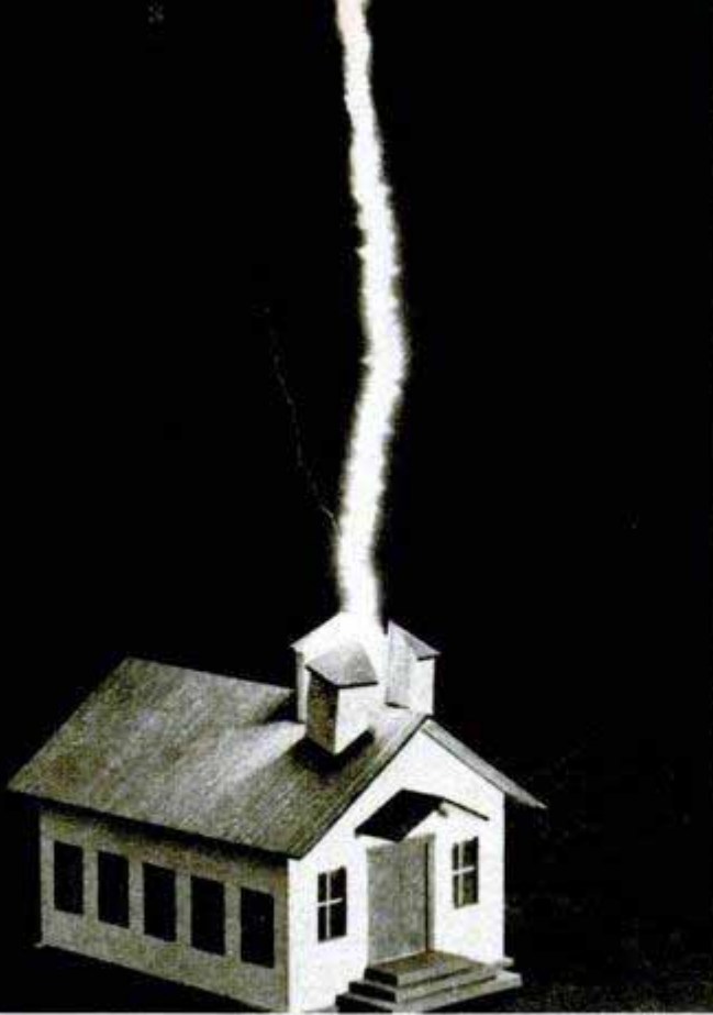
Ben Franklin invented the lightning rod about 200 years ago. Science now proves him right. Above, with no protection, tower on model splits open. Below, with it, the 2.4 million volts go harmlessly to ground
