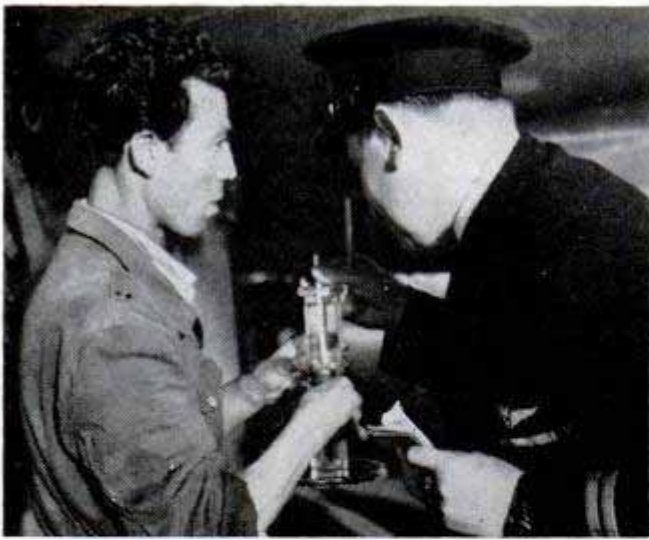
Measuring specific gravity of kerosene at Rome to determine accurate weight of fuel needed to Beirut
