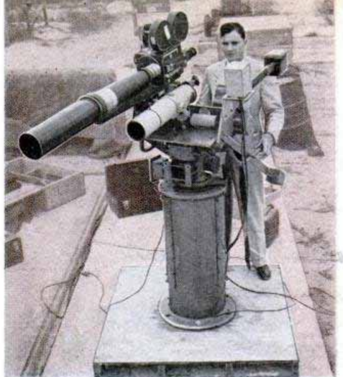
German-developed "Askania" camera simultaneously notes missile's trajectory, time of passage and speed
