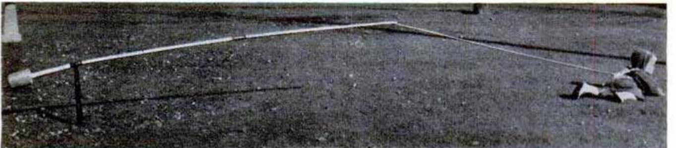
CHILD TETHER gives the youngster freedom of movement yet keeps him out of harm's way. He cannot become tangled in cord nor can he get close to the stake or counterweight. Cord remains gently tight at all times
