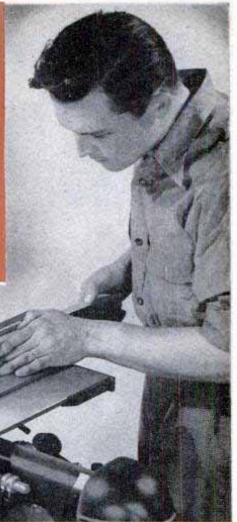
Stopblock shown clamped to the saw table stops each cut at precisely the same depth to form curved-bottom slot in the stock
