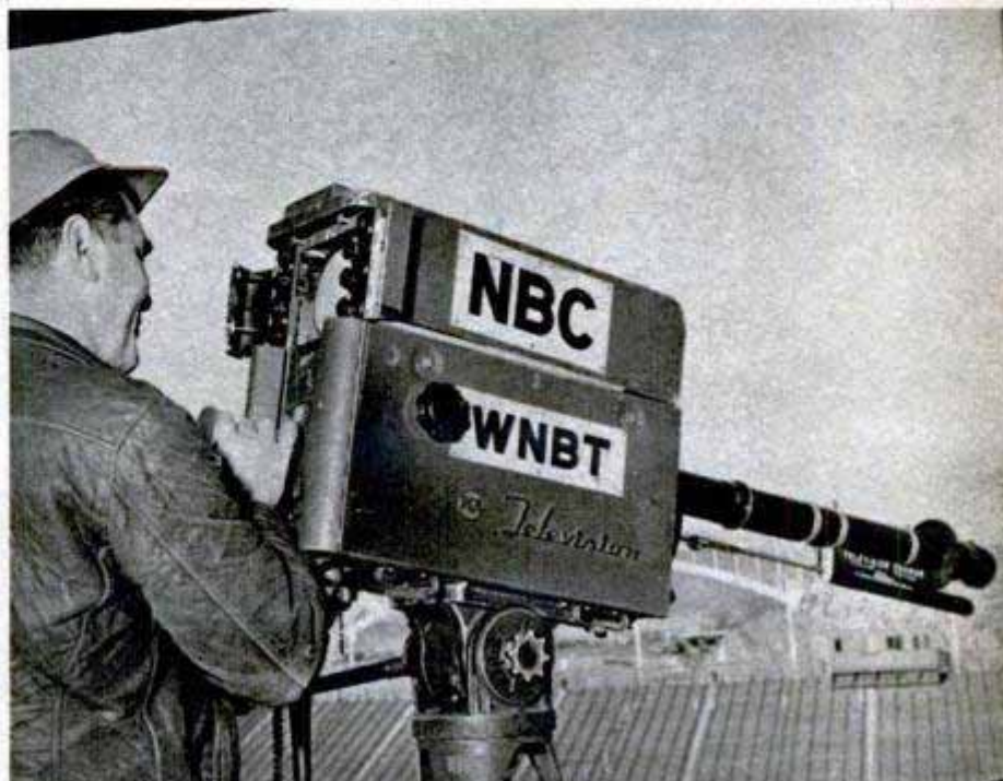
Mounted on a carrier's rotating mast, a TV dish antenna beams full view of mock war to armchair viewers. Below, three-foot "zoomar" lens brings in close-ups. When operator slides rod, lens stays in focus while picture moves in or farther away
