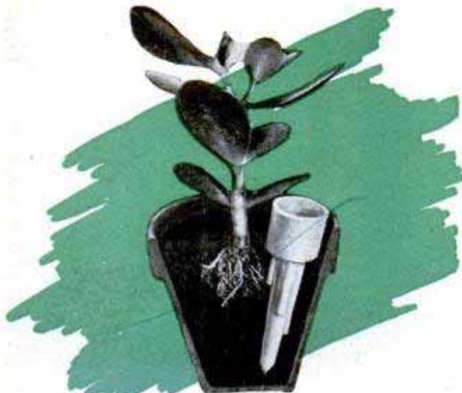
PLANT FEEDER directs water to roots of plant. Fertilizer is dissolved in water in cup on the top
