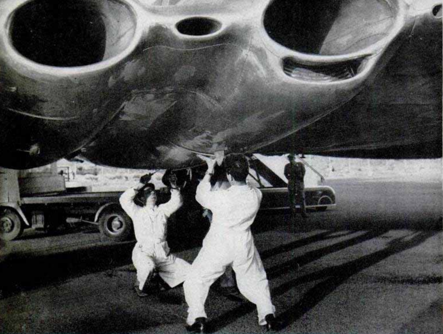
With propellerless jet craft, engines are nearer the ground and accessible for maintenance without platforms
