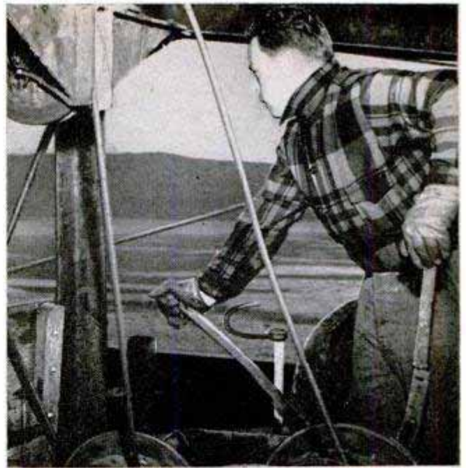
Big claw (shown on opposite page) is operated by an intricate system of levers and cables on the cutter
