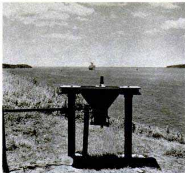
Metal baffle box of the beamed antenna is pointed straight out to sea. Box at rear houses the switch
