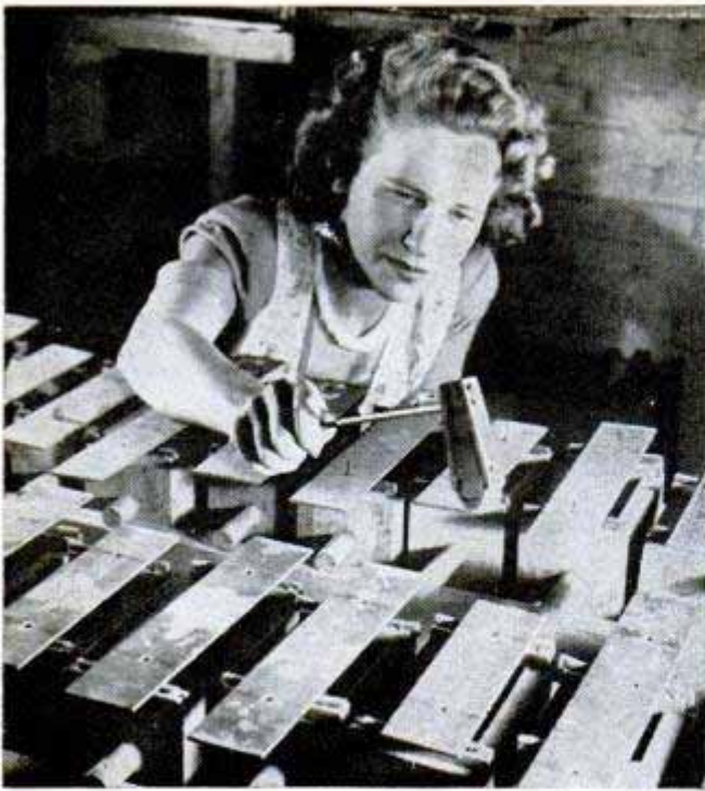
Wooden pipes are tested by a woman tuner in this manner. To provide the wide range of voices in the organ, both wooden and metal pipes have to be used
