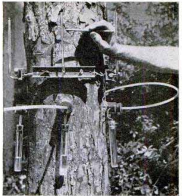
Left, pump in shelter at far left varies internal pressure of tree in experiments with ways to increase gum yield. Right, close-up of punch-hole taps. Top tubes show gum pressures; bottom tubes show flow volumes
