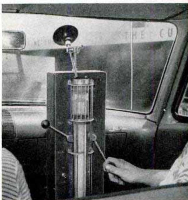
Above, special measuring device indicates specific fuel consumption over measured mile at given speed. Below, testing the Mercury over a rocky side road
