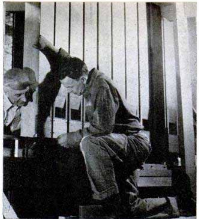
Woodworking is an important part of the organ-maker's art. These men are installing wooden pipes in organ for the final test of pitch, control and volume
