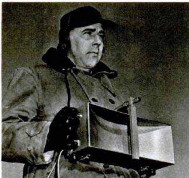
Crew member holds the receiver and positions it for the continuous signal heard when ship is on the beam
