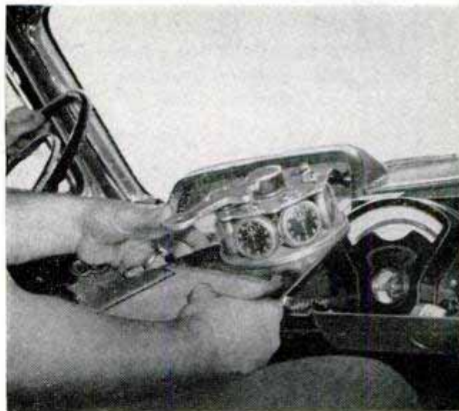
In making the acceleration test, left, Clymer used a barrage of seven stop watches, above, for accuracy
