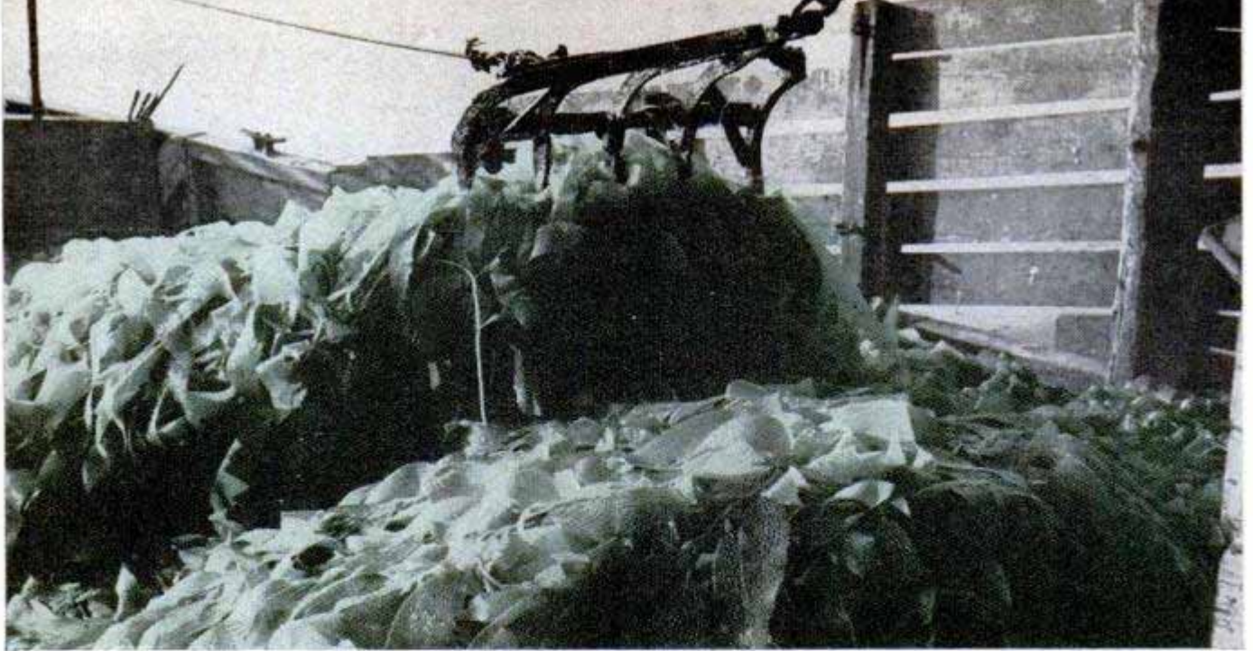
The giant claw in ship's hold easily moves a half ton of kelp with each swipe and reaches any part of hold
