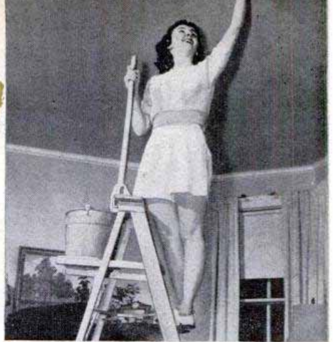
BALANCE BAR clamps to top of stepladder to provide a handgrip while you wash or paint the ceiling. With it, you can work near the ladder top in safety
