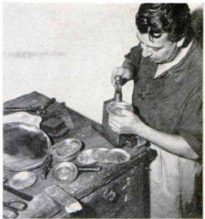
"Married metals" are made by routing a silver base, filling it with copper or bronze and hammering it
