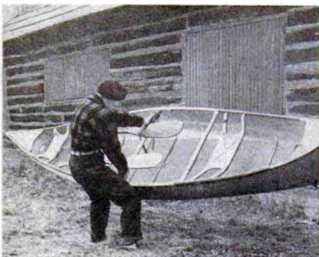
Above, once it has been tied in the correct position the tump-line need not be removed, as it does not interfere with placement of duffel or fishing gear in the mid-ship section of the canoe. Below, the first step in lifting an all-metal canoe into the carrying position
