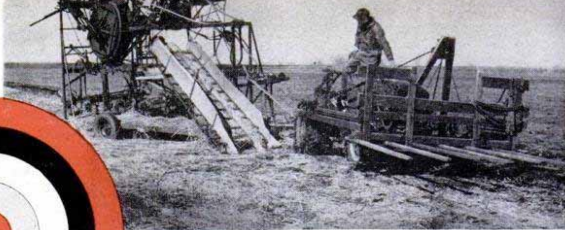
Marsh grass, twisted into a loose rope, is wrapped around a core to make the target by a machine that works in the field
