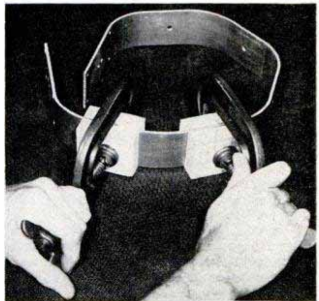
Above, the band is bent hexagonally by gripping with C-clamps and wooden pads. Below, holes for bulb sockets are cut in brackets with a coping saw
