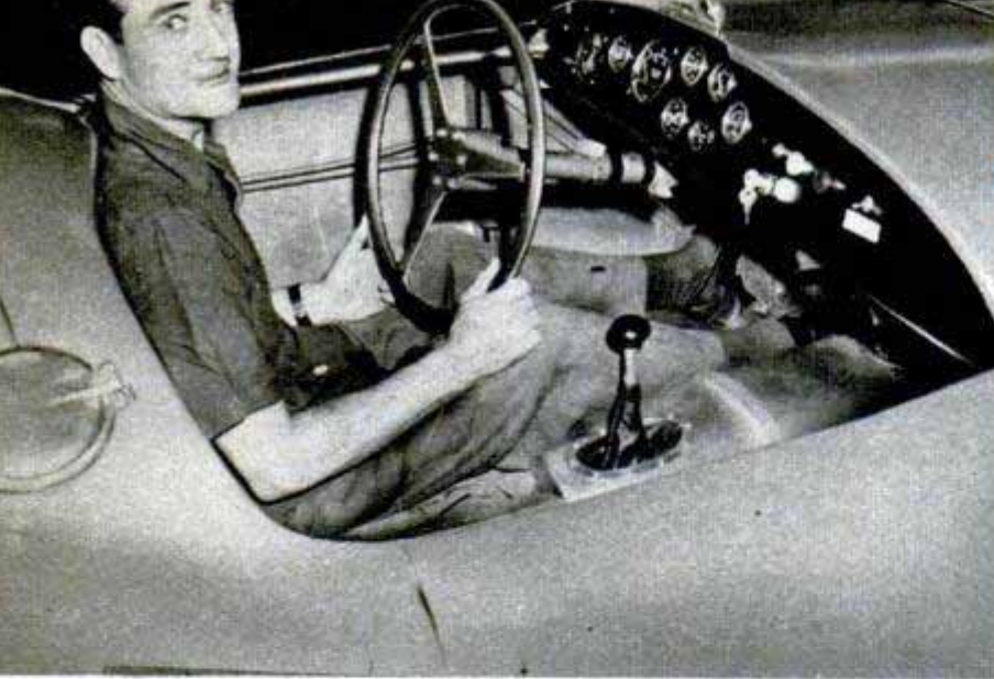
Briggs Cunningham sits in the cockpit of his new masterpiece, the C-4R. The safety steering wheel collapses in the event of a collision. Below, racing driver Phil Walters points to the cooling fins which force a stream of air over the brake drum
