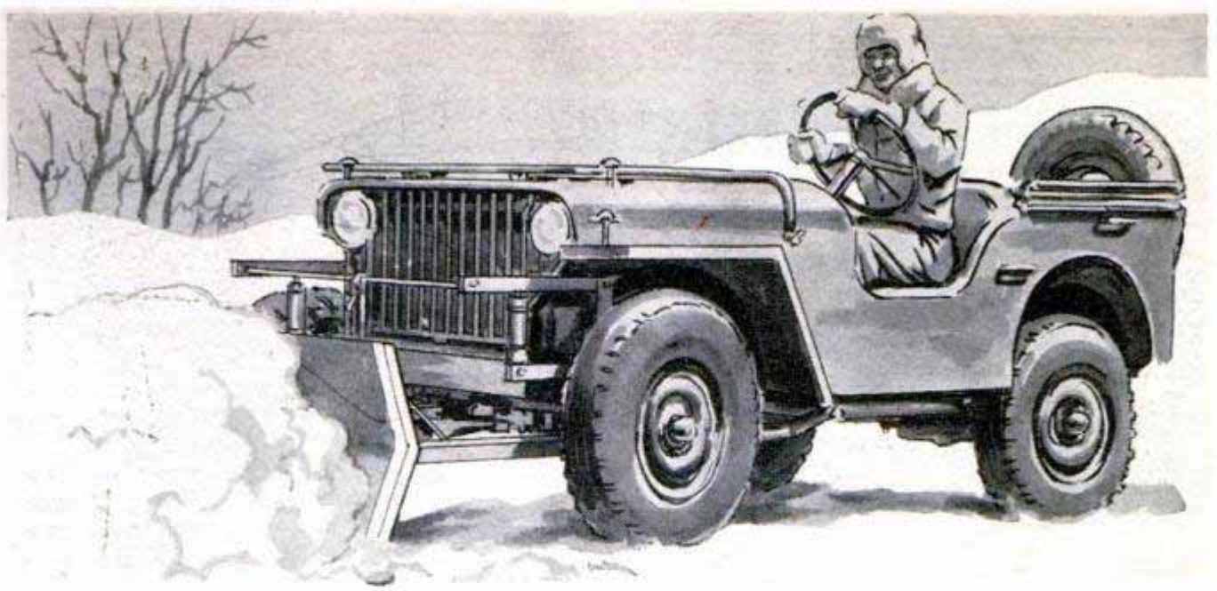
A Jeep or light truck fitted with this combination bulldozer-snowplow speeds up the job of clearing snow from driveways, feeding floors and farmyards. It also makes a fast, handy 'dozer for moving earth
