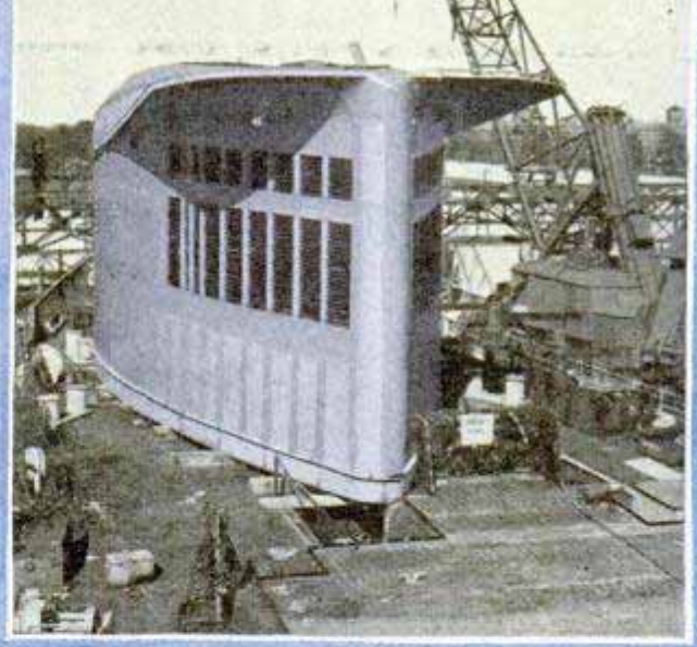
Forward stack measures a mighty 60 feet fore and aft, 55 feet high. Finlike projections prevent the smoke from swirling down to the deck. Cutaway at left shows how smoke ducts branch off into four huge dust-collecting drums
