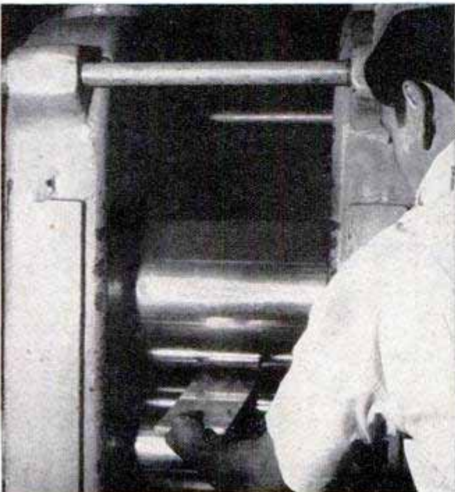
Silver ingot is forced between rollers which squeeze it out into a sheet of exactly the right thickness
