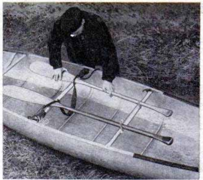
The oar blades are inserted under the tump-line and through copper-wire loops attached to the thwart. Shanks of the oars are lashed to the forward center thwart. In this position oars can be made to support all or part of the weight on the shoulders
