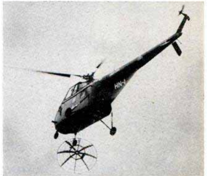
Helicopter, above, carries TV antenna to mountaintop relay point, below. Wing tank of jet plane, lower left, was adapted to sample air for radioactivity
